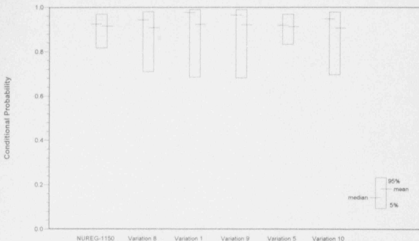
Figure 4.19 Conditional probability of avoiding containment failure for 24 hours in long-term blackouts with in-vessel FCIs included
