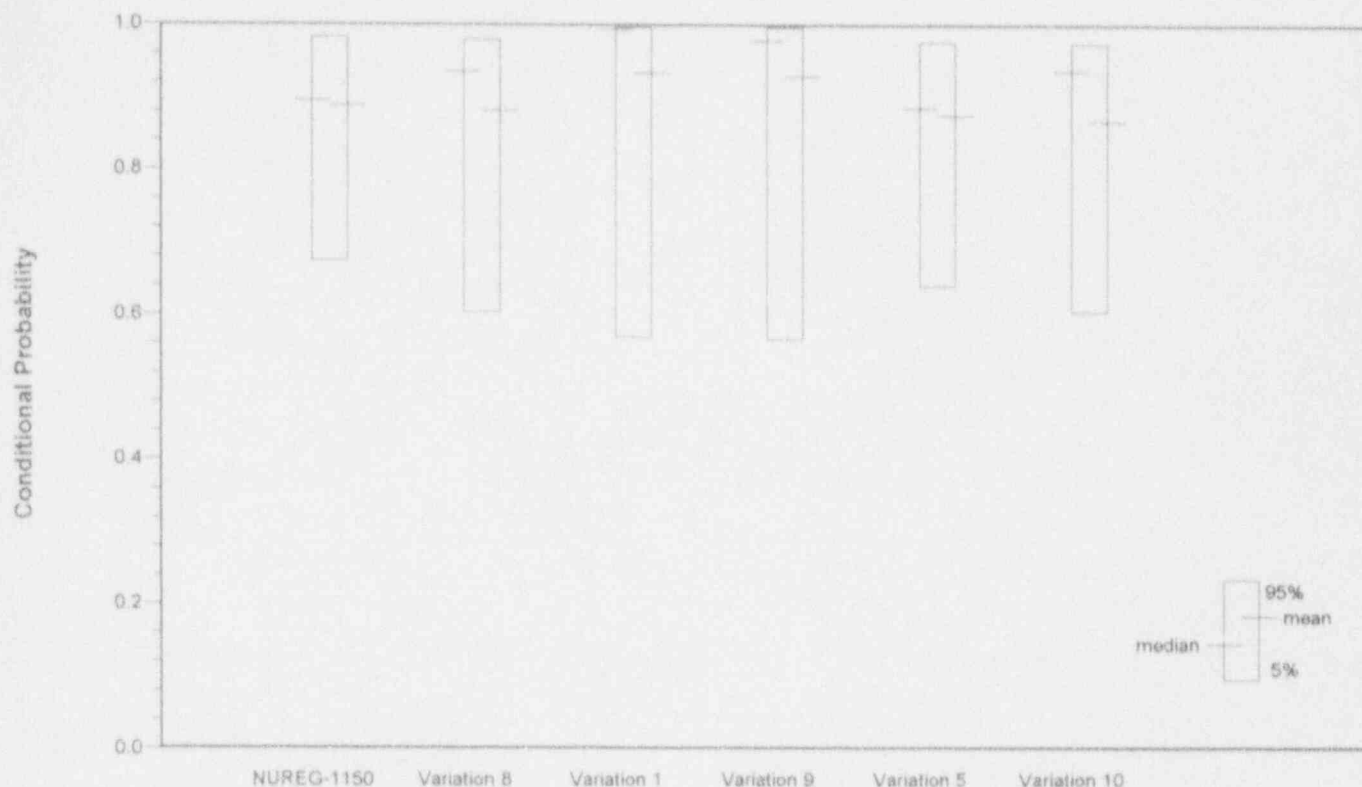
Figure 4.20 Conditional probability of avoiding containment failure for 24 hours in short-term blackouts with in-vessel FCIs included
