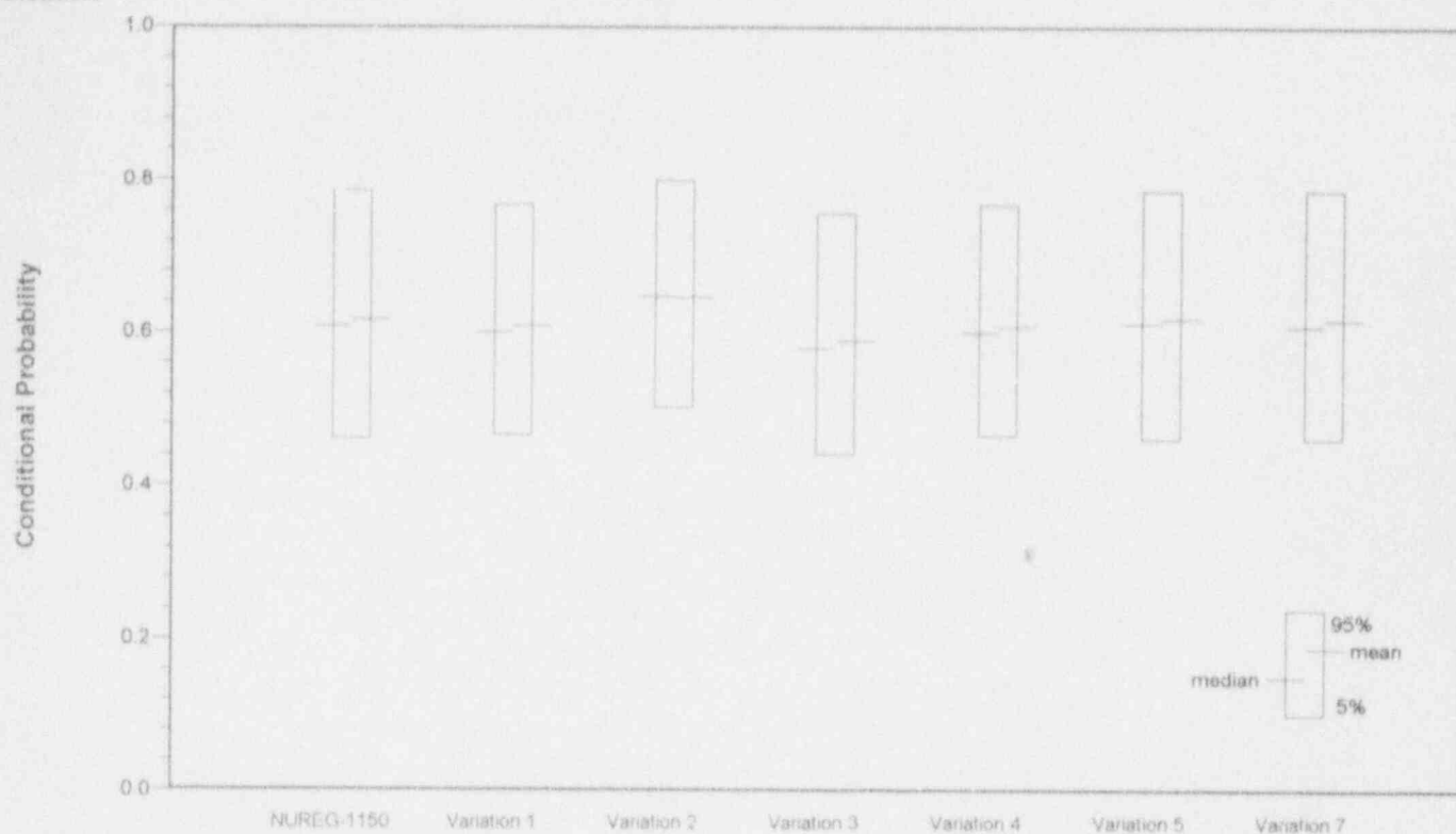
Figure 4.5 Conditional probability that core damage is arrested for long-term blackouts
