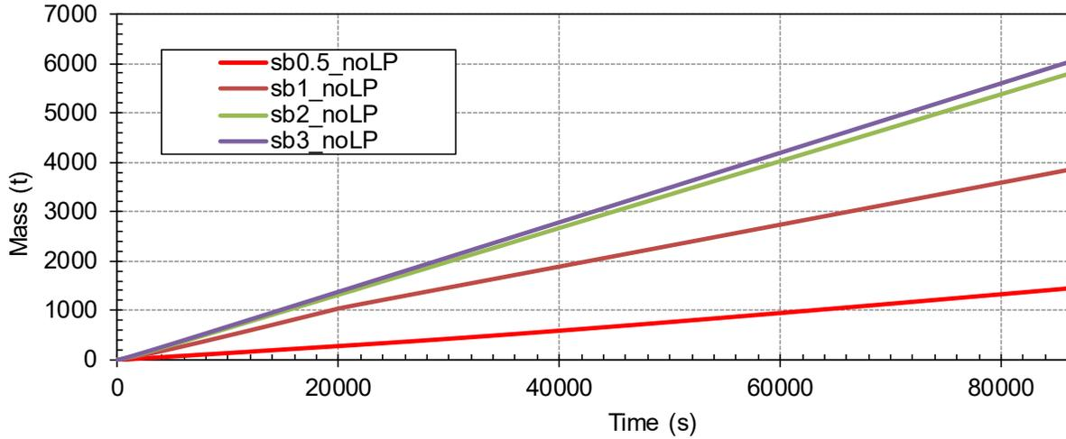
**Figure 3-26 Total Integrated HPIS Flow – noLP (1.27 cm to 7.62 cm)**
