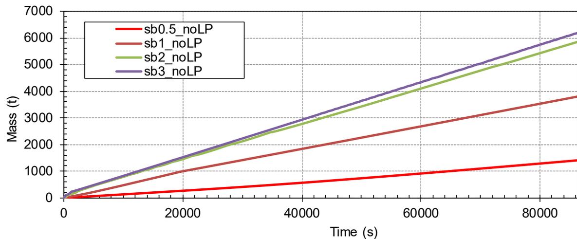
**Figure 3-24 Total Integrated Break Flow – noLP (1.27 cm to 7.62 cm)**
