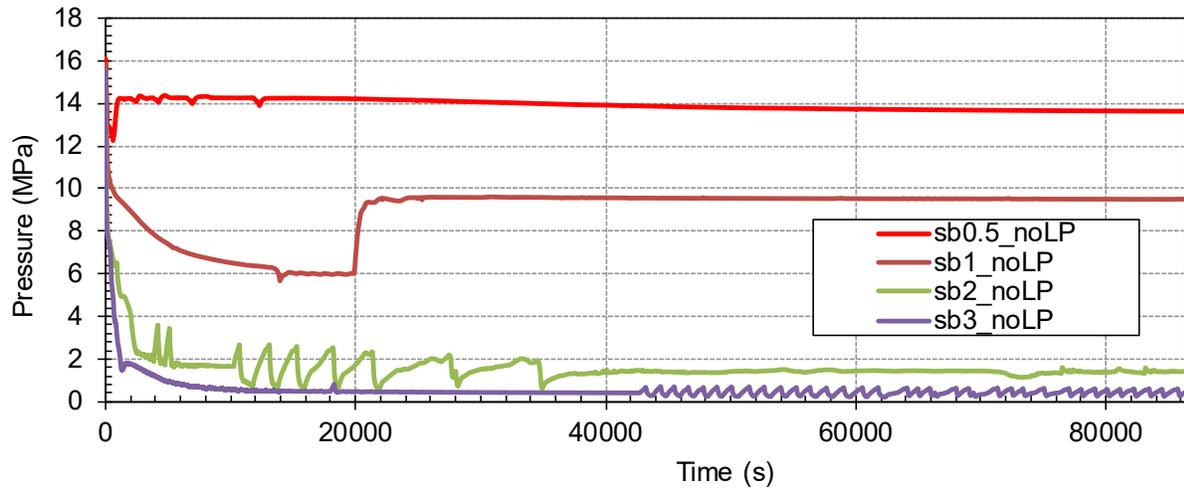
Figure 3-19 Pressurizer Pressure – noLP (1.27 cm to 7.62 cm)
