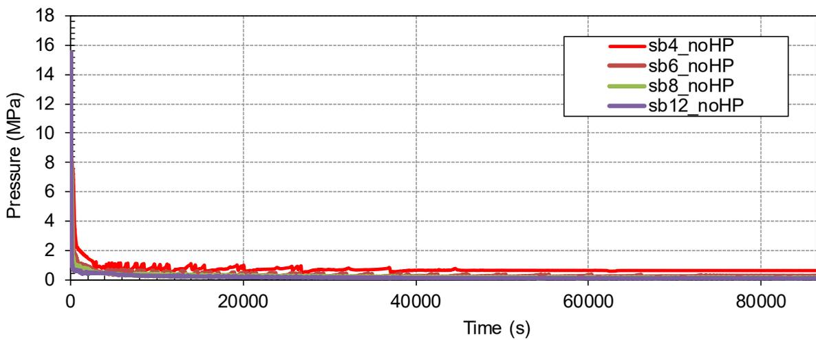
**Figure 3-10 Pressurizer Pressure – noHP (10.16 cm to 30.48 cm)**
