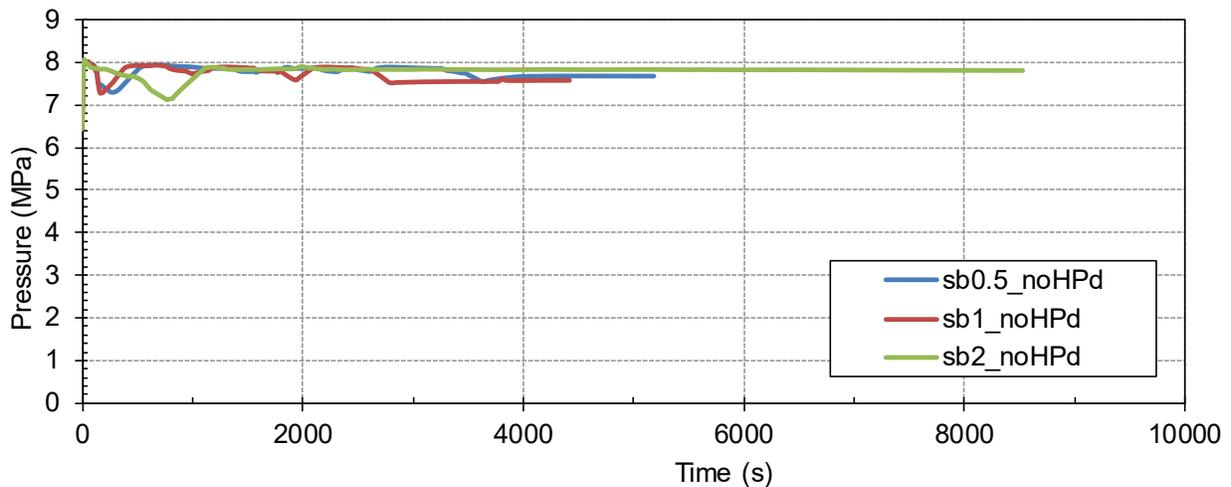
Figure 3-38 SG1 Pressure – noHP and AM1 (1.27 cm to 5.08 cm)
