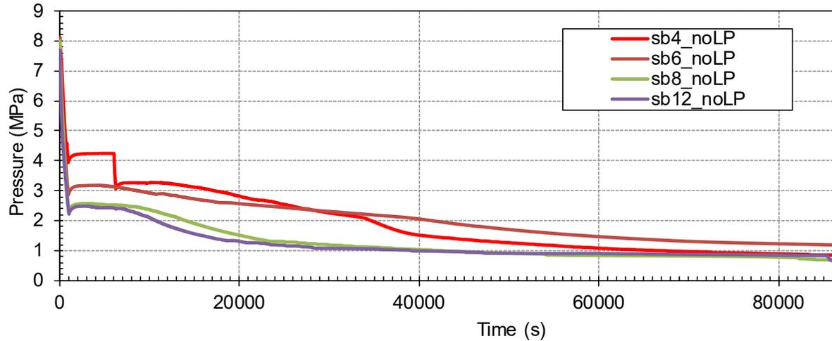
**Figure 3-29 SG1 Pressure – noLP (10.16 cm to 30.48 cm)**
