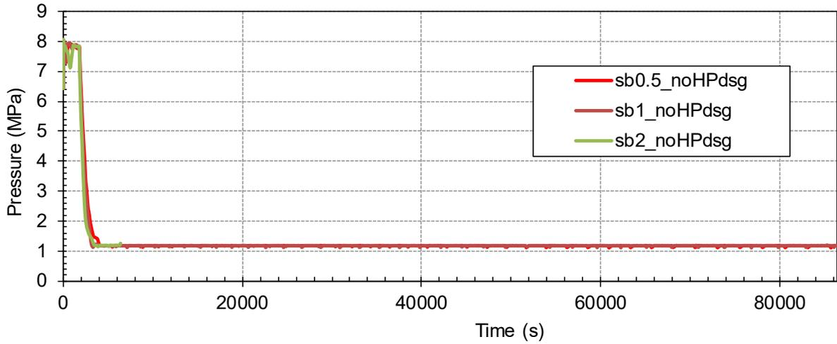
**Figure 3-47 SG1 Pressure – noHP and AM2 (1.27 cm to 5.08 cm)**
