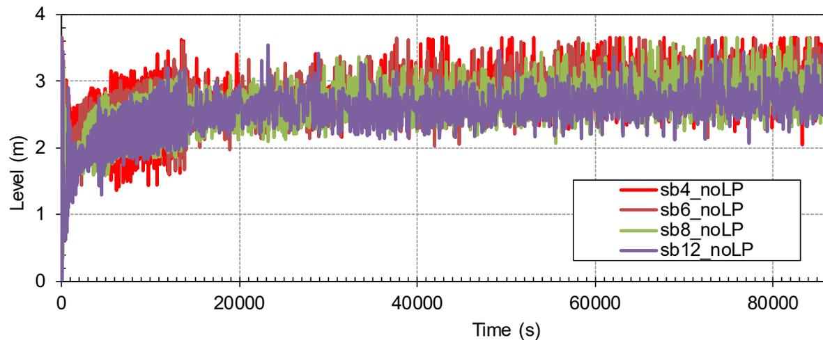
**Figure 3-30 Core Collapsed Liquid Level – noLP (10.16 cm to 30.48 cm)**
