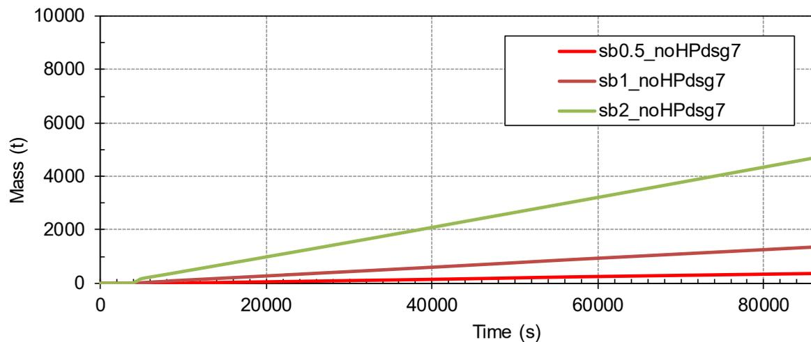
**Figure 3-60 Total Integrated Break Flow – noHP and AM3 (1.27 cm to 5.08 cm)**
