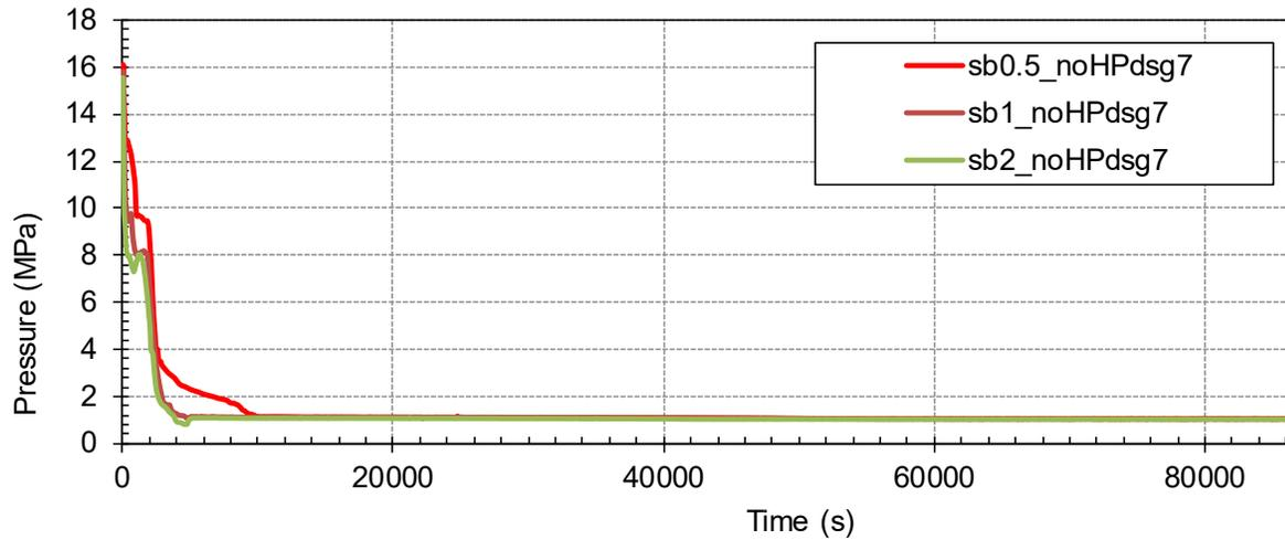
**Figure 3-55 Pressurizer Pressure – noHP and AM3 (1.27 cm to 5.08 cm)**
