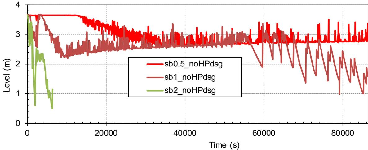
**Figure 3-48 Core Collapsed Liquid Level – noHP and AM2 (1.27 cm to 5.08 cm)**
