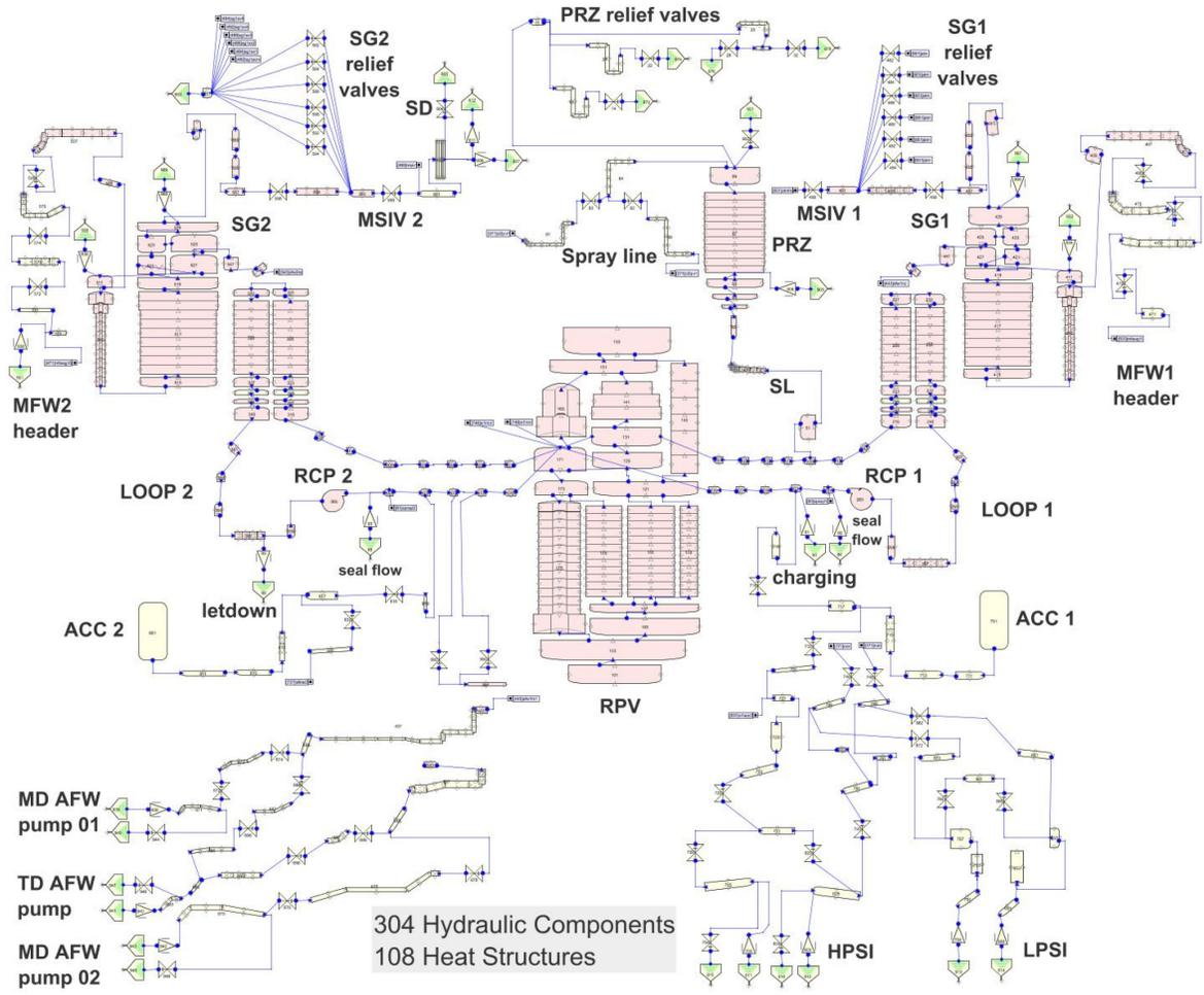
**Figure 2-1 RELAP5 Krško NPP Hydraulic Components View**
