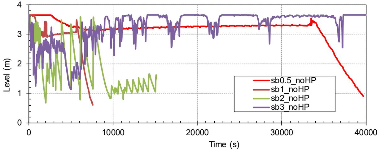
Figure 3-3 Core Collapsed Liquid Level – noHP (1.27 cm to 7.62 cm)
