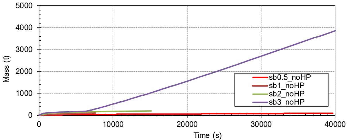
**Figure 3-6 Total Integrated Break Flow – noHP (1.27 cm to 7.62 cm)**
