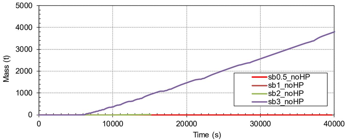
**Figure 3-9 Total Integrated LPIS Flow – noHP (1.27 cm to 7.62 cm)**
