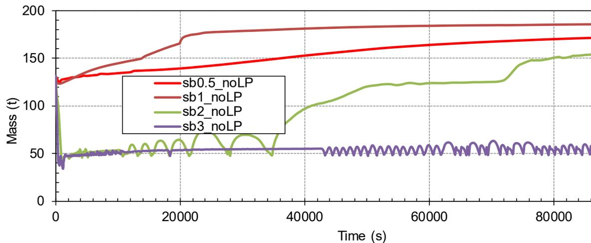
**Figure 3-23 Primary System Mass – noLP (1.27 cm to 7.62 cm)**
