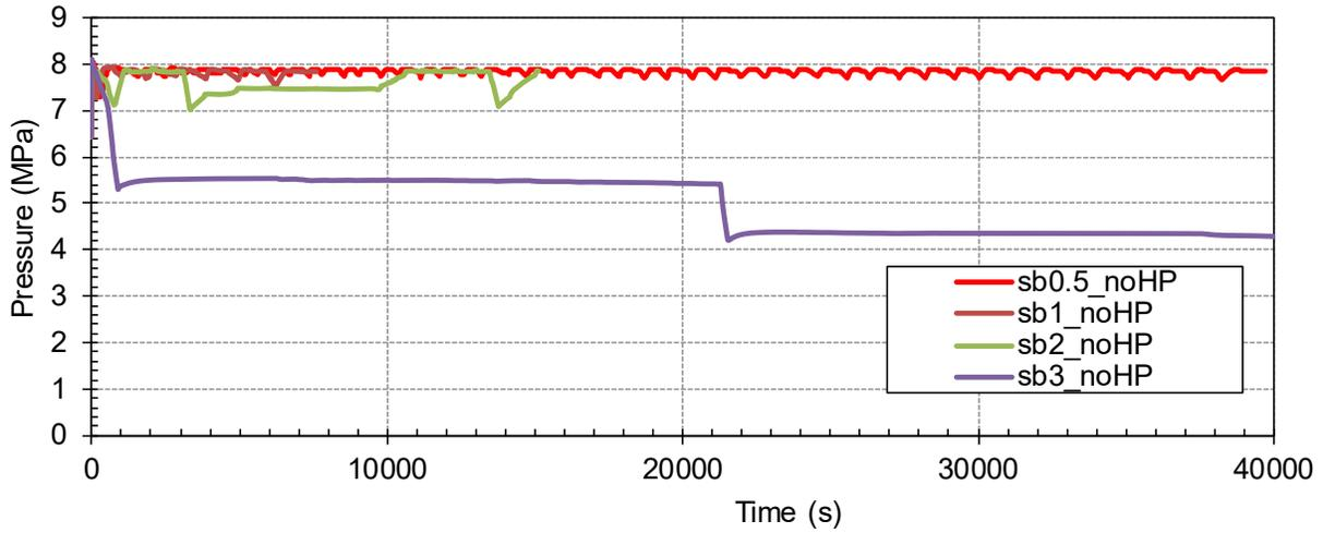
Figure 3-2 SG1 Pressure – noHP (1.27 cm to 7.62 cm)
