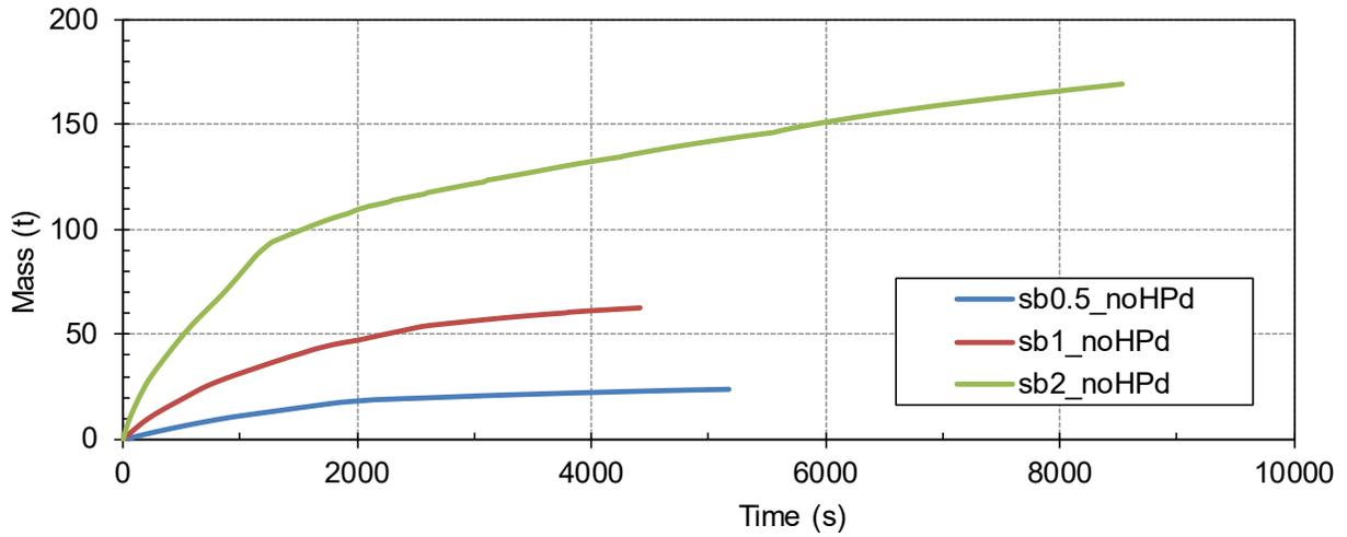
**Figure 3-42 Total Integrated Break Flow – noHP and AM1 (1.27 cm to 5.08 cm)**
