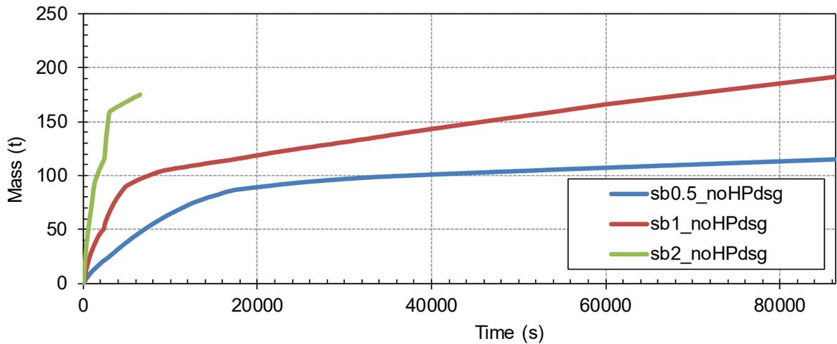
**Figure 3-51 Total Integrated Break Flow – noHP and AM2 (1.27 cm to 5.08 cm)**
