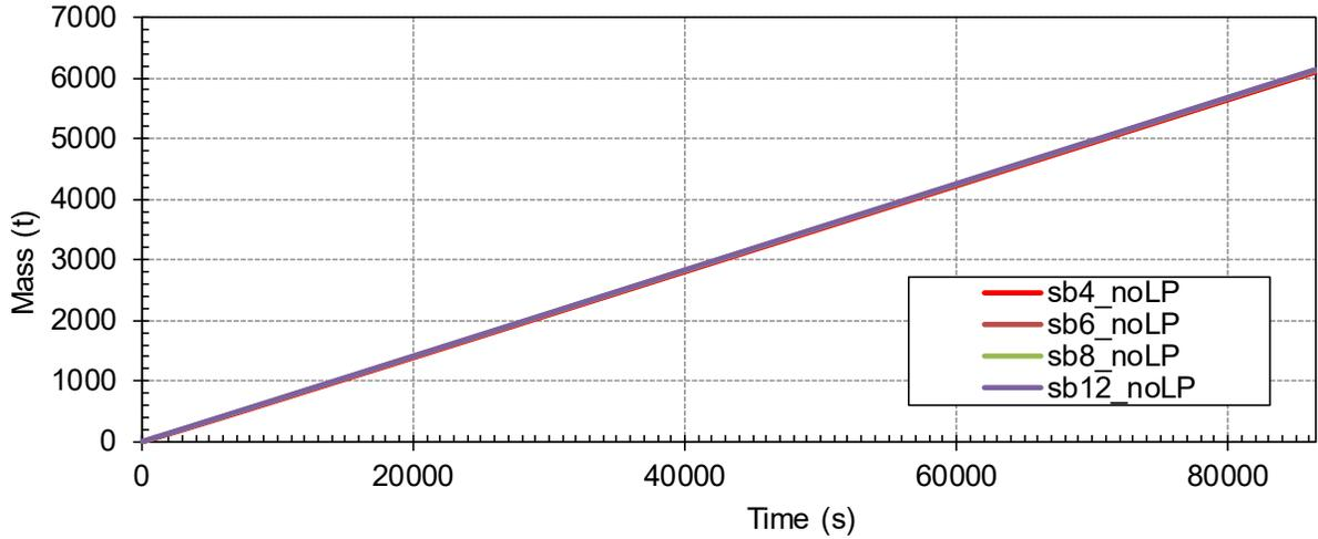
**Figure 3-35 Total Integrated HPIS Flow – noLP (10.16 cm to 30.48 cm)**
