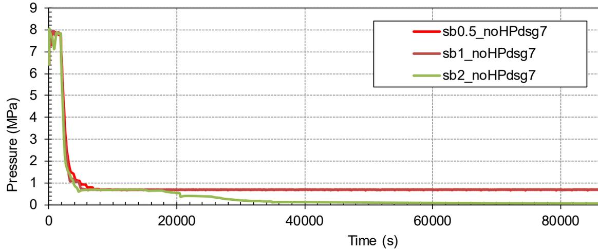
**Figure 3-56 SG1 Pressure – noHP and AM3 (1.27 cm to 5.08 cm)**
