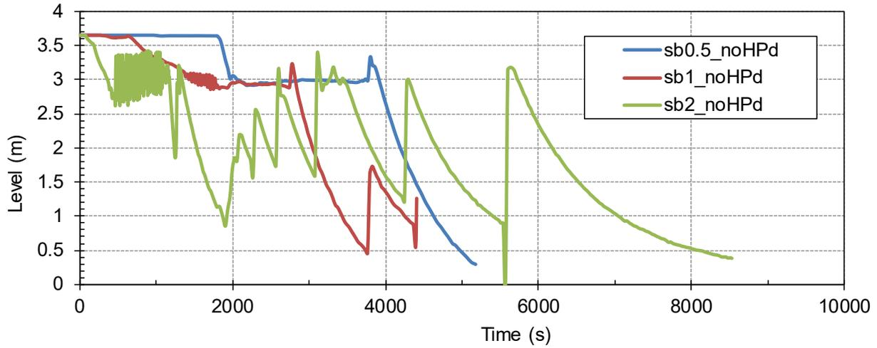
**Figure 3-39 Core Collapsed Liquid Level – noHP and AM1 (1.27 cm to 5.08 cm)**
