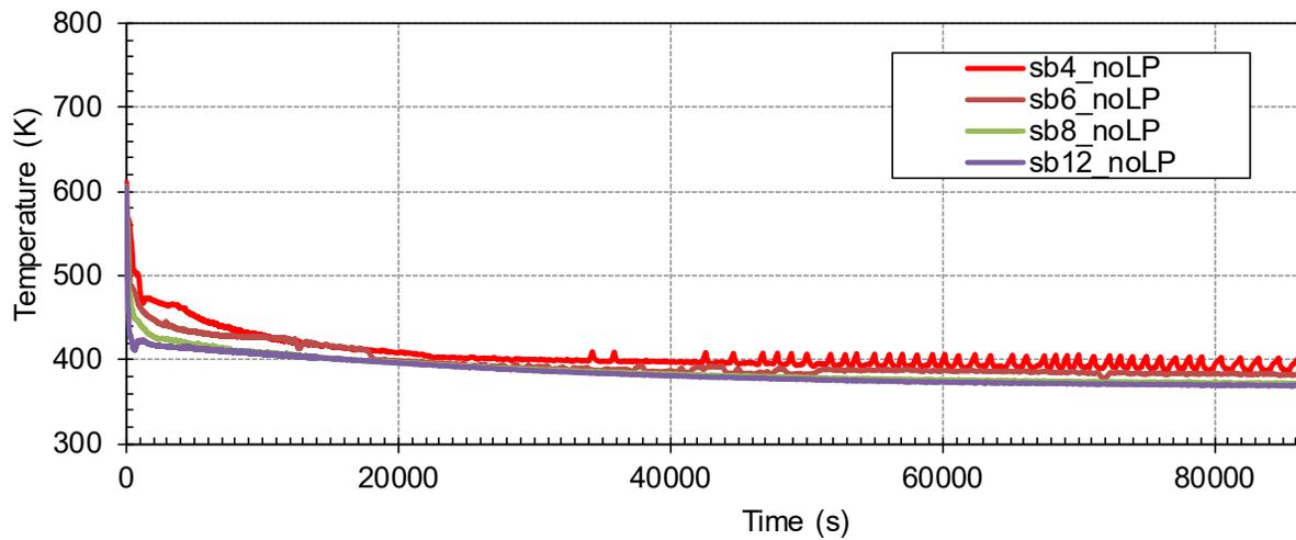
**Figure 3-31 Cladding Temperature – noLP (10.16 cm to 30.48 cm)**
