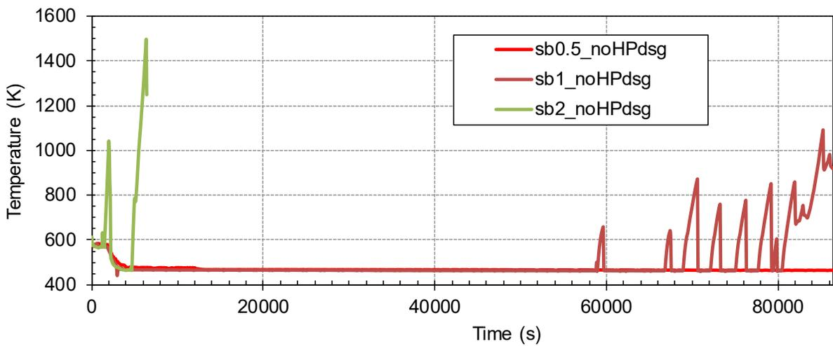
**Figure 3-49 Cladding Temperature – noHP and AM2 (1.27 cm to 5.08 cm)**
