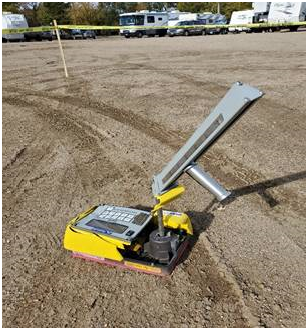
Figure 2 – The damaged Troxler Model 3430, S/N 73136. Visible in the picture are the boundaries put up by the gauge user following the damaging of the gauge and the skid-steer tire tracks. The gray and angled portion of the gauge is the index rod, and the cesium-137 source rod is the vertical portion beneath the index rod, with the bottom portion within the shielded block.
