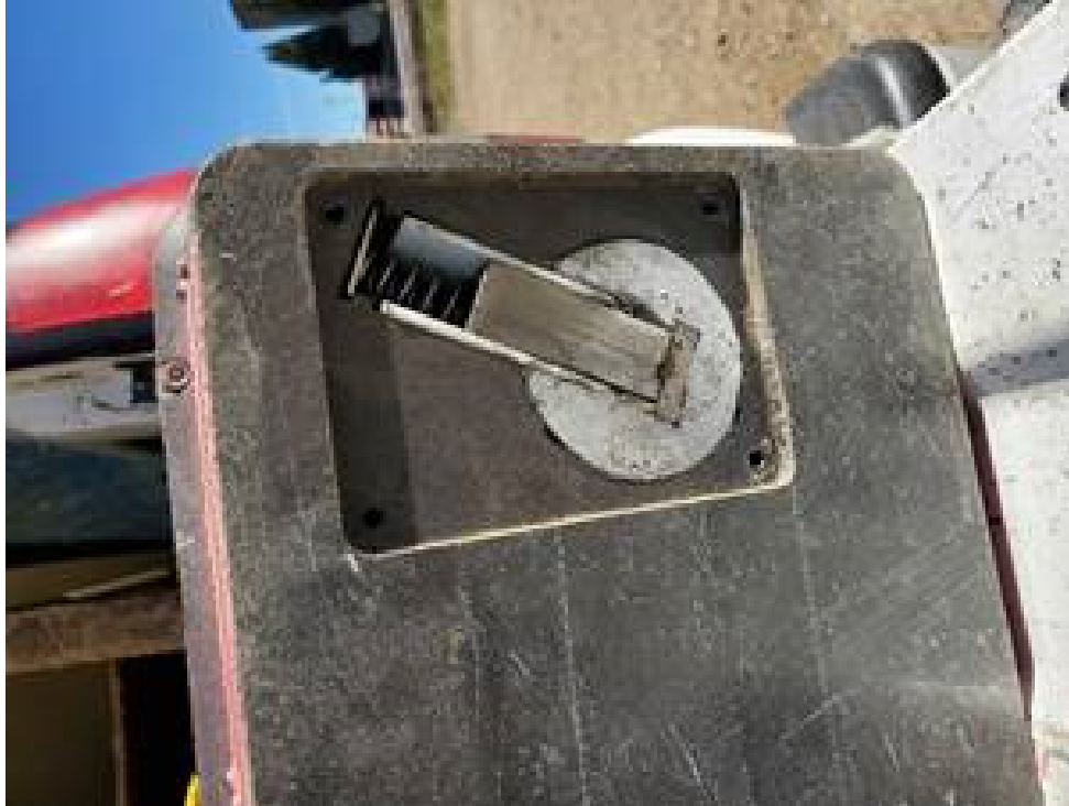
Figure 3 – The bottom of the Troxler Model 3430, with the bottom plate removed to show the sliding block. In this figure, the sliding block is in the fully closed and shielded position.
