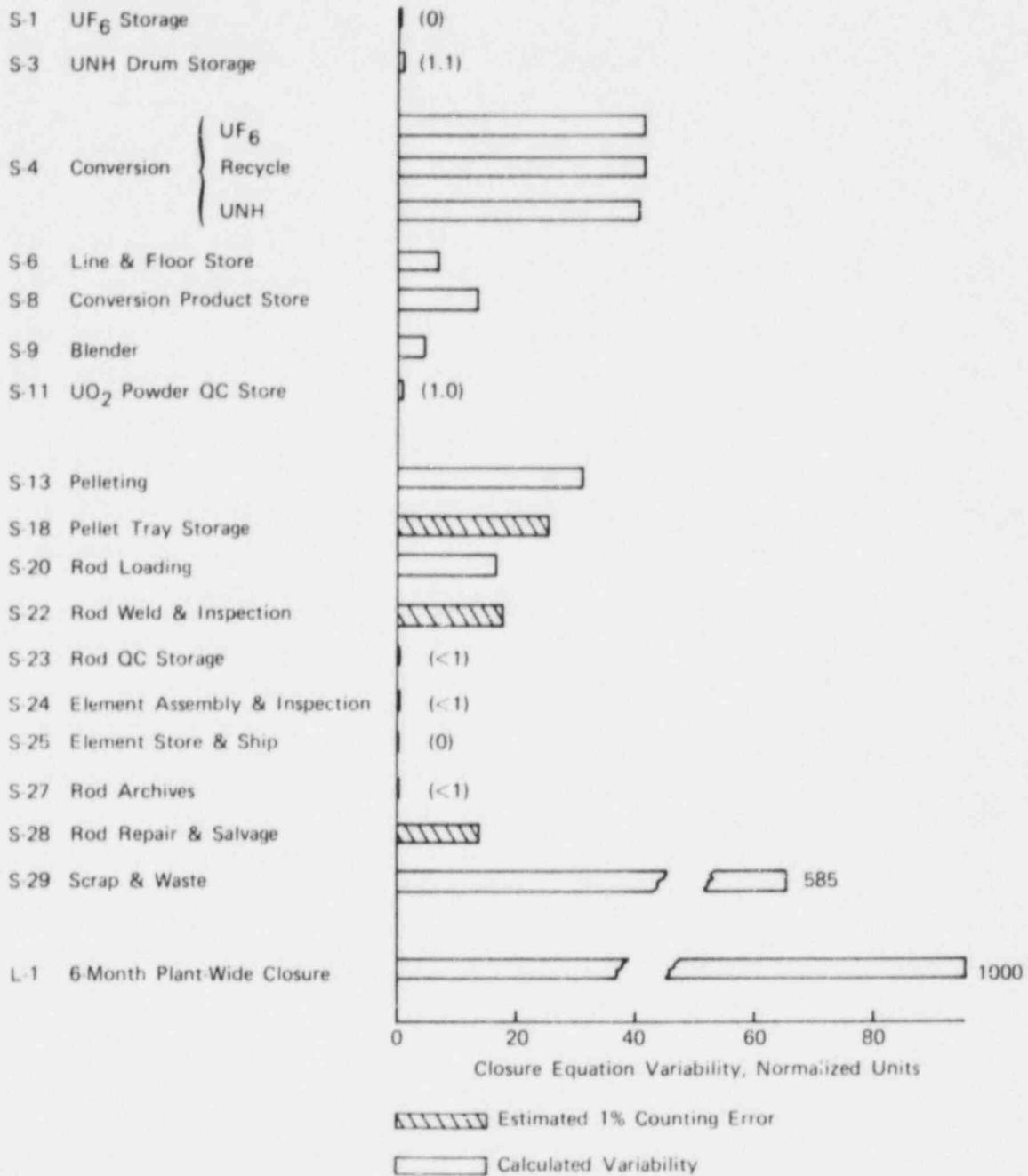
FIGURE 5.2 - Comparison of model-based closure equation variability (2σ normalized units).
