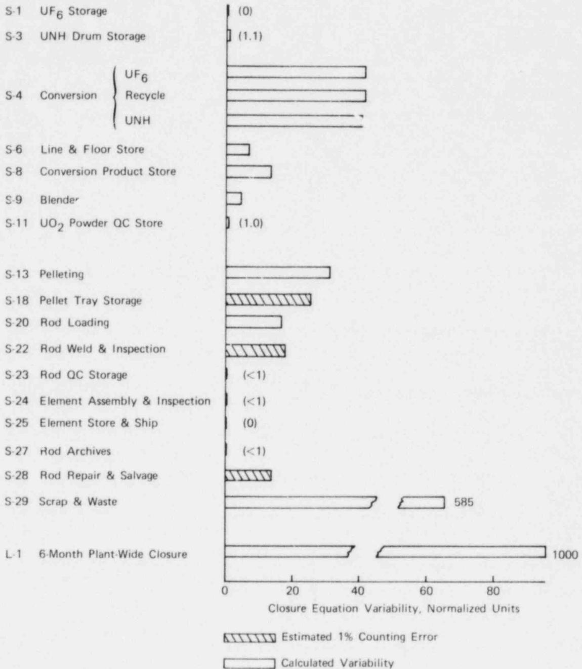
FIGURE 2 - Comparison of model-based closure equation variabilities (2σ normalized units).
