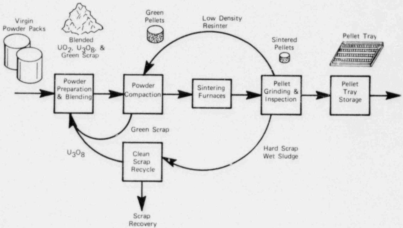
FIGURE A-3 - Flow diagram of UO<sub>2</sub> pelleting operation.
