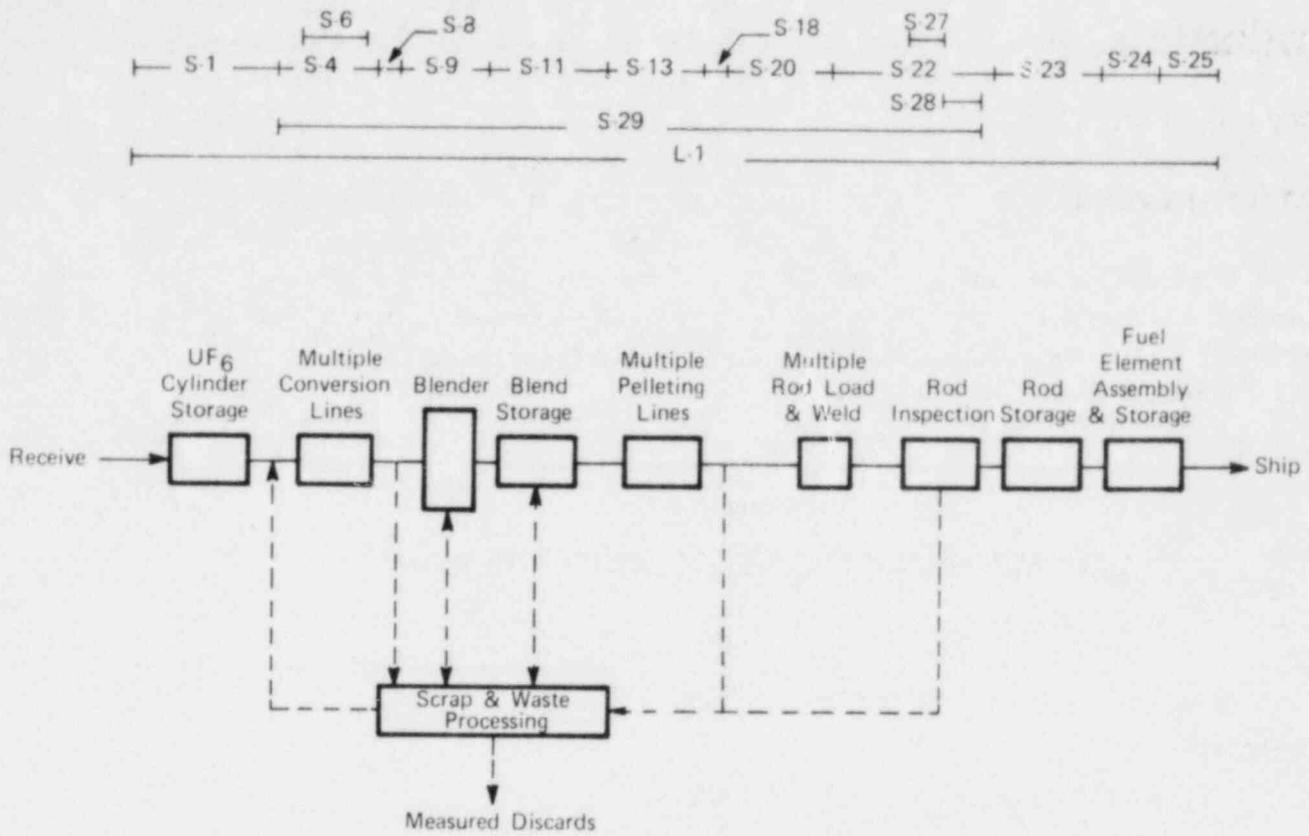
FIGURE E-1 - Process flow diagram showing plant-wide closure equations.
