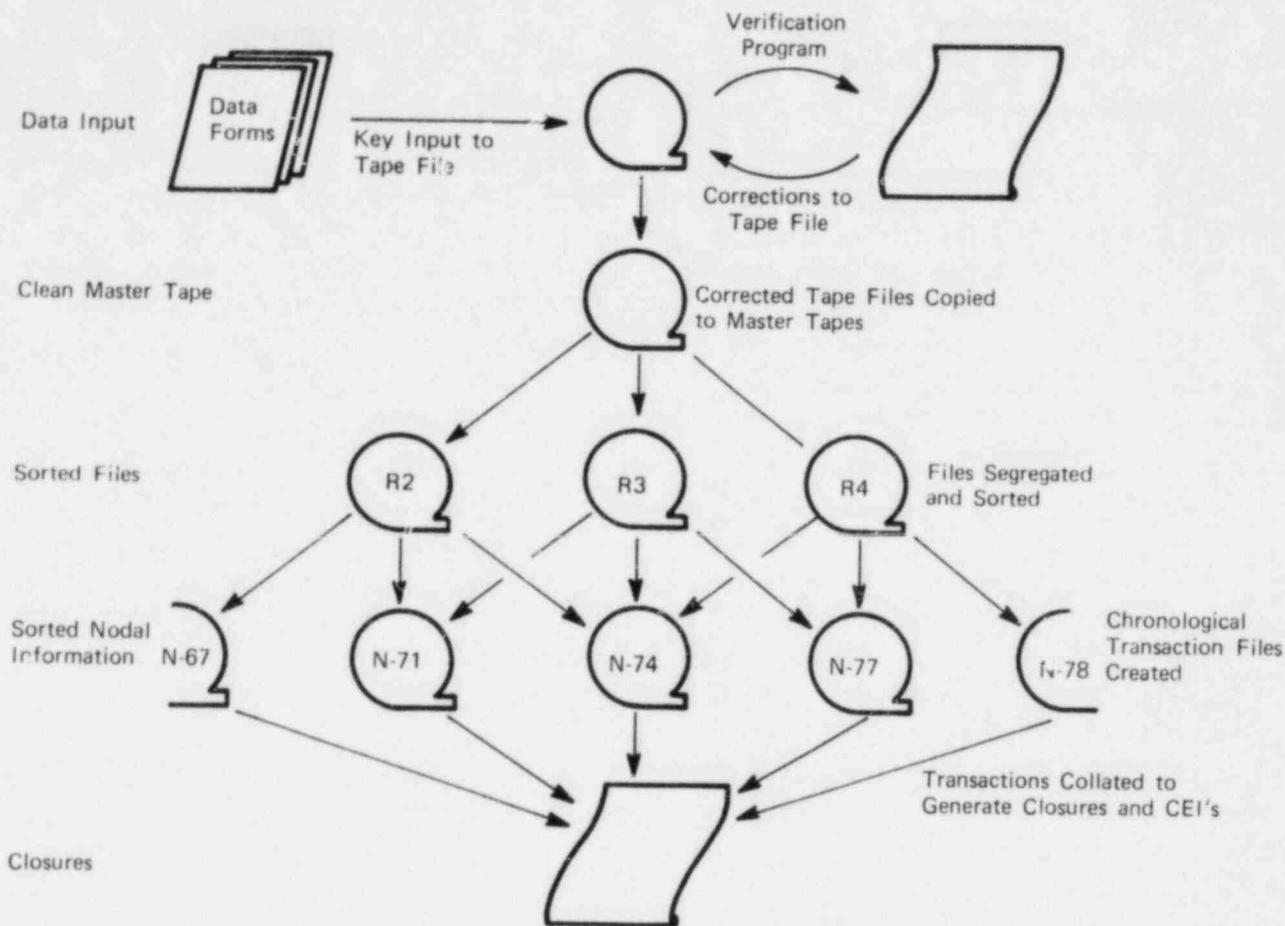
FIGURE C-1 - Scheme for generation of equation closures from process data sheets.
