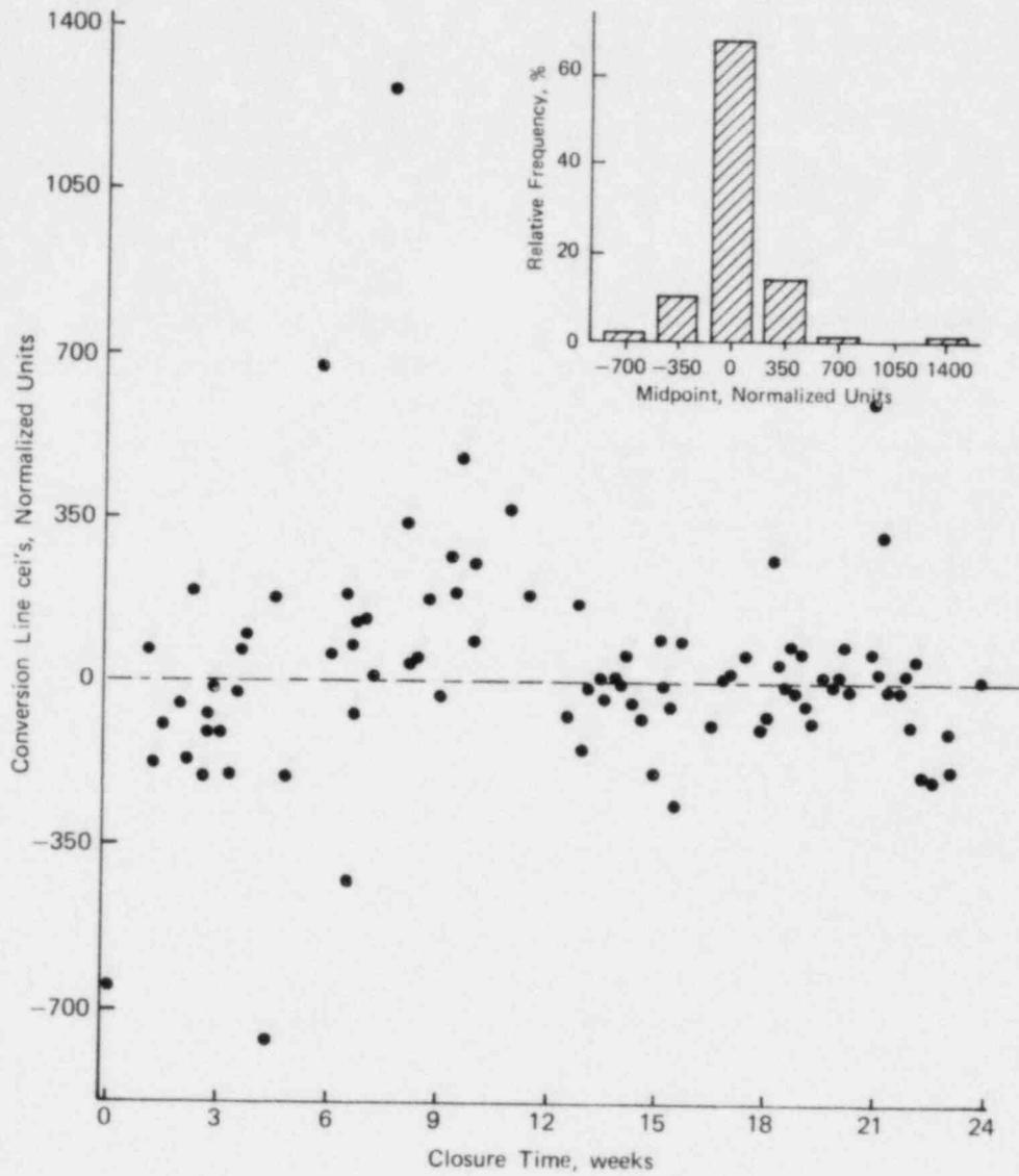
FIGURE 6.2.4 - Typical cei's for uncorrected conversion line closures.
