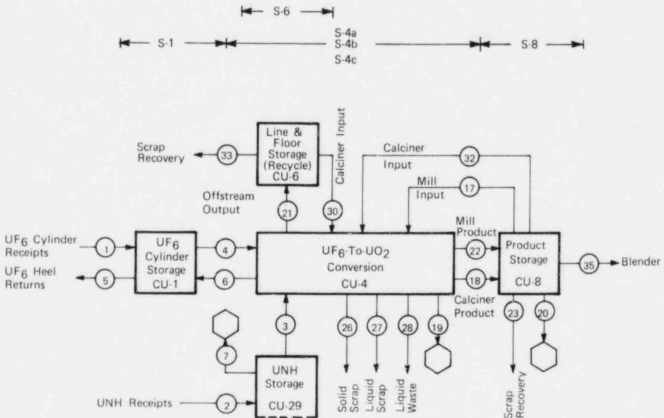
FIGURE 6.2.1 - Control units and closure equations for each conversion line.
