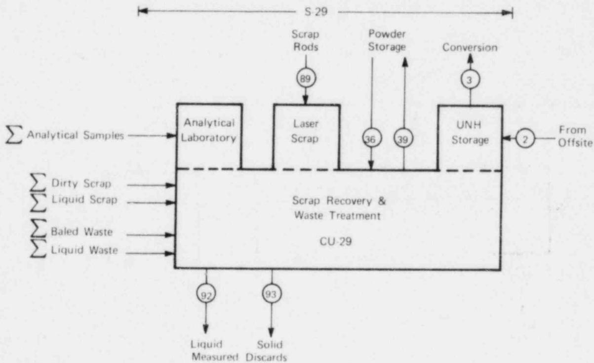
FIGURE E-6 - Control unit and closure equation for scrap recovery and waste processing facility.
