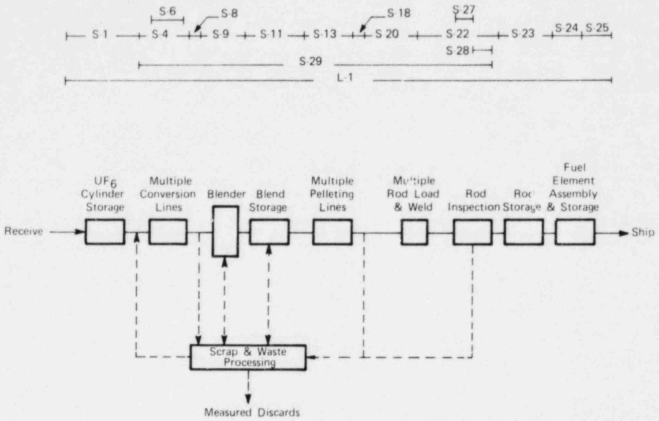
FIGURE 5.1 - Process flow diagram showing plant-wide closure equation network.
