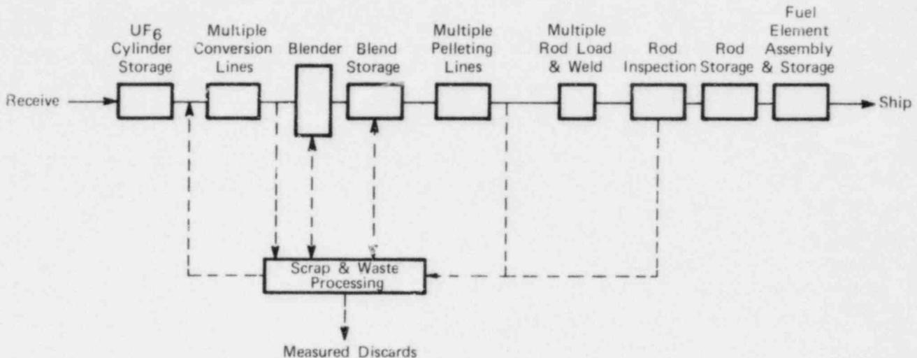
FIGURE 1 - Flow diagram of low-enrichment uranium fuel process showing spans of closure equations.
