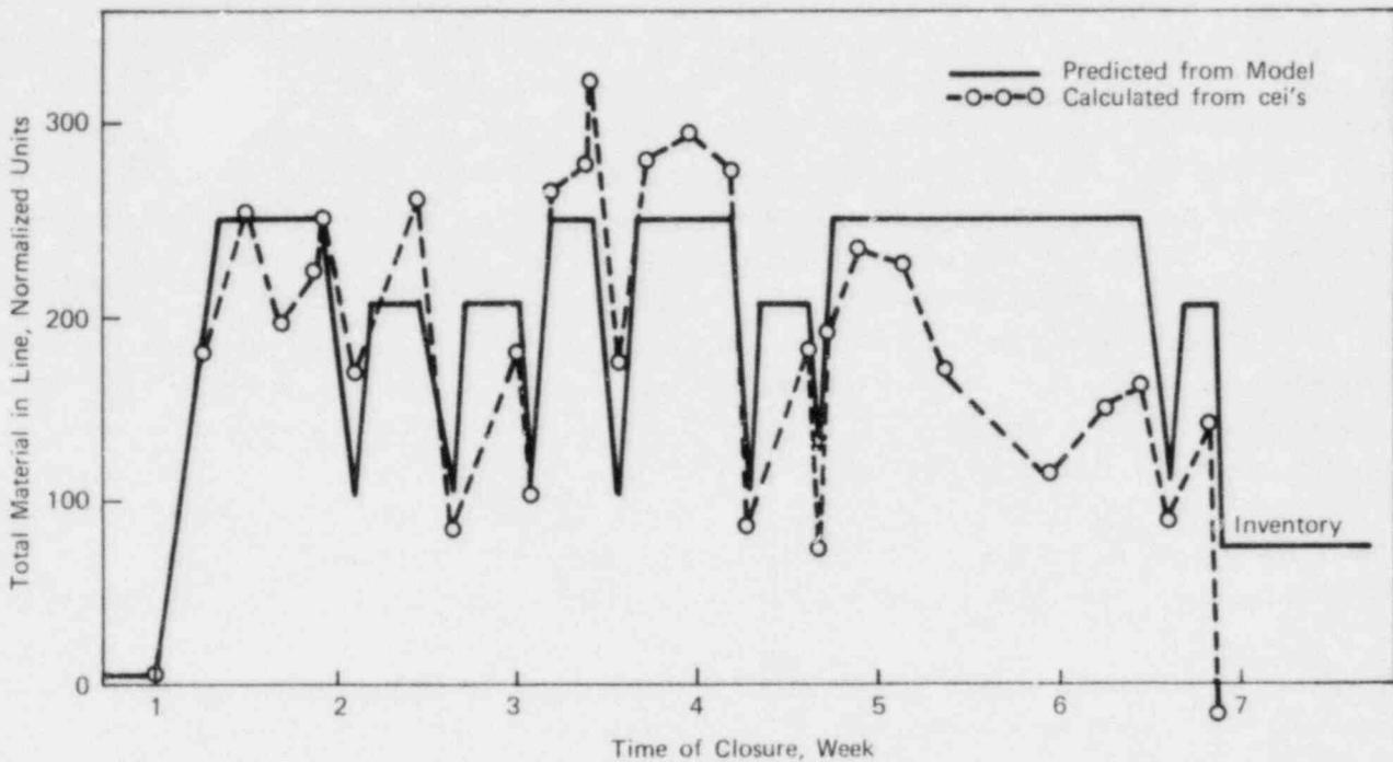
FIGURE 4 - Comparison of data-based conversion line in-process quantities with expected quantities based on the process model.
