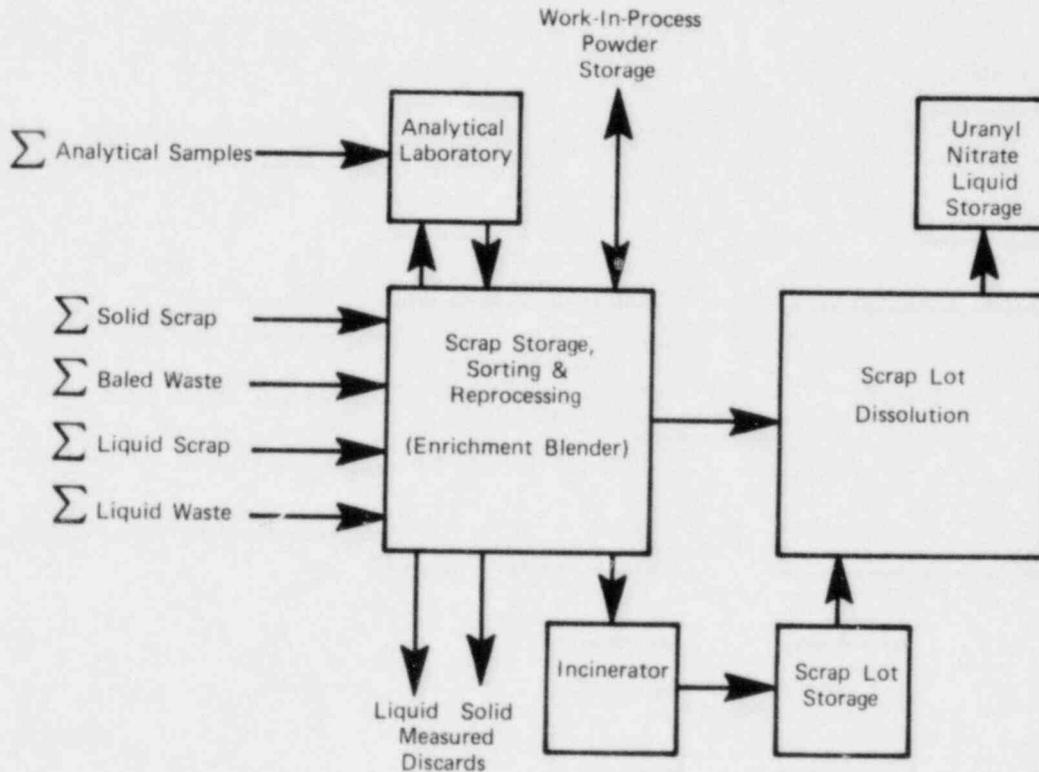
FIGURE A-6 - Flow diagram of scrap recovery and waste processing operations.
