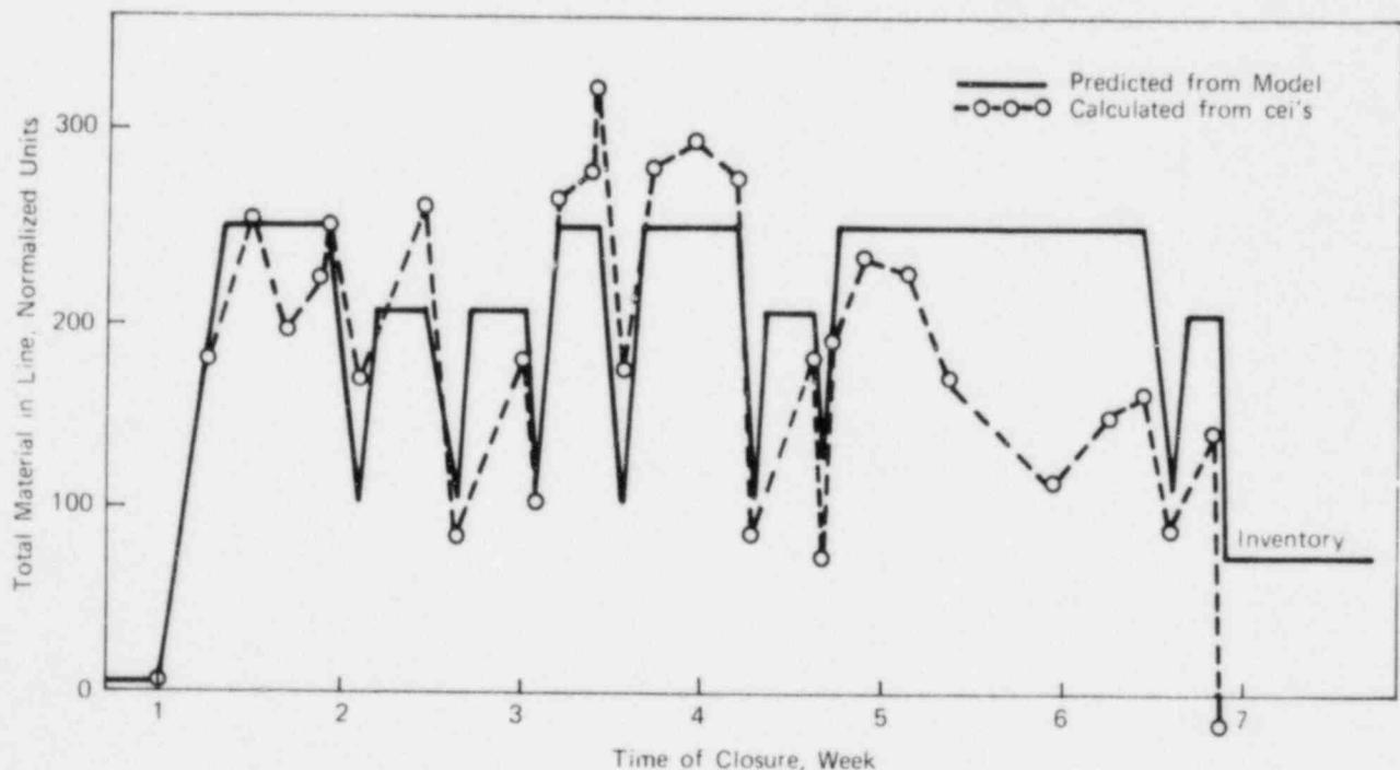
FIGURE 6.2.6 - Comparison of data-based conversion line in-process quantities with expected quantities based on the process model.
