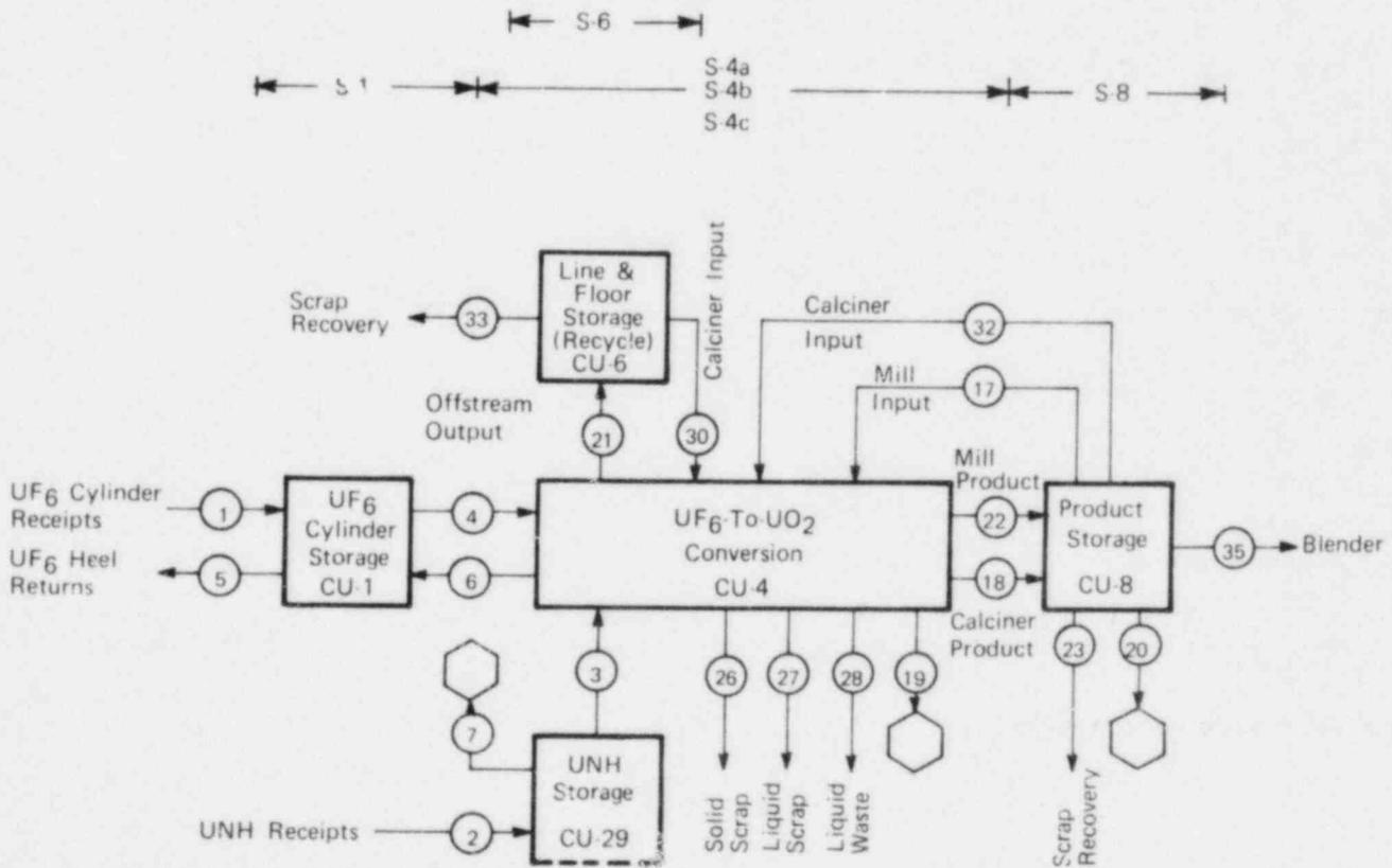
FIGURE E-2 - Control units and closure equations for each conversion line.
