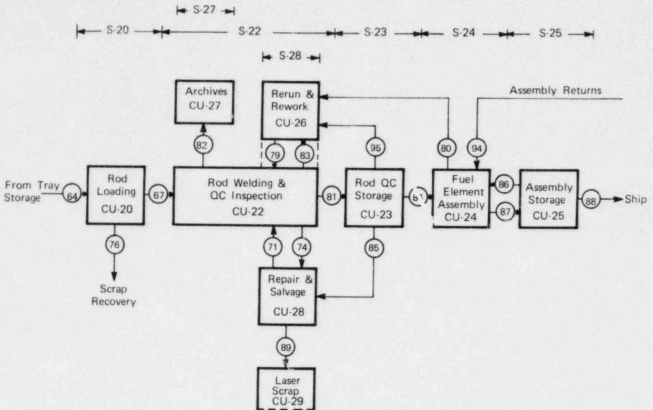
FIGURE 6.5.1 - Control units and closure equations for fuel rod fabrication and fuel element assembly.
