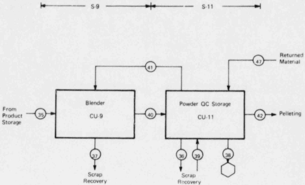
FIGURE E-3 - Control units and closure equations for blender, powder QC storage, and experimental conversion process.
