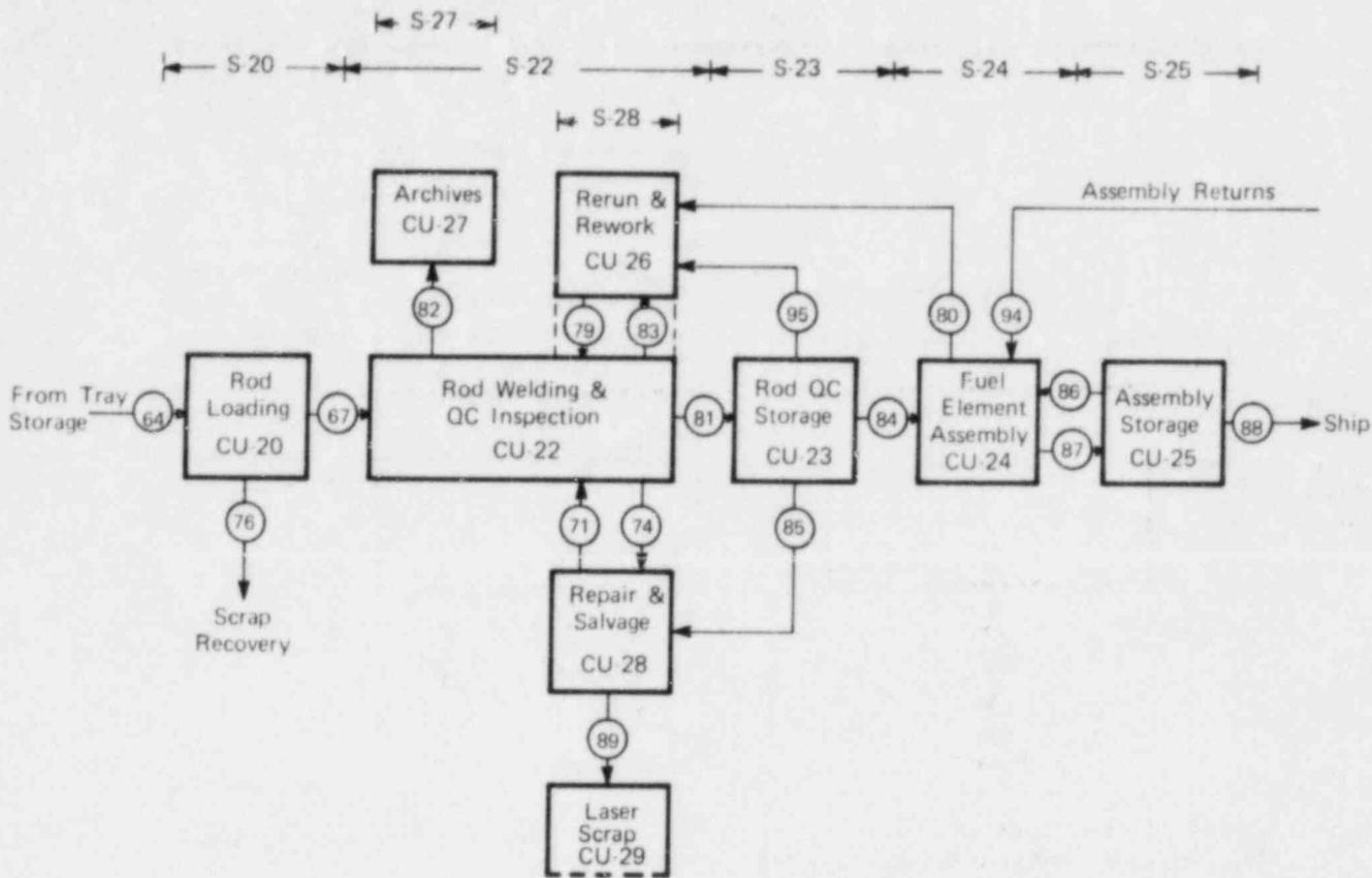
FIGURE E-5 - Control units and closure equations for rod fabrication and element assembly.
