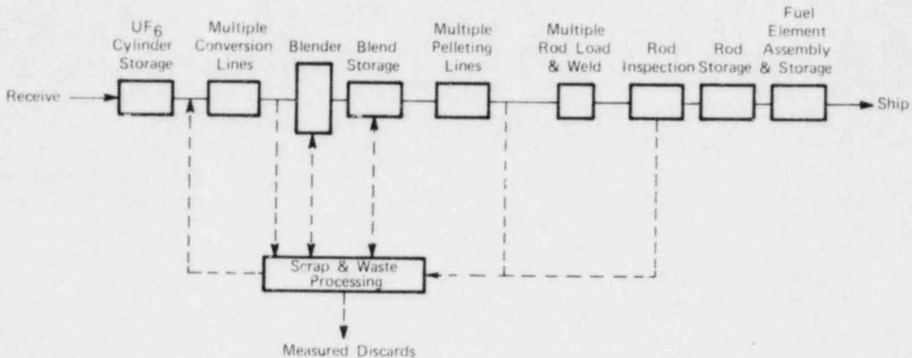
FIGURE 3-1 -low diagram of low-enrichment uranium fuel plant.
