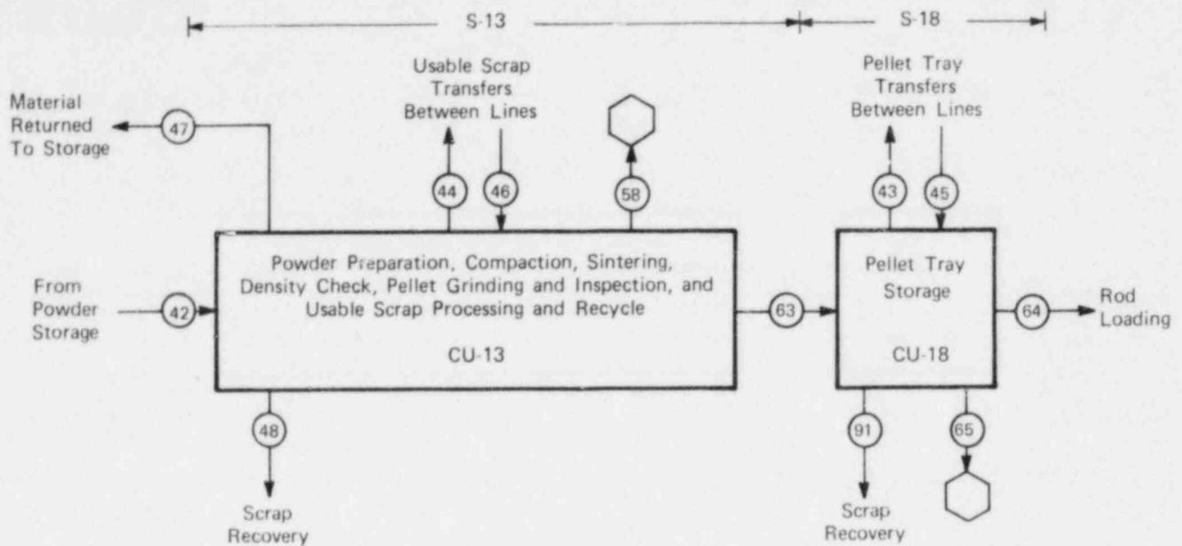
FIGURE 6.4.1 - Control units and closure equations for pelleting lines.
