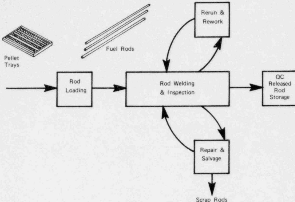
FIGURE A-4 - Flow diagram of fuel rod fabrication and inspection operations.
