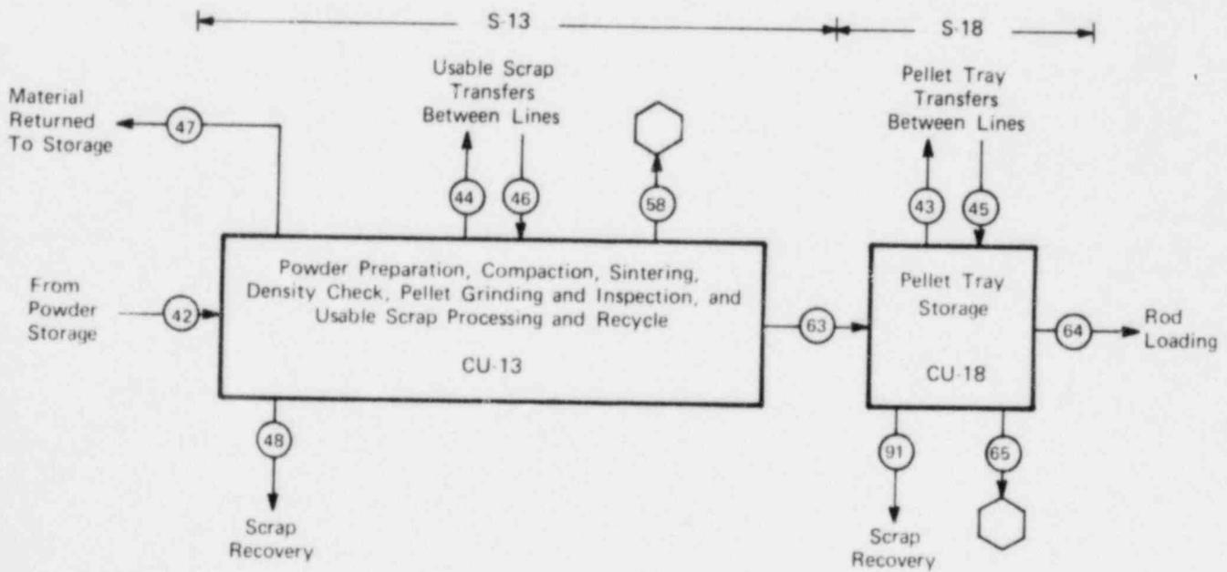
FIGURE E-4 - Control units and closure equations for pelleting lines.
