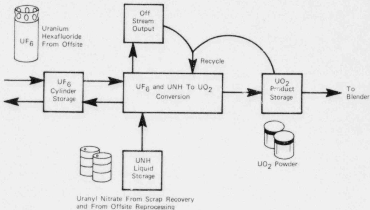
FIGURE A-1 - Flow diagram of conversion operations.
