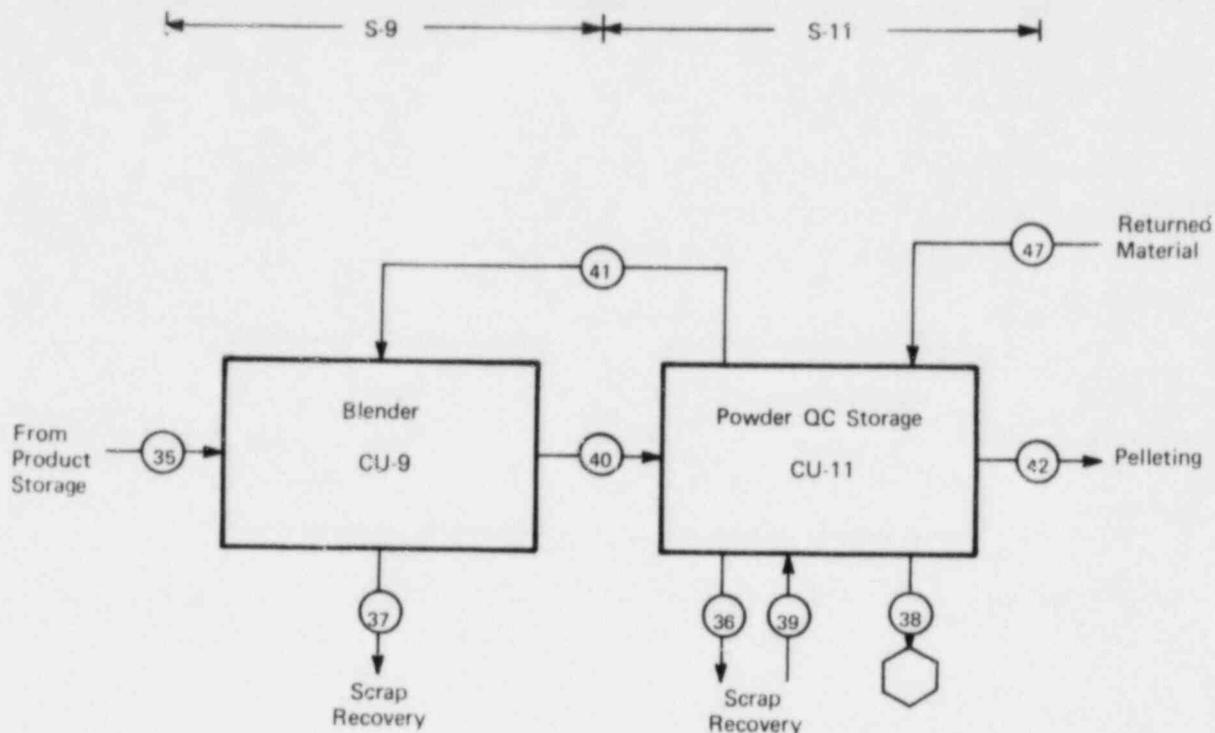
FIGURE 6.3.1 - Control units and closure equations for blender and powder QC storage.
