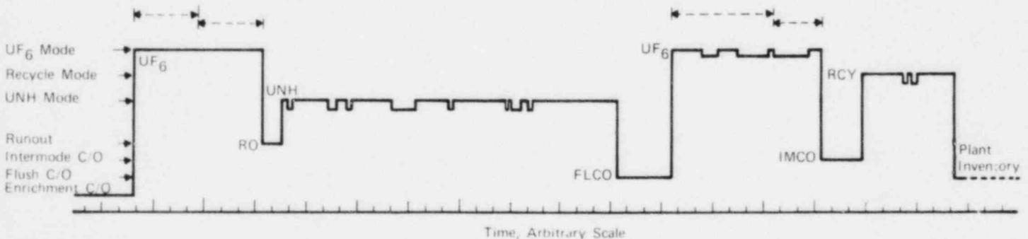
FIGURE 6.2.3 - Conversion line operational profile. (Small indentations in profile indicate temporary line shutdown; dashed lines indicate times individual UF<sub>6</sub> cylinders are on-line.)
