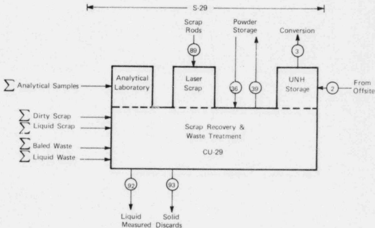
FIGURE 6.6.1 - Control unit and closure equation for scrap recovery and waste processing facility.
