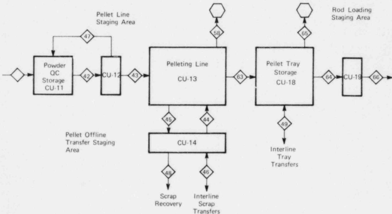
FIGURE 6.4.3 - Revised control units for pelleting lines.
