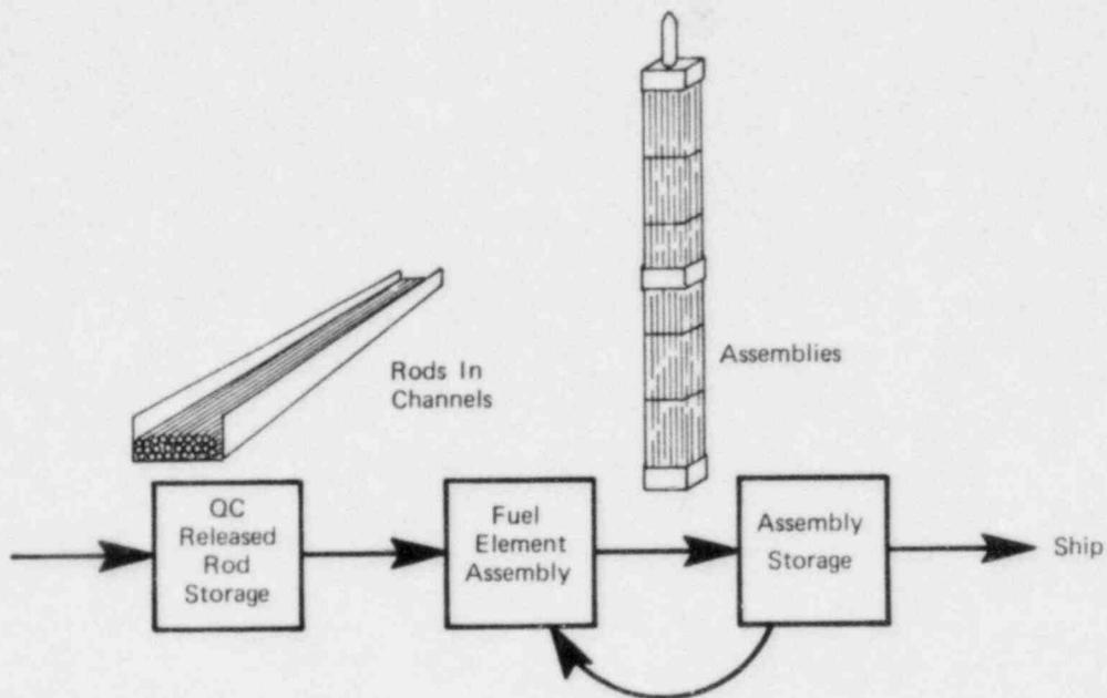
FIGURE A-5 - Flow diagram of fuel element assembly operations.
