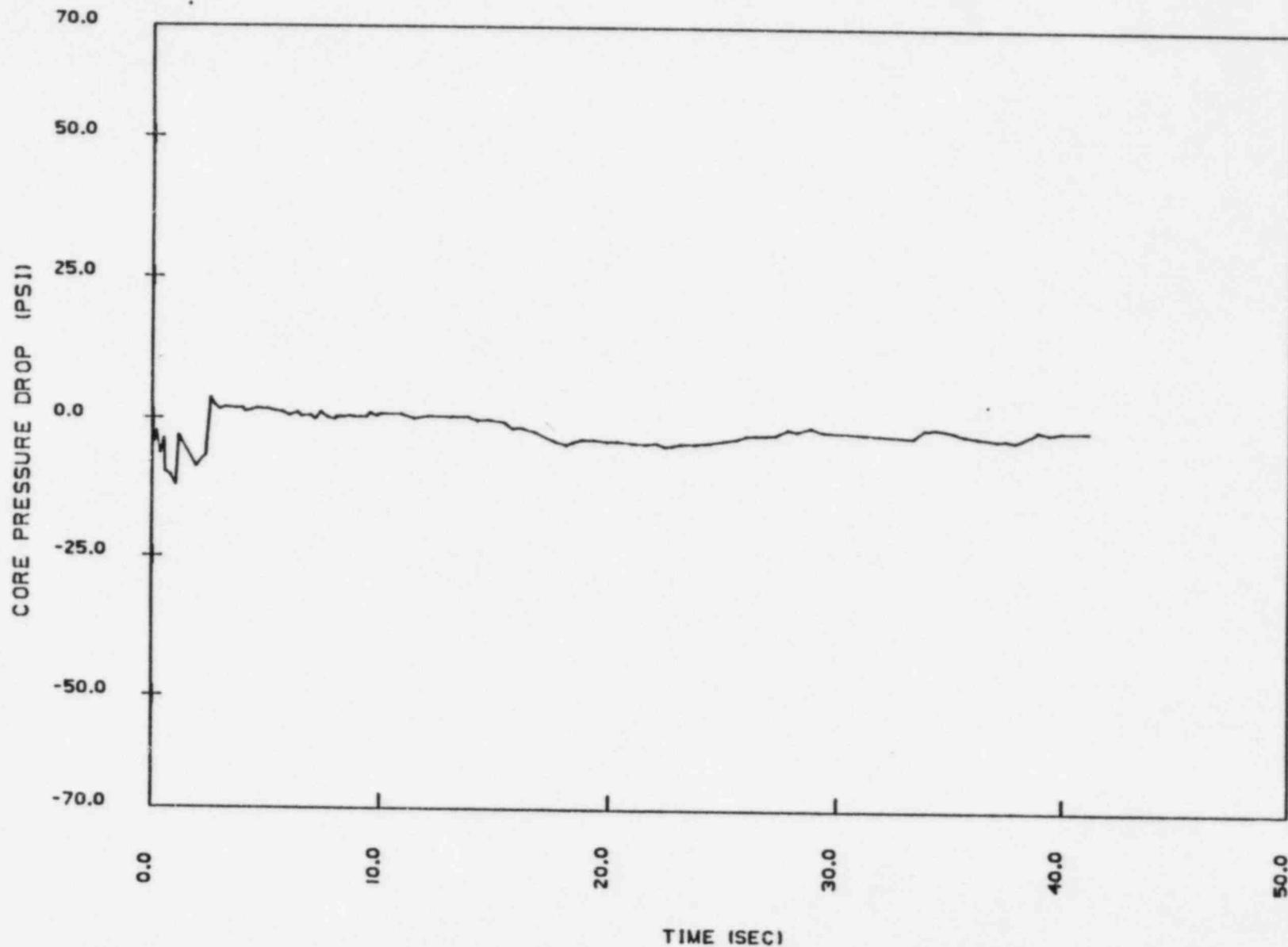
Figure 15.4-6A. Core Pressure Drop - DECLG ( $C_D = 0.4$ )
