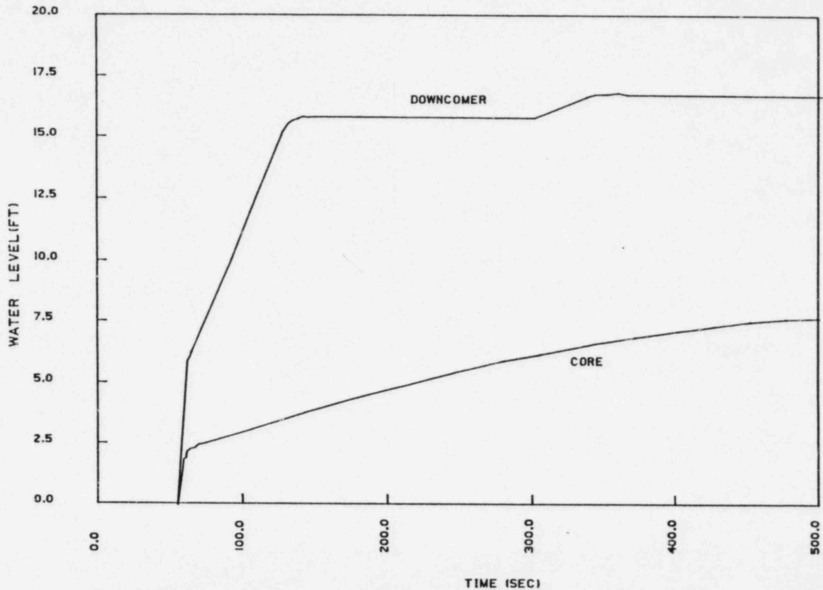
FIGURE 15.4-10A. Reflood Transient - DECLG ( $C_D = 0.4$ ) Inactive Loop Break
