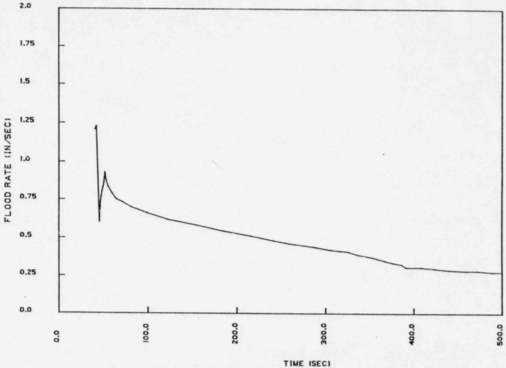
Figure 15.4-10F. Reflood Transient -  $DECLG(C_D = 0.4)$  Active Loop Break
