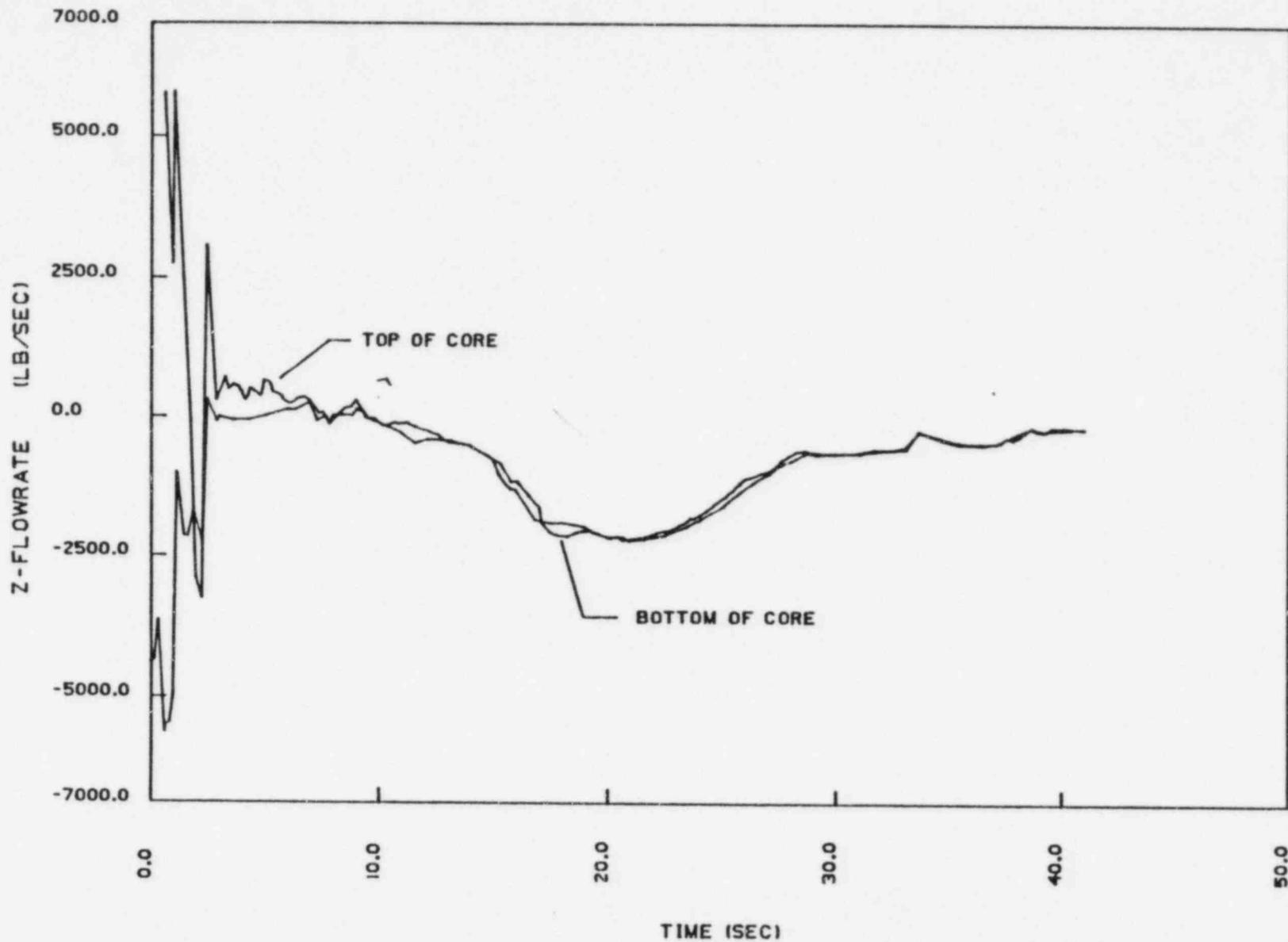
Figure 15.4-9A. Core Flow - Top and Bottom - DECLG ( $C_D = 0.4$ )
