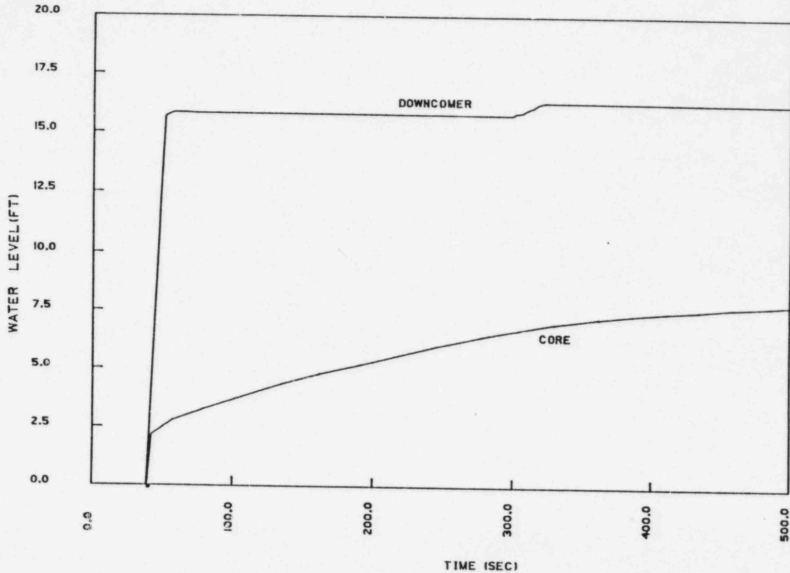
Figure 15.4-10C. Reflood Transient -  $DECLG(C_D = 0.4)$  Active Loop Break
