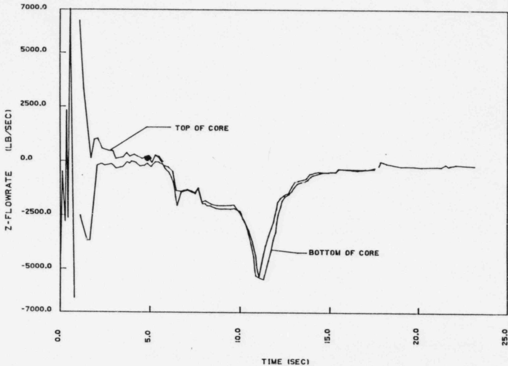
Figure 15.4-9B. Core Flow - Top and Bottom - DECLG ( $C_D = 0.6$ )
