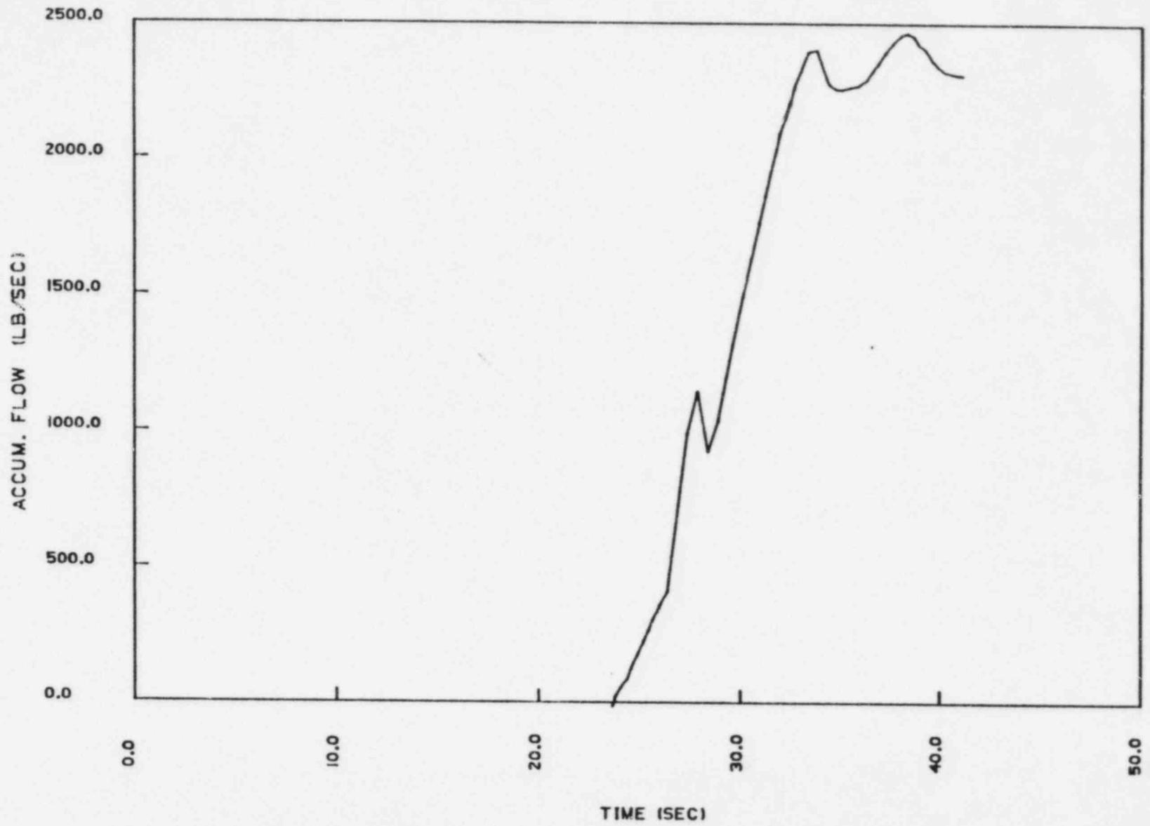
Figure 15.4-11A. Accumulator Flow (Blowdown) - DECLG ( $C_D = 0.4$ )
