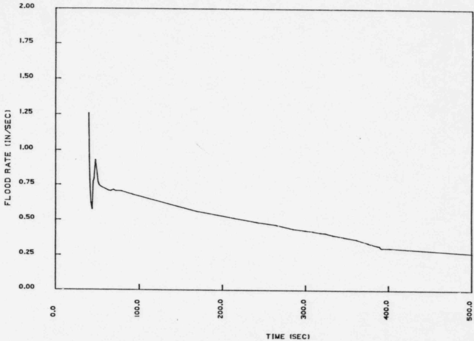
Figure 15.4-10E. Reflood Transient - DECLG ( $C_D = 0.6$ ) Active Loop Break Core Inlet Velocity
