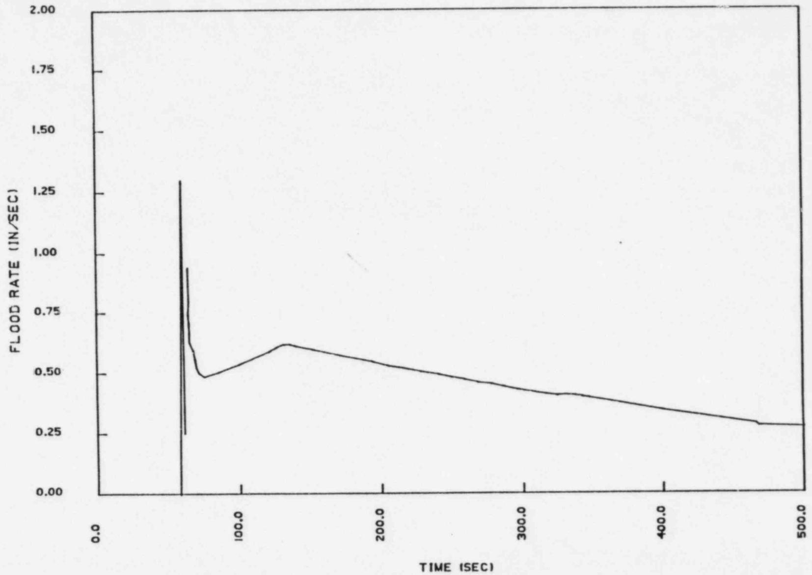
FIGURE 15.4-10D. Reflood Transient - DECLG (C<sub>D</sub>=0.4) Inactive Loop Break
