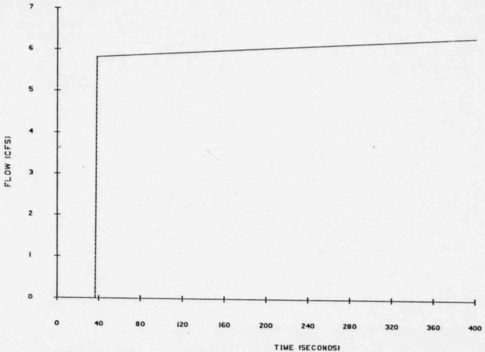
Figure 15.4-12B. Pumped Safety Injection Flow During Reflood: ( $C_D=0.6$ ) DECLG, Active Loop Break
