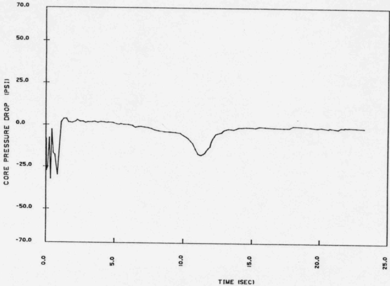
Figure 15.4-6B. Core Pressure Drop - DECLG ( $C_D = 0.6$ )
