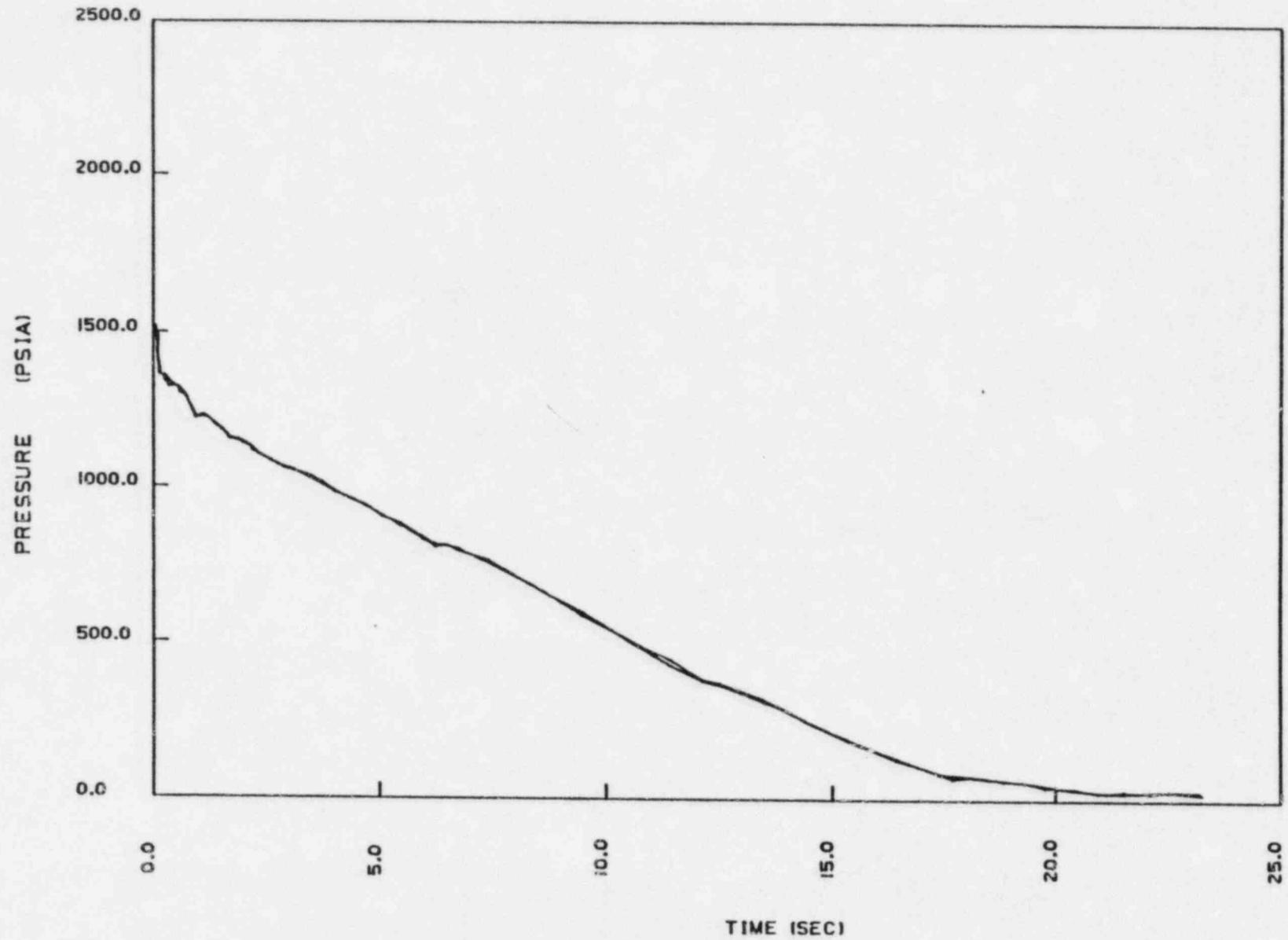
Figure 15.4-4B. Core Pressure - DECLG ( $C_D = 0.6$ )
