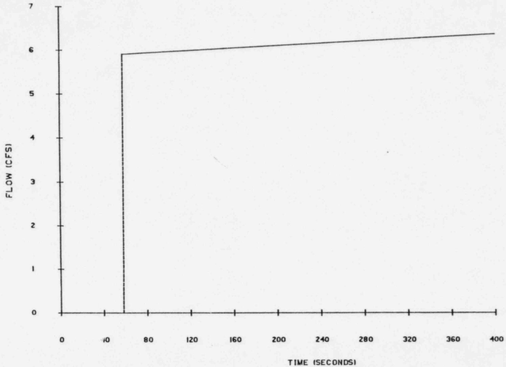
Figure 15.4-12A. Pumped Safety Injection Flow During Reflood: ( $C_D=0.4$ ) DECLG, Inactive Loop Break
