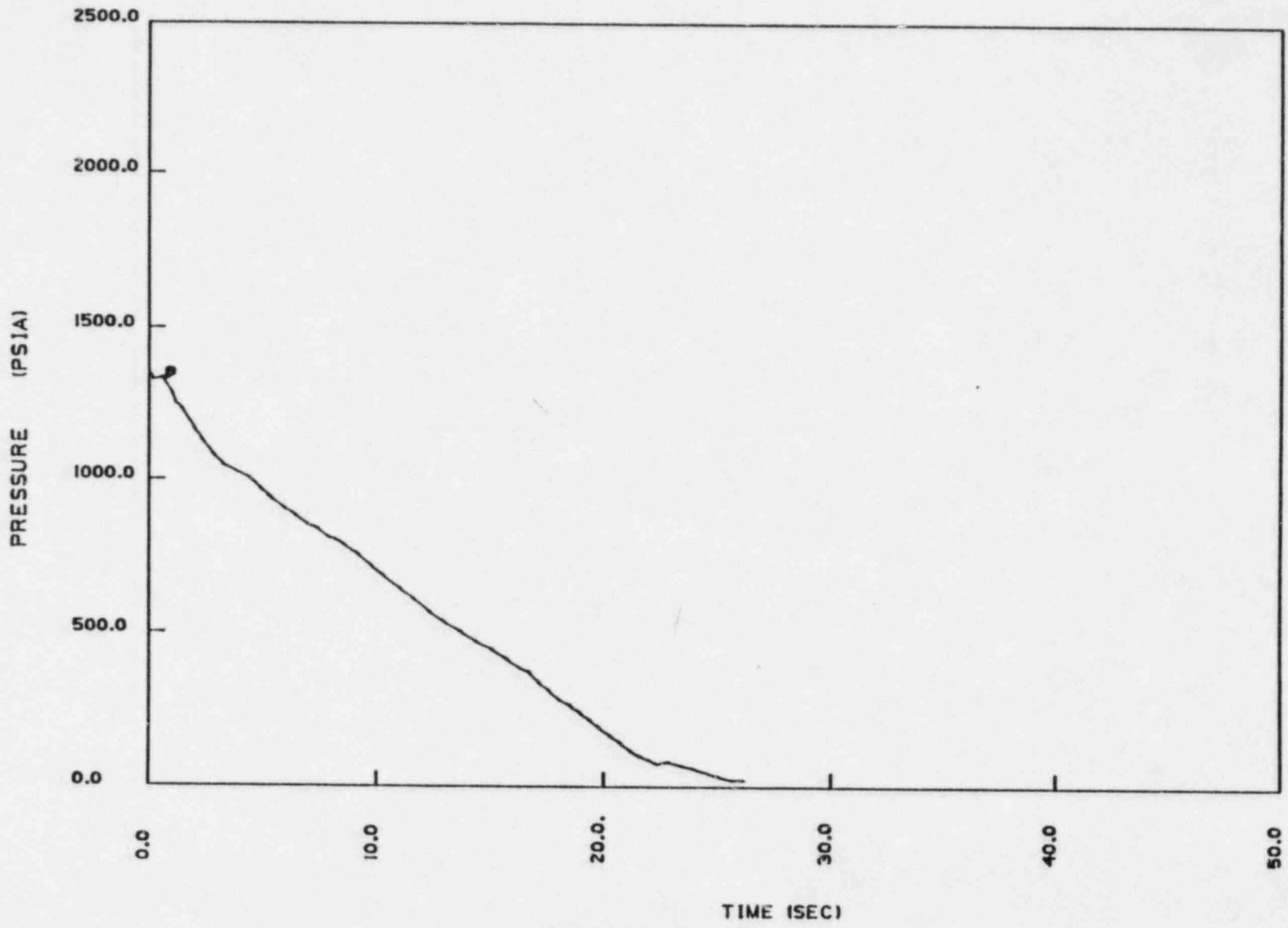
Figure 15.4-4C. Core Pressure - DECLG ( $C_D = 0.4$ )
