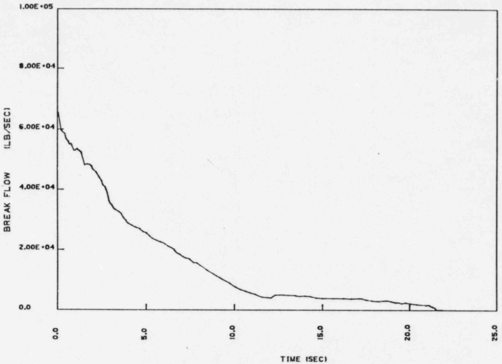
Figure 15.4-5B. Break Flow Rate - DECLG ( $C_D = 0.6$ )
