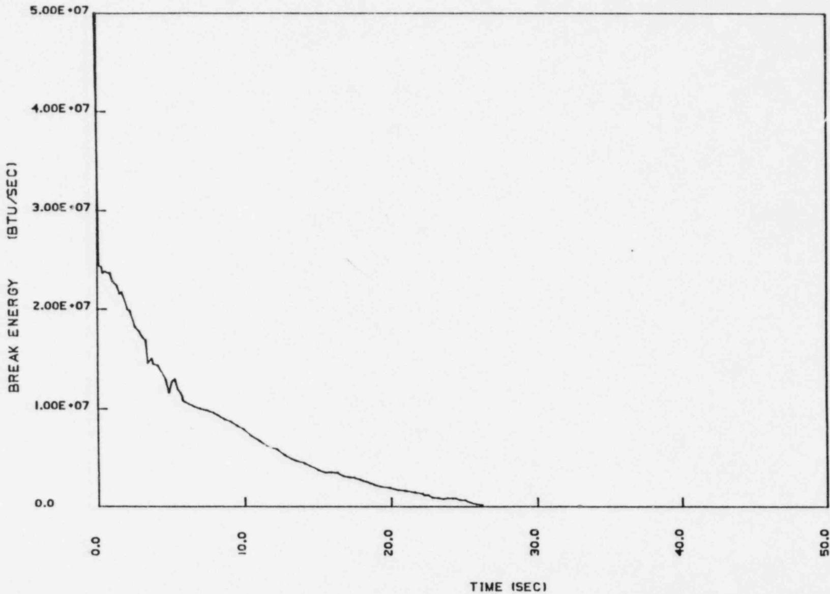
Figure 15.4-15. Break Energy Flow, ( $C_D = 0.4$ ) DECLG
