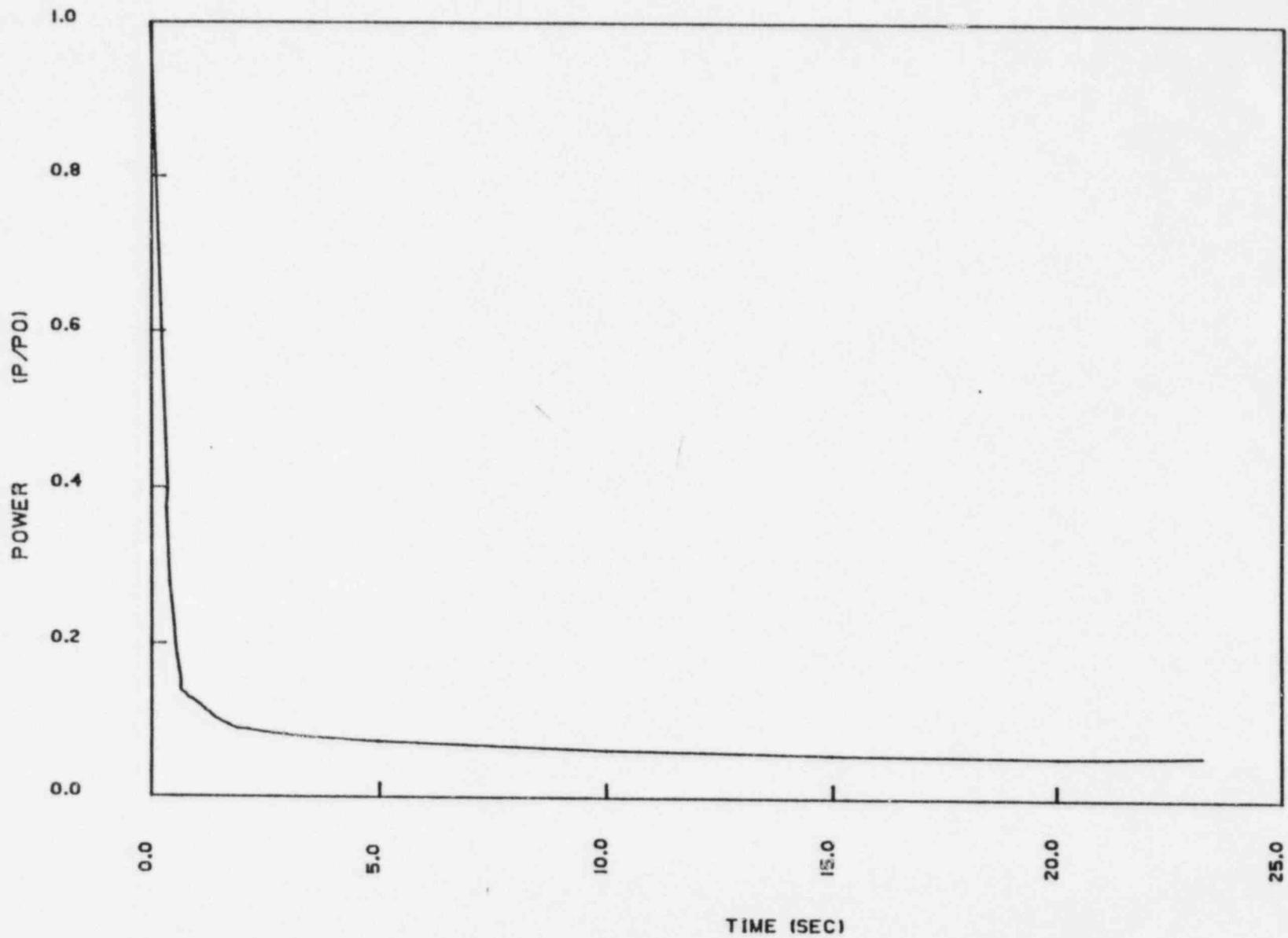
Figure 15.4-14B. Core Power Transient - DECLG ( $C_D = 0.6$ )
