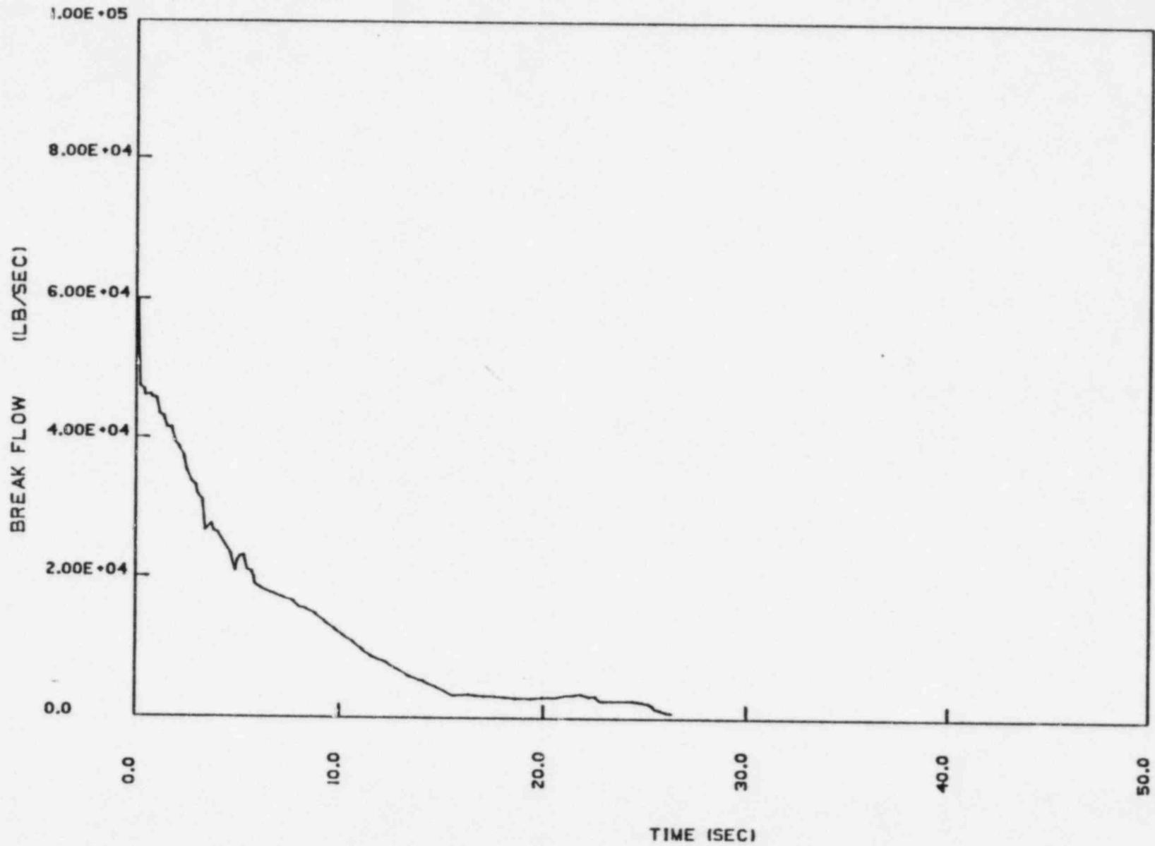
Figure 15.4-5C. Break Flow Rate - DECLG ( $C_D = 0.4$ )
