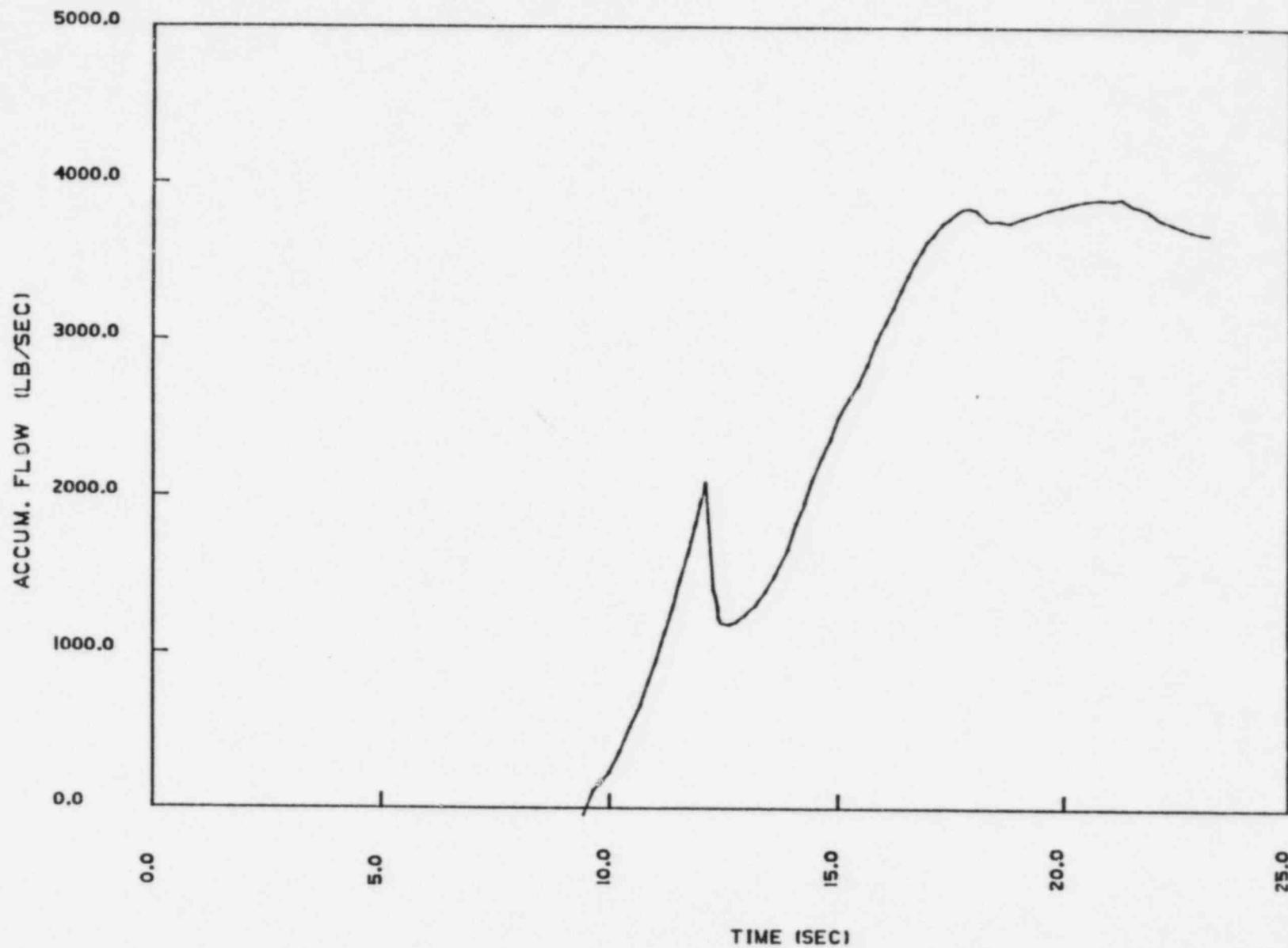
Figure 15.4-11B. Accumulator Flow (Blowdown) - DECLG ( $C_D = 0.6$ )
