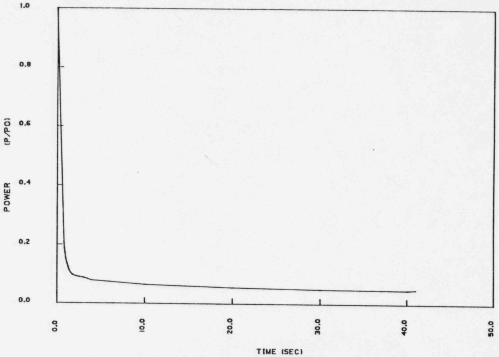
Figure 15.4-14A. Core Power Transient - DECLG ( $C_D=0.4$ )
