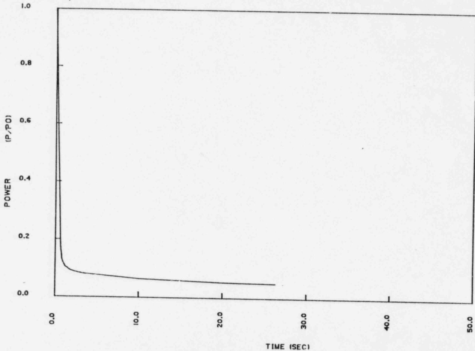
Figure 15.4-14C. Core Power Transient - DECLG ( $C_D=0.4$ )
