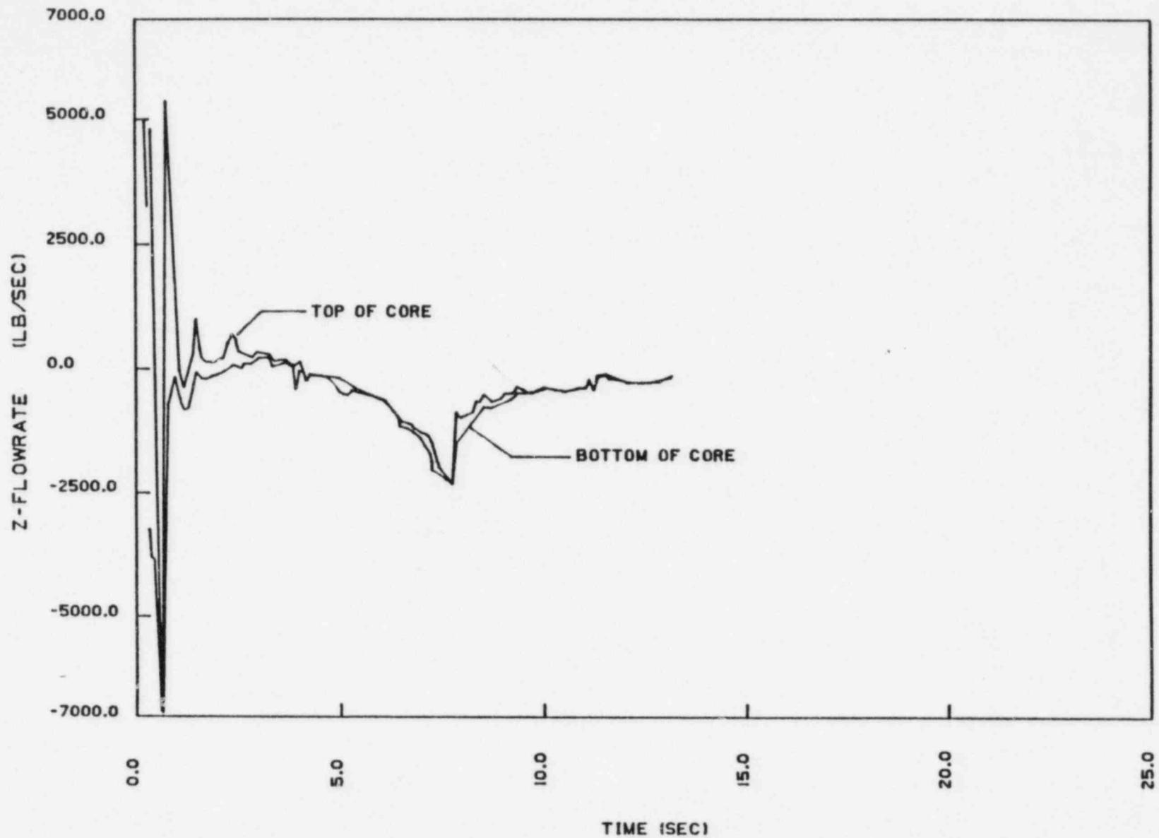
Figure 15.4-9C. Core Flow - Top and Bottom - DECLG ( $C_D = 0.4$ )
