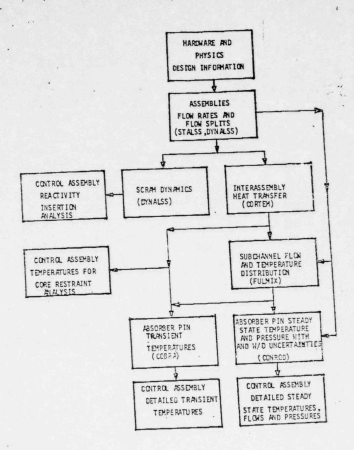
FIGURE 4.4-65 SECONDARY CONTROL ASSEMBLY AND ABSORBER PIN THEIMAL-HUDDAULIC MALYSIS FLOW DIAGRAM
