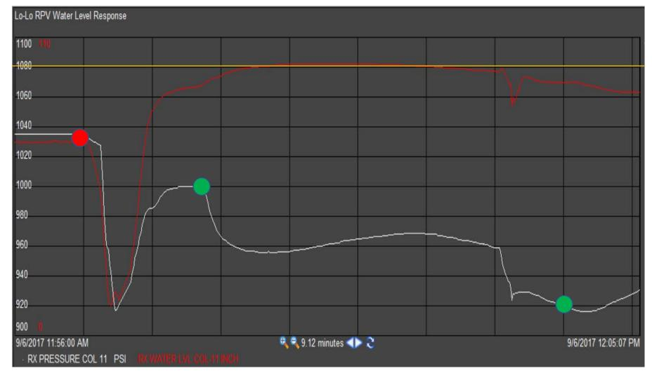
NMP1 Scram 9/6/17 Lo Reactor Water Level ~1157 – 13 Feedwater Flow Control Valve rapidly closed
