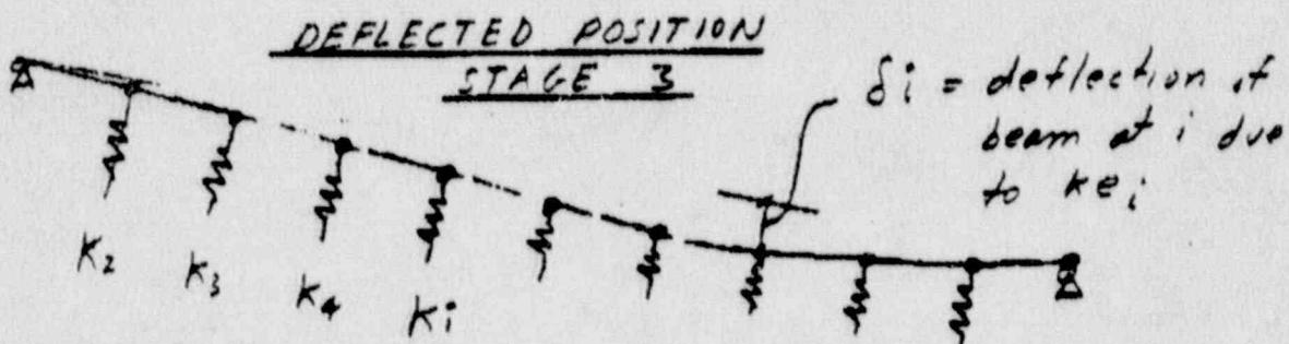
The Strain Energy,  $S_e$  for each spring is  $S_e = \frac{1}{2} k_i \delta_i^2$  at max. deflection
