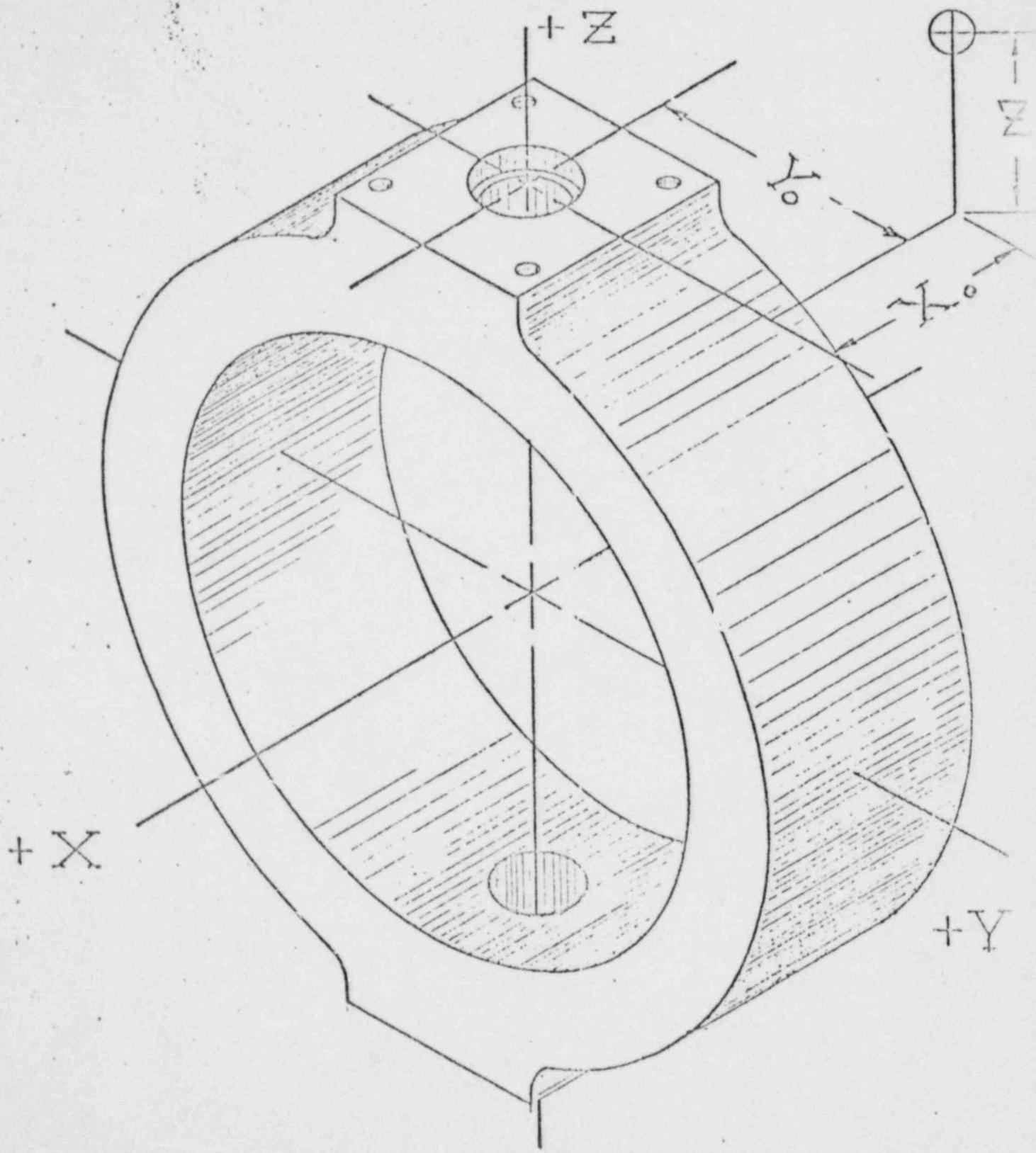
Figure 1 VALVE BODY SPATIAL ORIENTATION
