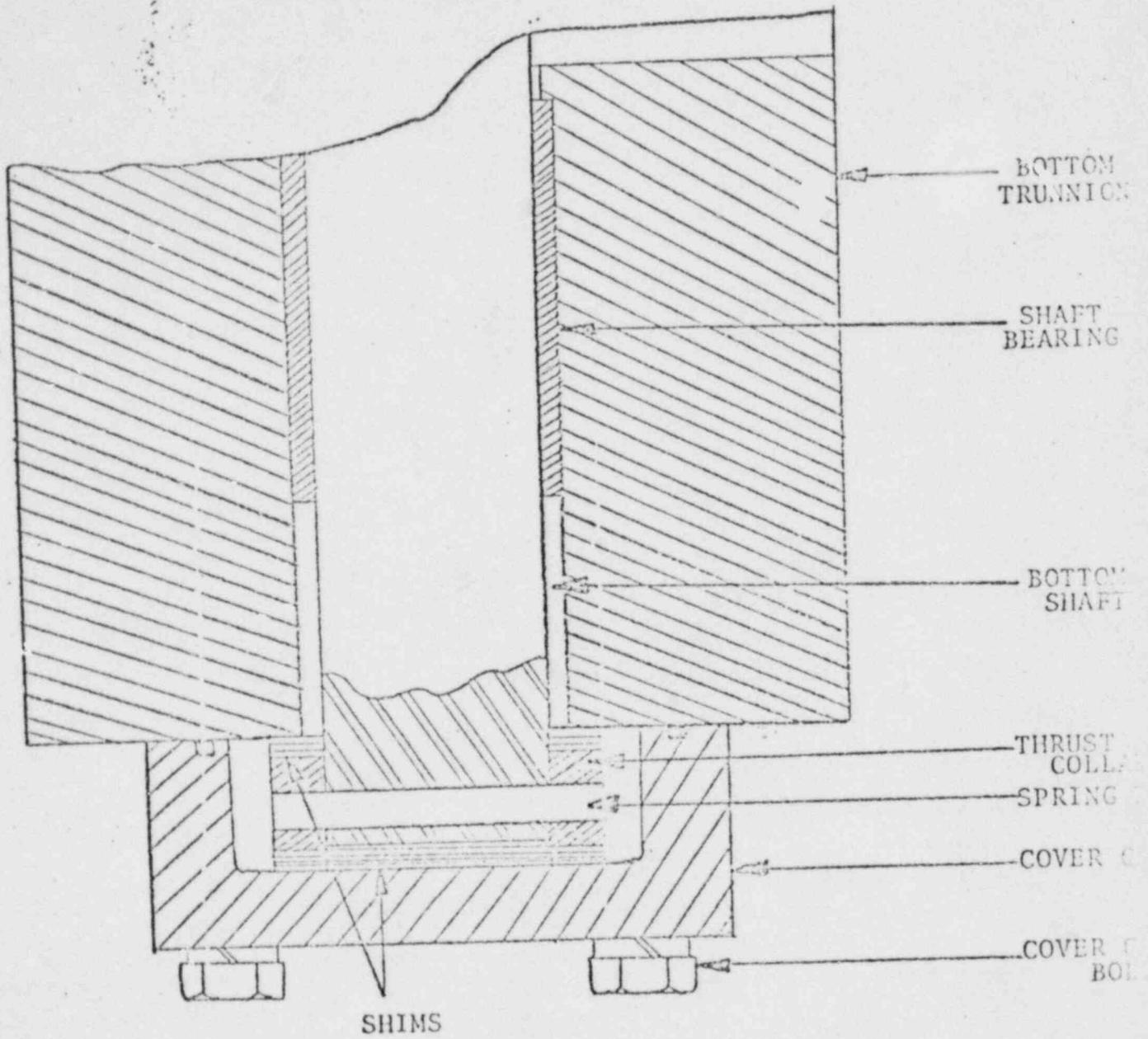
BOTTOM TRUNNION AND THRUST BEARING ASSEMBLY
