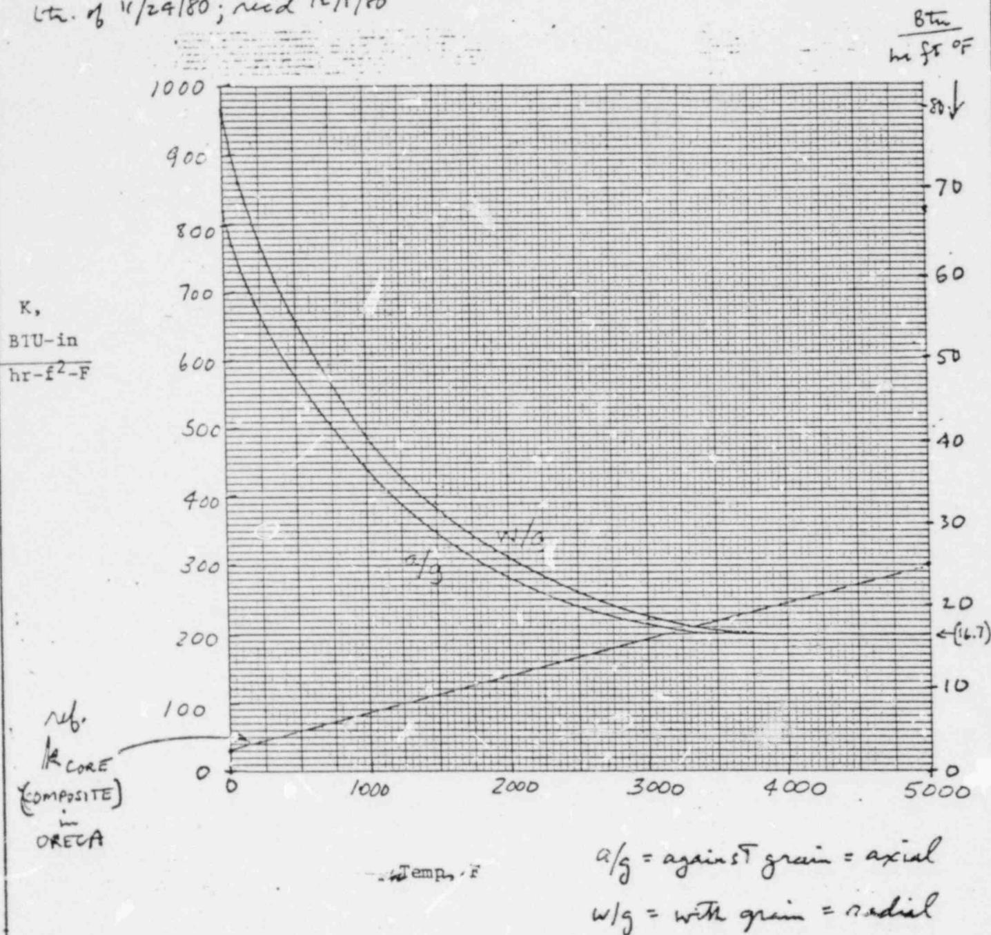
Figure 4-16. Average PGX Graphite Thermal Conductivity vs. Temperature
