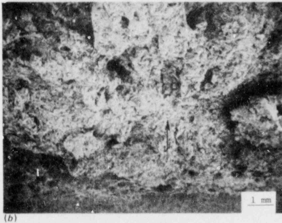
Fig. 2.18. Fracture surface of IT compact specimen (2TP33) of ORNL steel tested at -4^{\circ}\text{C} . (a) Arrow and box identify fracture origin, (b) fracture-initiation region corresponds to box in (a).
