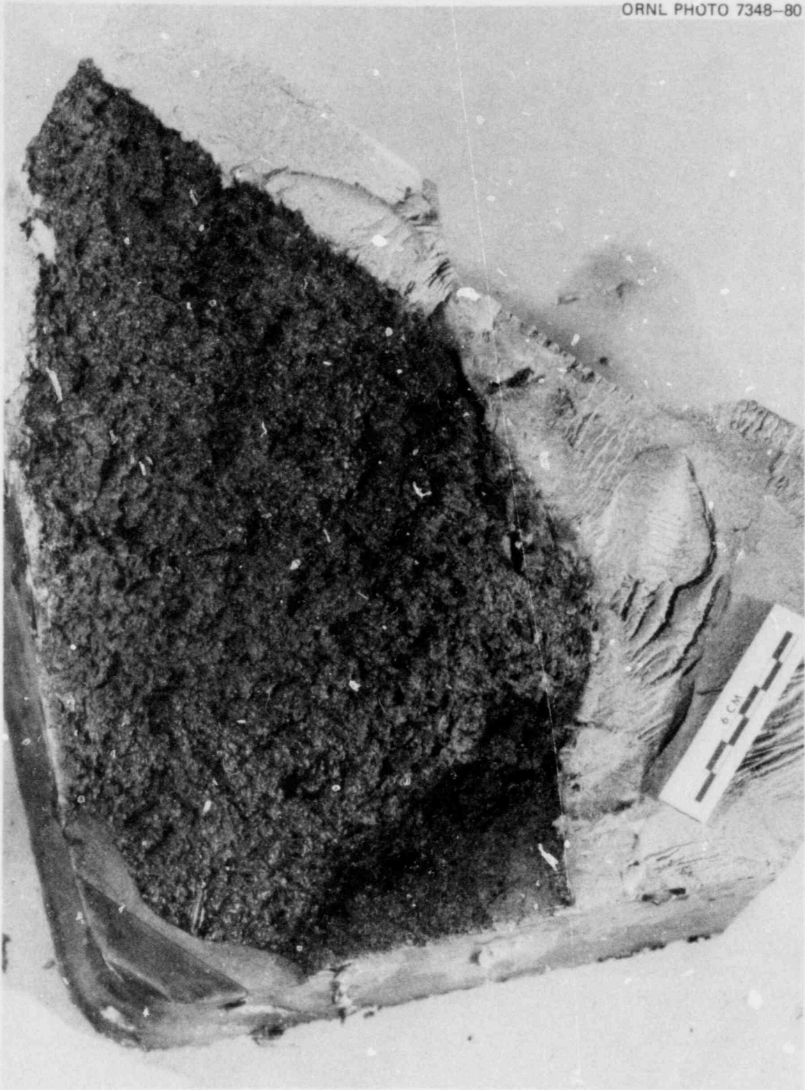
Fig. 5.20. Vessel V-5, right-side flawed region.
