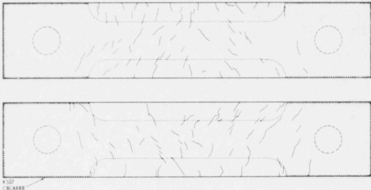
FIGURE 1. Test Specimen - KS07 Degraded Steel
