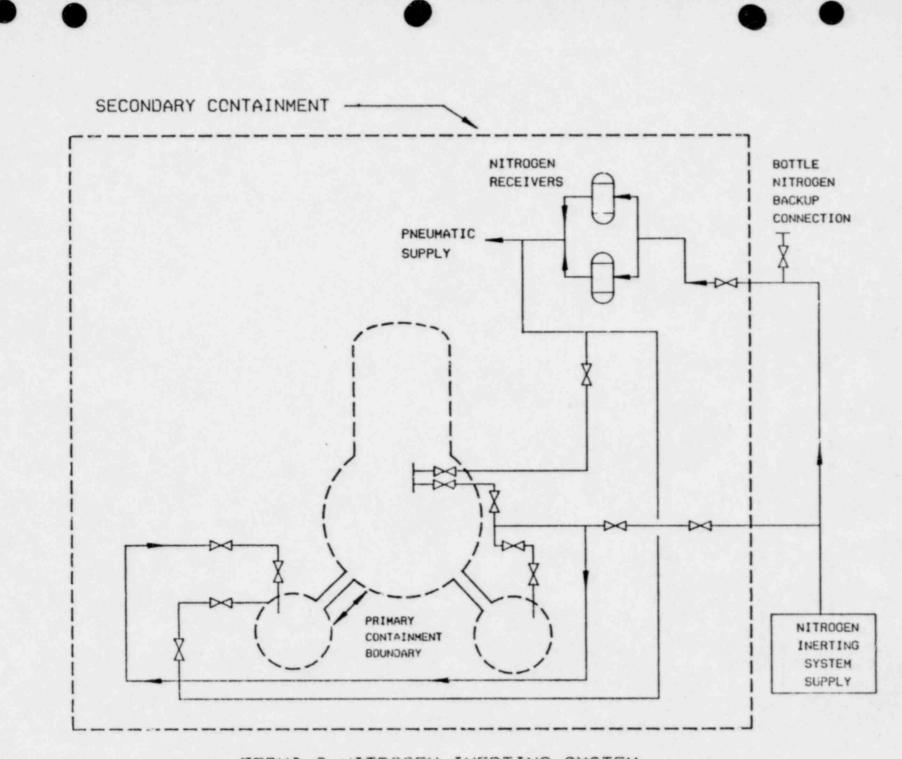
FERMI 2 NITROGEN INERTING SYSTEM
