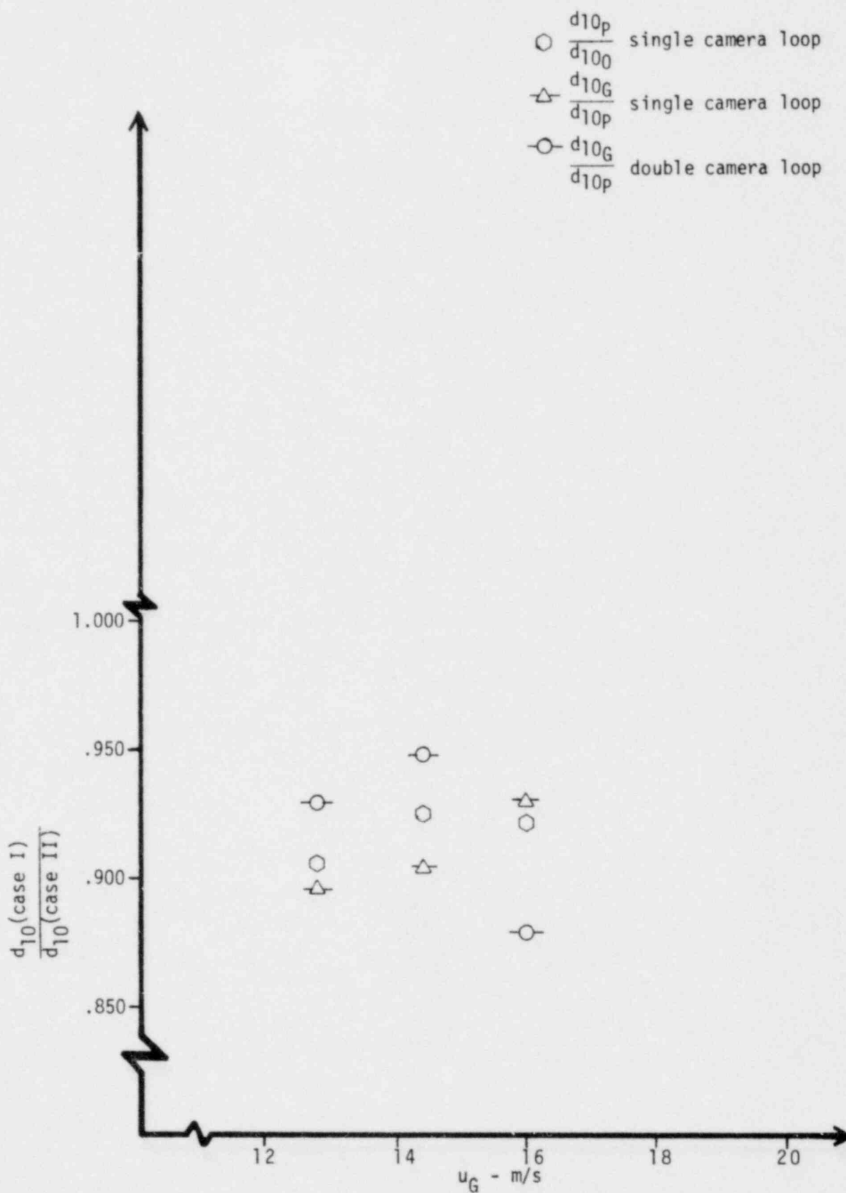
Figure 9. Droplet diameter ( d_{10} ) ratios to show geometry effect (lower portion) and with hydraulic diameter ratio (upper portion).
