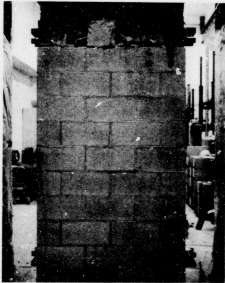
FIG. 3.14 FAILURES OF BRICK-BLOCK CAVITY WALLS From Reference (6)
