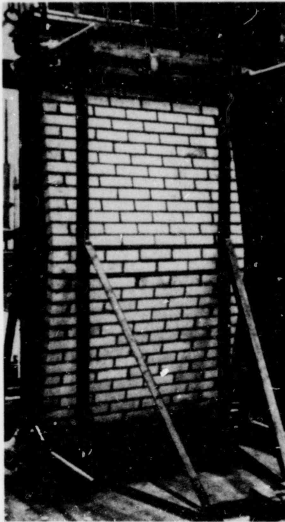
FIG. 3.12 TYPICAL FAILURE OF BRICK WALLS WITH LOW VERTICAL COMPRESSIVE LOADS From Reference (6)
