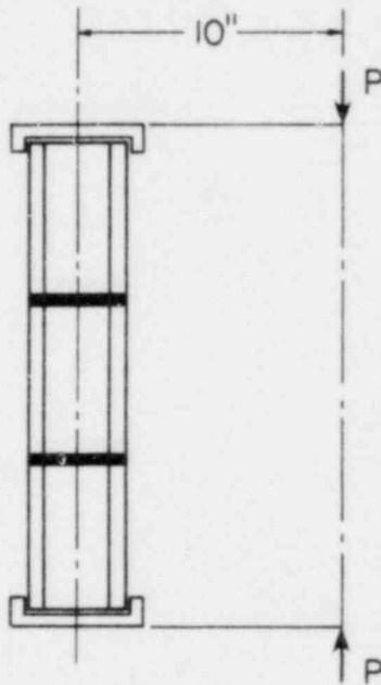
FIG. 2.3 WALLETTE TEST EQUIPMENT From Reference (24)
