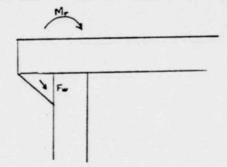
The reaction force of the weld can be applied at the center of the weld throat.
