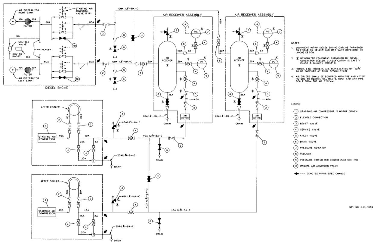
Figure 9.5-8 Standby Diesel Generator Starting Air System
