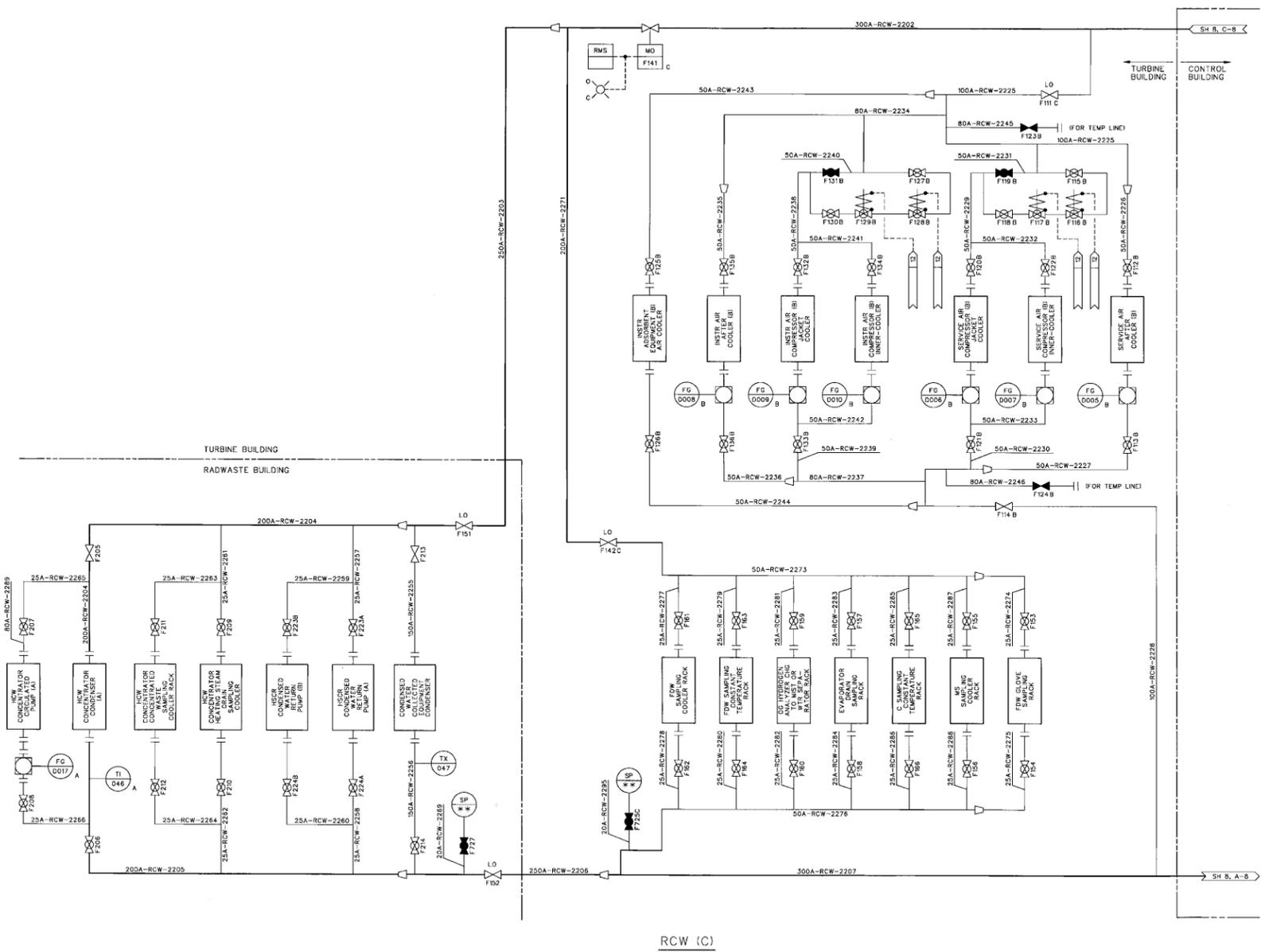
Figure 9.2-1 Reactor Building Cooling Water System P&ID (Sheet 9 of 9)
