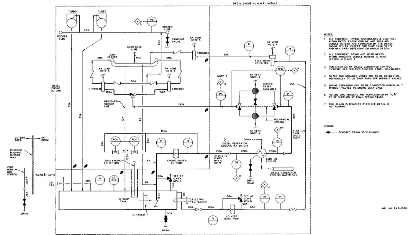
Figure 9.5-9 Standby Diesel Generator Lubricating Oil System
