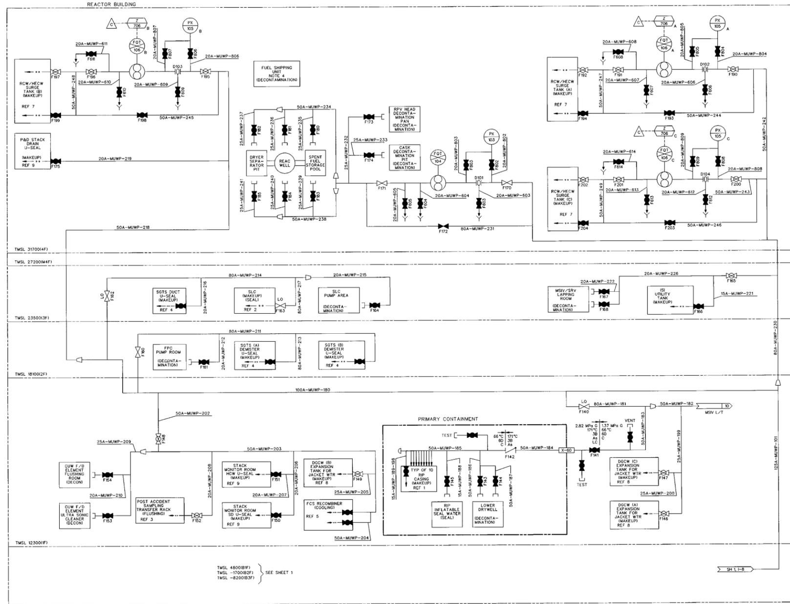
Figure 9.2-5 Makeup Water System (Purified) P&ID (Sheet 2 of 3)
