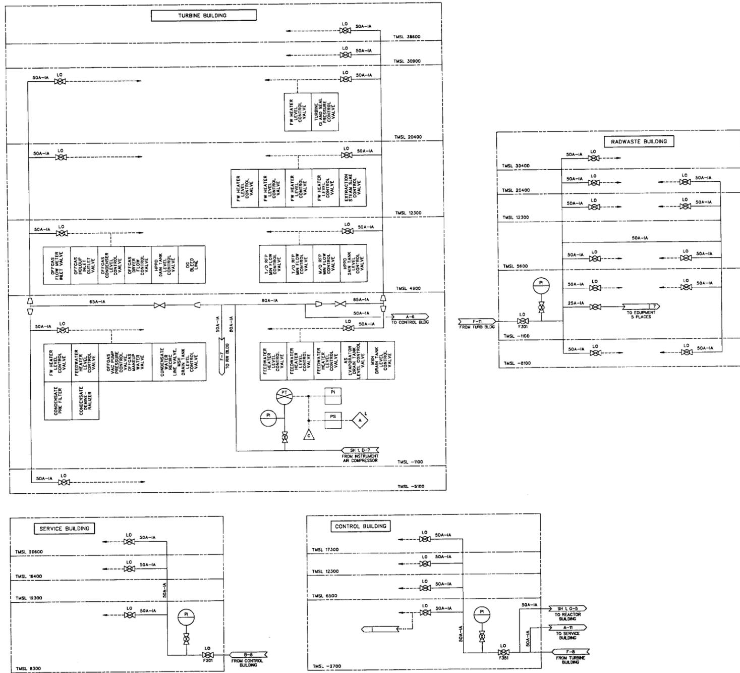
Figure 9.3-6 Instrument Air System P&ID (Sheet 2 of 2)
