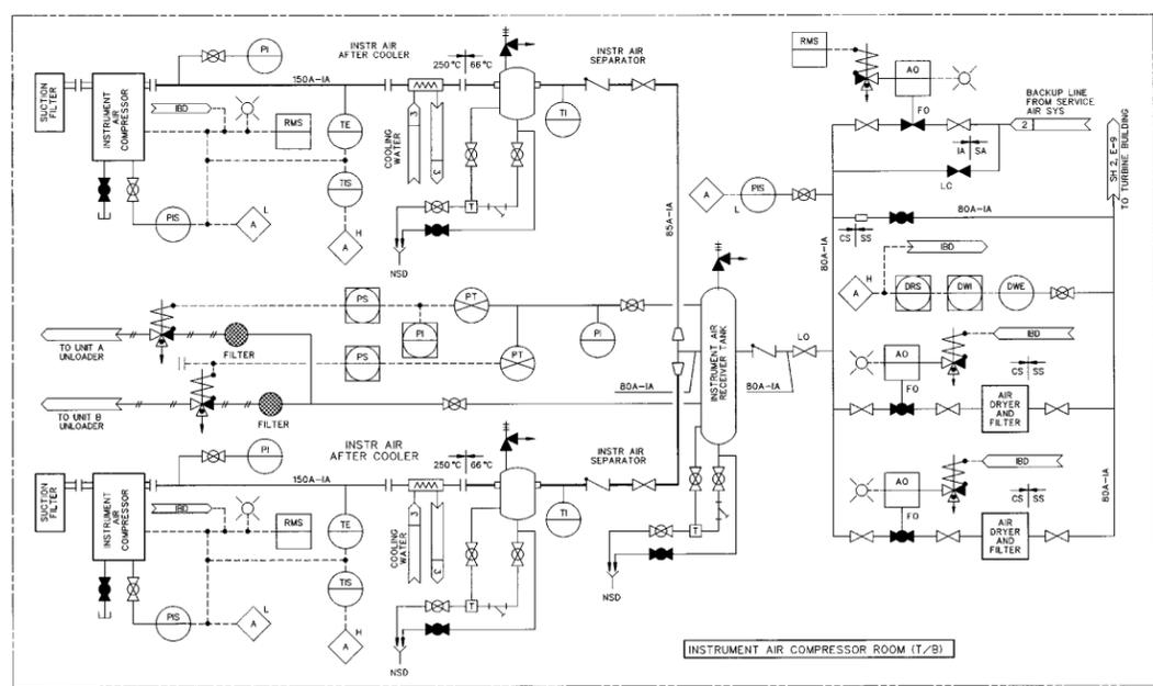
Figure 9.3-6 Instrument Air System P&ID (Sheet 1 of 2)
