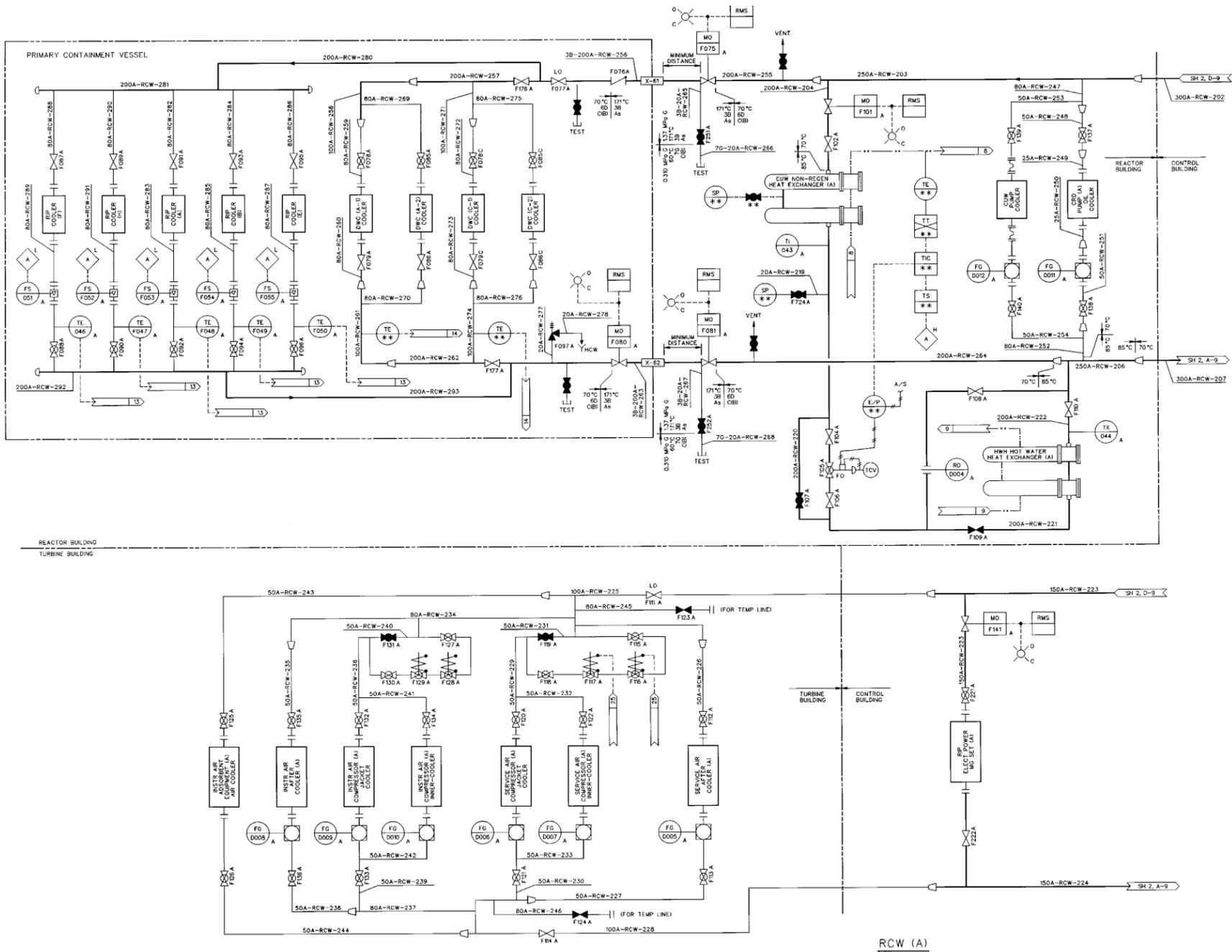
Figure 9.2-1 Reactor Building Cooling Water System P&ID (Sheet 3 of 9)
