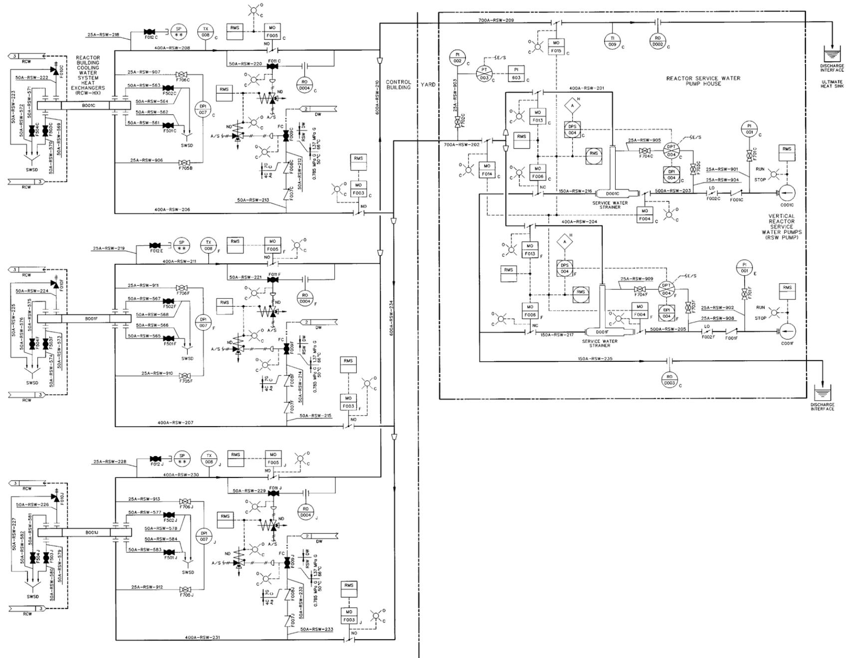
Figure 9.2-7 Reactor Service Water System P&ID (Sheet 3 of 3)
