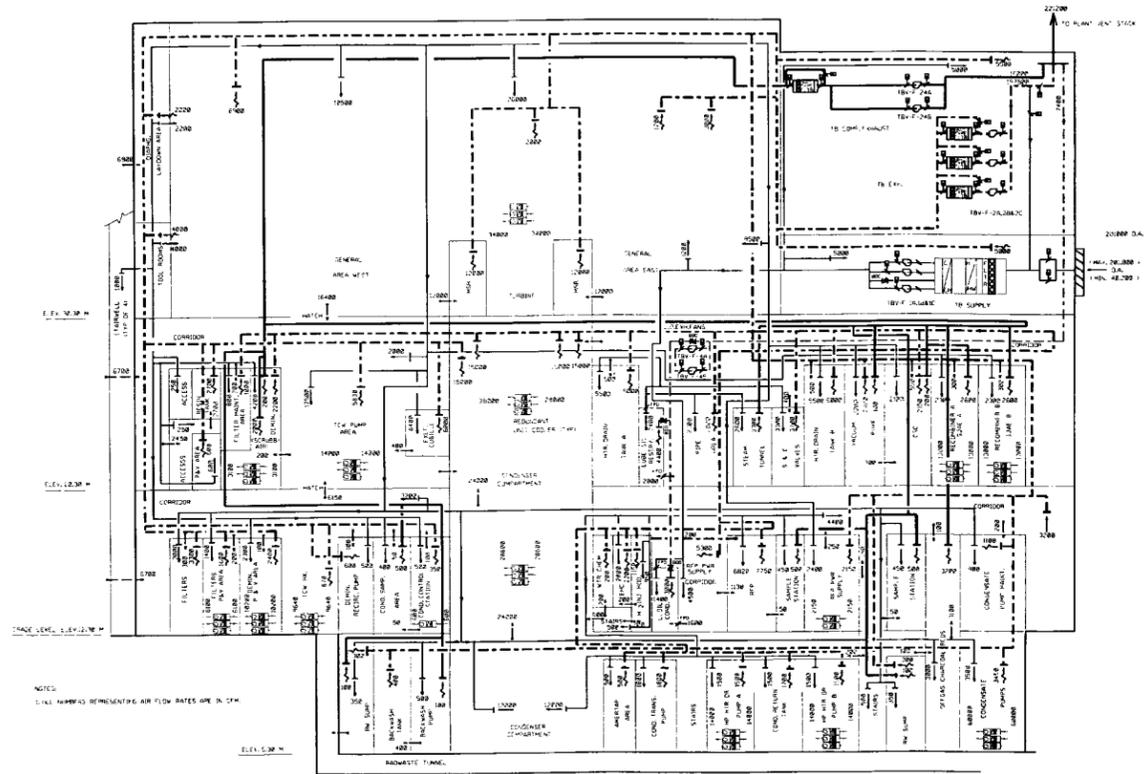
Figure 9.4-2a Turbine Building Ventilation System Air Flow Diagram
