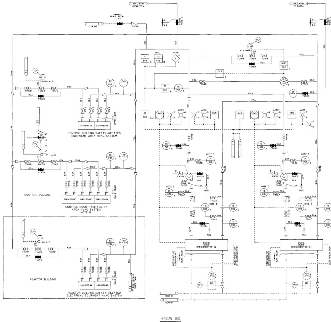
Figure 9.2-3 HVAC Emergency Cooling Water System P&ID (Sheet 2 of 3)
