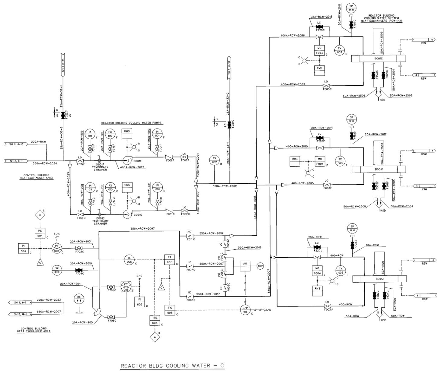
Figure 9.2-1 Reactor Building Cooling Water System P&ID (Sheet 7 of 9)
