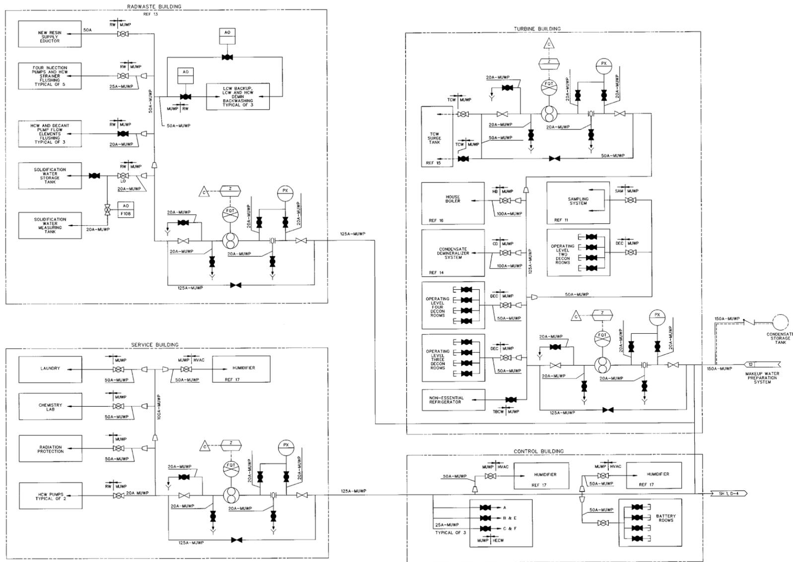
Figure 9.2-5 Makeup Water System (Purified) P&ID (Sheet 3 of 3)
