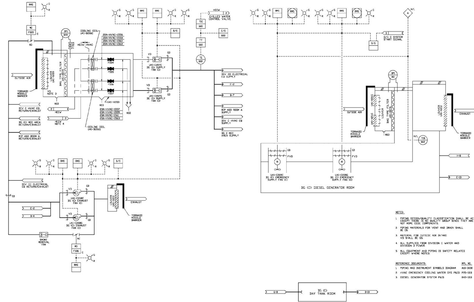
Figure 9.4-4 R/B Safety-Related Electrical Equipment HVAC System (Sheet 3 of 3)
