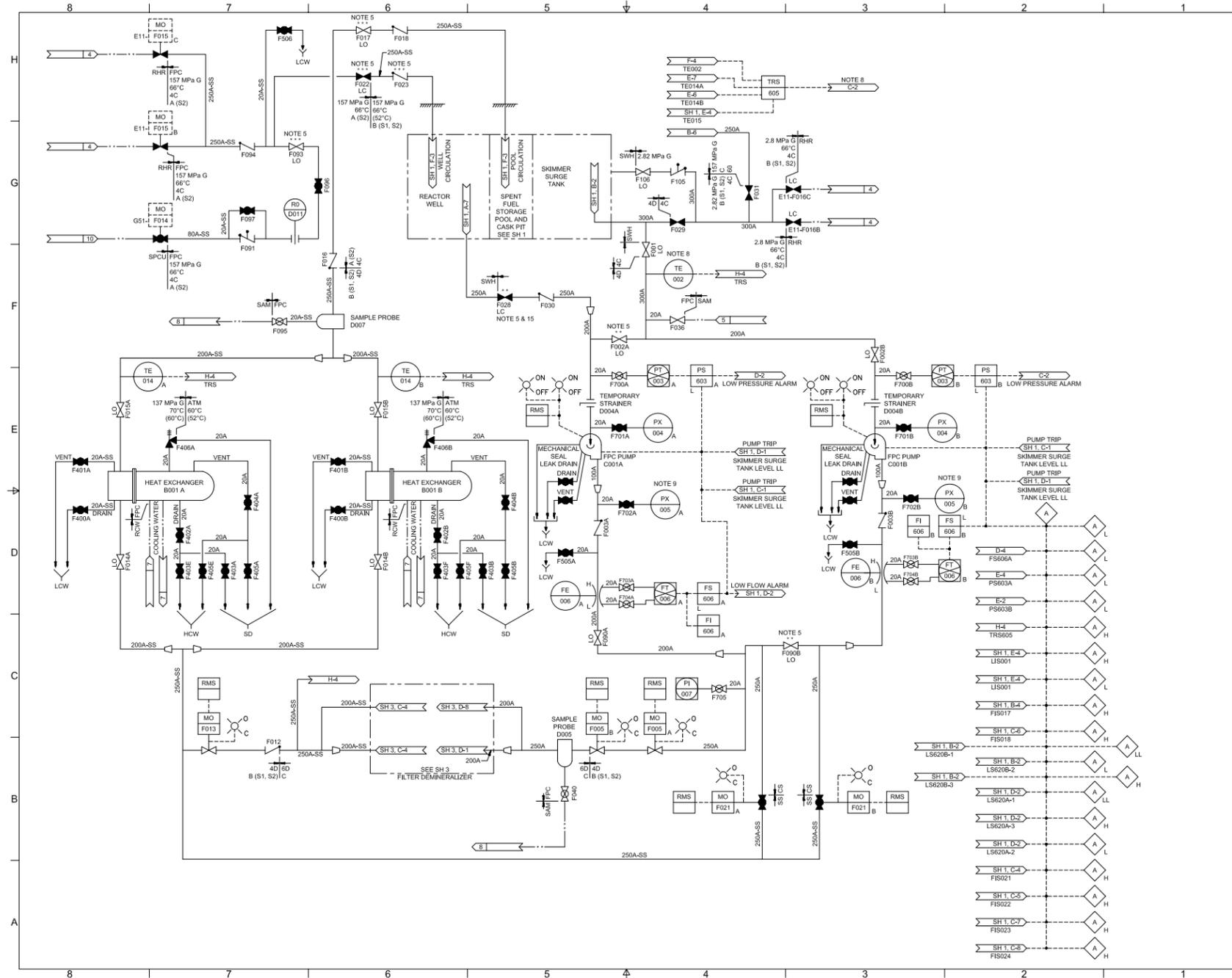
Figure 9.1-1 Fuel Pool Cooling and Cleanup System P&ID (Sheet 2 of 3)
