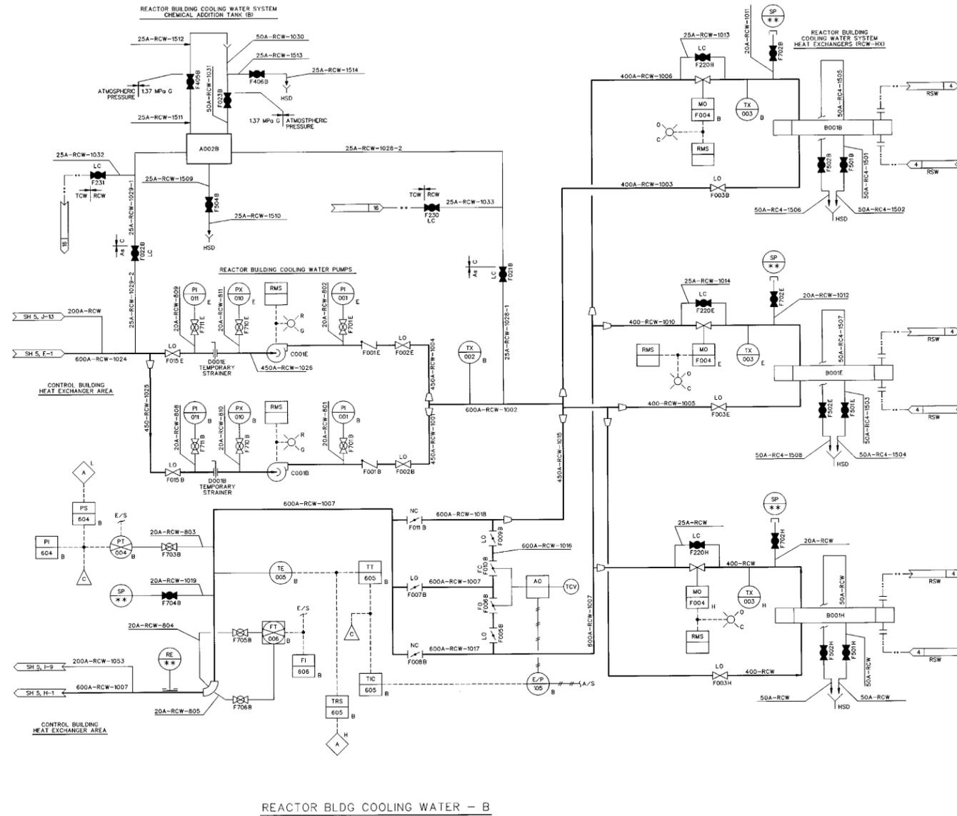
Figure 9.2-1 Reactor Building Cooling Water System P&ID (Sheet 4 of 9)
