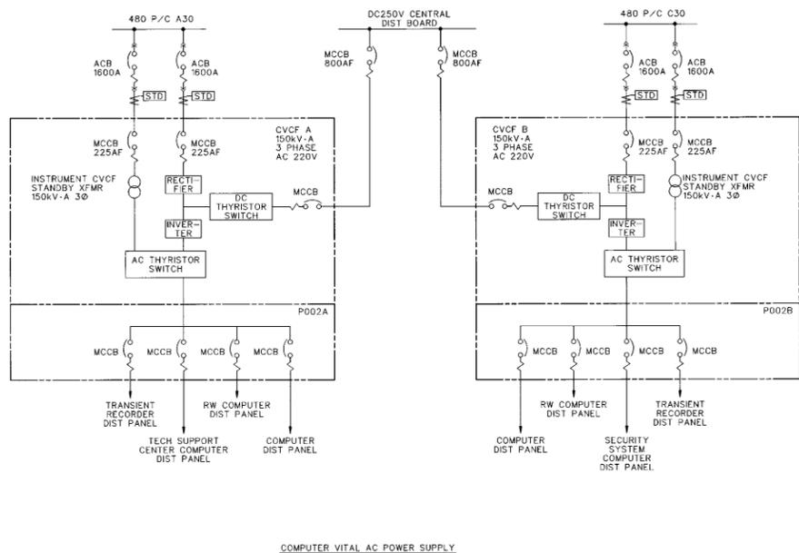
Figure 8.3-3 Plant Vital AC Power Supply System SLD (Sheet 2 of 2)
