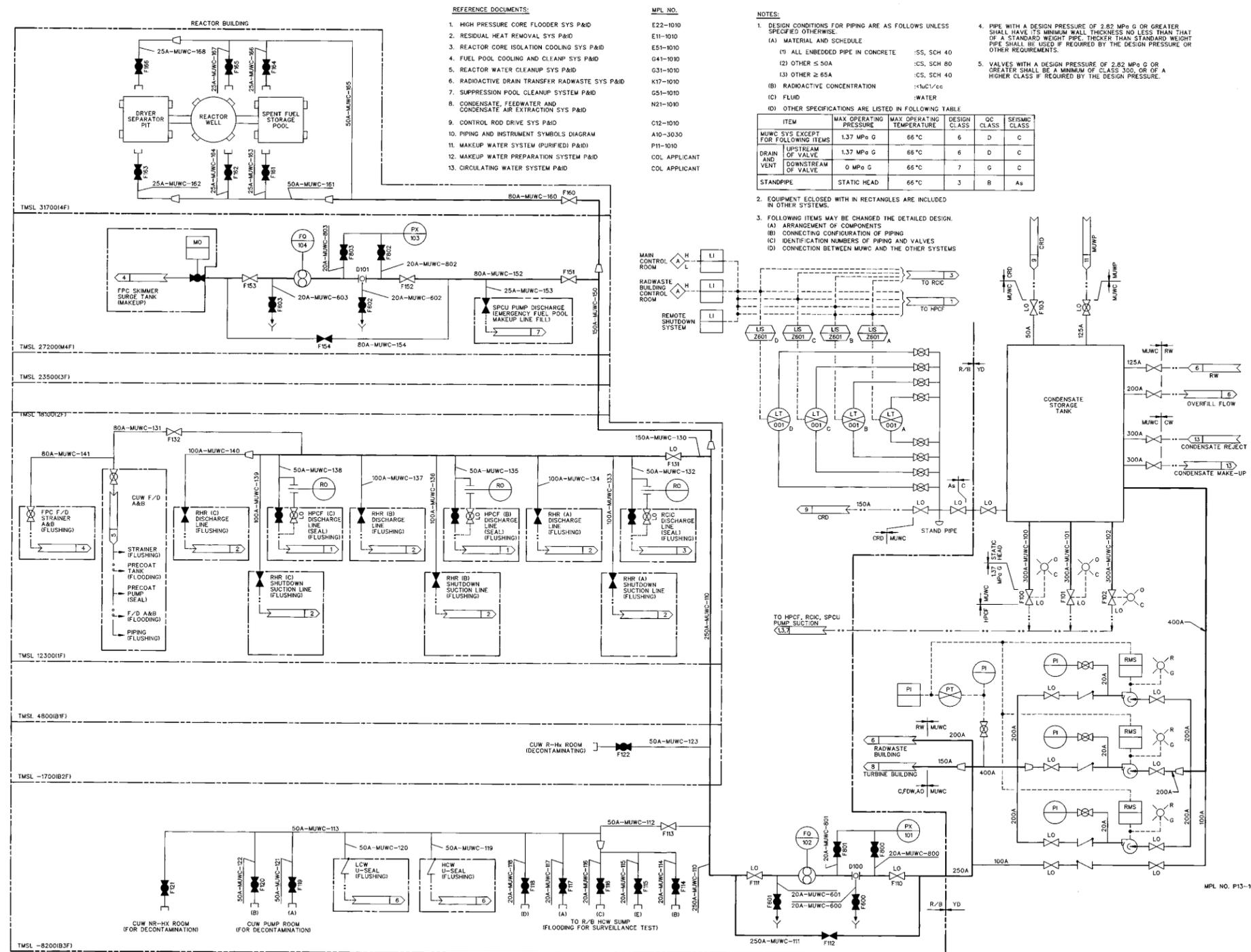
Figure 9.2-4 Makeup Water System (Condensate) P&ID
