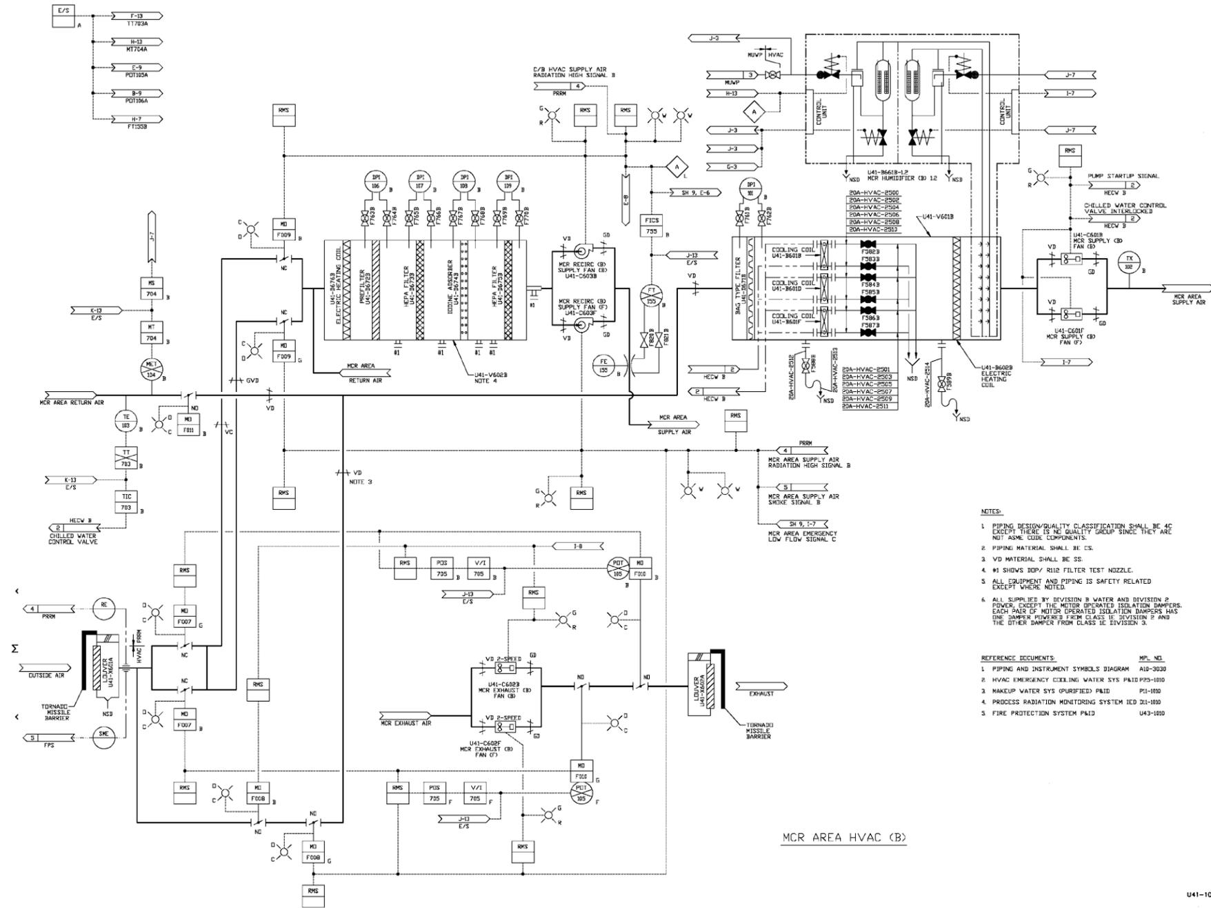
Figure 9.4-1 Control Building HVAC Flow Diagram (Sheet 1 of 5)
