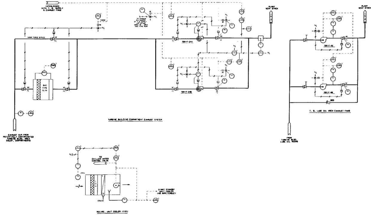
Figure 9.4-2b Turbine Building Ventilation System Control Diagram (Sheet 2 of 2)
