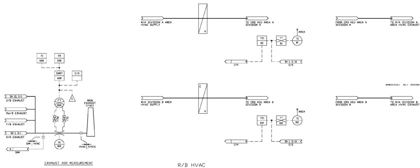
Figure 9.4-3 Secondary Containment HVAC System (Sheet 3 of 3)
