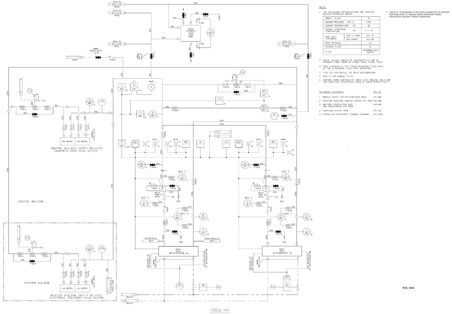
Figure 9.2-3 HVAC Emergency Cooling Water System P&ID (Sheet 1 of 3)
