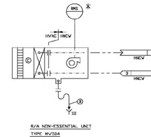
Figure 9.4-3 Secondary Containment HVAC System (Sheet 2 of 3)
