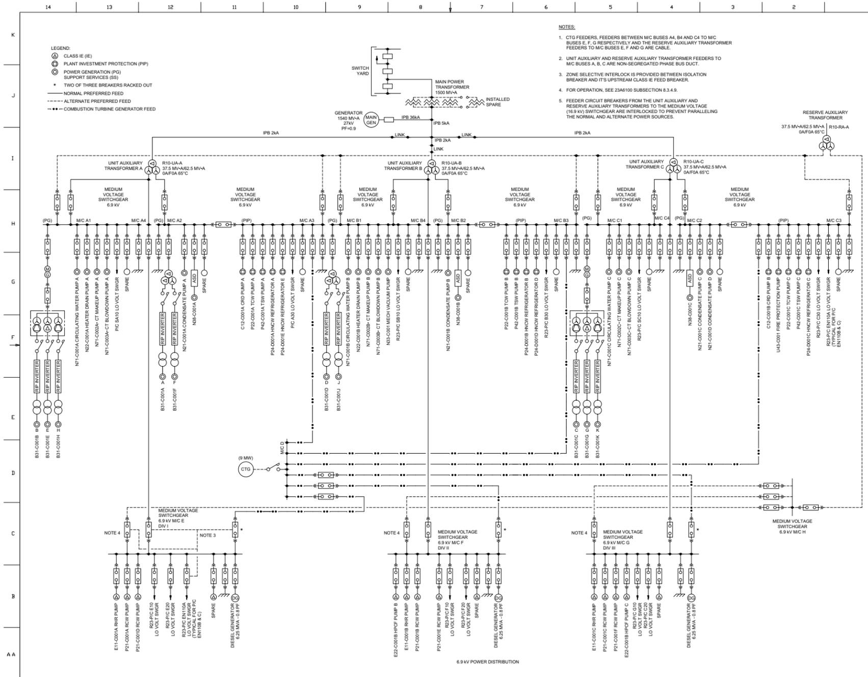
Figure 8.3-1 Electrical Power Distribution System SLD (Sheet 1 of 3)
