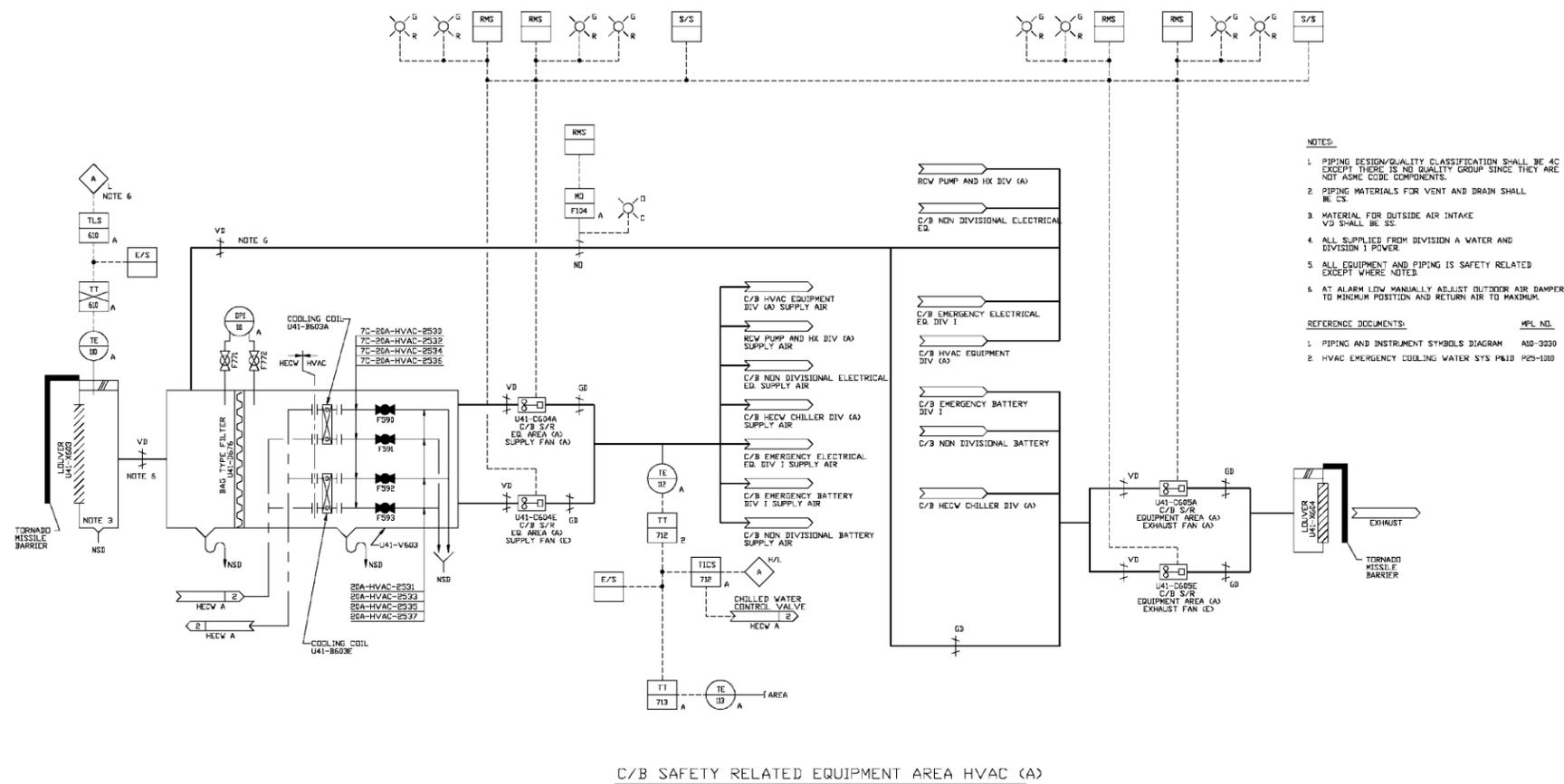
Figure 9.4-1 Control Building HVAC Flow Diagram (Sheet 3 of 5)
