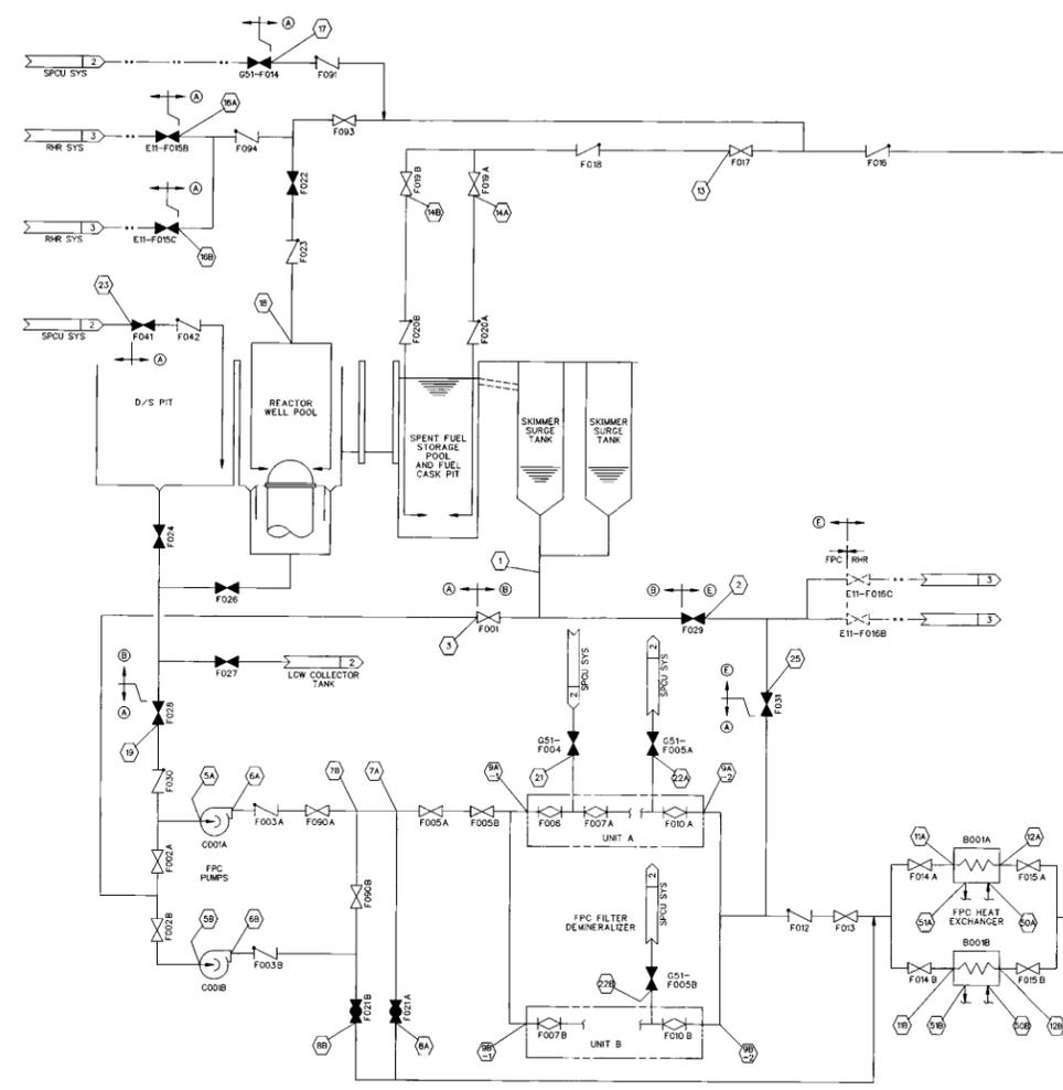
MODE A FPC SYSTEM FLOW DIAGRAM
