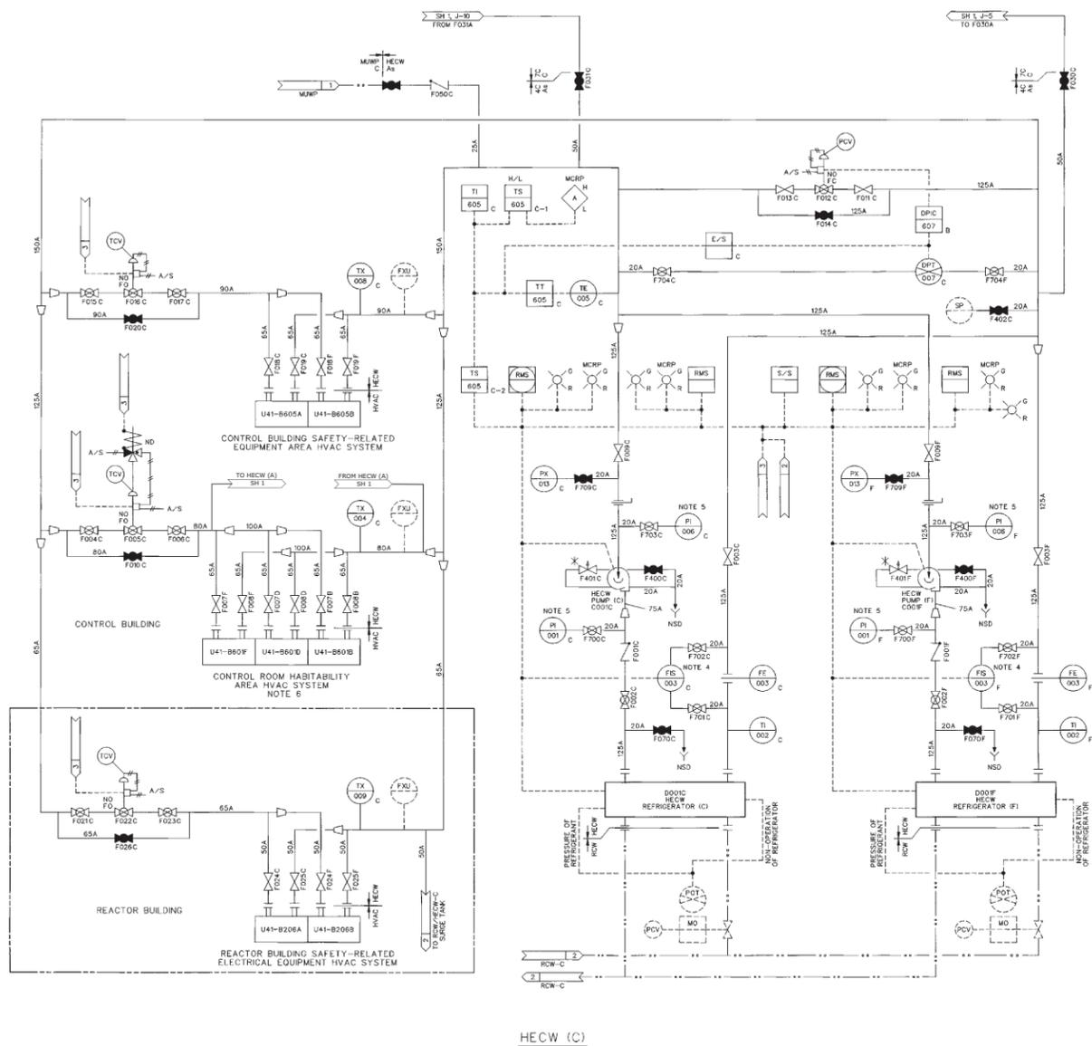
Figure 9.2-3 HVAC Emergency Cooling Water System P&ID (Sheet 3 of 3)
