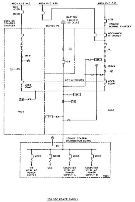
Figure 8.3-4 Plant DC Power Supply System SLD (Sheet 3 of 3)
