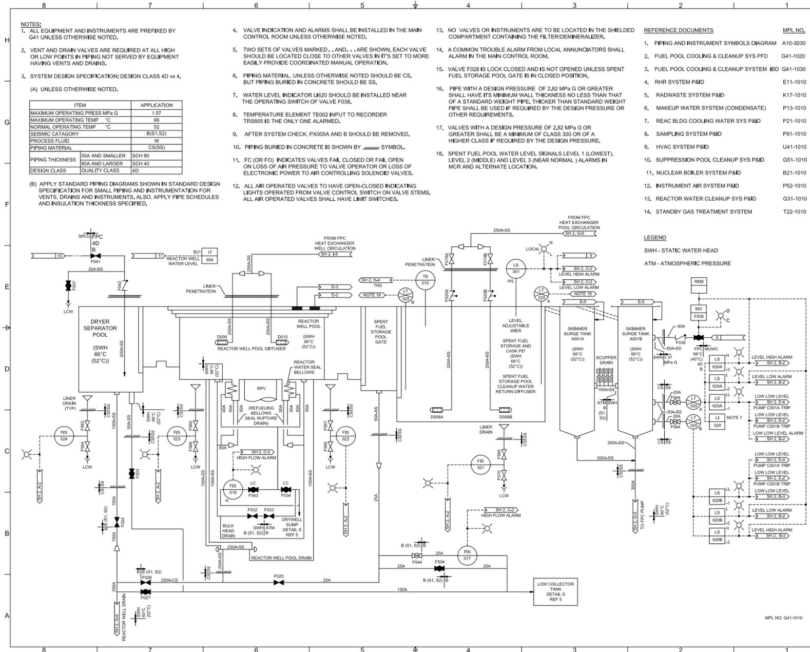
Figure 9.1-1 Fuel Pool Cooling and Cleanup System P&ID (Sheet 1 of 3)
