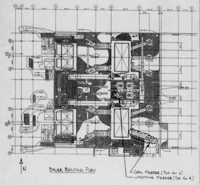
From Black and Veatch drawing no. 12713-1135A-MIIO4A showing location and platform accessibility to 10 feeders containing nuclear devices.
