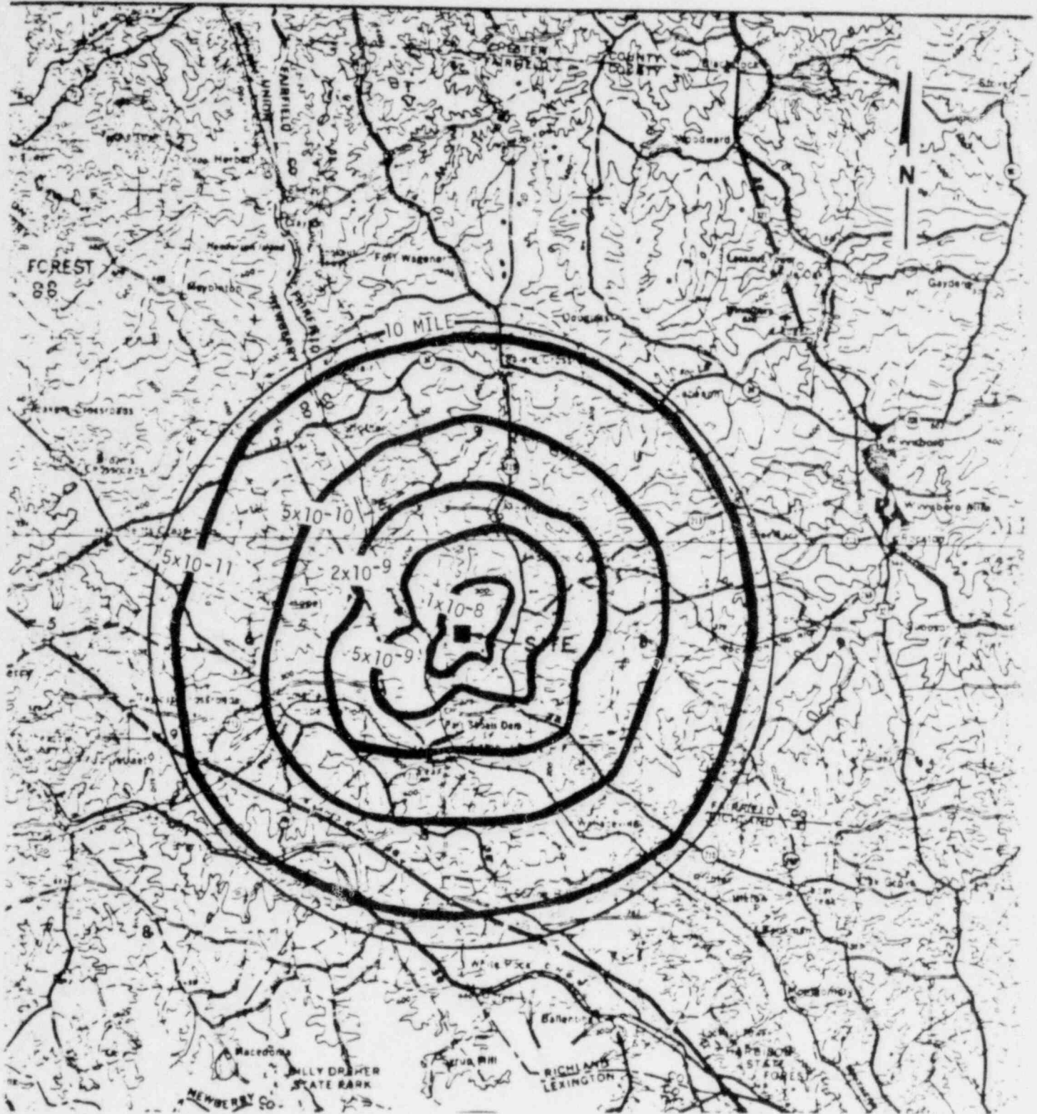
ISOPLETHS OF RISK OF LATENT CANCER FATALITY PER REACTOR YEAR TO AN INDIVIDUAL
