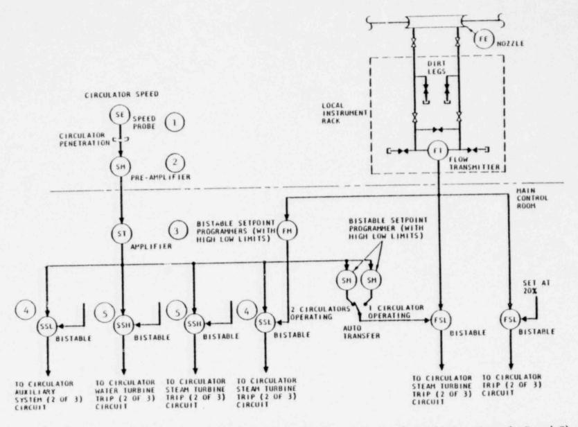
Circulator speed and feedwater flow instrument channels (typical for channels B and C)
