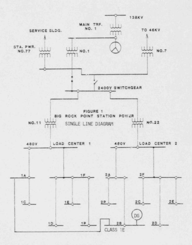
transformer No. 1 (from the unit generator on the 138kV grid) or by the 46kV grid.
