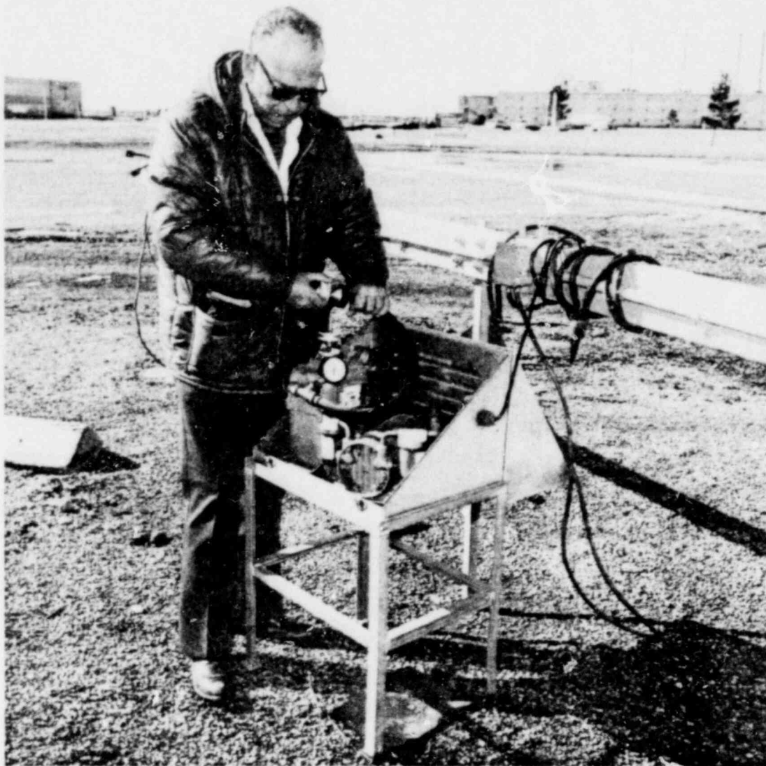
Figure 4. Technician changing the filter on a low-volume air sampler used at the INEL Site.
