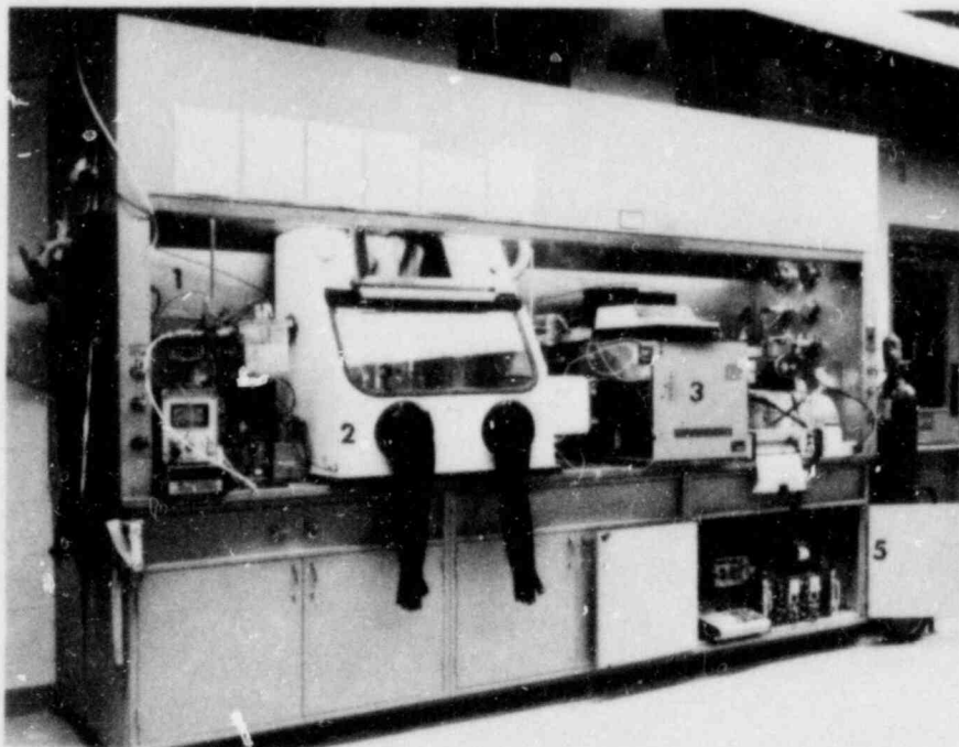
Respirator cartridges are tested against radioactive and nonradioactive iodine vapors in this experimental test apparatus at Los Alamos Scientific Laboratory (LASL). It was used to provide information on the use of respirators during early recovery operations after the TMI accident. The numbered sections are (1) airflow and humidity control, (2) radioiodine containment glovebox, (3) gas-chromatograph and methyl iodide samplers, (4) charcoal traps and detectors for radioiodine measurements, and (5) counting electronics and data logging.
