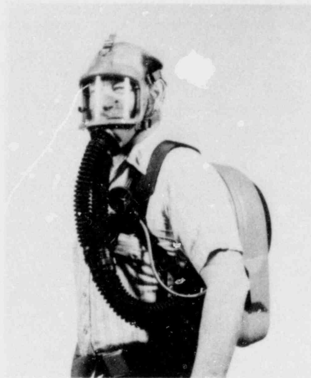
In this closed-circuit, self-contained breathing apparatus, air is supplied from the back-carried unit through one of the tubes to the mask. The exhaled air returns through the other tube to the back unit for cleaning, restoration to breathing quality and recirculation. LASL tests such respirators and makes recommendations to the NRC.
