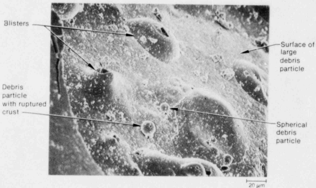
Figure 17. Scanning electron photomicrographs of the surface of debris particles from the RIA-ST-4 experiment.
