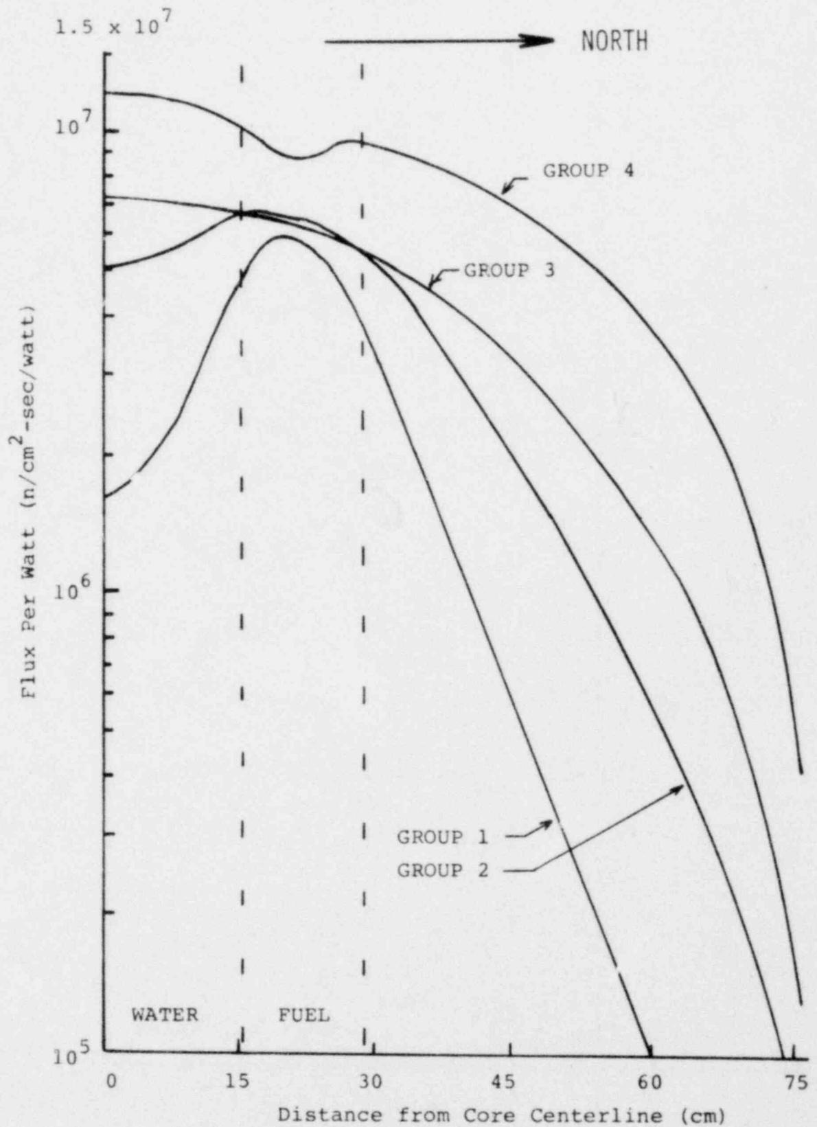
Figure 4-16. Group-Dependent Fluxes Along the North-South Direction--CORA Code Calculations. (23)
