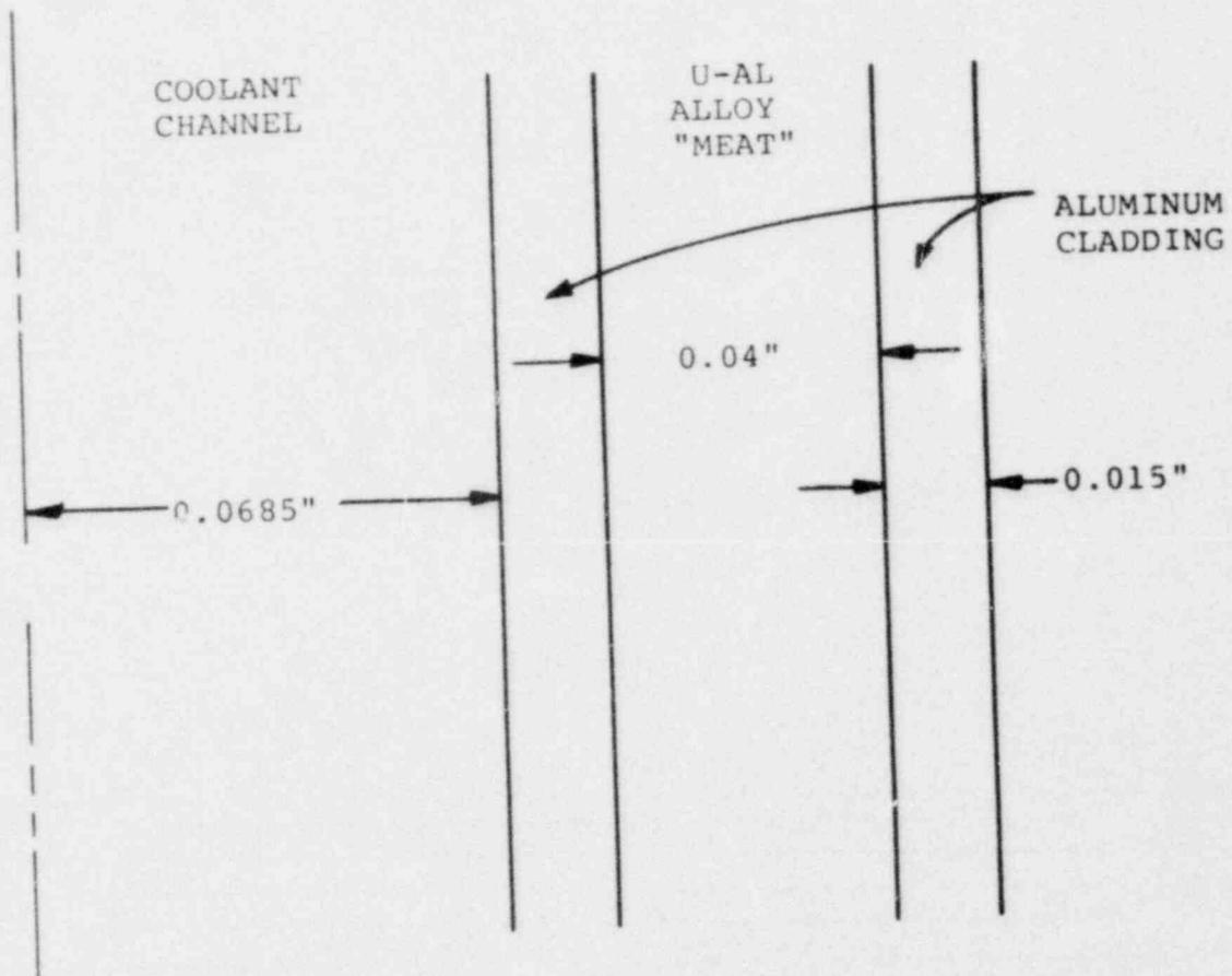
Figure 4-12. Fuel Plate/Coolant Channel Enlargement Showing UFTR Fuel Cell Arrangement Detail.
