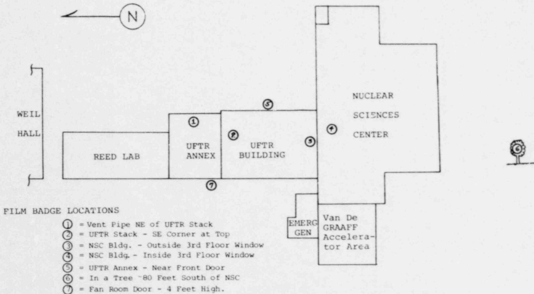
Figure 12-9. Location of Film Badges Used for Monitoring UFTR Site and Environs.
