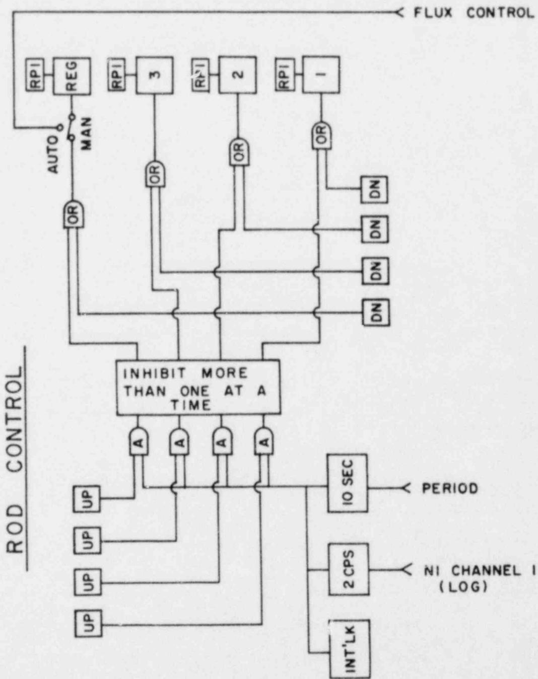
Figure 7-5. ROD CONTROL: UFTTR Control-Blade (Rod) Withdrawal Inhibit System.
