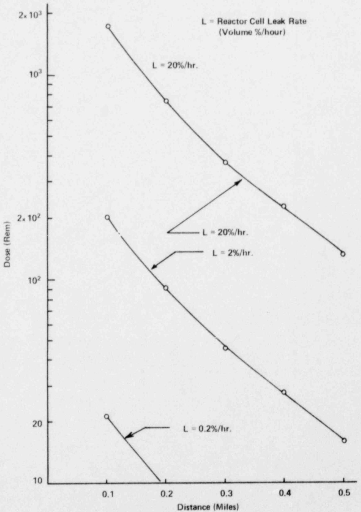
Figure 15-6. Two-Hour Thyroid Dose for UFTR Operation at 100 KWth Using NRC Standard Meteorology.
