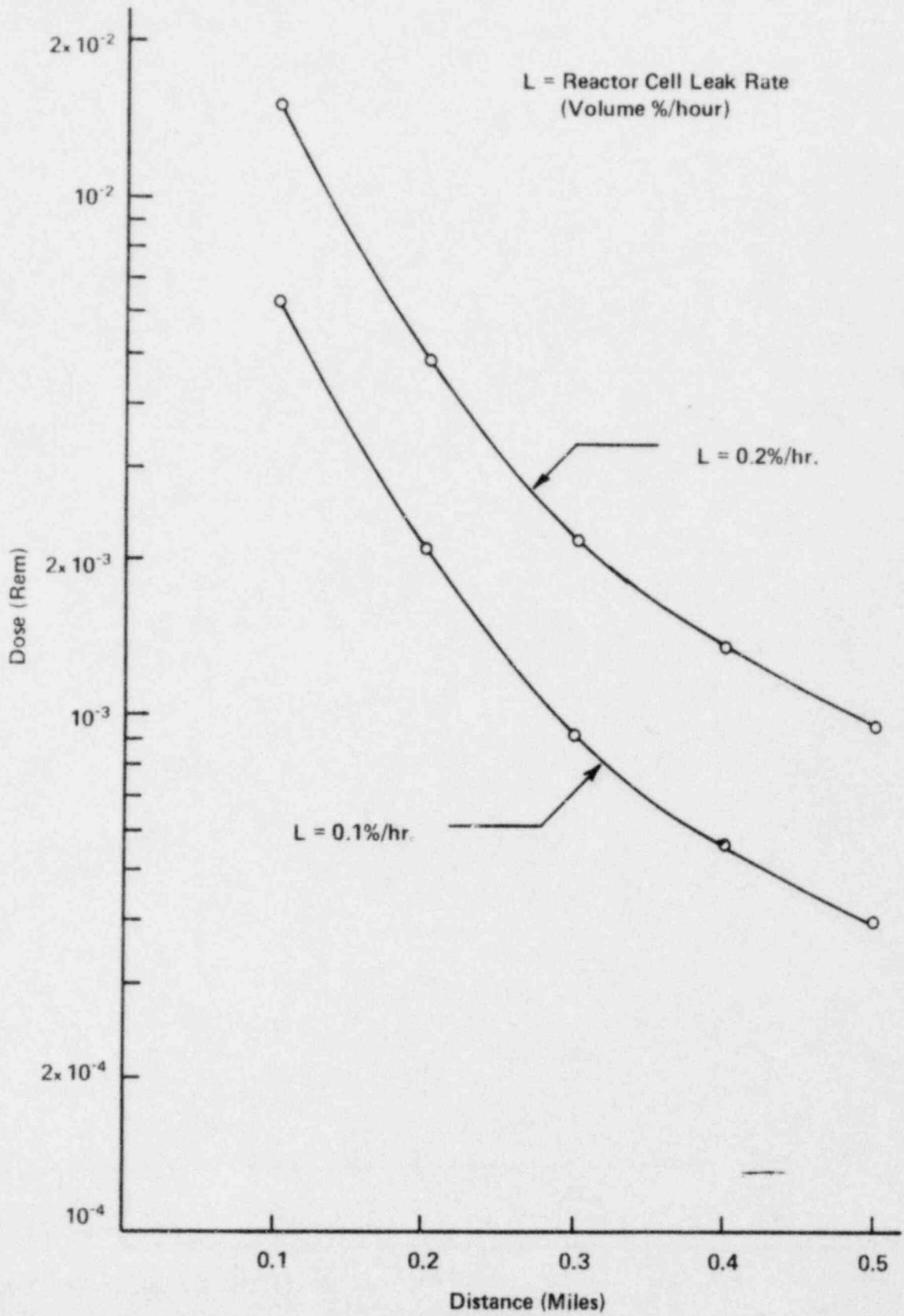
Figure 15-9. Two-Hour Whole Body Dose for UFTR Operation at 100 KWth Using Local Meteorology.
