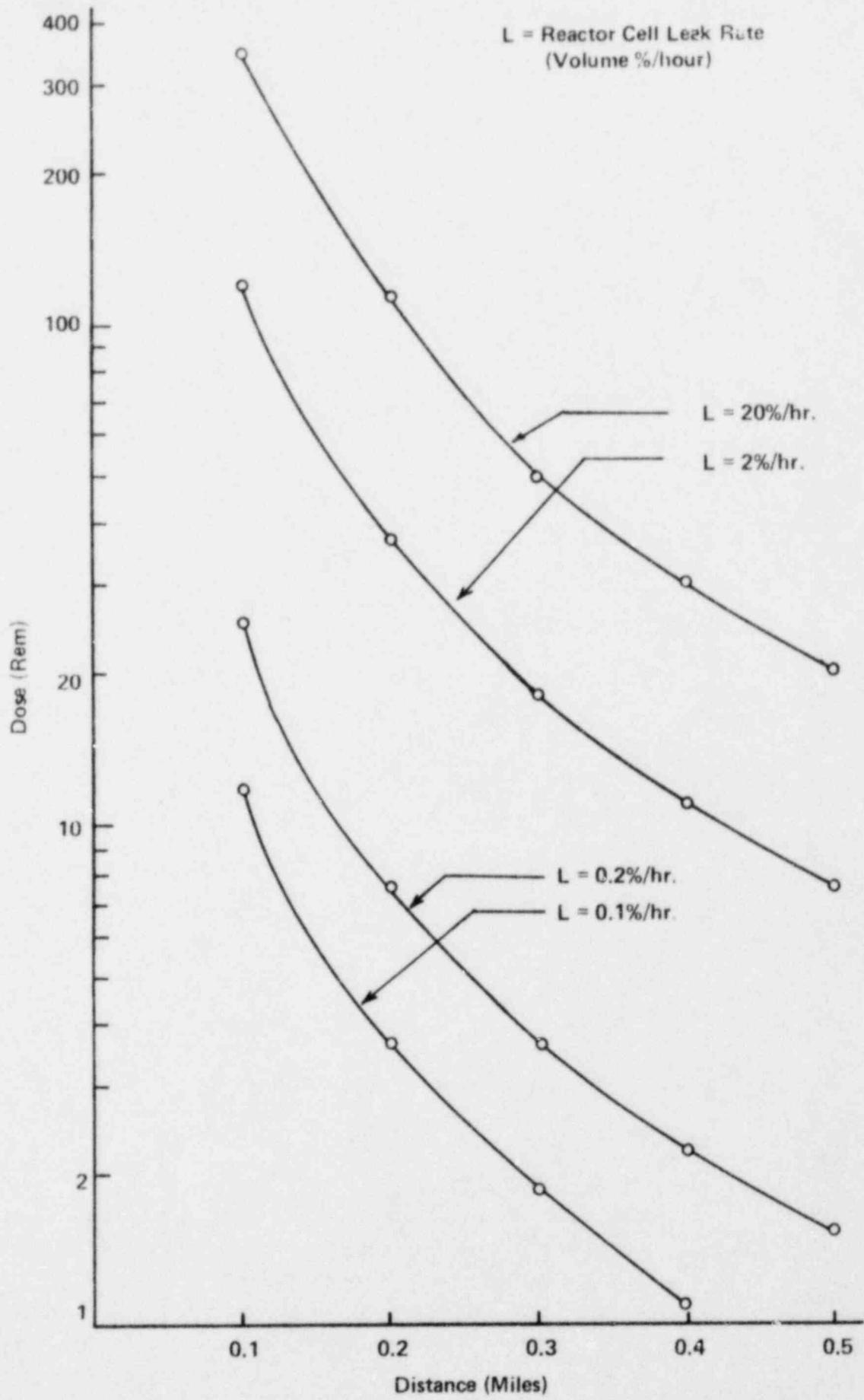
Figure 15-5. Thirty Days Thyroid Dose for UFTR Operation at 100 KWth Using Local Meteorology.
