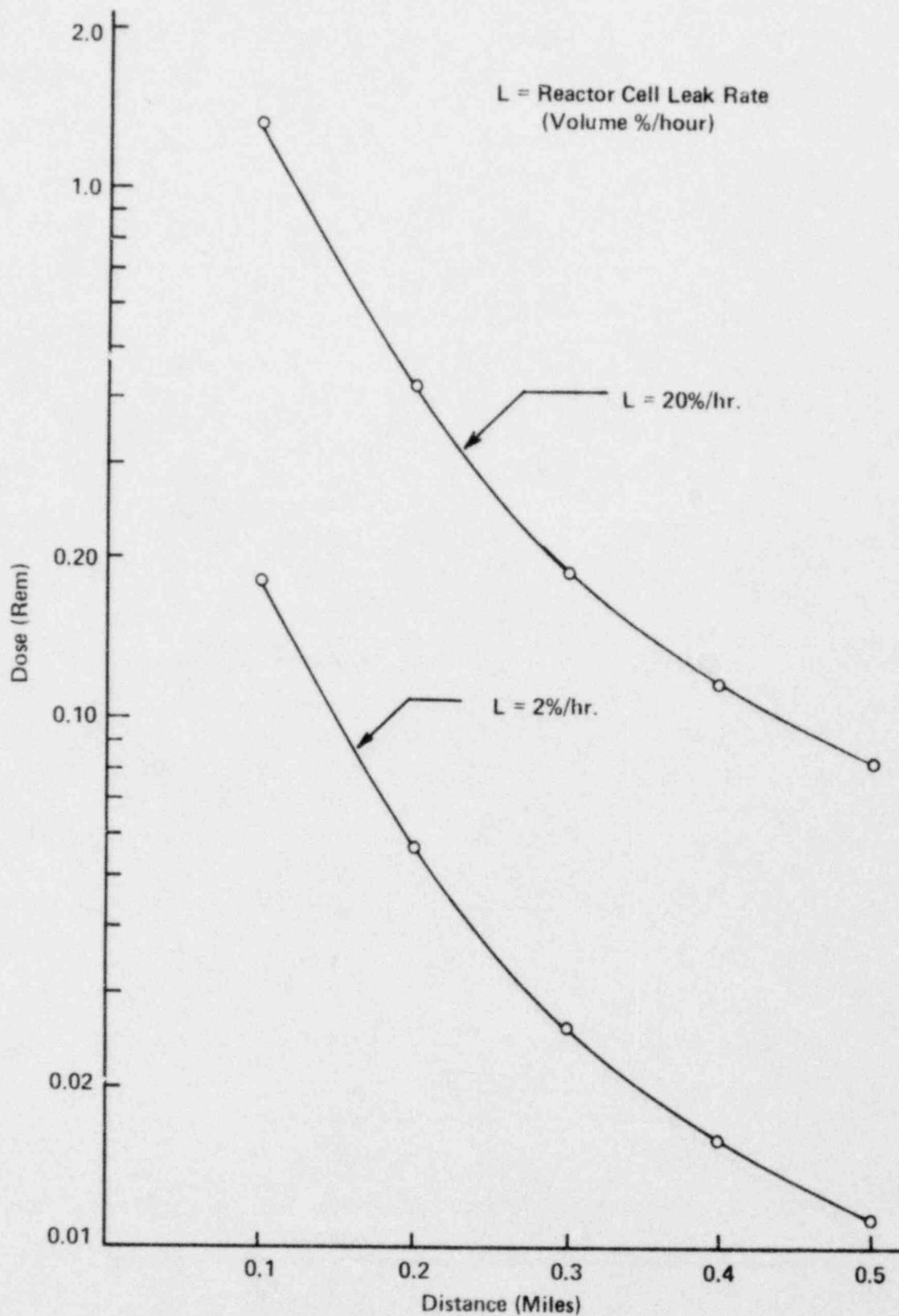
Figure 15-8. Two-Hour Whole Body Dose for UFTR Operation at 100 KWth Using Local Meteorology.
