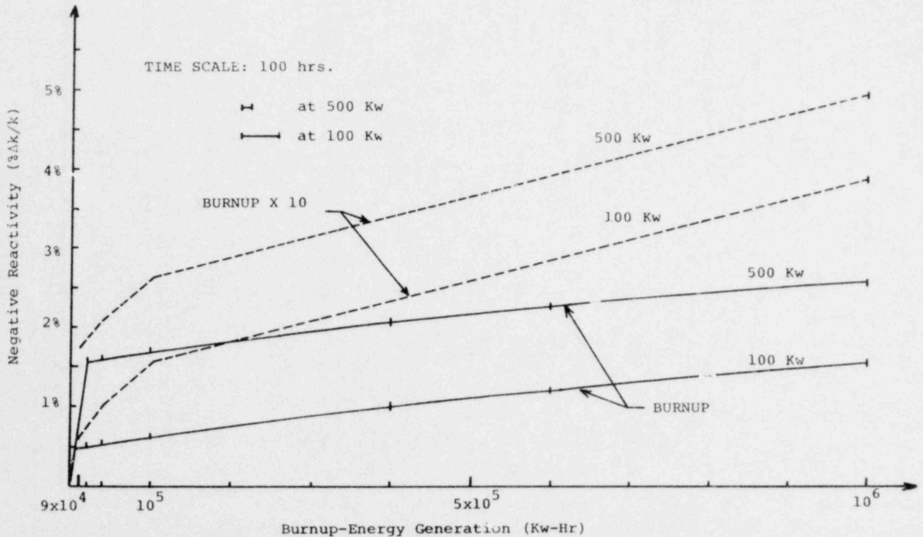
Figure 4-21. Reactivity Drop with Burn-up for Operation at 100 and 500 KW.
