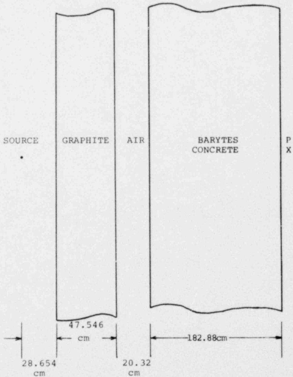
Figure 12-8. Core Gamma Shielding Model for North or South Face of the UFTR.
