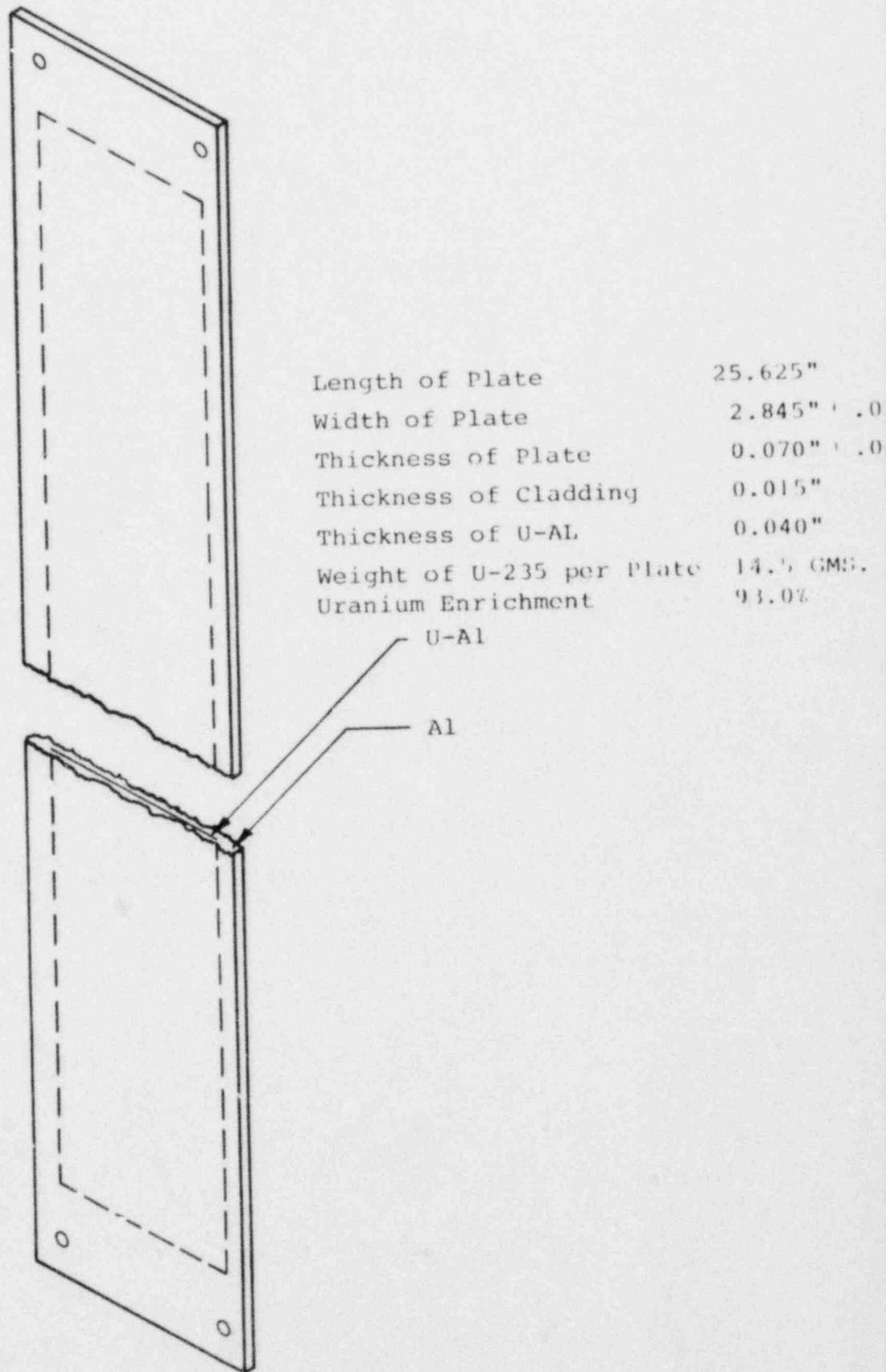
Figure 4-10. Schematic Showing UFTR Fuel Plate Geometry.
