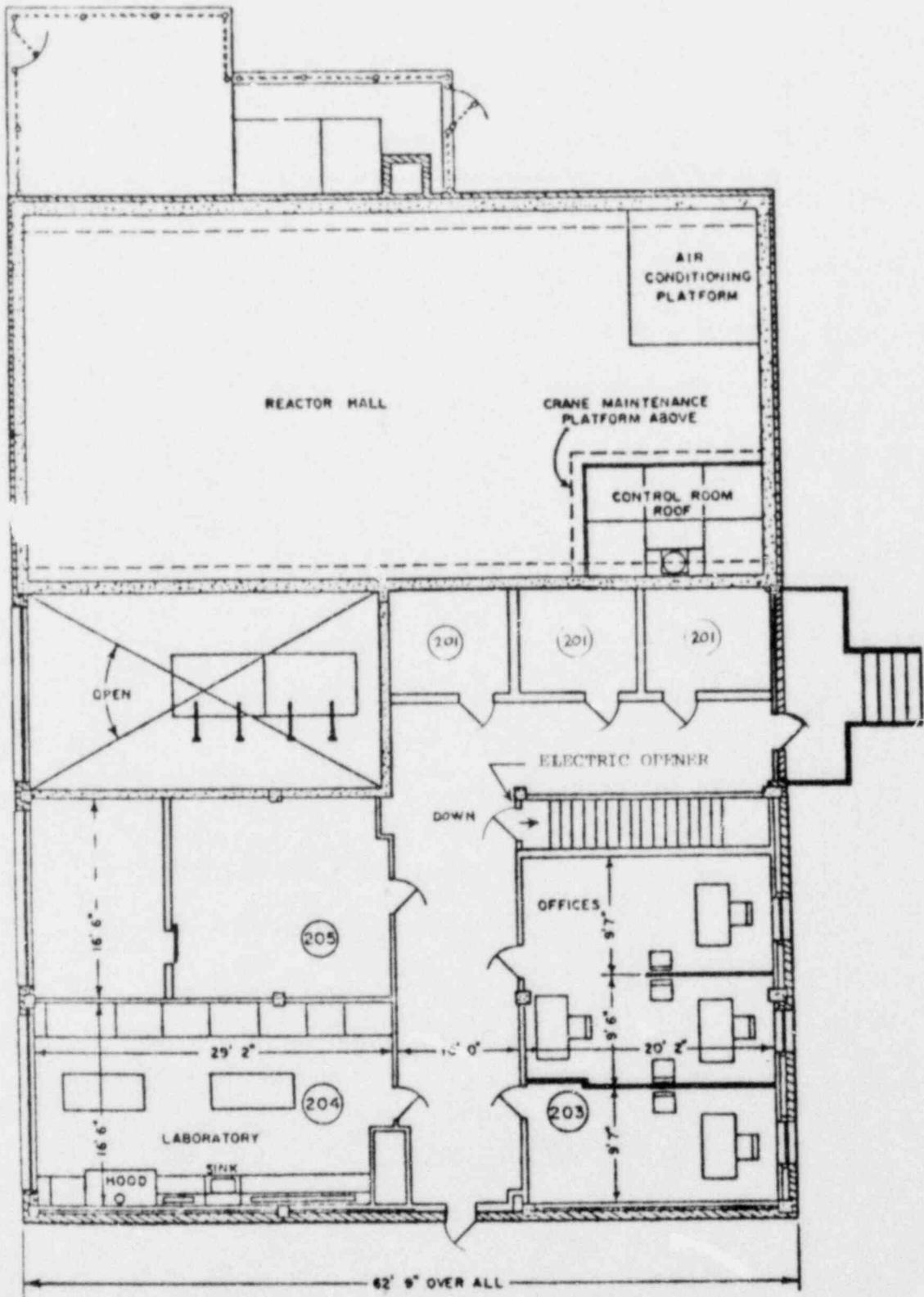
Figure 3-3. Second Floor Plan for the University of Florida Training Reactor Building
