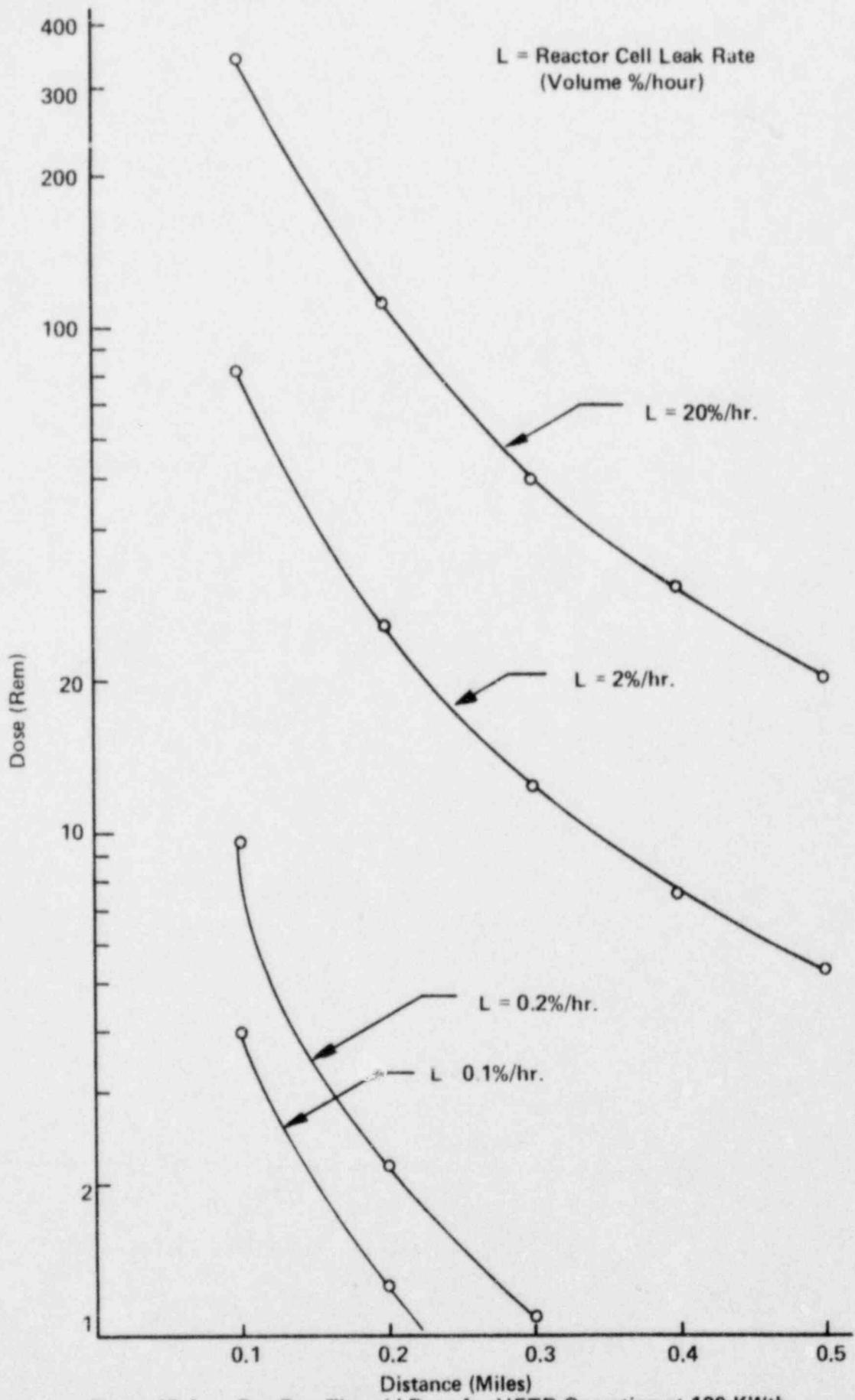
Figure 15-4. One Day Thyroid Dose for UFTR Operation at 100 KWth Using Local Meteorology.
