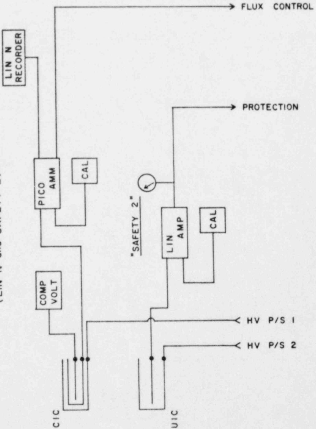
Figure 7-4. Nuclear Instrumentation Channel 2 (Linear N and Safety #2 Channels).
