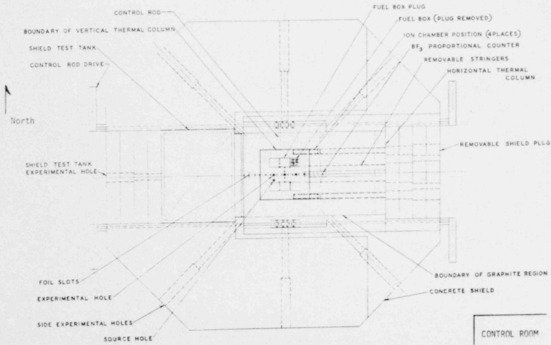
Figure 4-7. Geometric Arrangement of Major UFTR Experimental Facilities.
