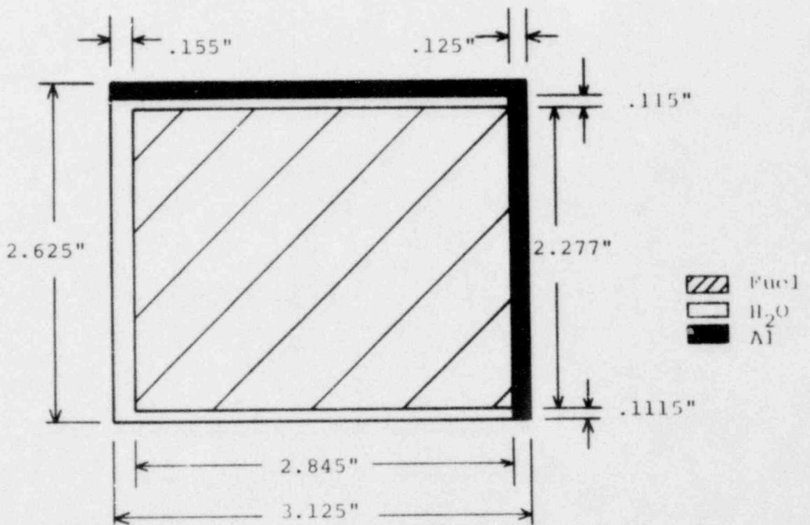
Figure 4-14B. UFTR Quarter Fuel Box Unit Assembly.
