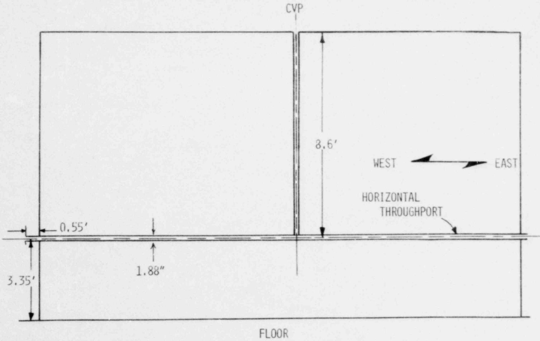
Figure 4-6. UFTR Cross Section Showing Center Vertical Port (CVP) and East-West Through Port (EWTP) Arrangement with Dimensions. (Not to scale)
