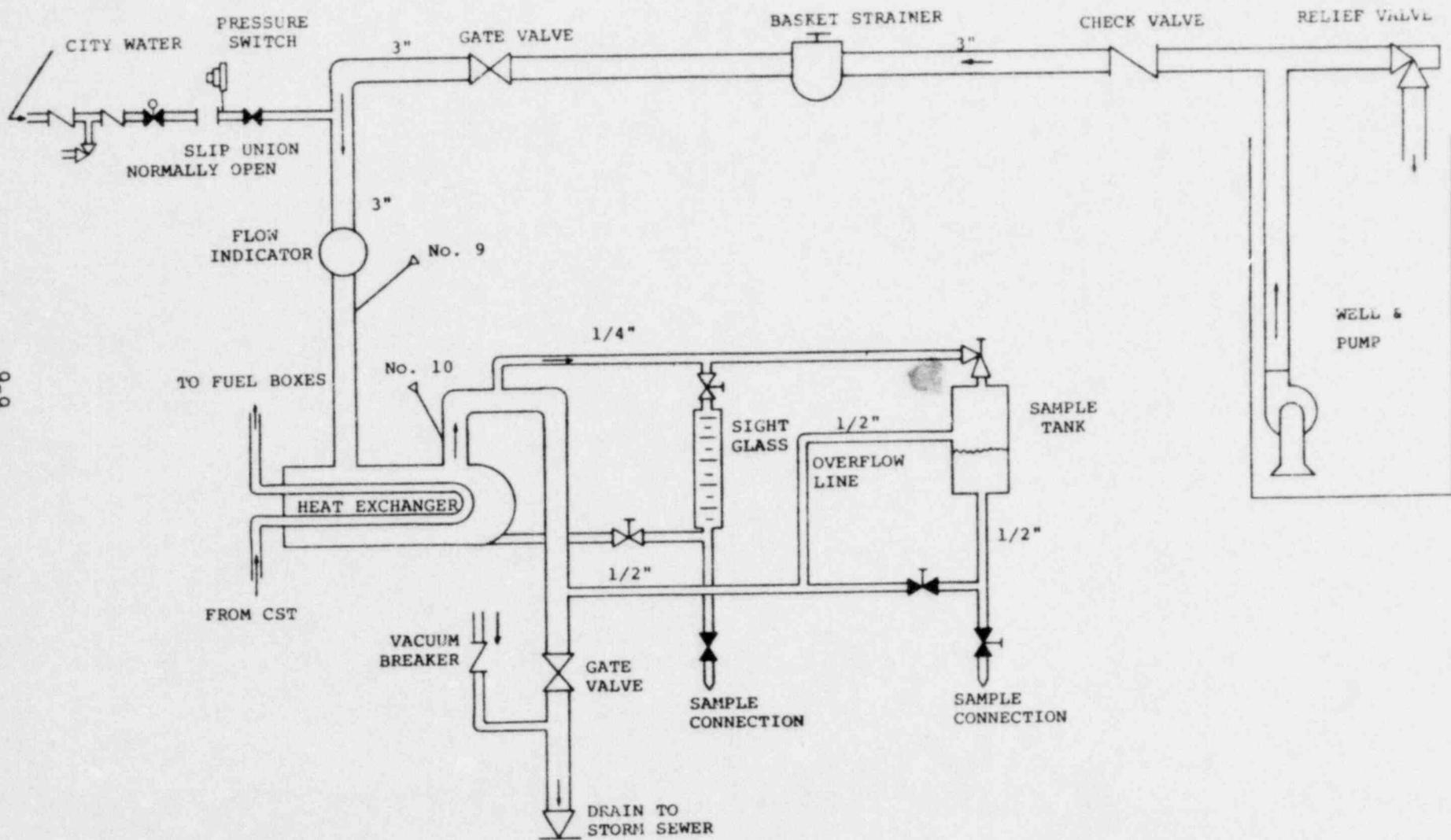
Figure 9-3. UFTR Secondary Water Cooling System.
