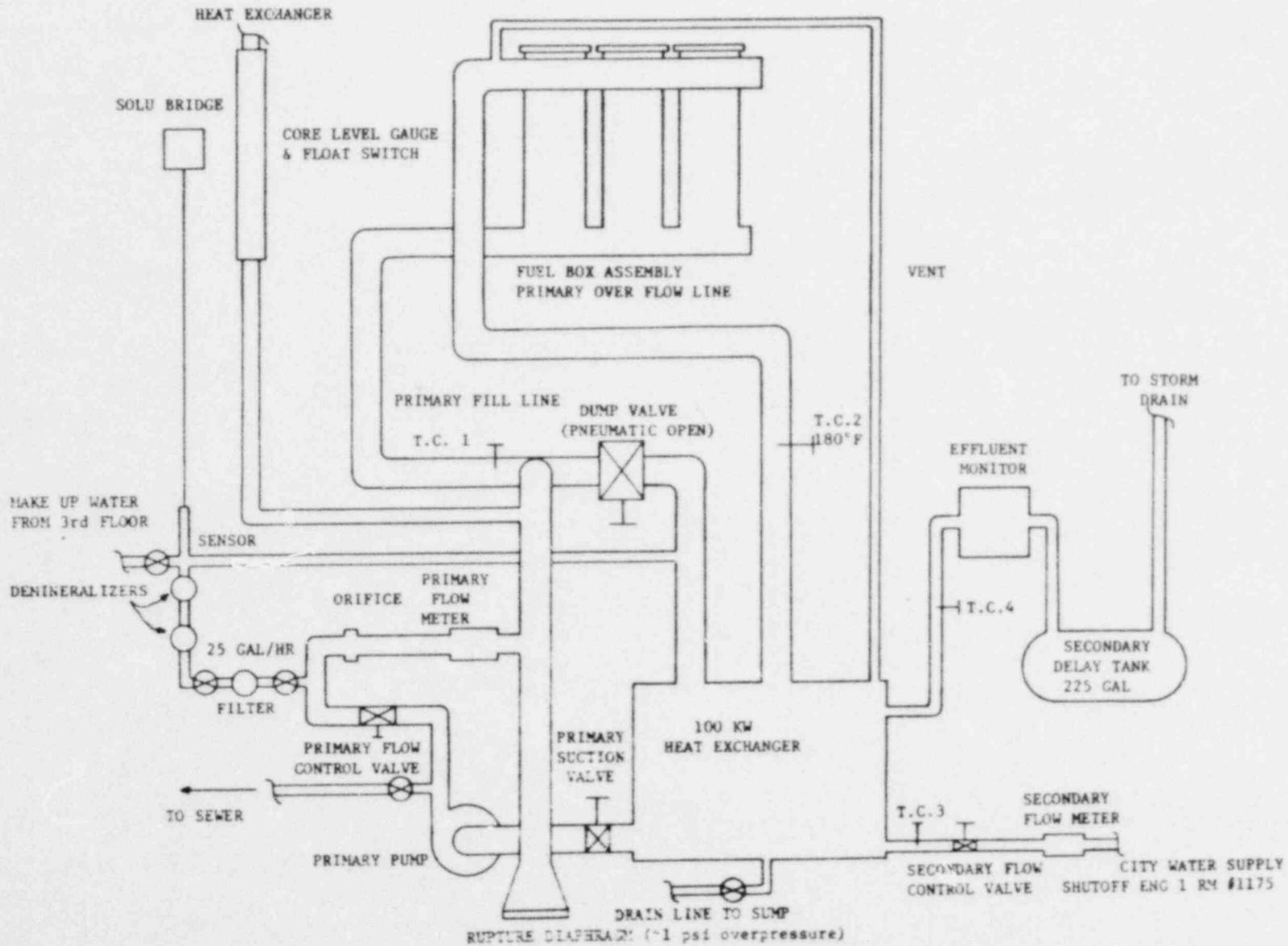
Figure 1-3. UCLA R-1 Reactor Cooling Systems.
