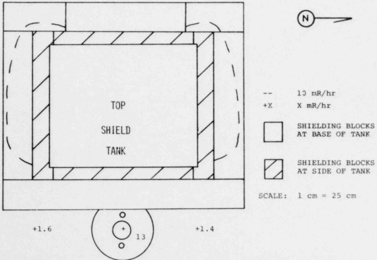
Figure 12-6. Gamma Exposure Rates Around the UFTTR Shield Tank for 100 KWth Operation with Readings Made At the Top of Base Shielding (25 cm above the reactor surface).
