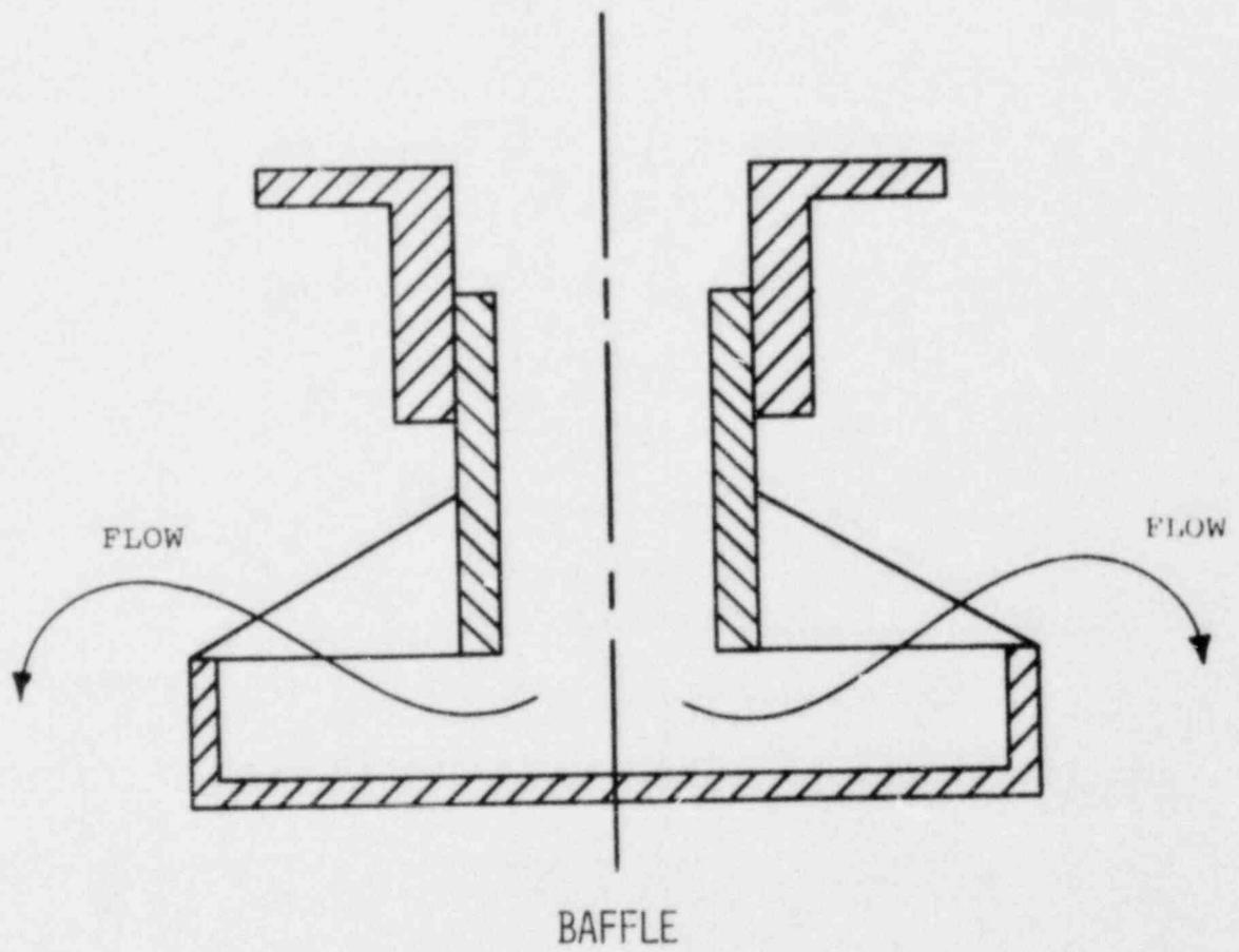
Figure 5-3. UFTTR Coolant Storage Tank Aluminum Bucket Baffle.
