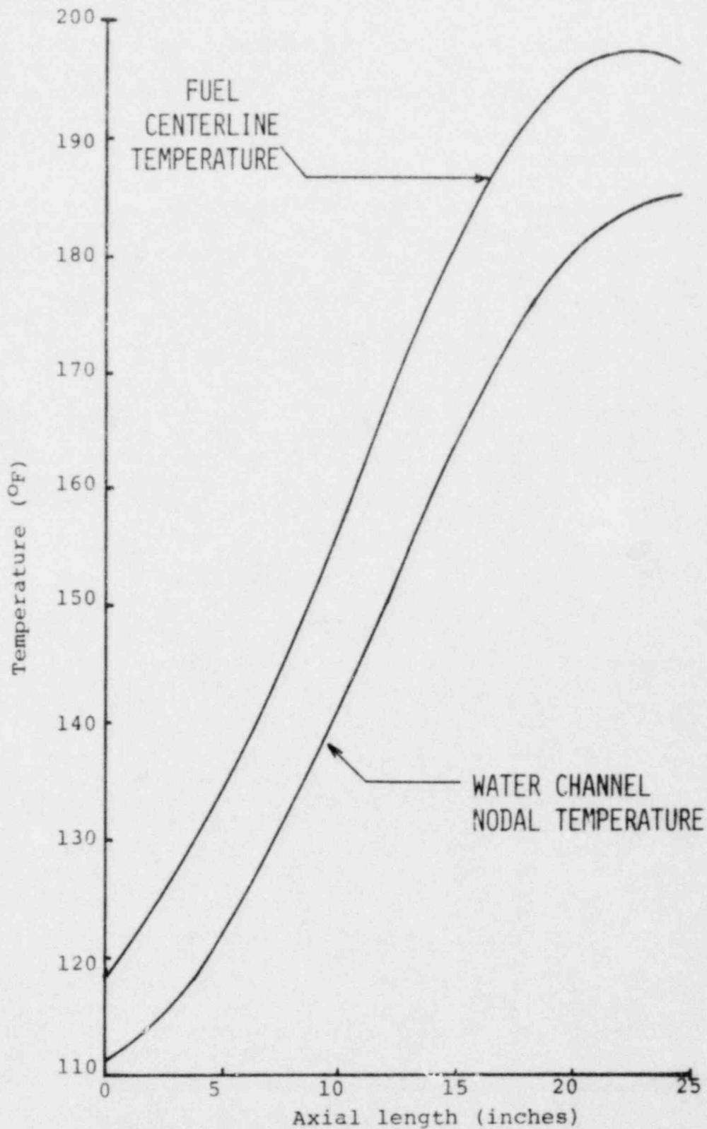
Figure 4-24. Temperature Distribution of the "Hottest" Fuel Plate and Water Channel at 500 KWth (Coolant Flow Rate = 65 gpm).
