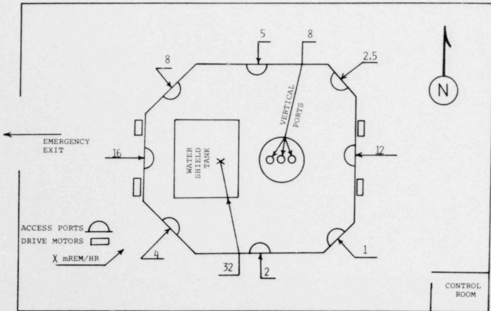
Figure 12-3. Results of Radiation Survey Around UFTR at 100 KWth Power Operation. (23)
