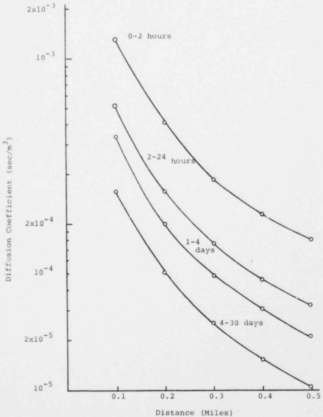
Figure 2-23. Design Basis Accident Diffusion Coefficients with Site-Specific Meteorology for Several Short-Term Time Periods.
