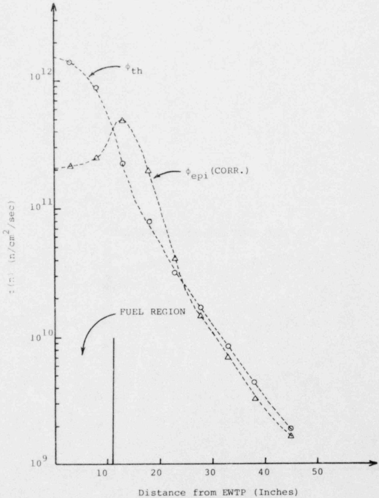
Figure 4-13. UFTR Absolute Flux Measurements Results in CVP (Gold Foil). (5)
