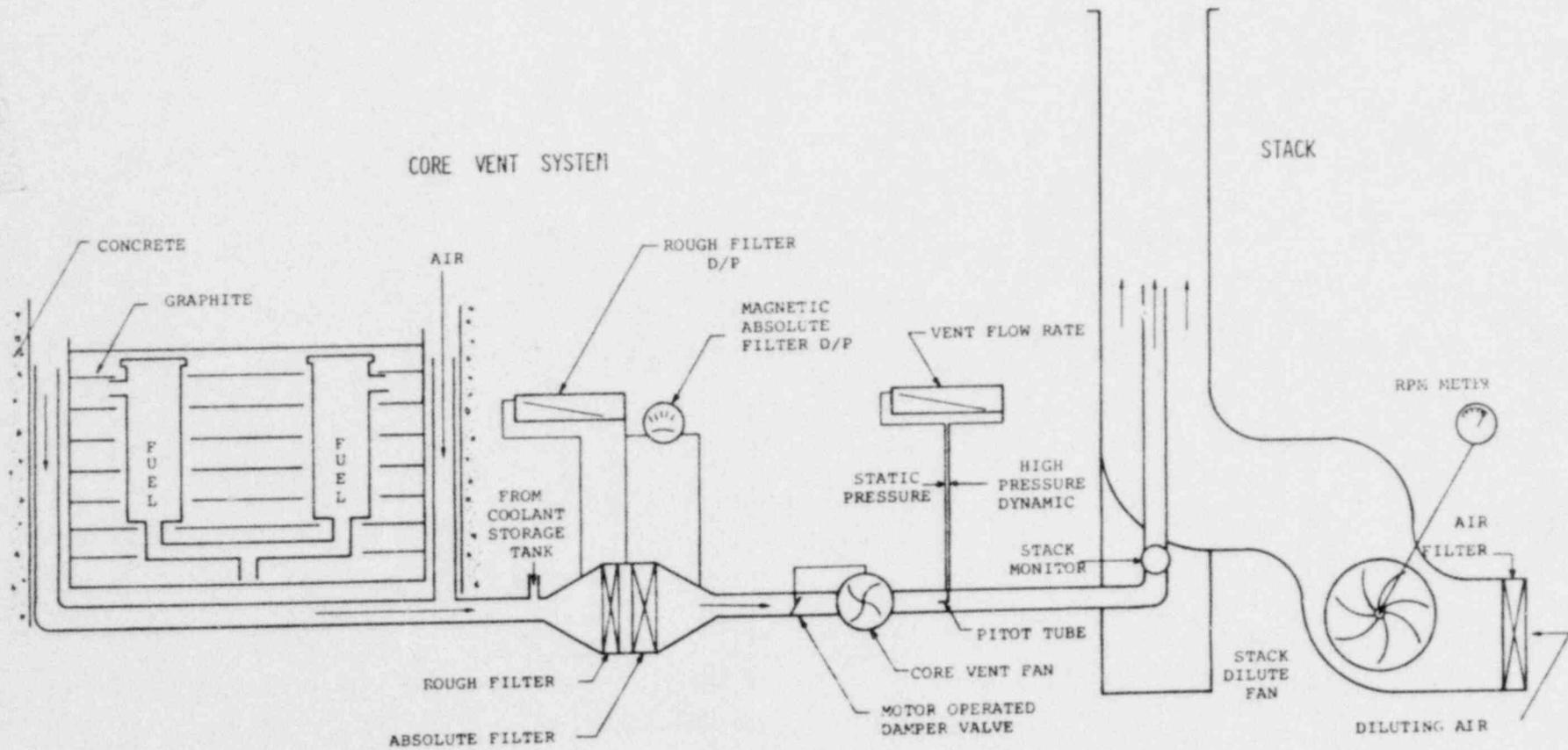
Figure 9-5. Side-View Schematic Diagram of UFTR Core Vent System.
