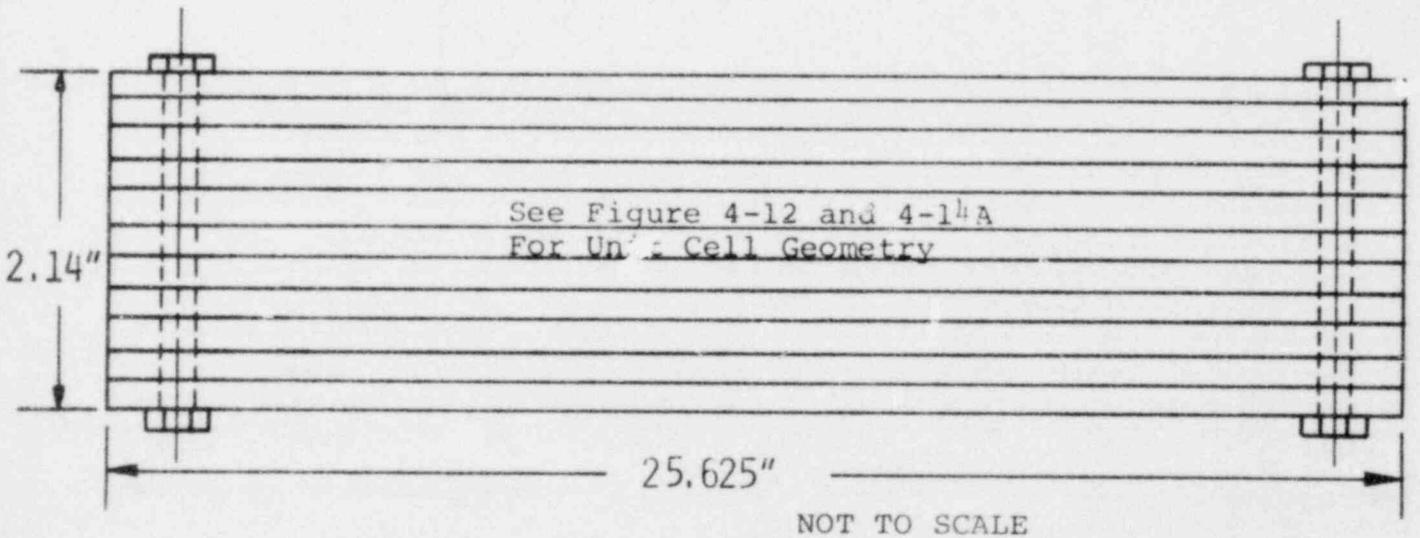
Figure 4-11. UFTR Fuel Plate and Fuel Bundle Geometric Arrangement.
