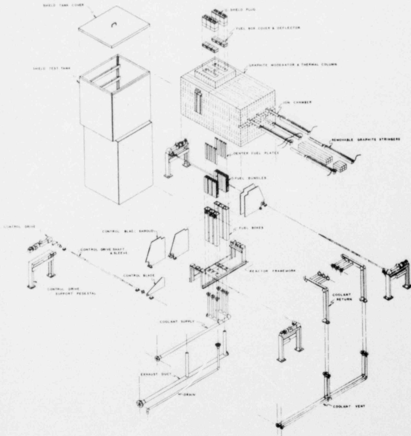
Figure 4-5. Isometric Diagram of UFTR Components.
