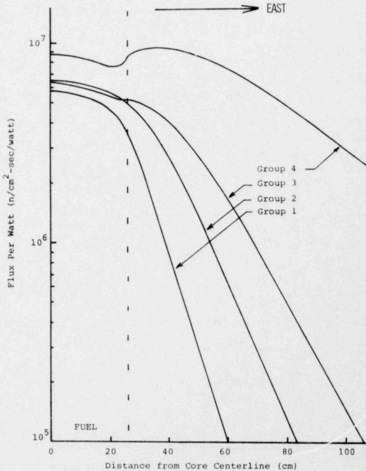
Figure 4-17. Group-Dependent Fluxes Along the East-West Direction--CORA Code Calculation (23)
