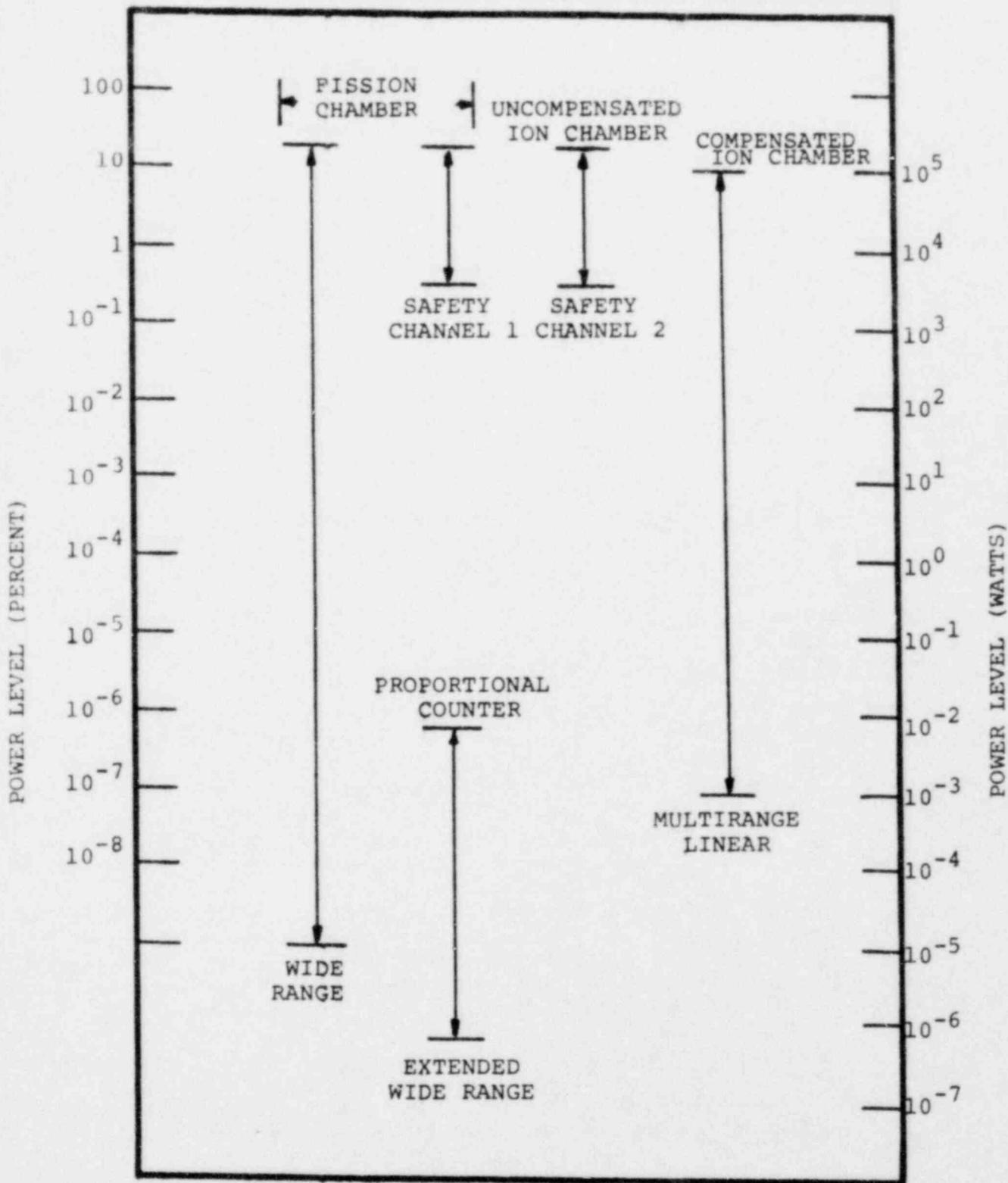
Figure 7-2. Operating Range of UFTR Neutron/Power Level Detectors.
