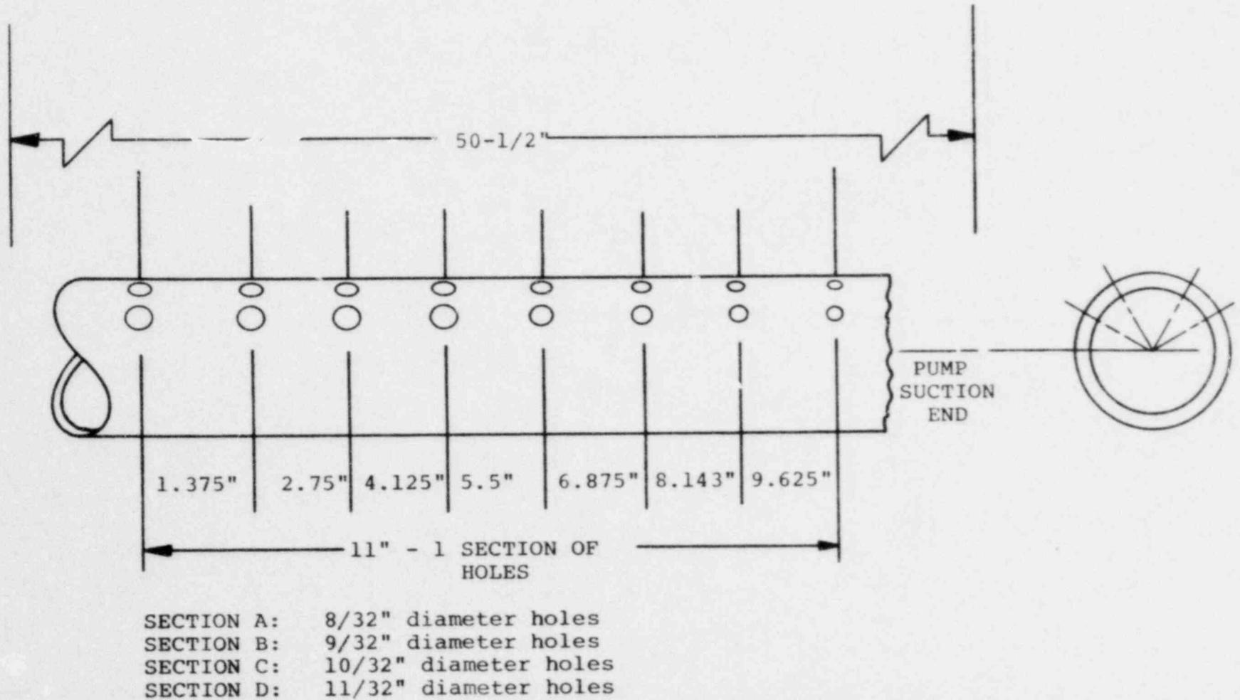
Figure 5-2. UFTTR Storage Tank Diffuser Arrangement (Vortex Eliminator)
