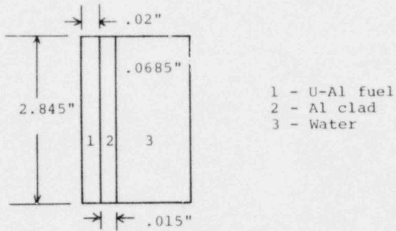
Figure 4-14A. UFTR Fuel Plate Unit Cell
