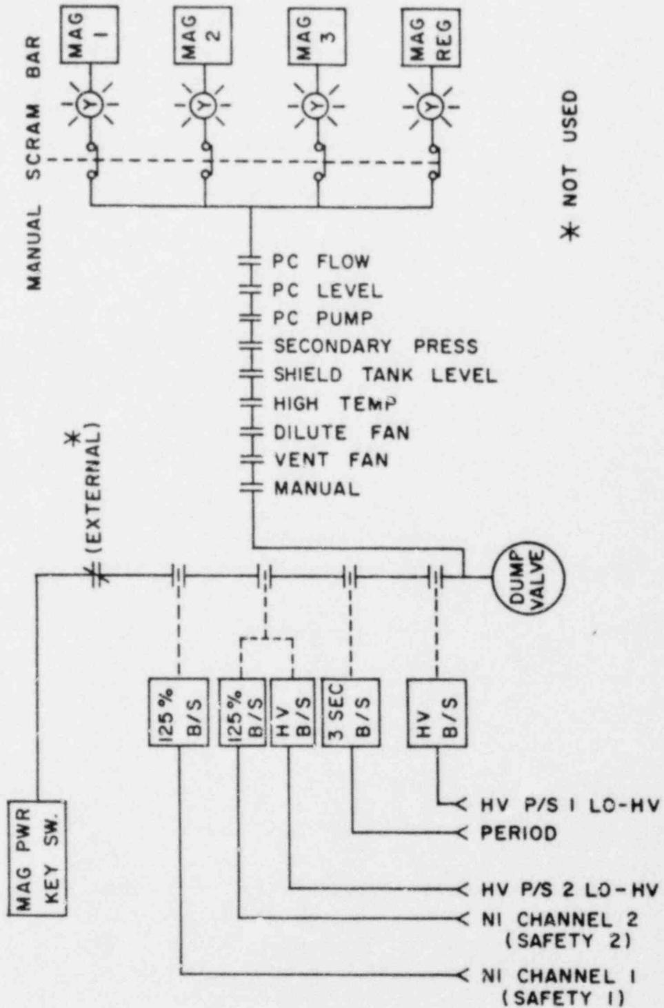
Figure 1-7. PROTECTION: Schematic Diagram of the UFTR Reactor Protection System.
