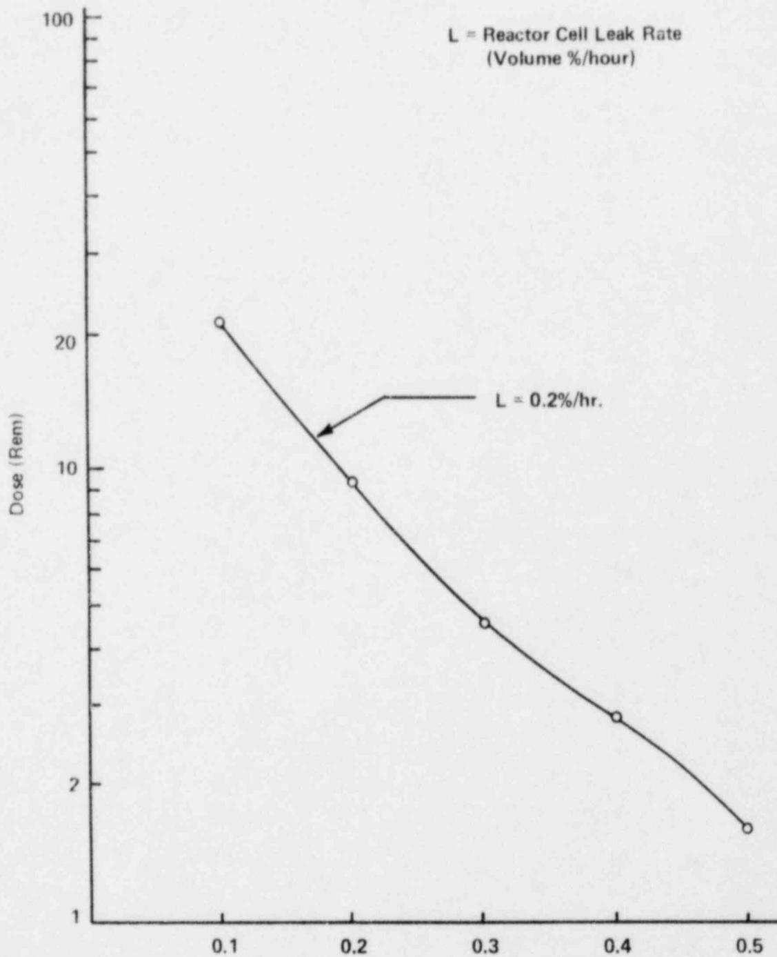
Figure 15-7. Two-Hour Thyroid Dose for UFTR Operation at 100 KWth Using NRC Standard Meteorology.
