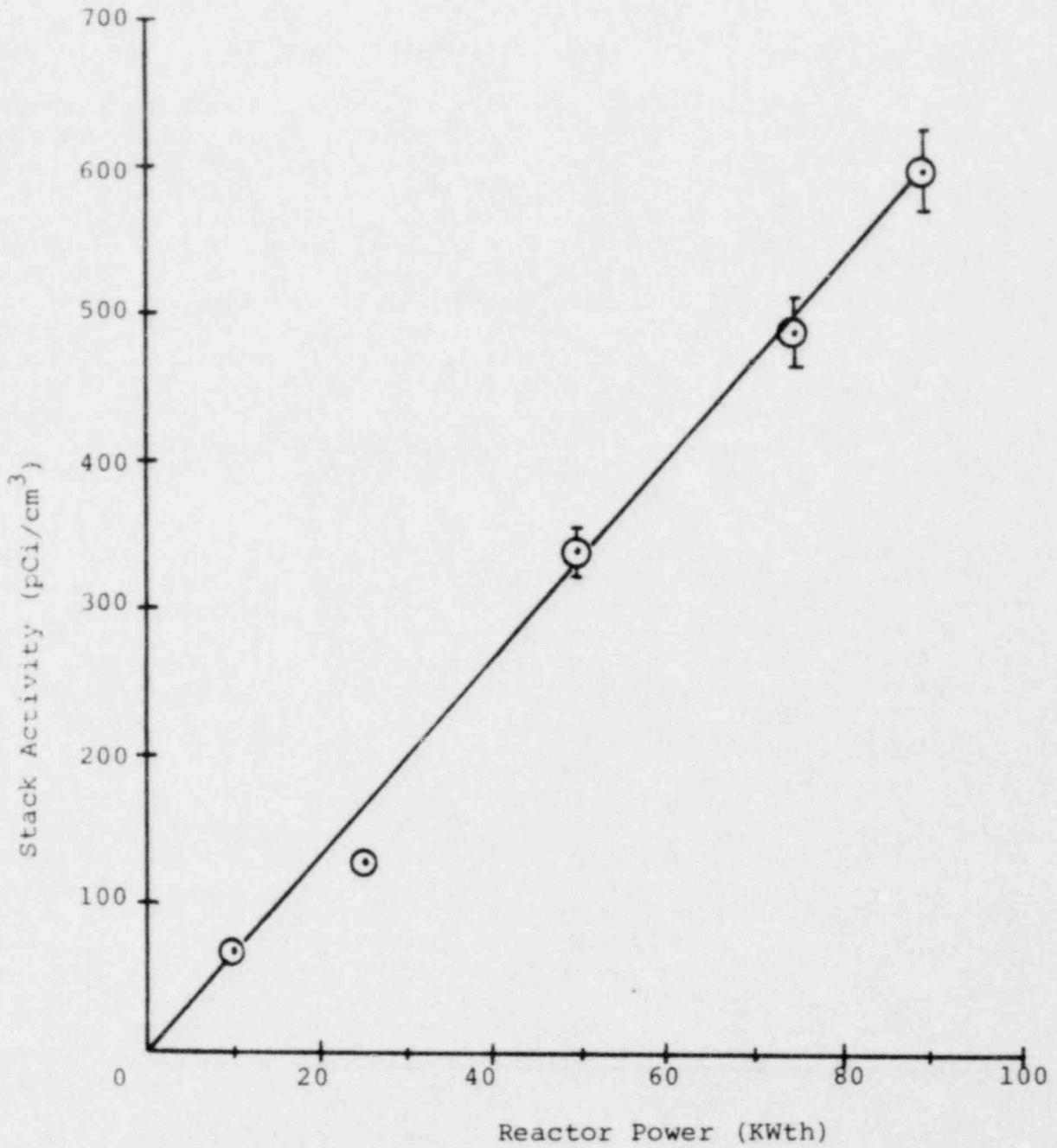
Figure 11-2. Experimental Determination of Argon-41 Stack Concentration Variation With UFTR Operating Power. (31)
