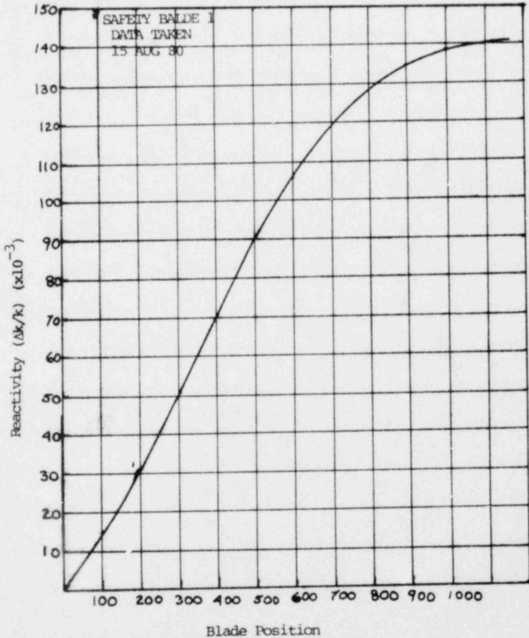
Figure 4-26. Reactivity Integral Rod Worth Curve for UTR Safety Blade #1.
