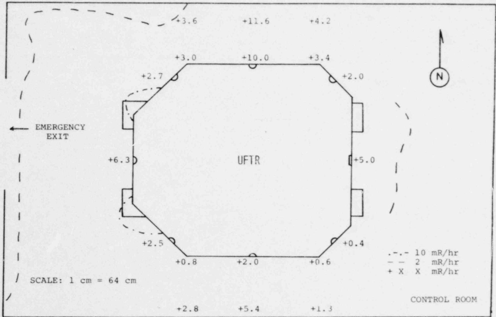
Figure 12-4. Gamma Exposure Rates at Port Level for 100 KWth Operation With No External Shielding and Top Shield Block Removed.
