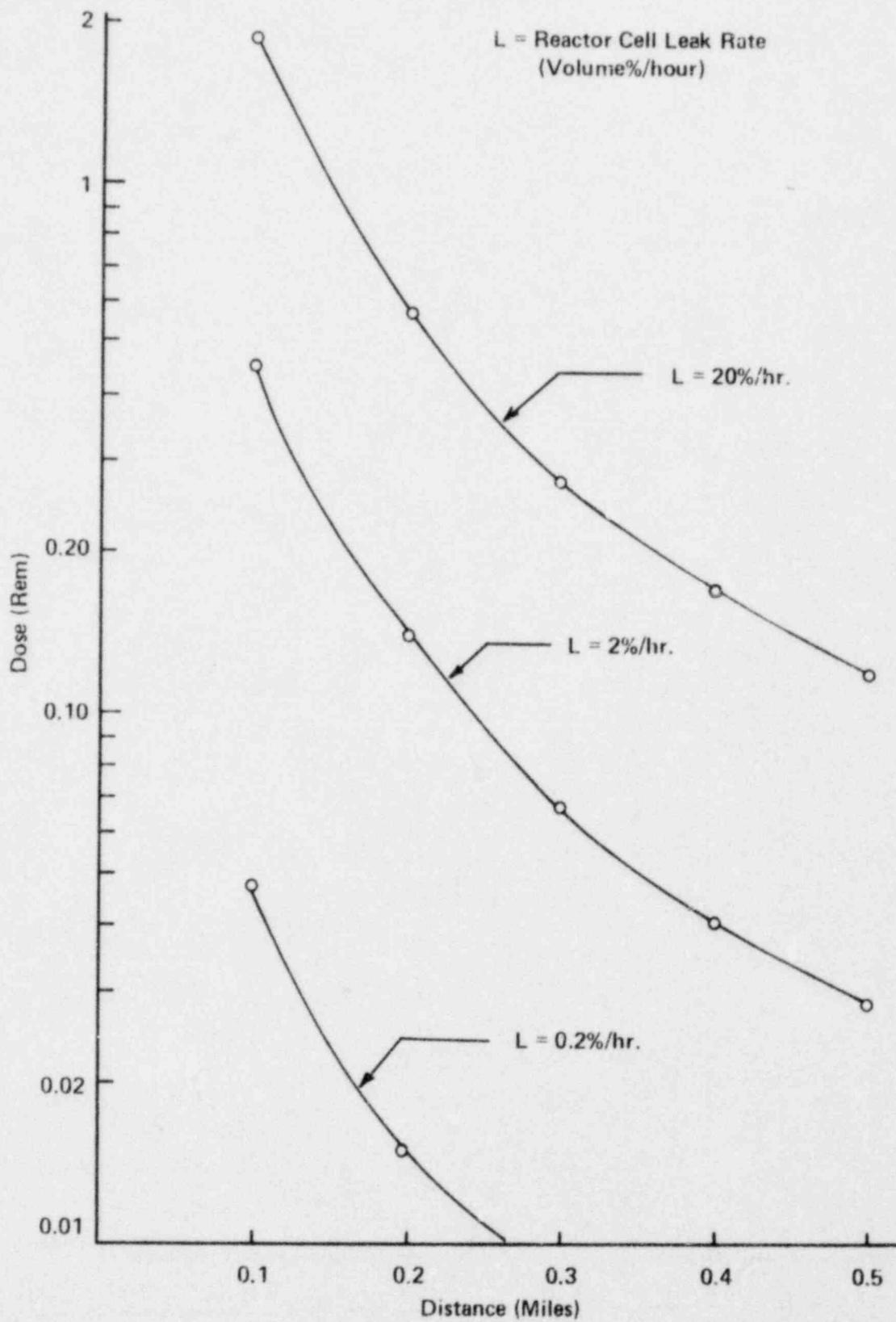
Figure 15-10. One Day Whole Body Dose for UFTR Operation at 1000 kWth Using Local Meteorology.
