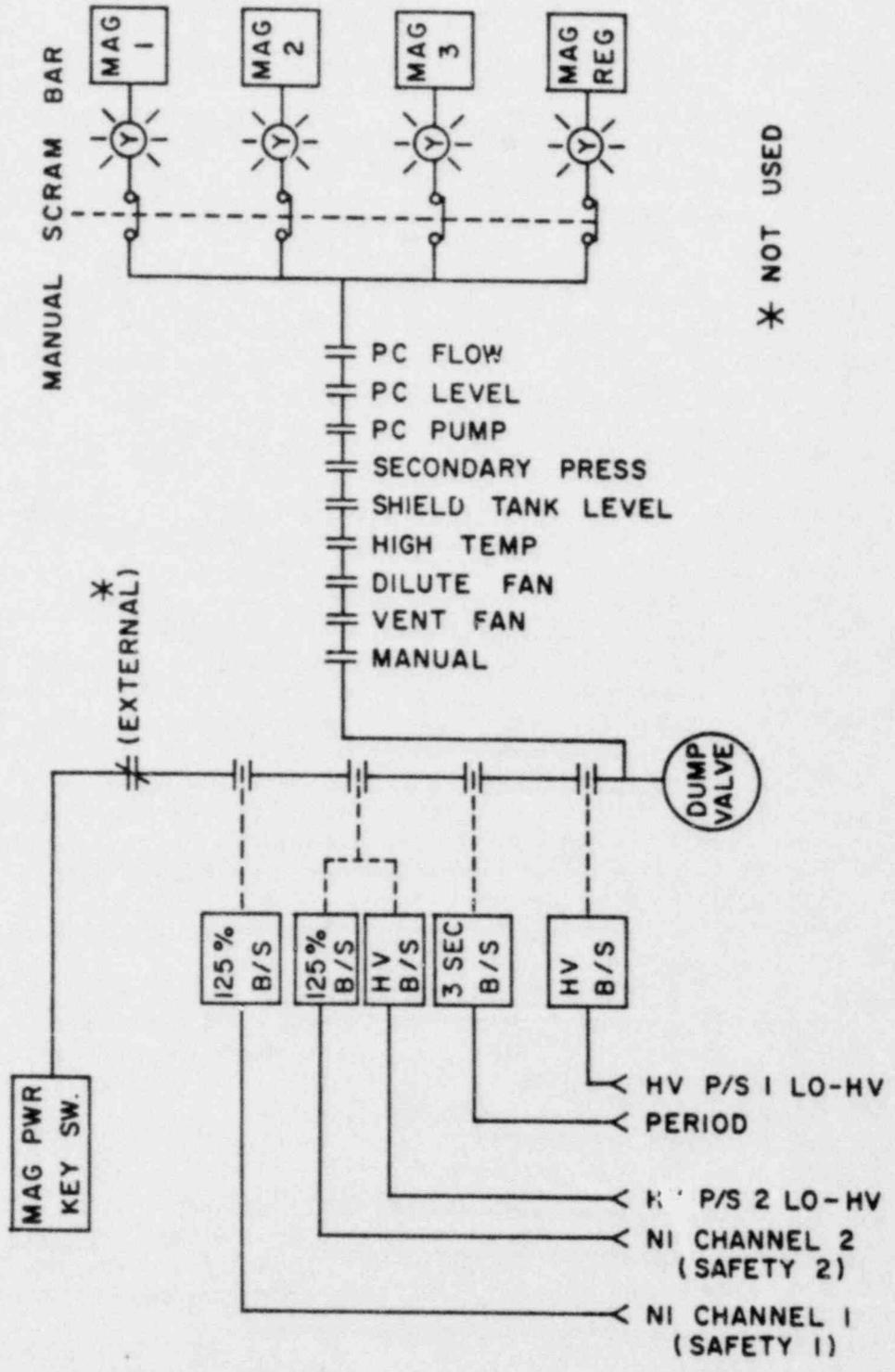
Figure 7-7. PROTECTION: Schematic Diagram of the UFTR Reactor Protection System.
