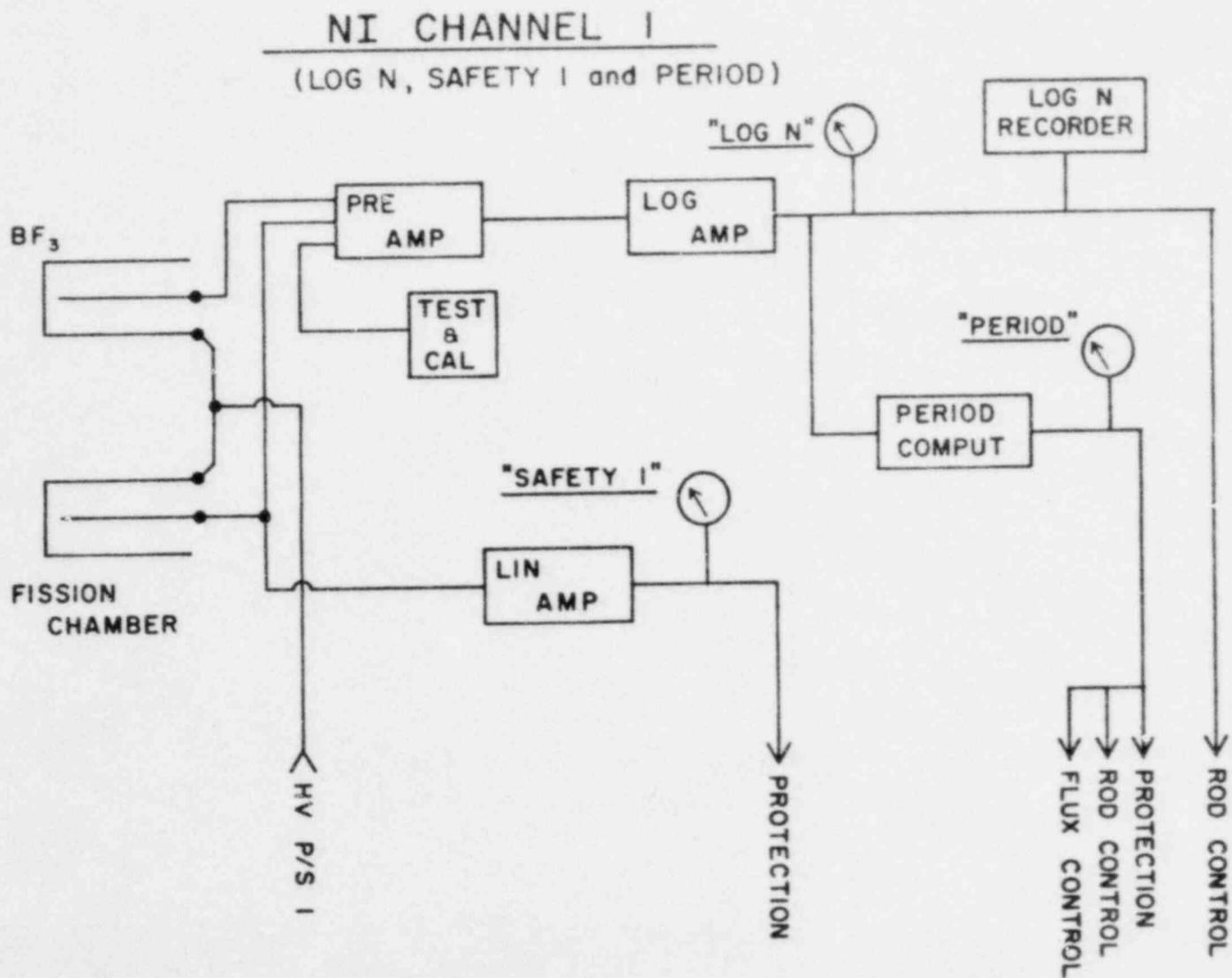
Figure 1-8. NI CHANNEL 1: UFTR Nuclear Instrumentation Channel 1 Diagram (Log N, Safety #1 and Period Channels).
