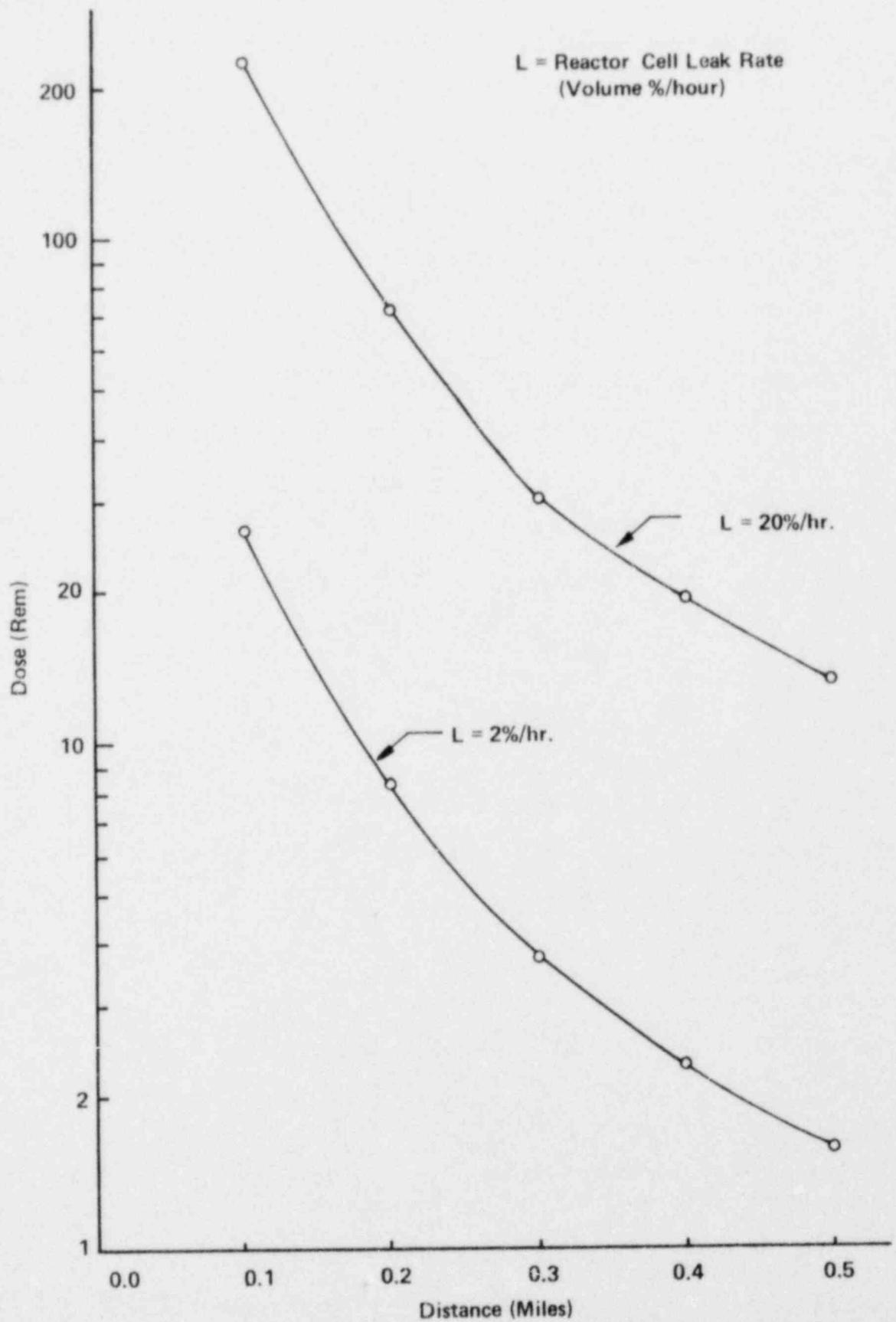
Figure 15-2. Two-Hour Thyroid Dose for UFTR Operation at 100 KWth Using Local Meterology.
