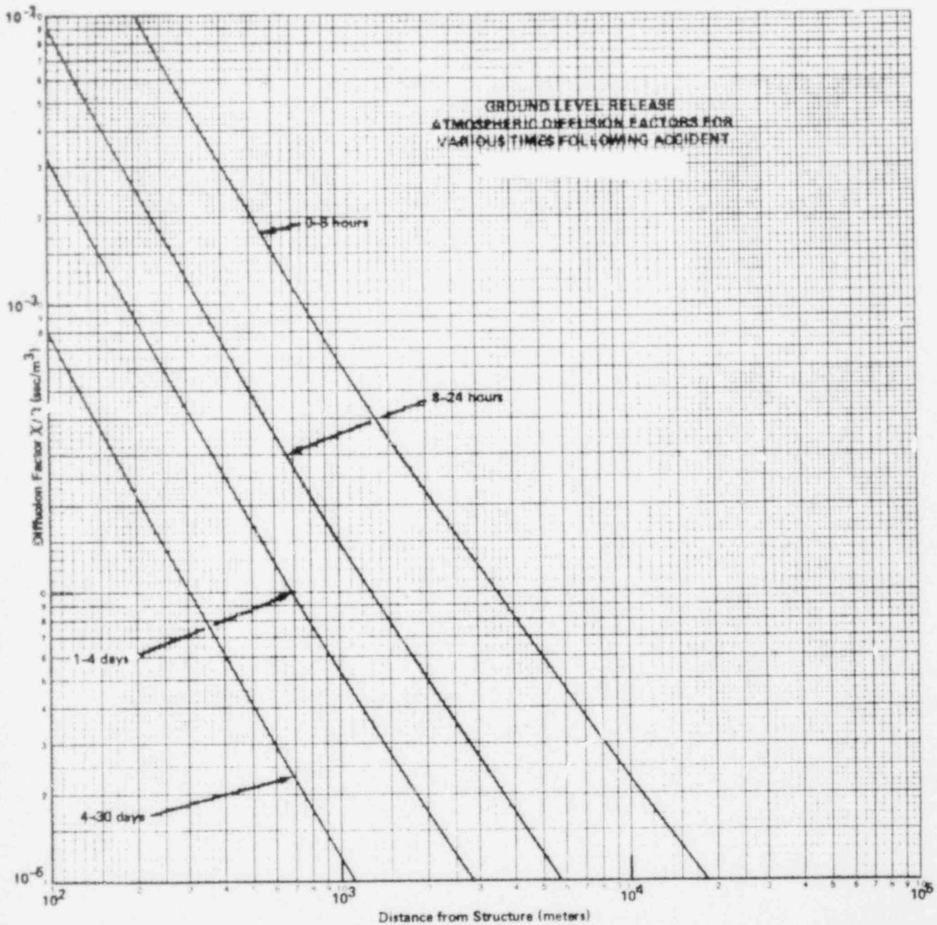
Figure 2-21. Design Basis Accident Diffusion Coefficients With NRC Standard Methodology, Reference 20.
