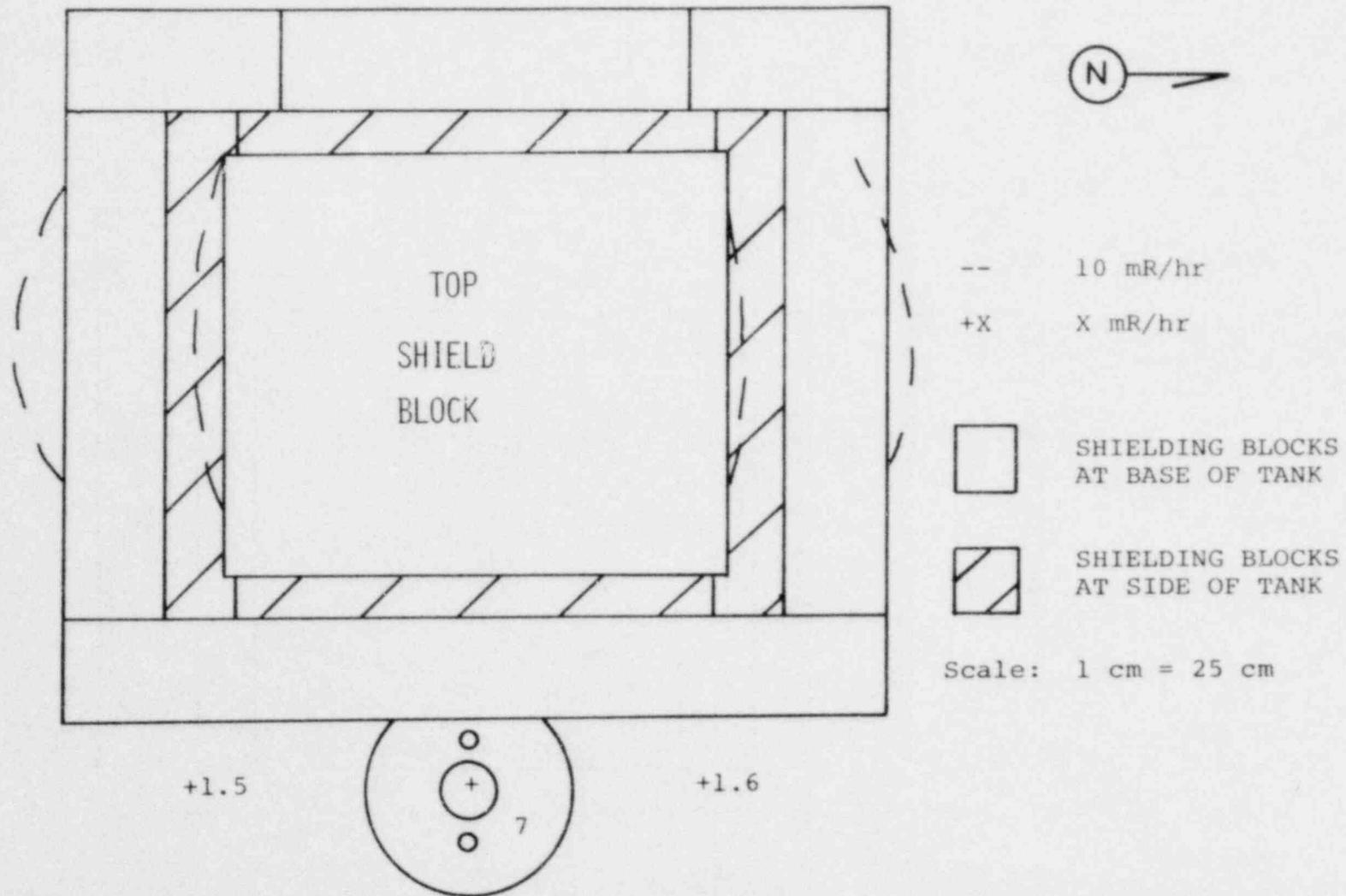
Figure 12-7. Gamma Exposure Rates Around the UFTR Shield Tank for 100 KWth. Operation With Readings Made At the Top of the Top Shield Block (101 cm Above the Reactor Surface).
