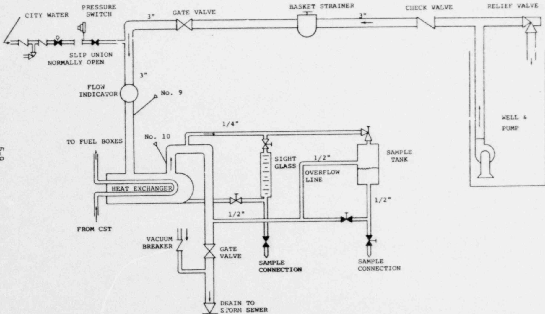
Figure 5-5. Schematic of UFTR Secondary Water Cooling System.
