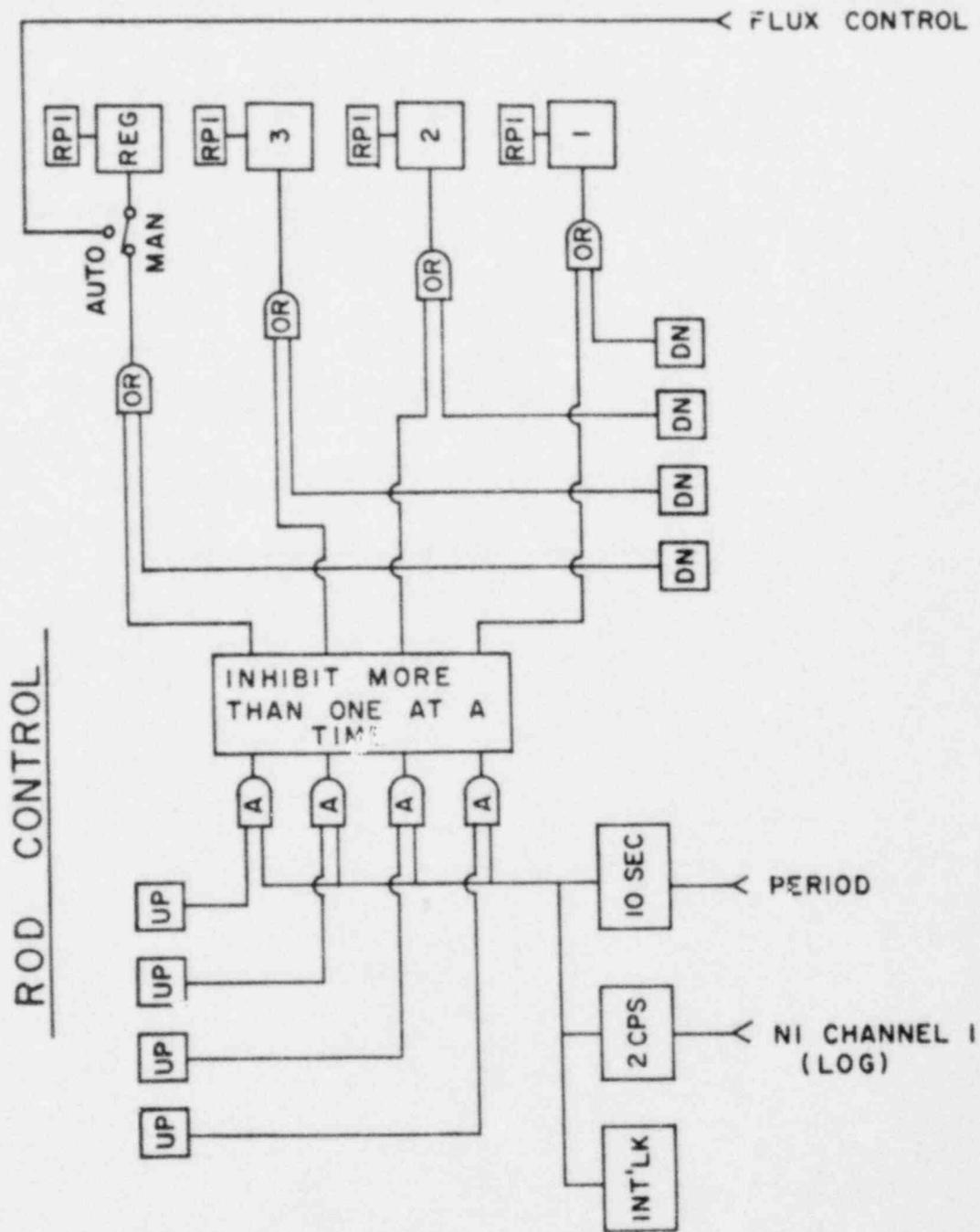
Figure 1-5. ROD CONTROL: UFTR Control Blade (Rod) Withdrawal Inhibit System.
