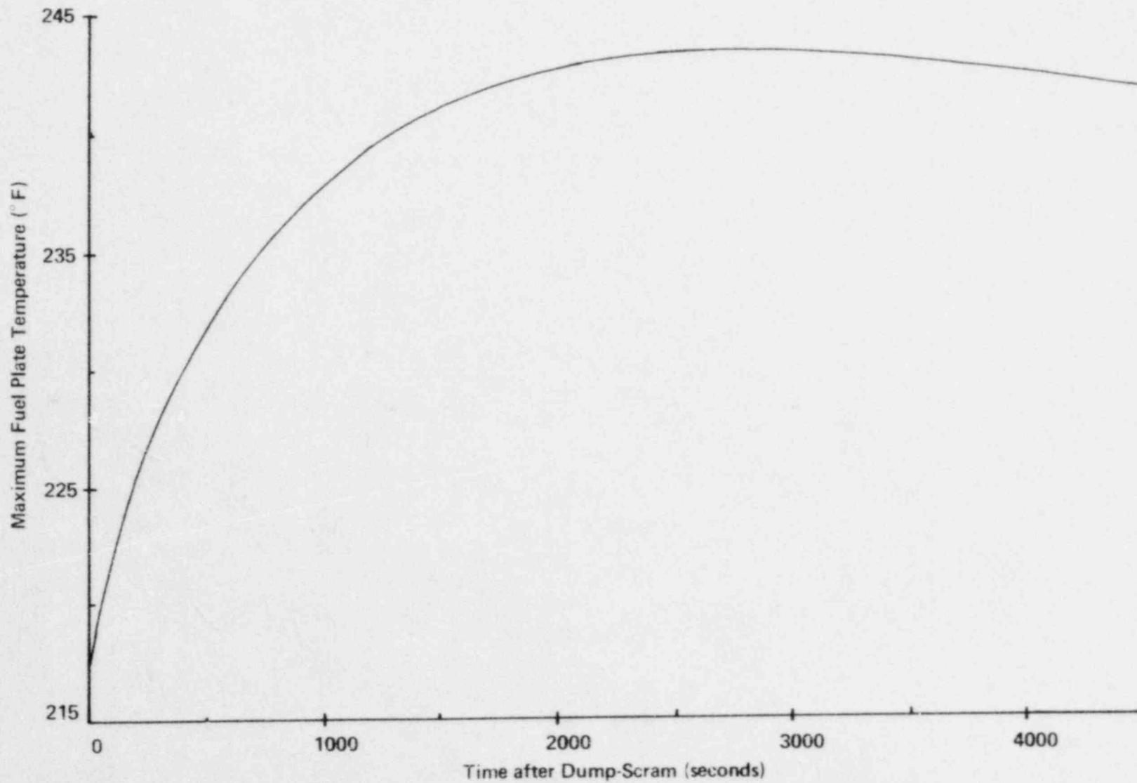
Figure 15-1. Calculated Fuel Plate Temperature Rise due to Decay Heating for Dump-Scram following UFTR Operation at 625 KWth.
