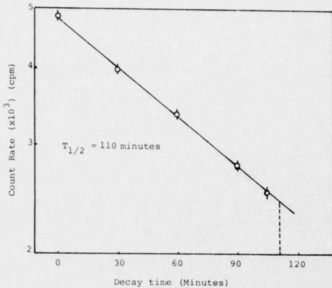
Figure 11-1. Data for Half-Life Determination of UFTR Stack Sample. (31)
