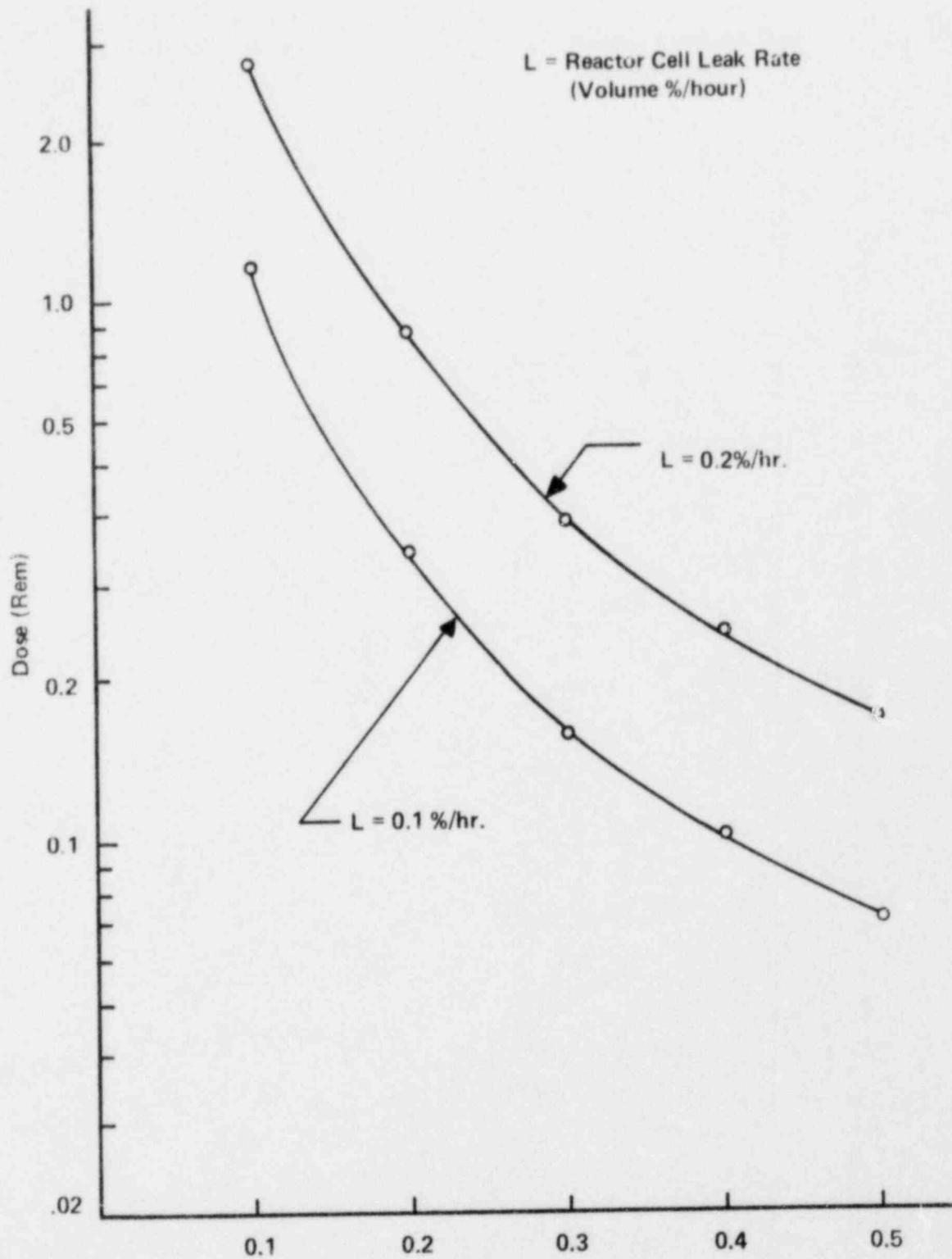
Figure 15.3. Two-Hour Thyroid Dose for UFTR Operation at 200 KW th Using Local Meteorology.
