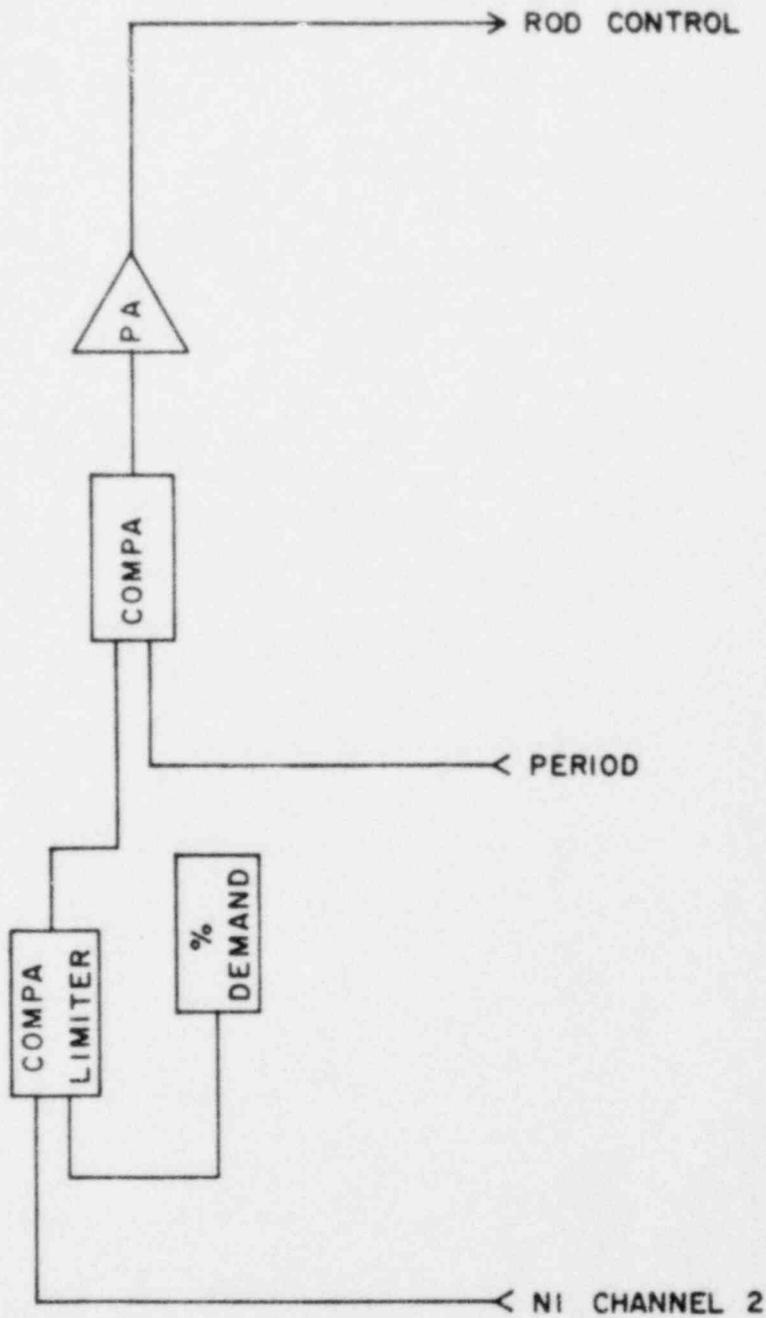
Figure 1-6. FLUX CONTROL: Schematic for UFR Neutron Flux Control System.
