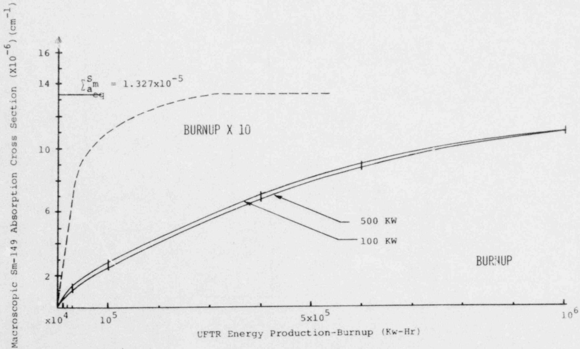
Figure 4-20. Samarium-149 Buildup for Operation at 100 and at 500 KWth.
