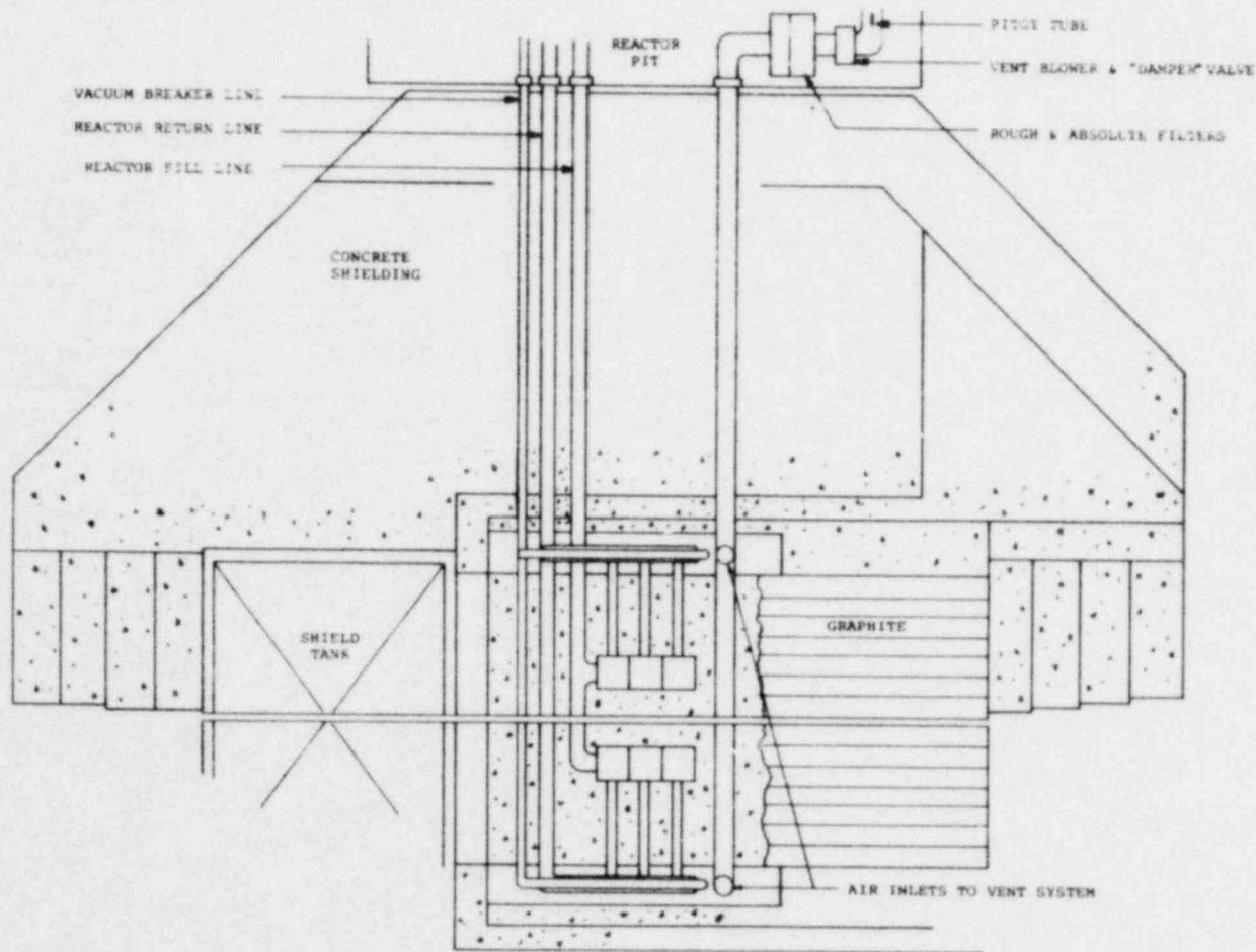
Figure 9-4. Vertical View Schematic Flow Diagram Showing Physical Arrangement of UFTR Core Vent System.
