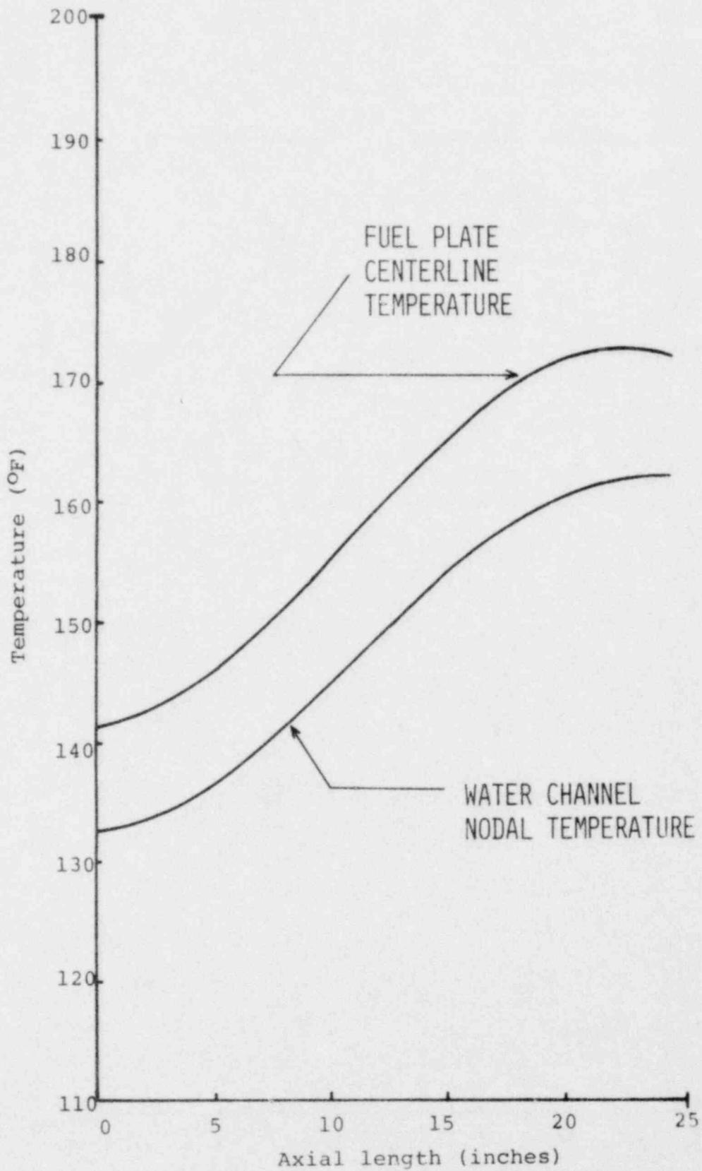
Figure 4-23. Temperature Distribution of the "Hottest" Fuel Plate and Water Channel at 100 KWth (Coolant Flow Rate = 31.2 gpm).
