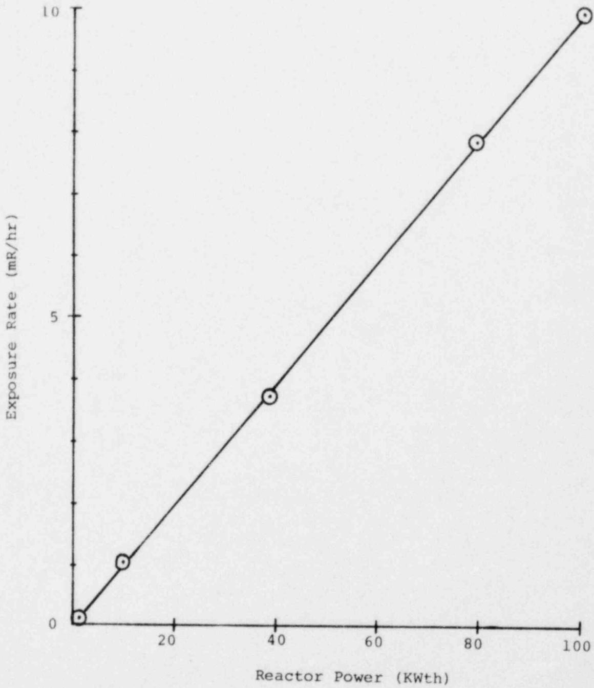
Figure 12-2. Exposure Rate Versus UFTR Operating Power (23)
