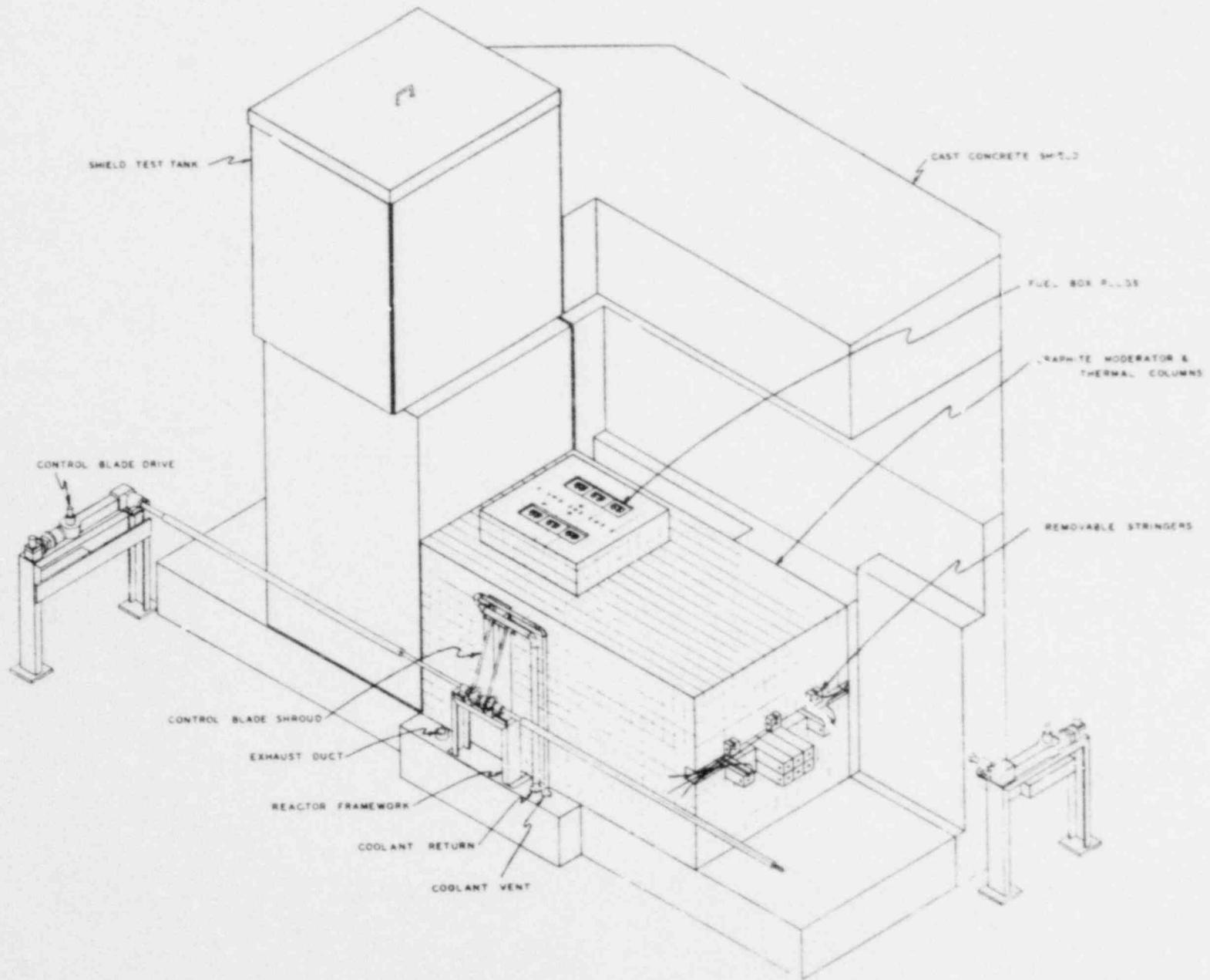
Figure 4-4. Isometric Sketch of the UFTR With Shielding Removed.
