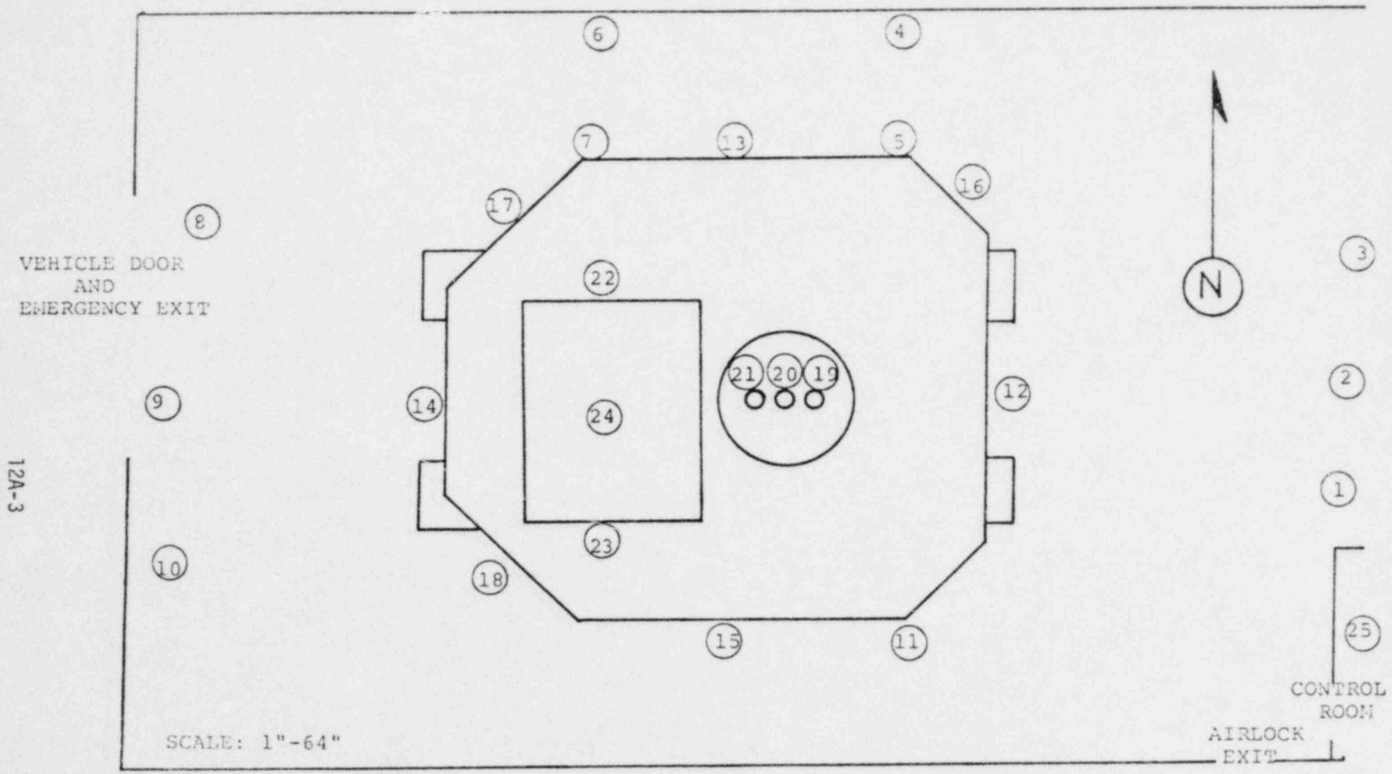
Figure 12A-1. Positions in UFTR Reactor Cell for Measurement of Radiation Levels at 100 KWth Steady-State Power Level with All Shielding Properly Emplaced. (Numbered Circle Indicate Points Where the Survey Was Taken to Correlate with Radiation Levels Recorded in Table 12-A-1.)
