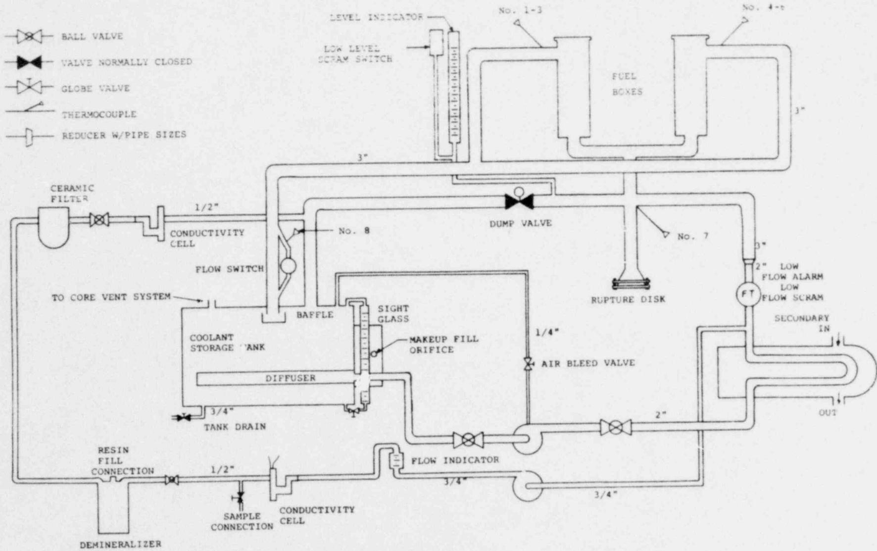
Figure 9-2. Schematic of UFTR Primary Coolant Loop and Purification Systems.
