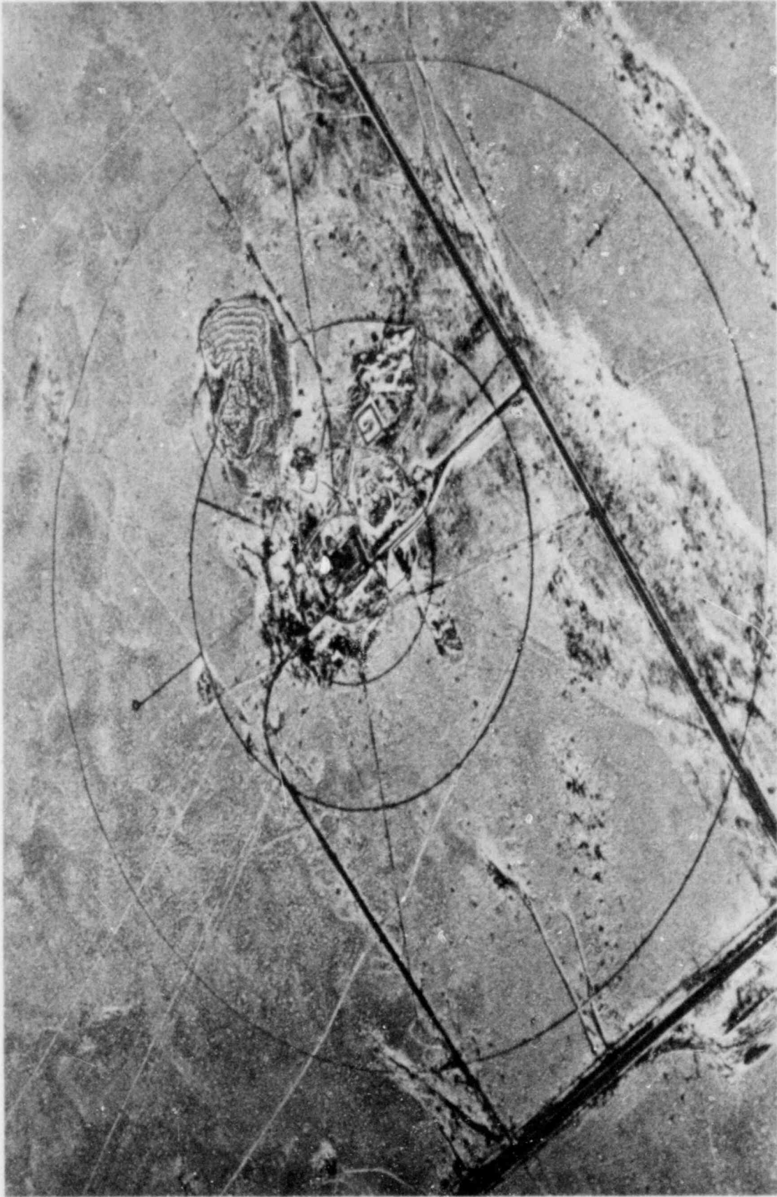
Figure 4. Aerial view of the innermost arcs of the EOCR grid. Photograph may be compared to the plot plan shown in figure 3. The outer circle corresponds to the 300 m arc of fig. 3. North is at the top of the picture.
