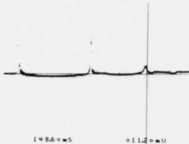
Fig. 2. Pressure data from FAST 44 (pressure measured underwater, 229 mm from test sample). Note that second pressure pulse, which occurred ~80 ms after sample burst, is larger in magnitude than burst pulse.
