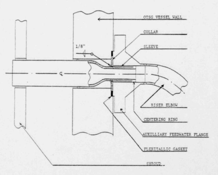
AUXILLIARY FEEDWATER NOZZLE/COLLAR/THERMAL SLEEVE CONFIGURATION
