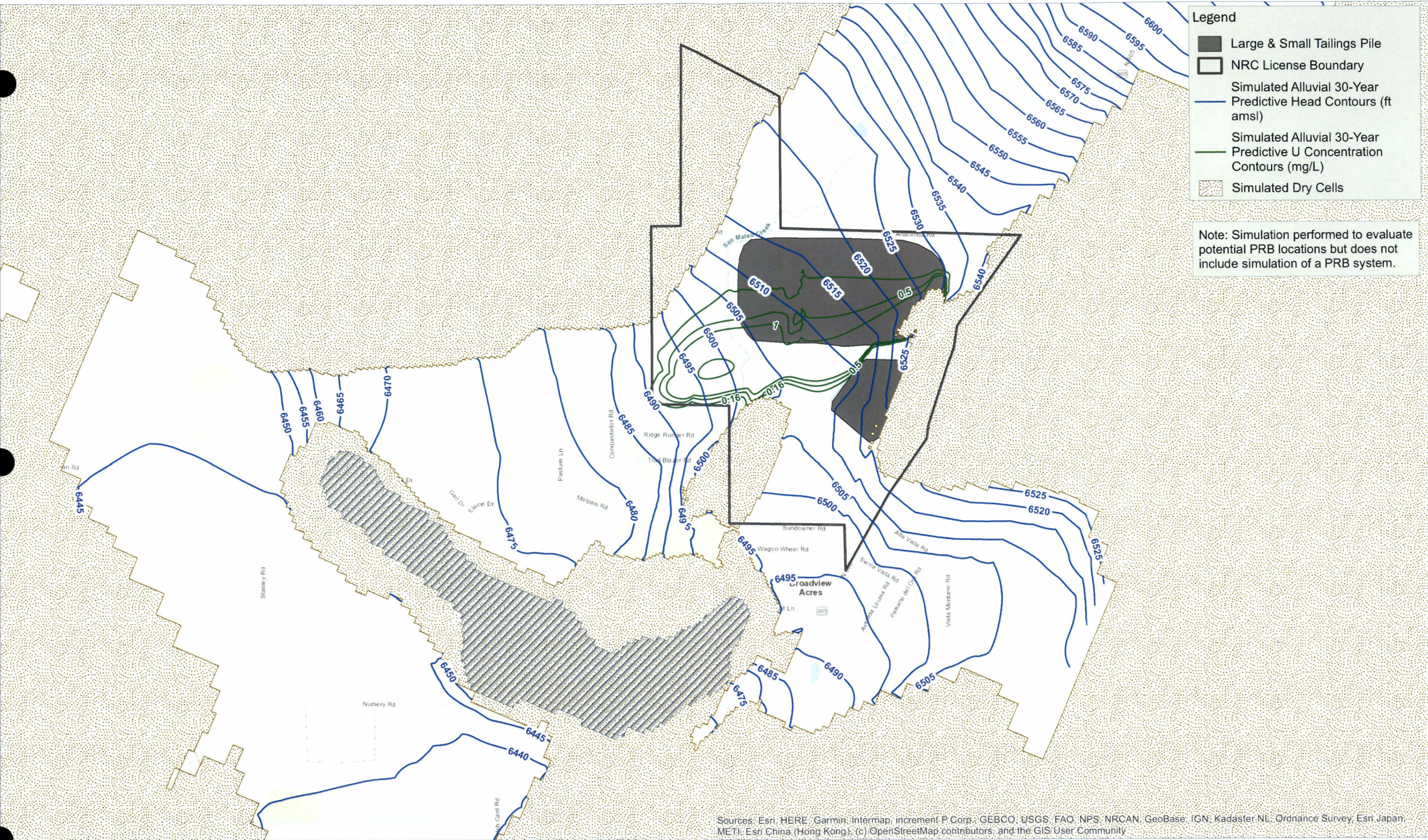
Figure 3-22 Alluvial Aquifer Simulated Predictive 30-Year Uranium Concentration Contours with 10 Years of Active Groundwater Collection and Injection
