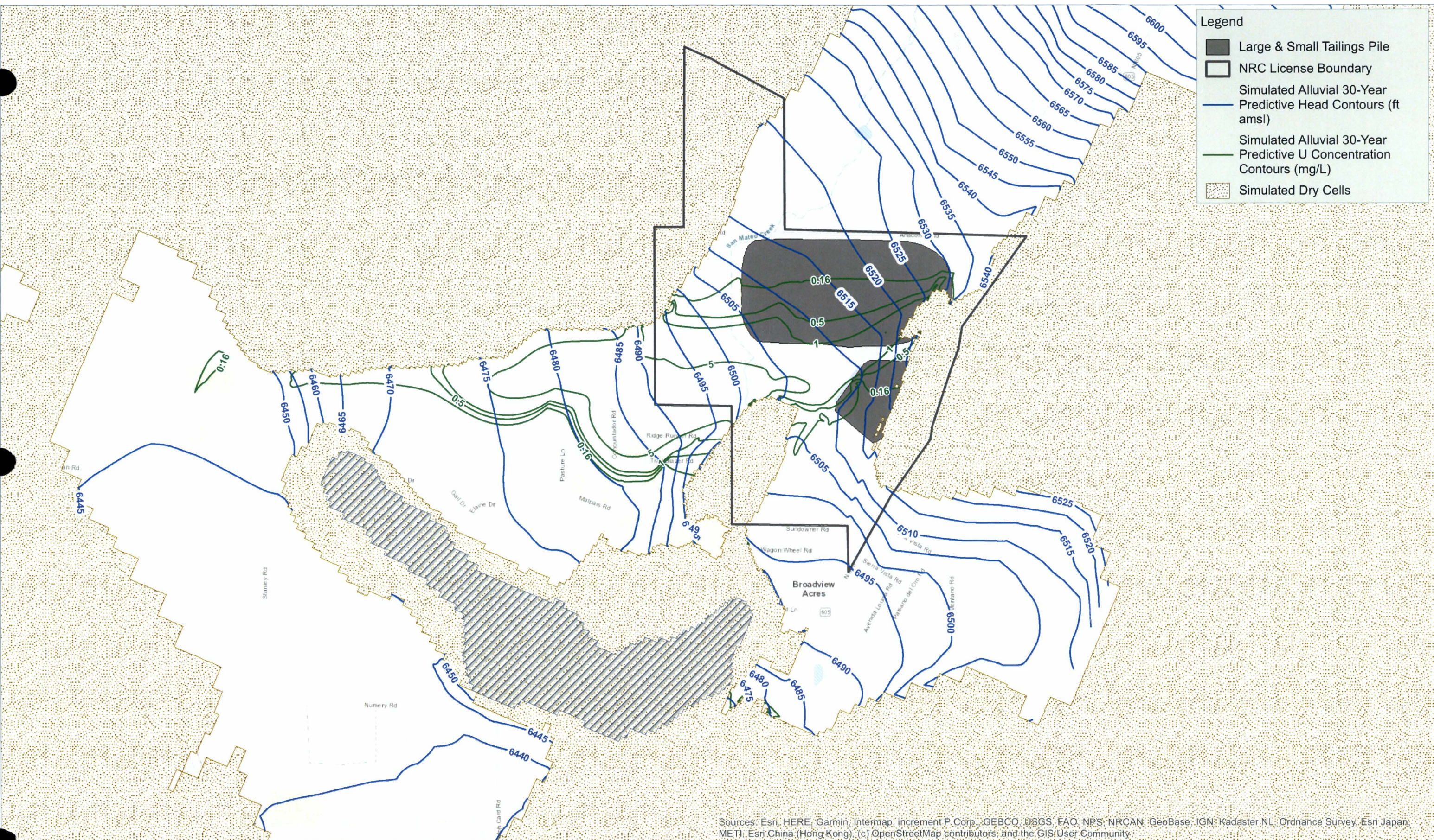
Figure 3-3 Alluvial Aquifer Simulated Predictive 30-Year Uranium Concentration Contours Natural Attenuation
