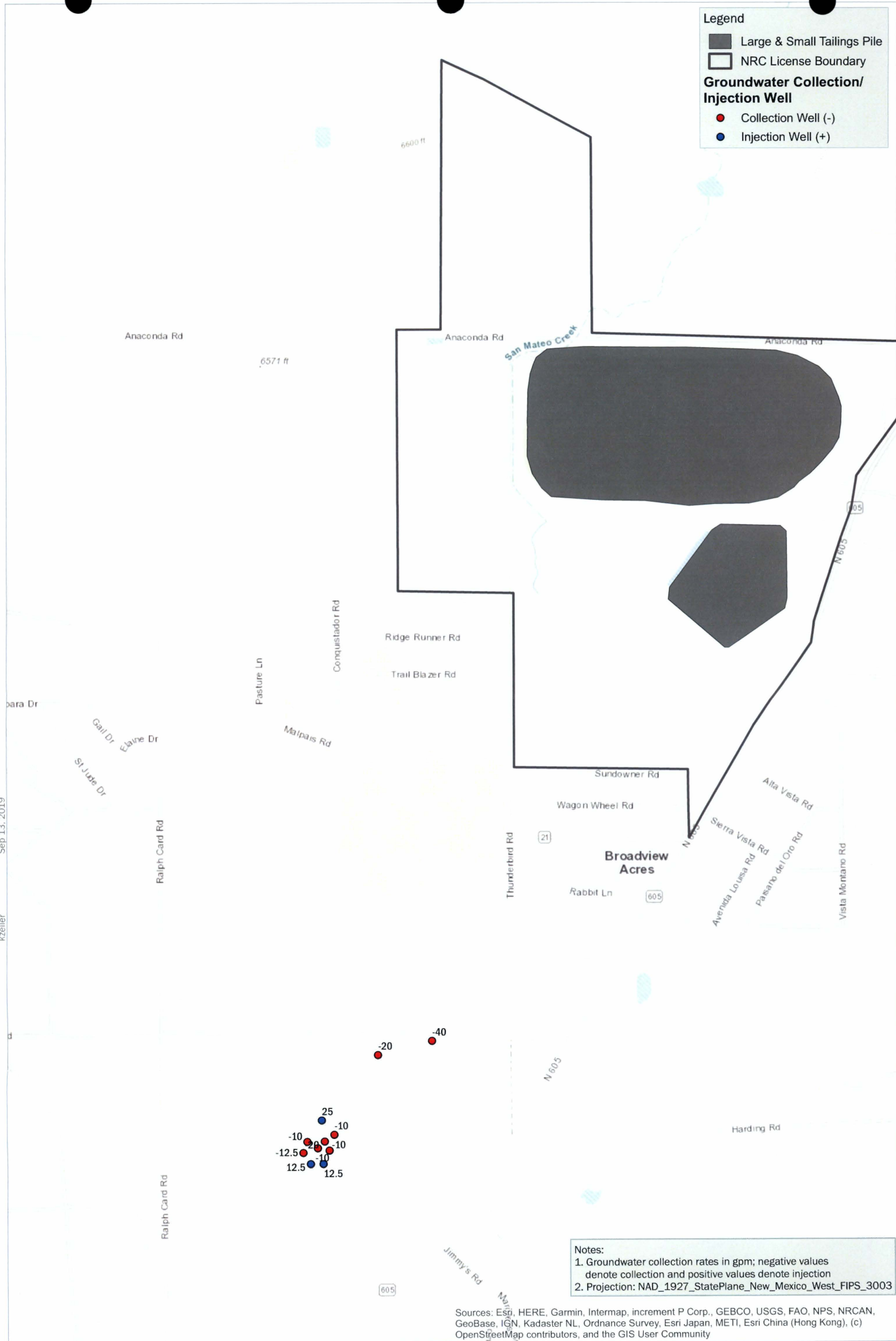
Figure 2-4 Lower Chinle Aquifer Simulated Predictive Year 1 to 2 Groundwater Collection and Injection Rates
