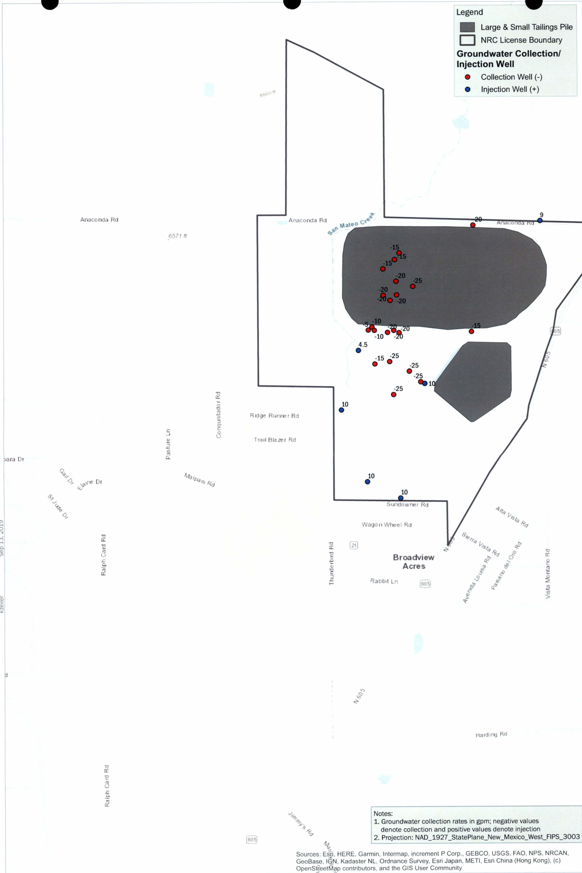
Figure 2-22 Upper Chinle Aquifer Simulated Predictive Year 11 to 12 Groundwater Collection and Injection Rates
