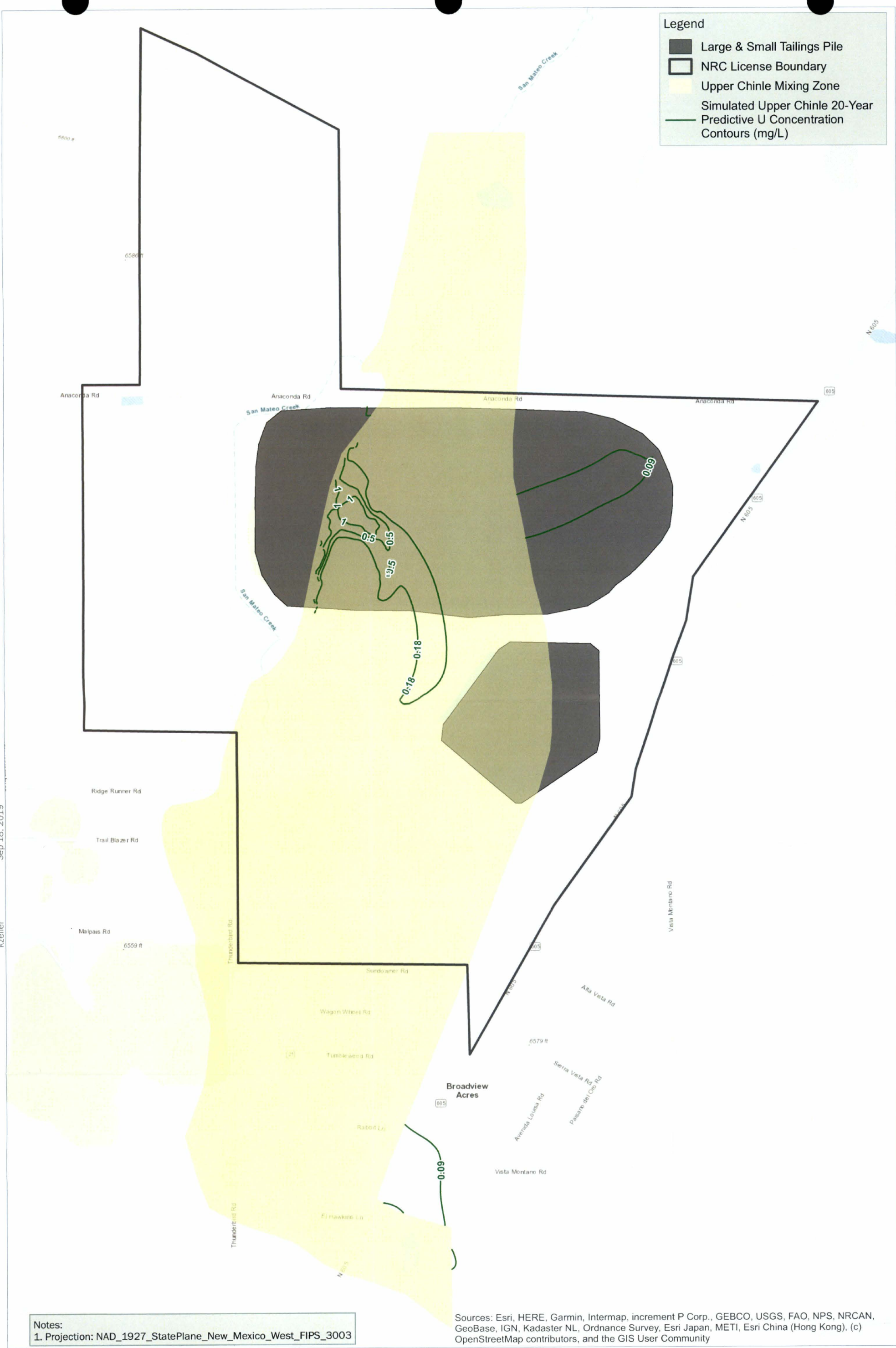
Figure 3-17 Upper Chinle Aquifer Simulated Predictive 20-Year Uranium Concentration Contours with 24 Years of Active Groundwater Collection and Injection
