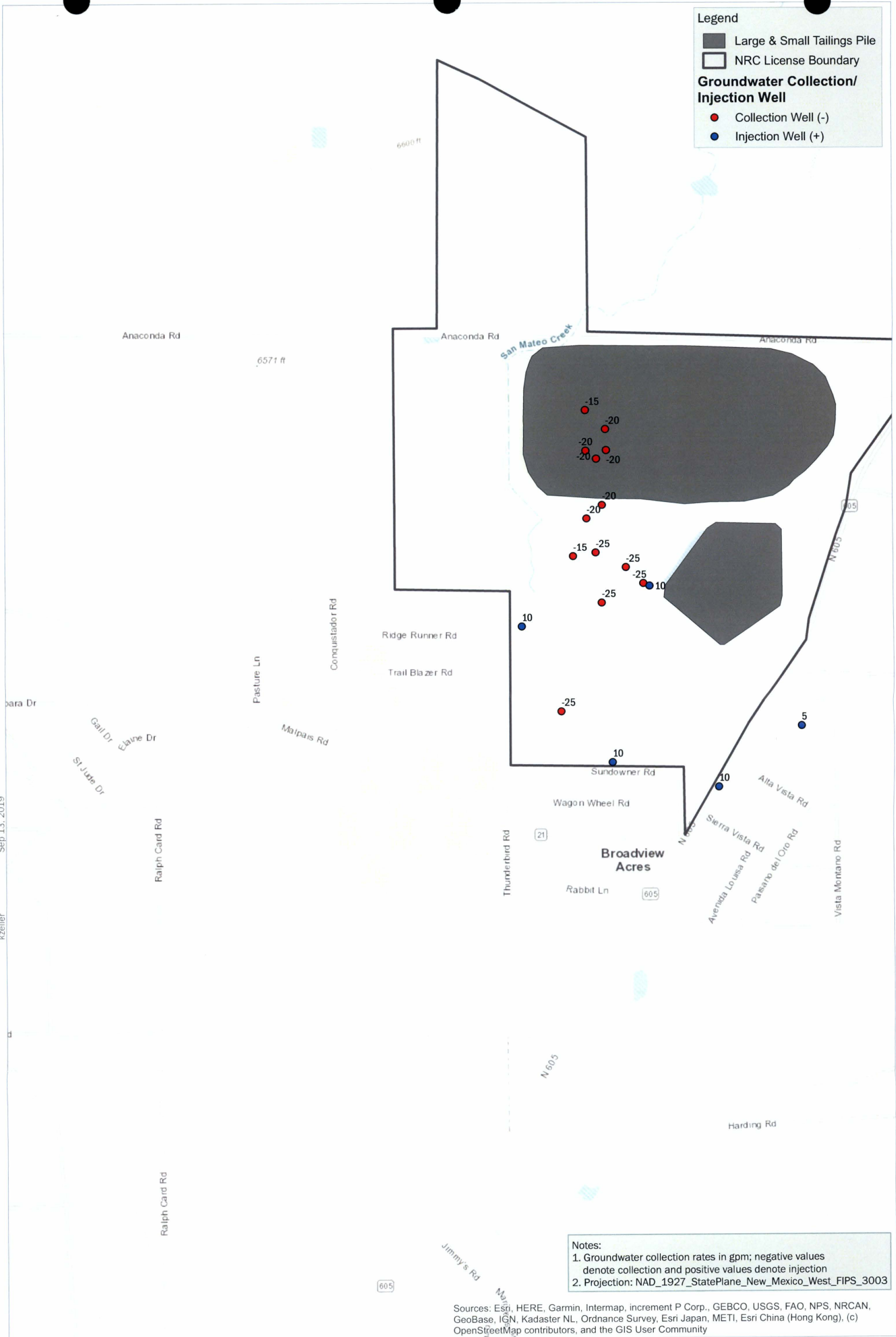
Figure 2-2 Upper Chinle Aquifer Simulated Predictive Year 1 to 2 Groundwater Collection and Injection Rates
