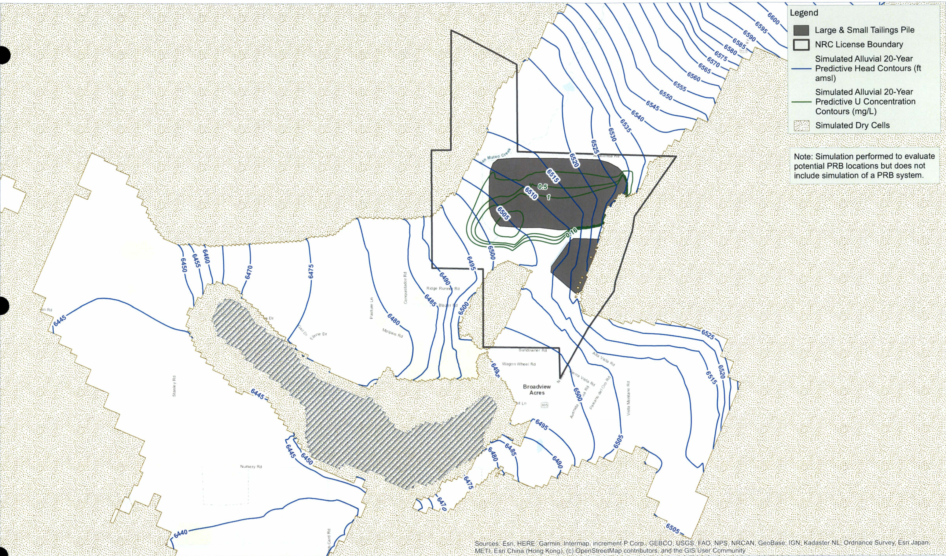
Figure 3-21 Alluvial Aquifer Simulated Predictive 20-Year Uranium Concentration Contours with 10 Years of Active Groundwater Collection and Injection
