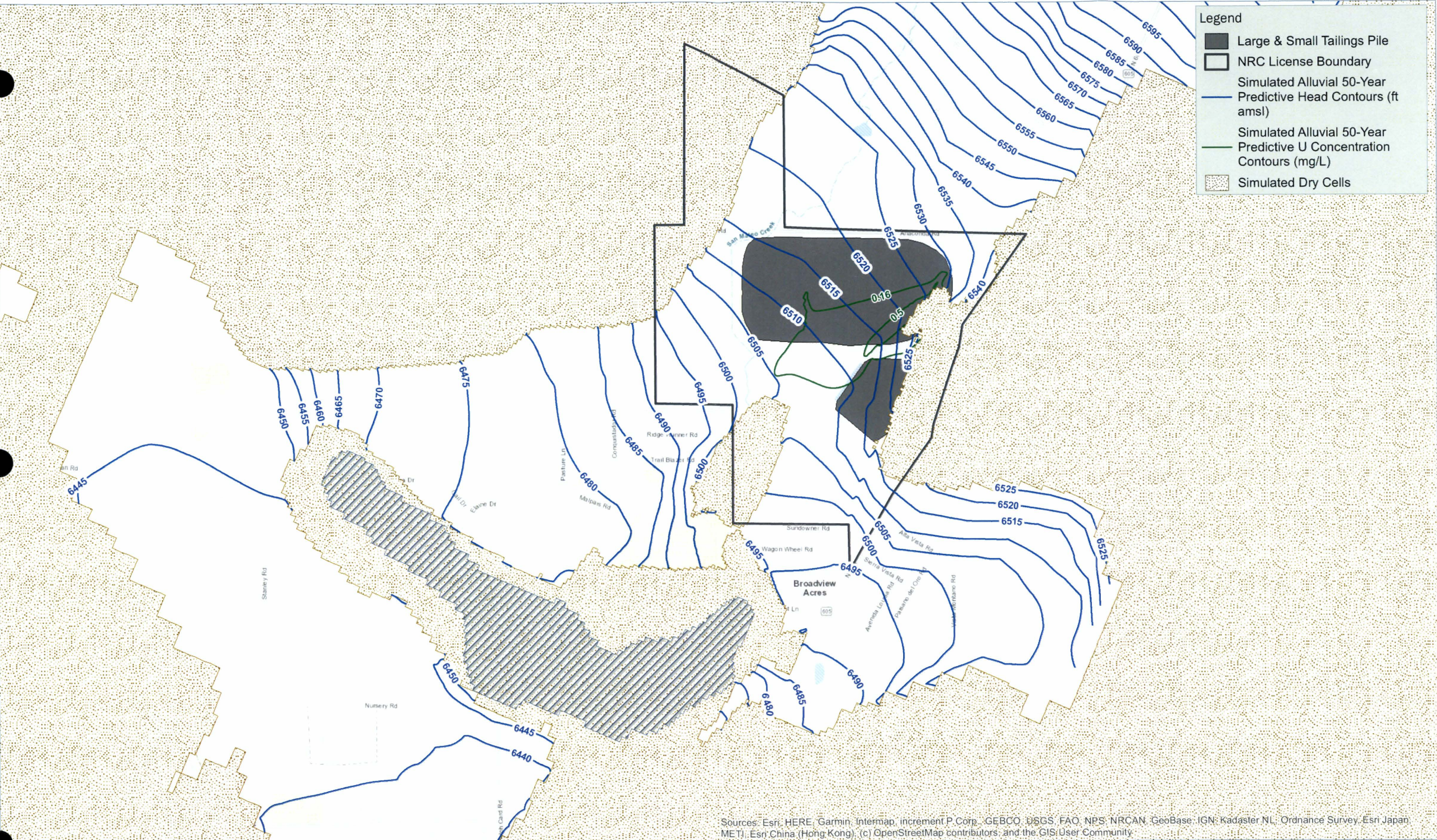
Figure 3-15 Alluvial Aquifer Simulated Predictive 50-Year Uranium Concentration Contours with 24 Years of Active Groundwater Collection and Injection
