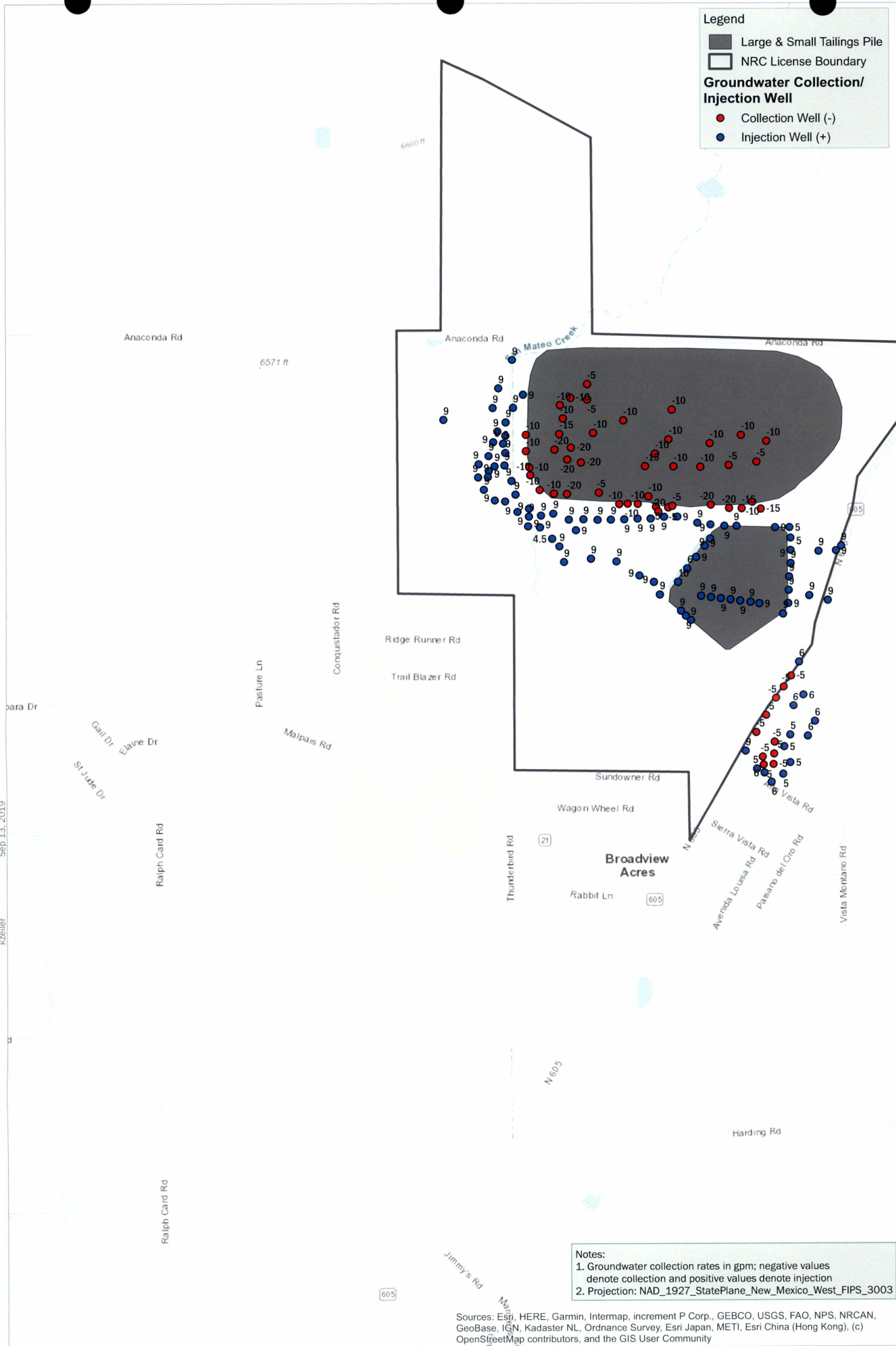
Figure 2-25 Alluvial Aquifer Simulated Predictive Year 13 to 16 Groundwater Collection and Injection Rates
