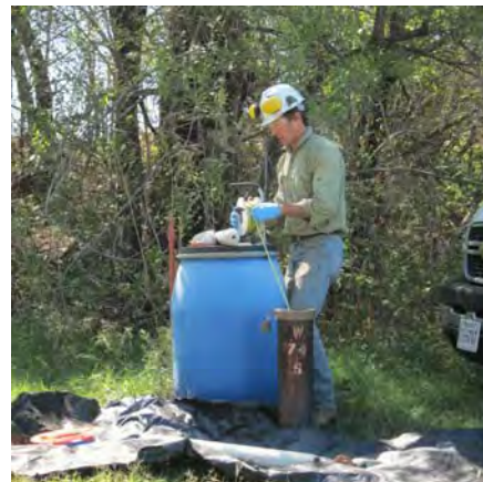
Figure 12 - Measuring height of water column in MW
