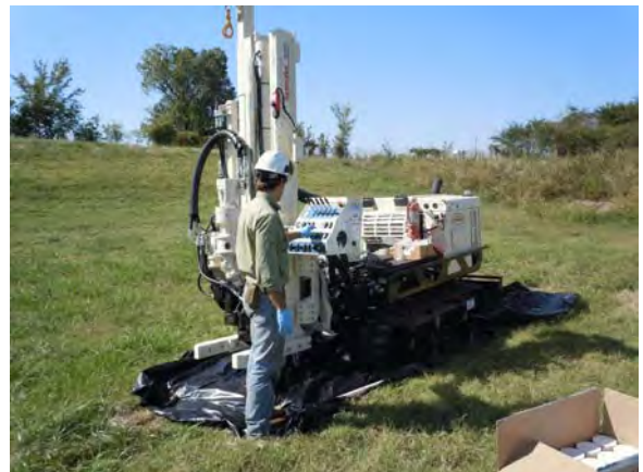
Figure 4 - Collecting subsurface sample using Geoprobe
