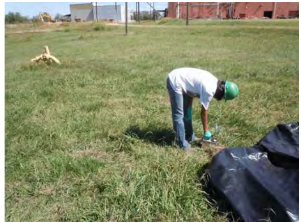
Figure 2 - Measuring ambient gamma exposure rate at subsurface soil sample collection location
