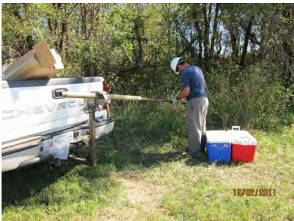
Figure 5 - Removing soil sample from sample sleeve
