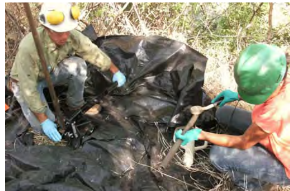
Figure 10 - One-meter deep sample collection using hammer drill
