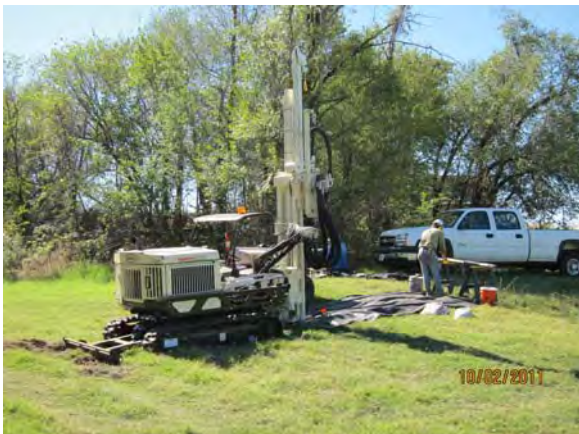
Figure 3 - Collecting subsurface sample using Geoprobe
