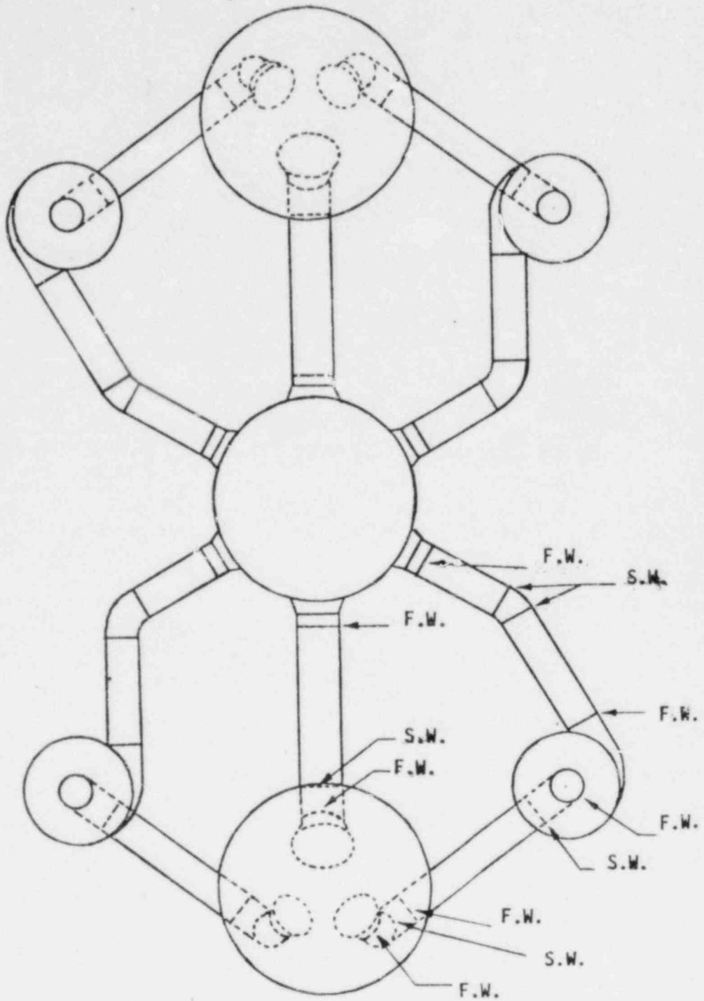
FIGURE 2-12 Weld location for Fort Calhoun Unit 1
