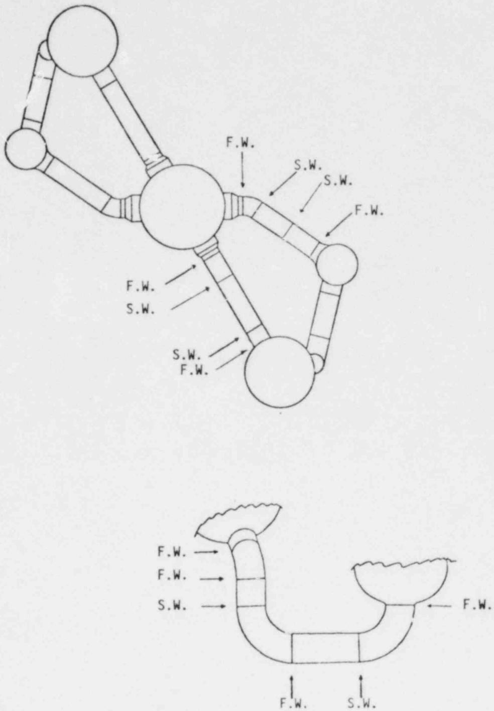
FIGURE 2-9 Weld location for Point Beach Units 1 and 2
