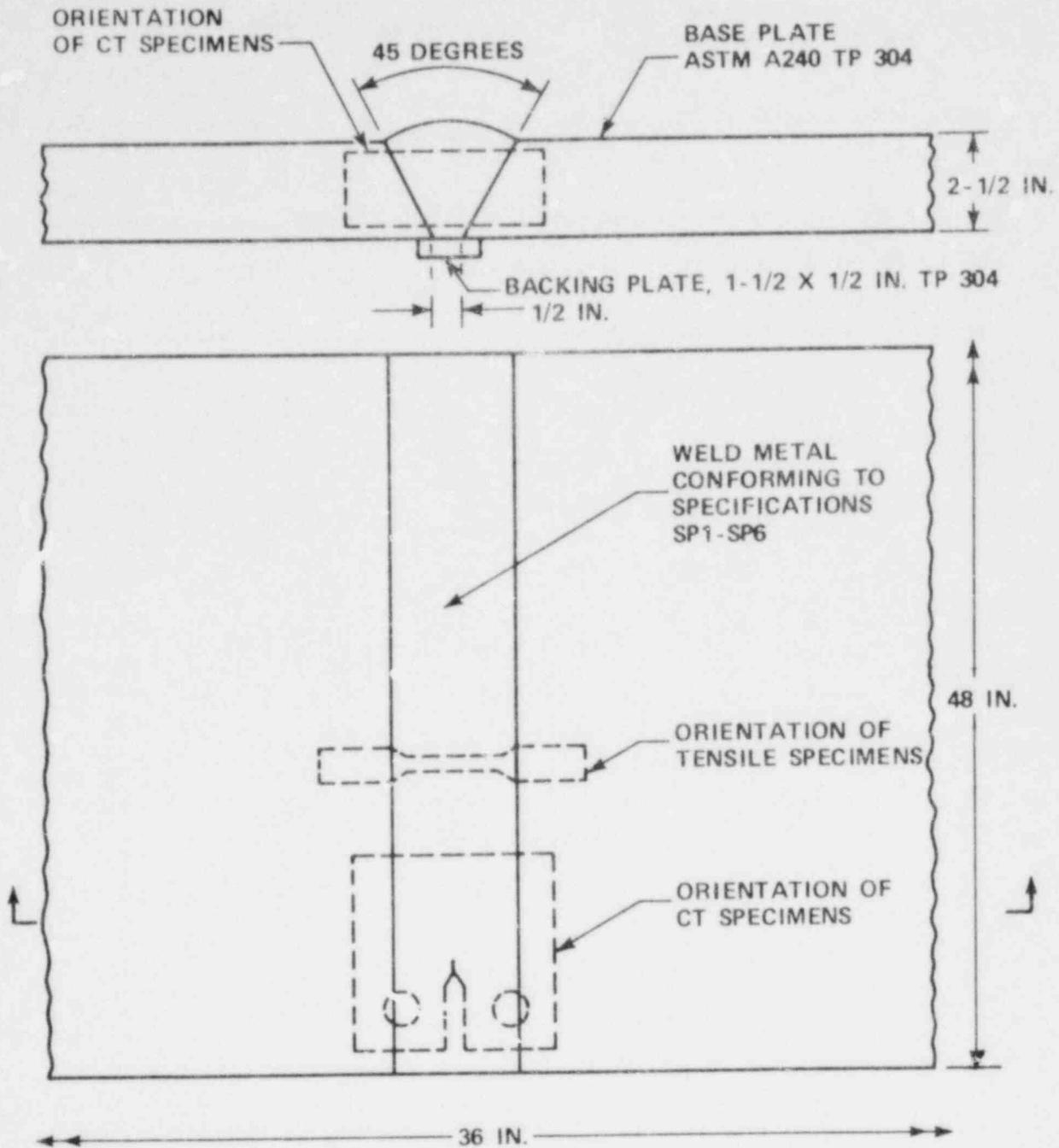
Figure 4-1 Weldment Configuration Showing the Orientation of Specimens
