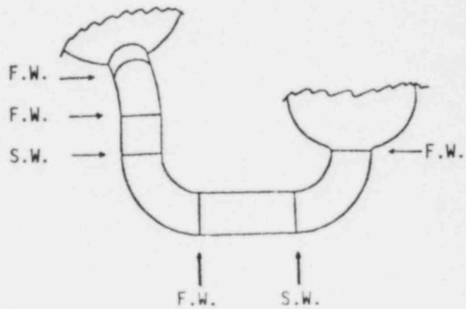
FIGURE 2-3 Weld location for Zion Units 1 and 2
