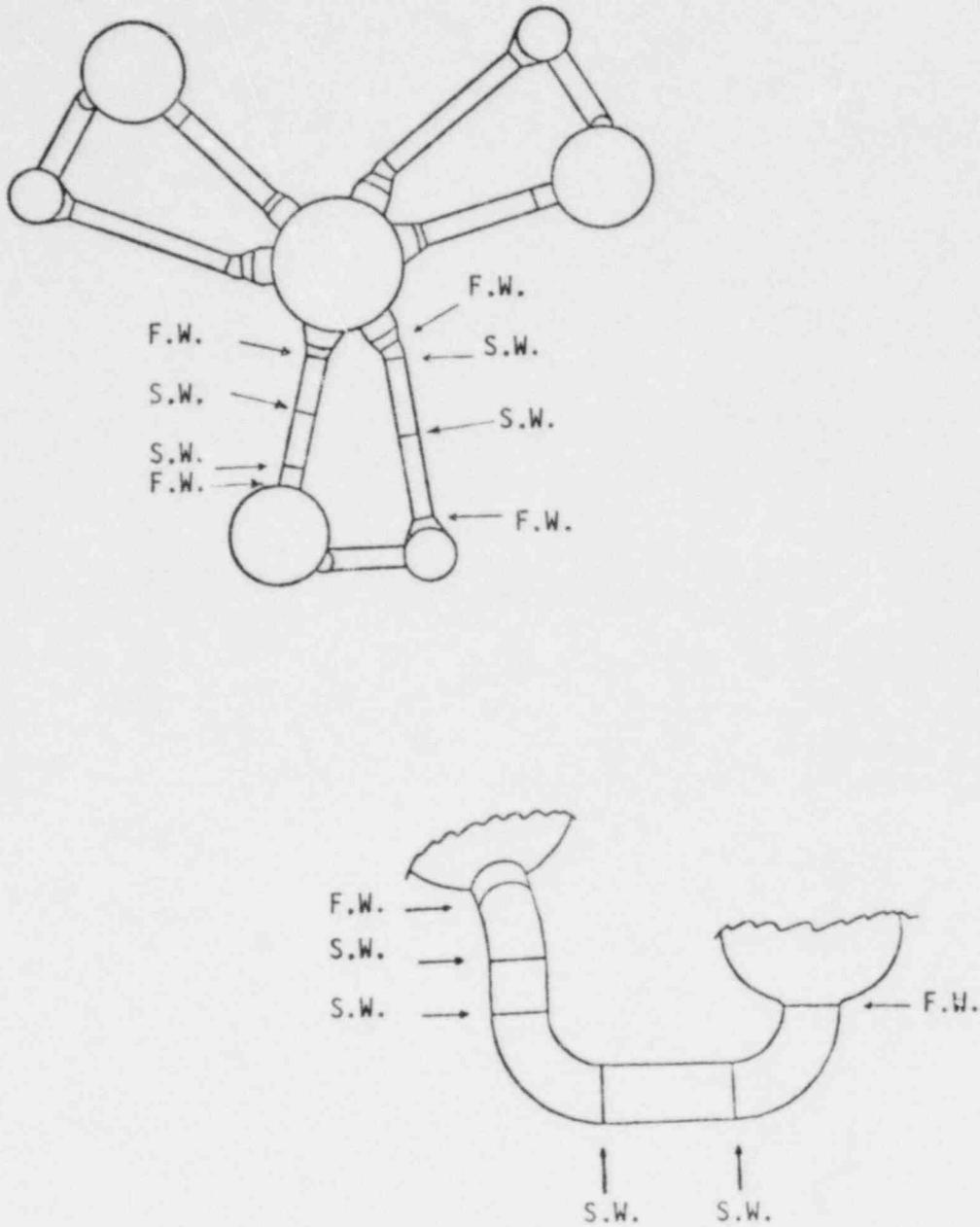
FIGURE 2-7 Weld location for San Onofre Unit
