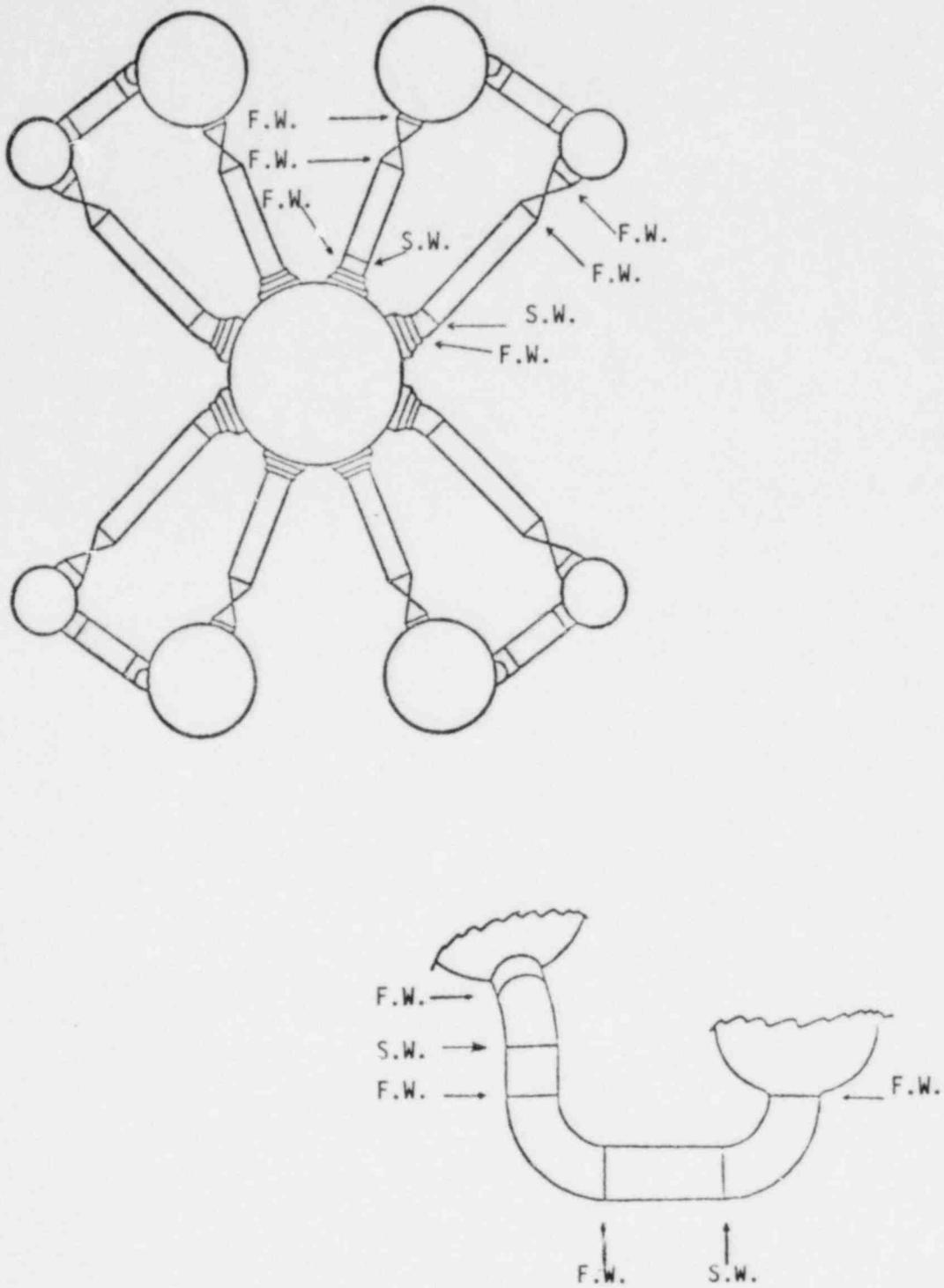
FIGURE 2-11 Weld location for Yankee Rowe Unit
