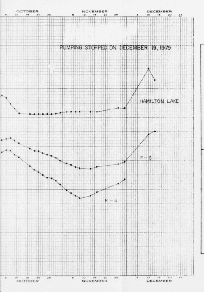
AND OBSERVATION WELLS F-4 AND F-6 DURING PUMP TESTS FIGURE 2.4-15
