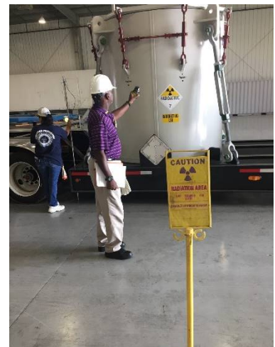
An NRC inspector verifies radiation levels from a radioactive material shipment being prepared for transport.
