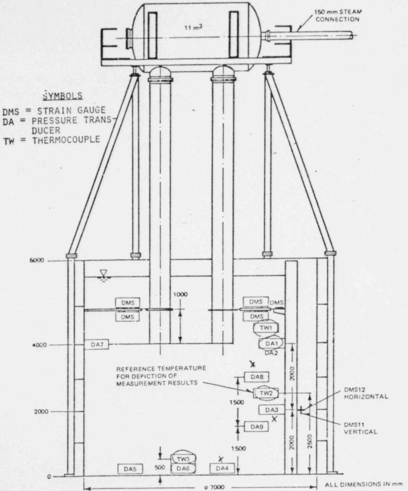
Figure 5-1. Test Set-up and Instrumentation, 600 mm Vents - Side View
