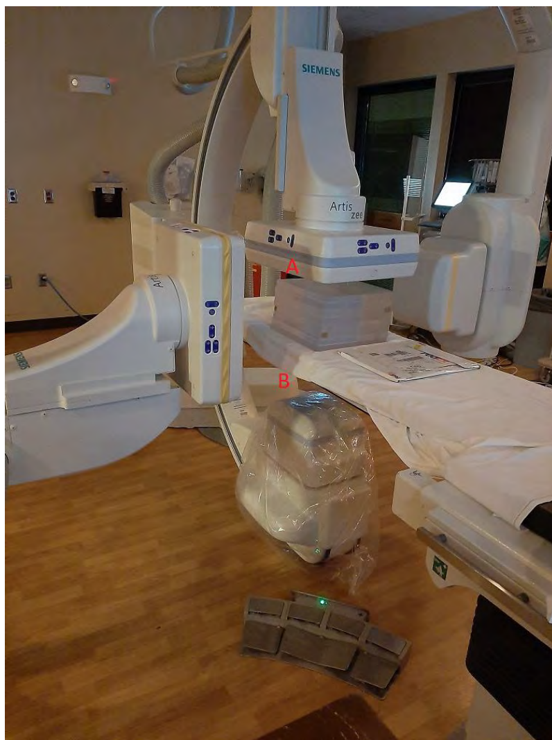
Figure 1 – Scatter measurement set-up in the interventional suite
