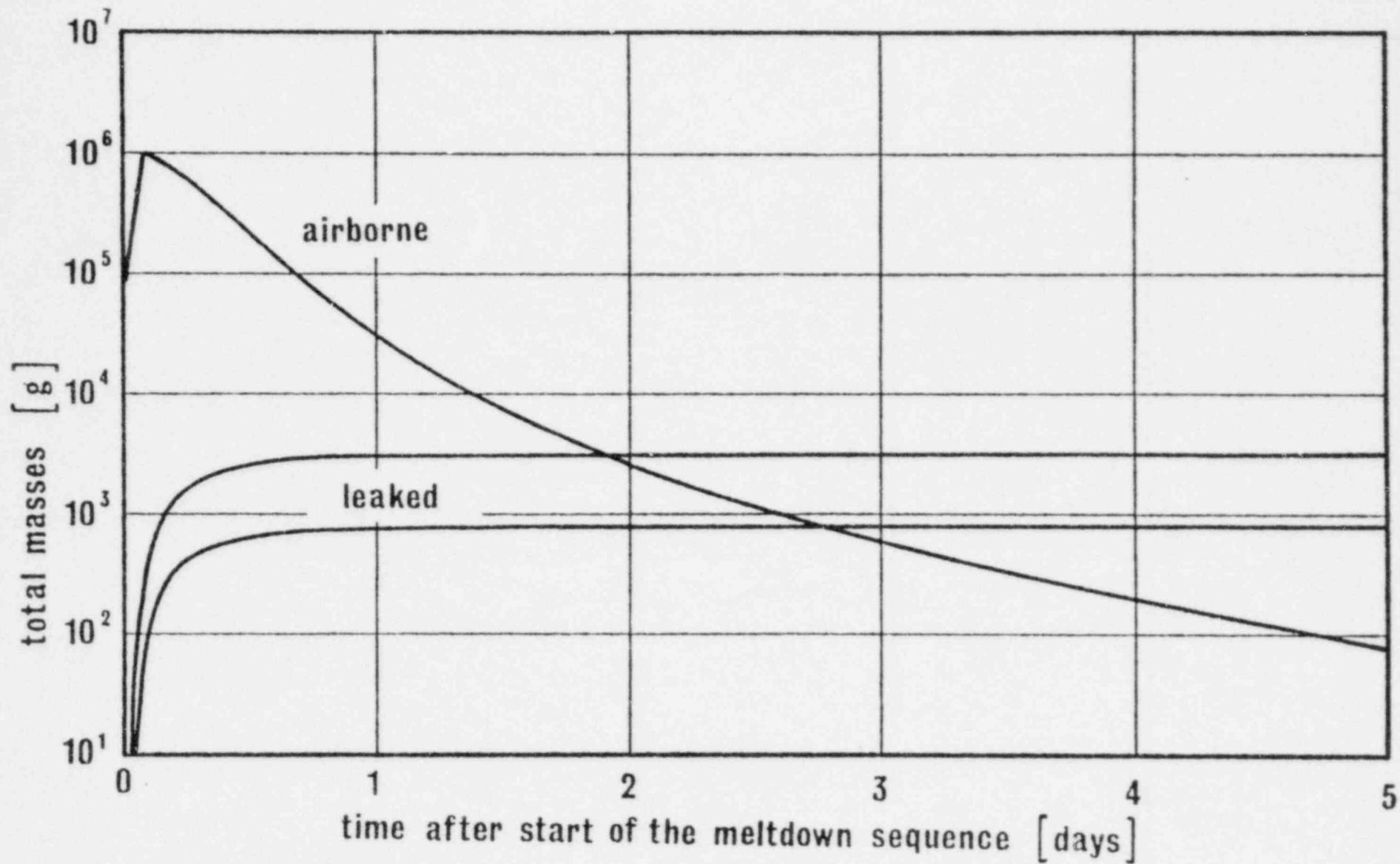
Fig. 4: Airborne mass in the containment and leaked mass.
