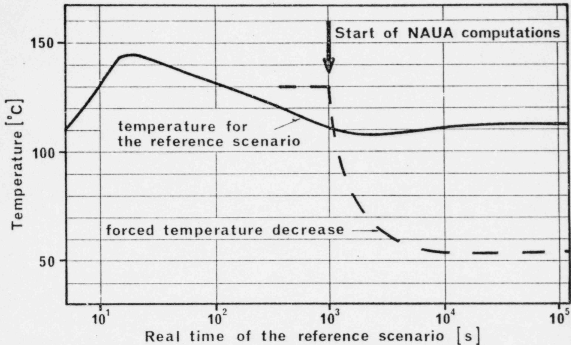
Fig. 2: Containment temperature-function for the NAUA calculations
