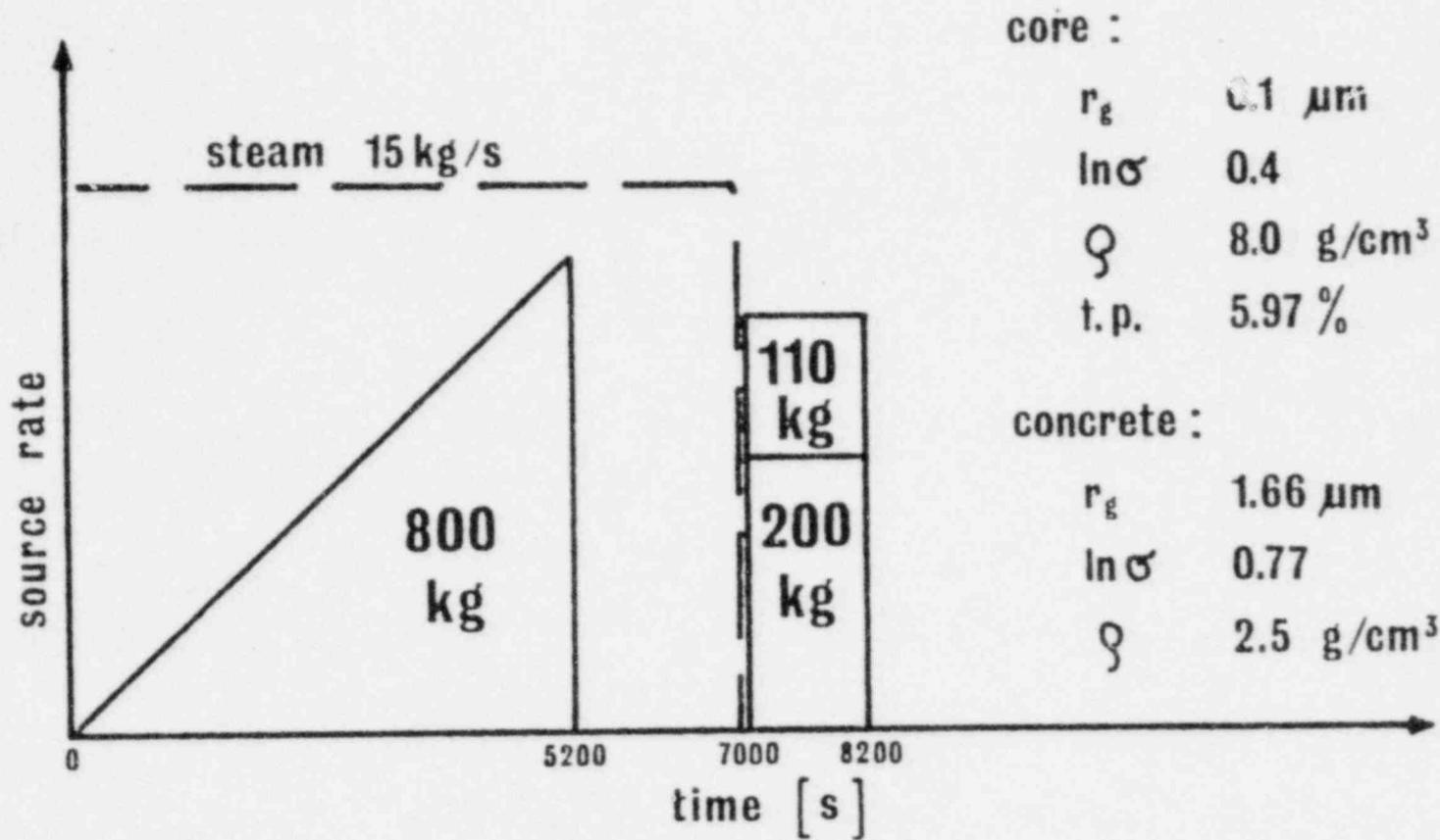
Fig. 3: Aerosol and steam sources for the NAUA calculations
