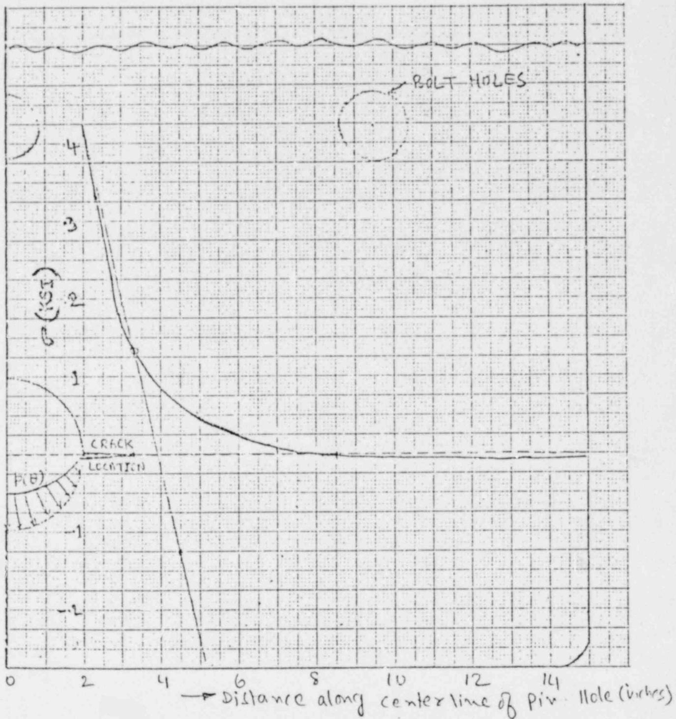
Figure 4 Normal stress distribution across Lug width
