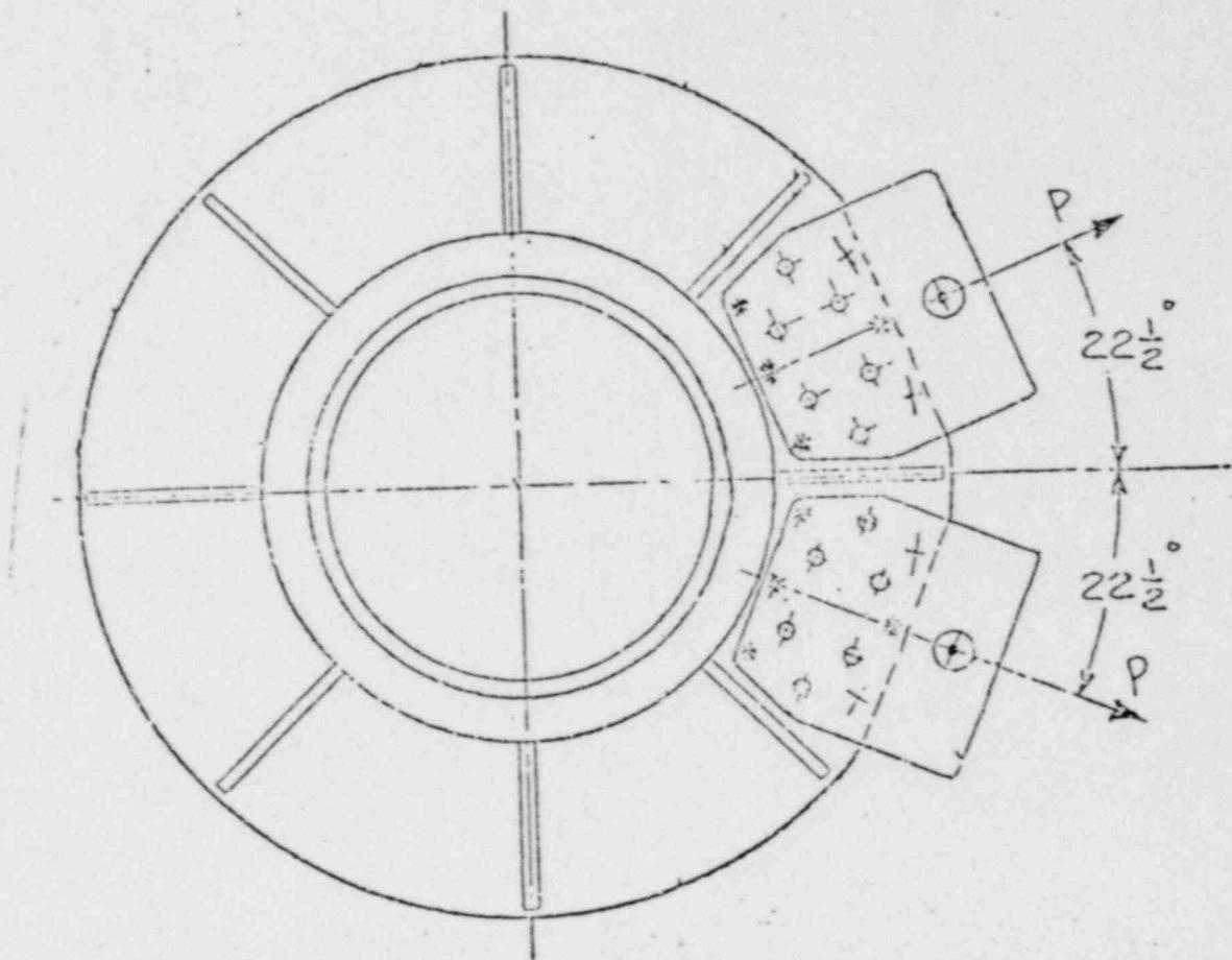
Figure 1. Configuration of Seismic Snubber Lugs of Arkansas Nuclear power plant Reactor. Coolant Pump.
