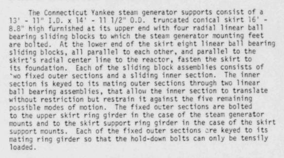
During assembly, all of the hold-down bolts were equally preloaded to a level in excess of the maximum bolt load that could be induced in the event of a design level earthquake or a primary loop piping rupture. The preloading was accomplished by heating the bolts and nuts in an electric oven to 725°F, inserting the bolt in place and, when thermocouple measurement showed that the bolt had cooled to 675/670°F, the nut was drawn up hand tight.
