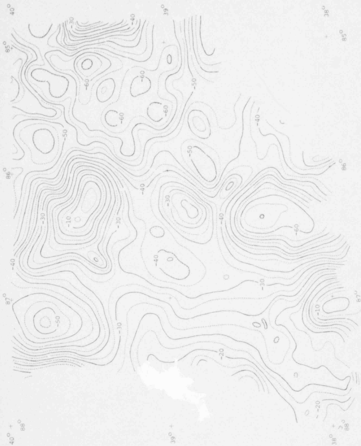
Figure 12. Bouguer gravity anomaly map of southern Indiana-1980. Contour interval is 2.5 mgals. Reduction based on I.G.S.N. 1971, G.R.S. 1967 and a density of 2.67 gm/cc.
