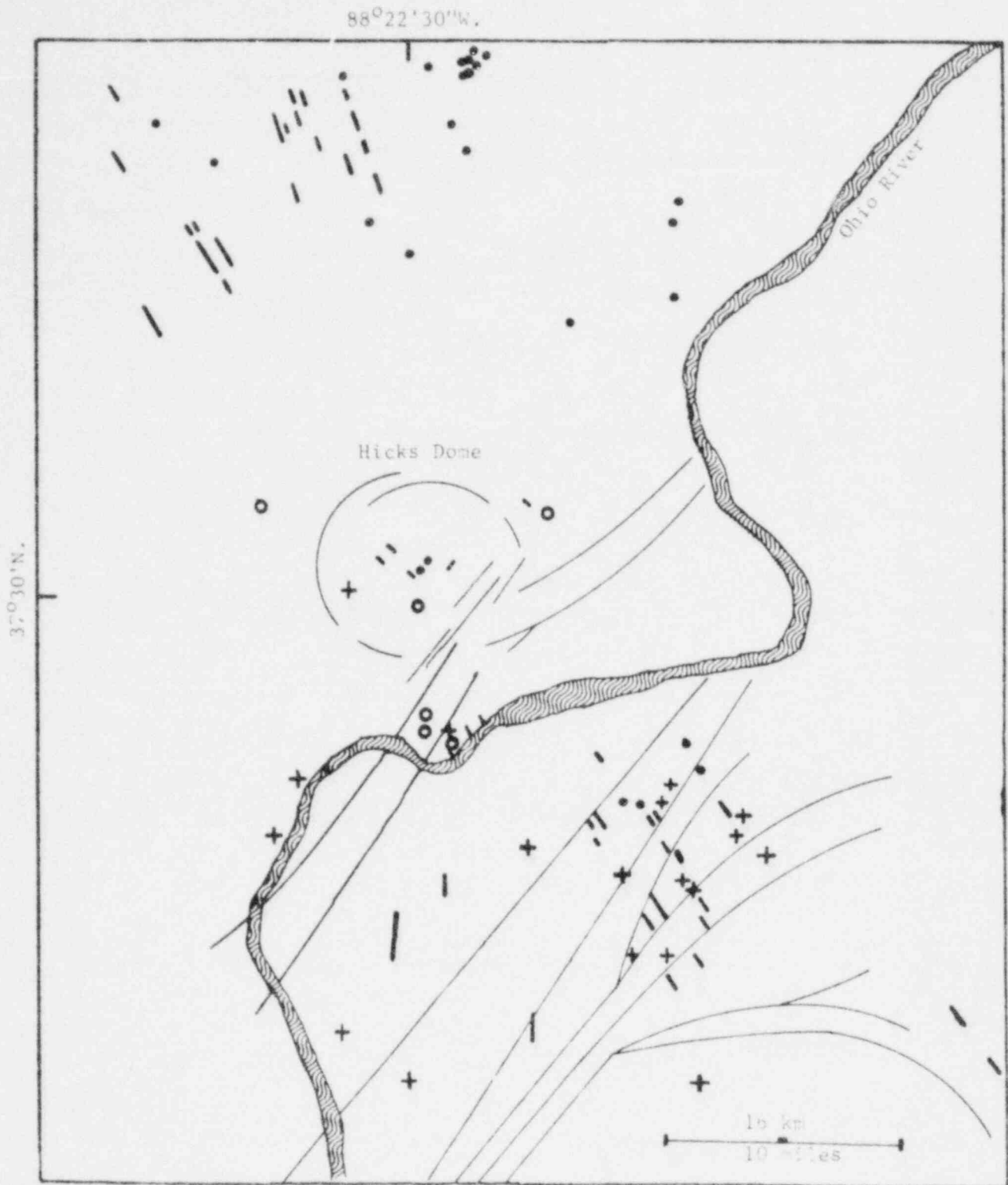
Figure 21. Distribution of mafic and ultramafic intrusions in southern Illinois and western Kentucky. Thin solid lines, high angle faults; thick solid lines, surface dikes showing trend; plus symbol, surface dike with unknown trend; open circle, surface igneous diatreme; closed circle, subsurface dikes in drill holes.
