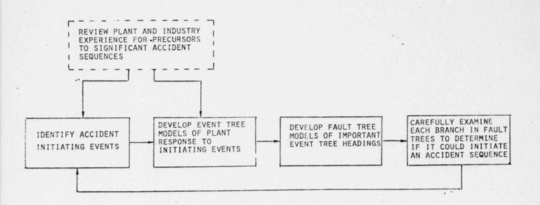
FLOW DIAGRAM OF ITERATIVE PROCESS TO ASSURE COMPLETENESS IN PRA ACCIDENT SEQUENCE DEFINITION
