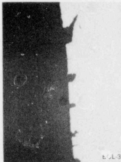
(e) Cladding inner surface near crack
