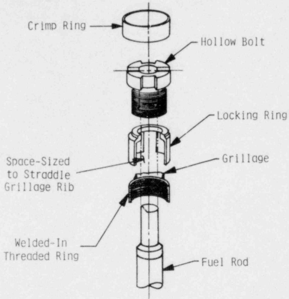
Figure 4-4. Removable Fuel Rod UEF Components
