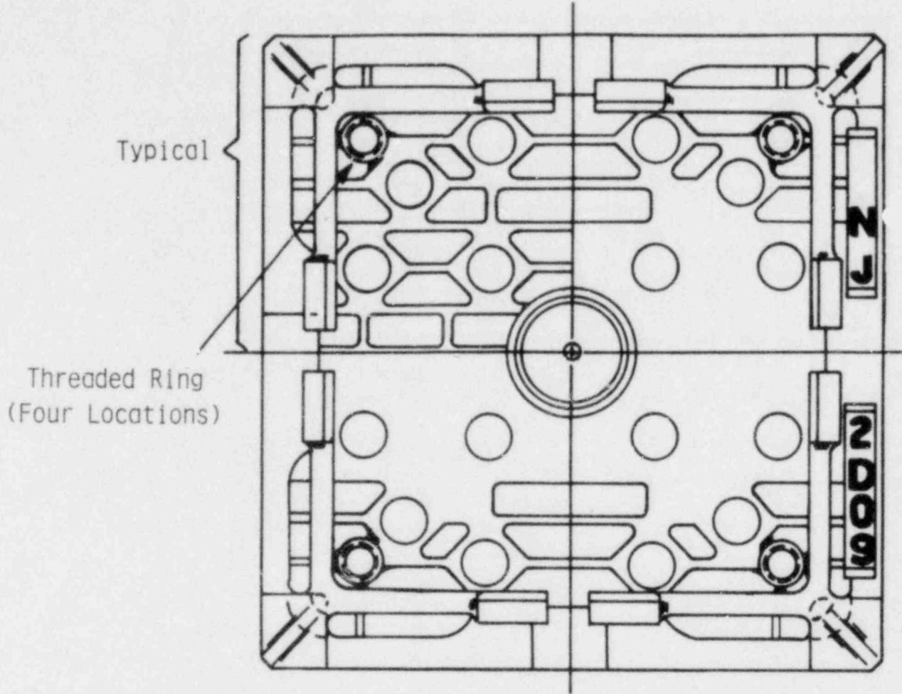
Figure 4-3. Removable Fuel Rod UEF Components
