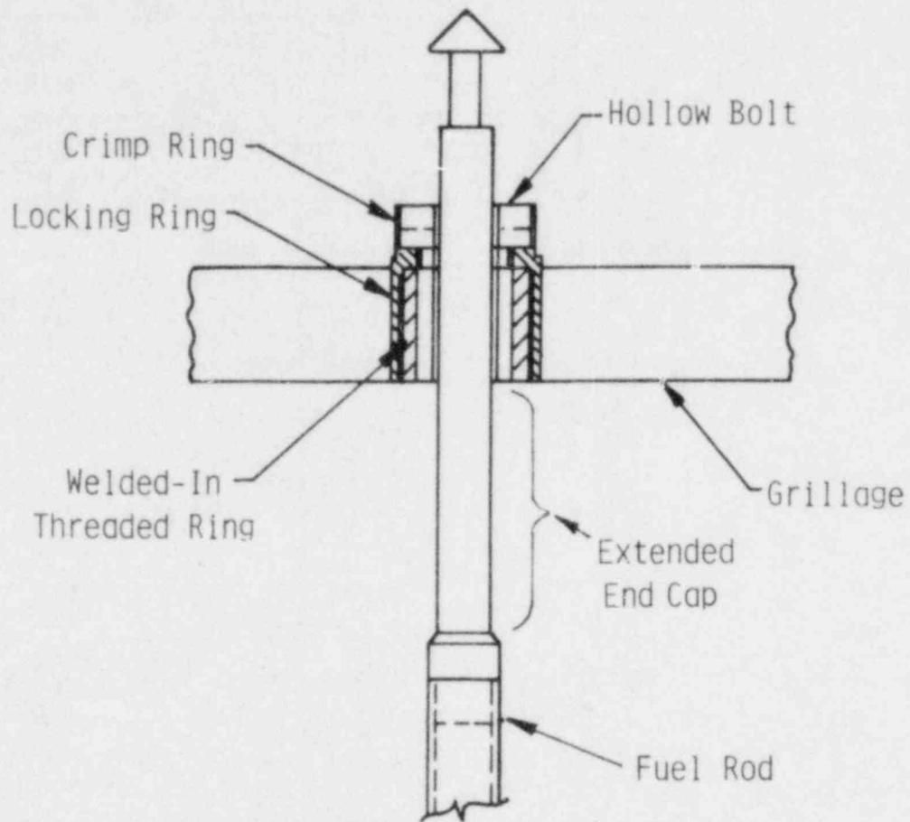
Figure 4-2. Removable Fuel Rod UEF Threaded Ring
