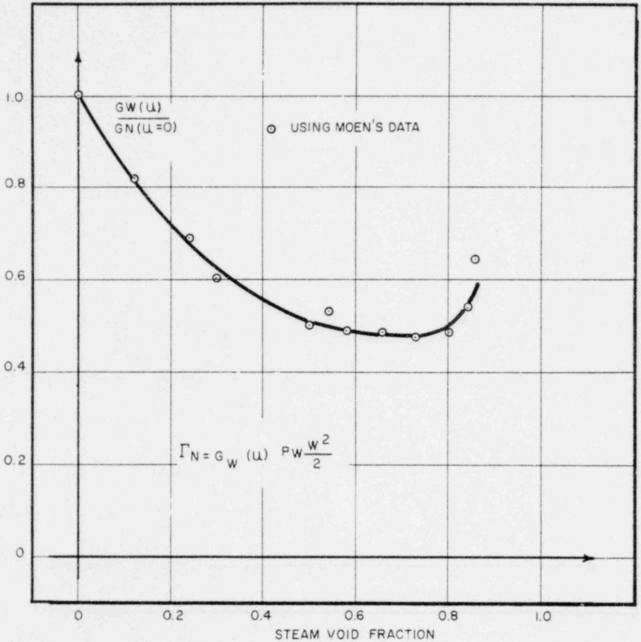
DEPENDENCE OF WATER-PIPE FRICTION PRESSURE DROP ON VOID FRACTION
