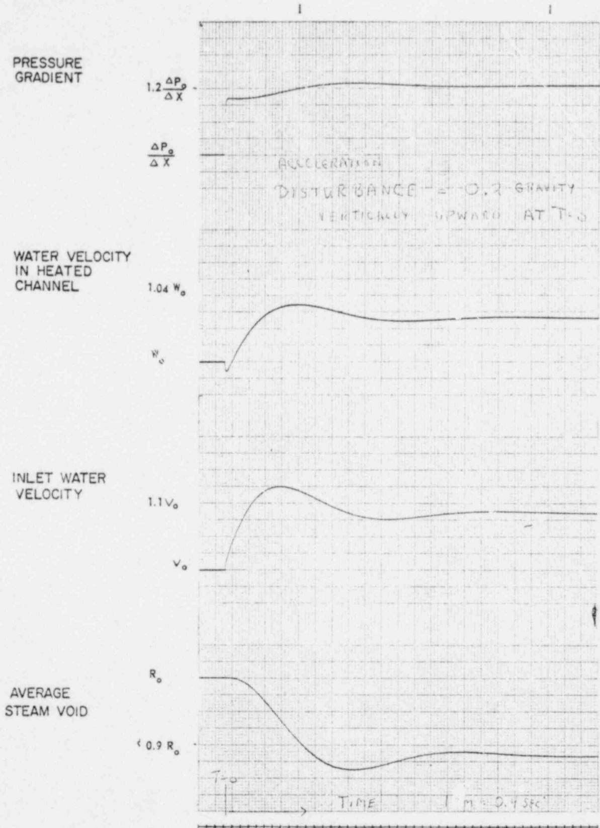
FIGURE 13 FLOW TRANSIENT CAUSED BY ACCELERATION
