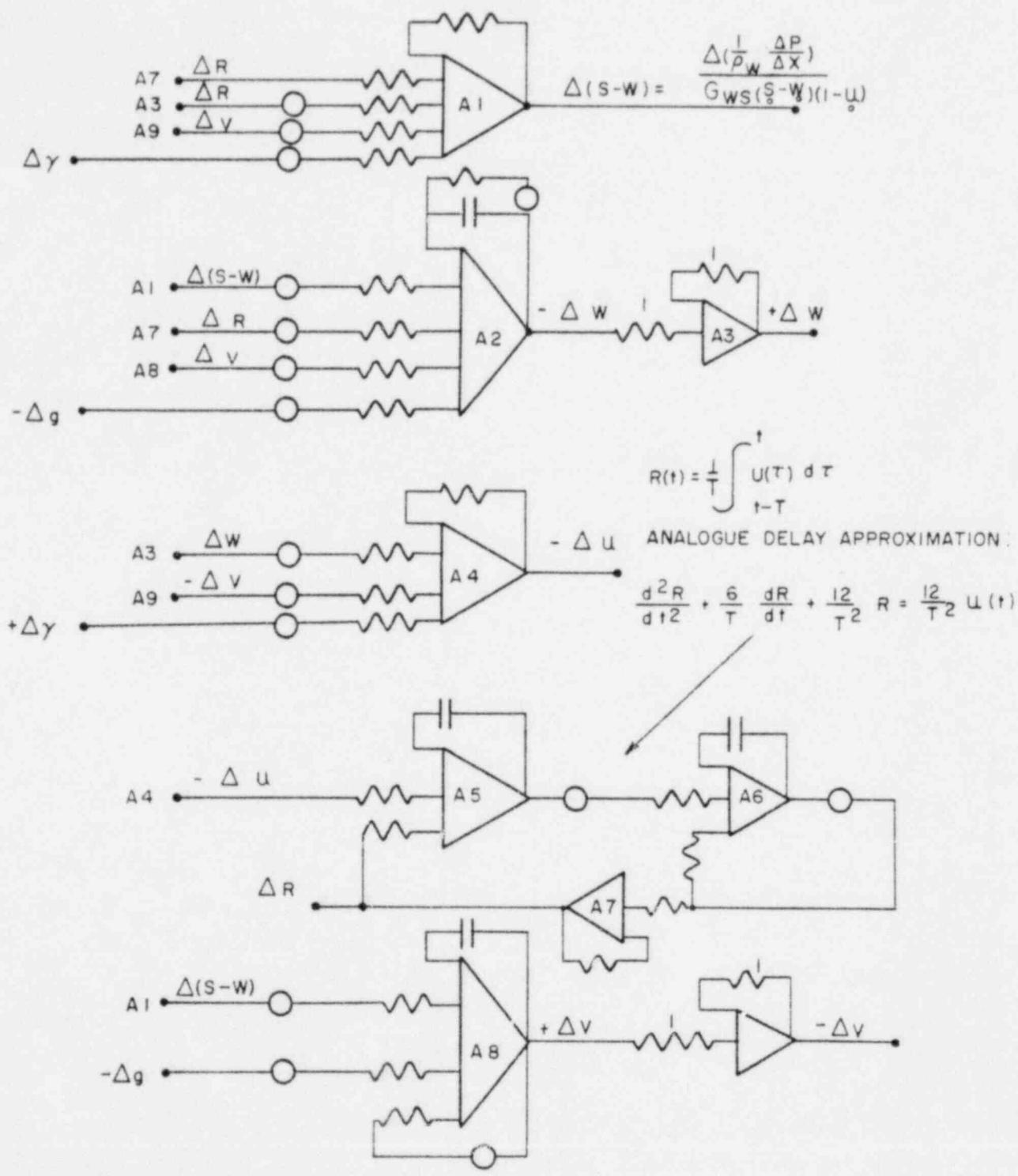
ANALOG COMPUTER CIRCUIT FOR TRANSIENT SOLUTION OF LOOP DYNAMICS
