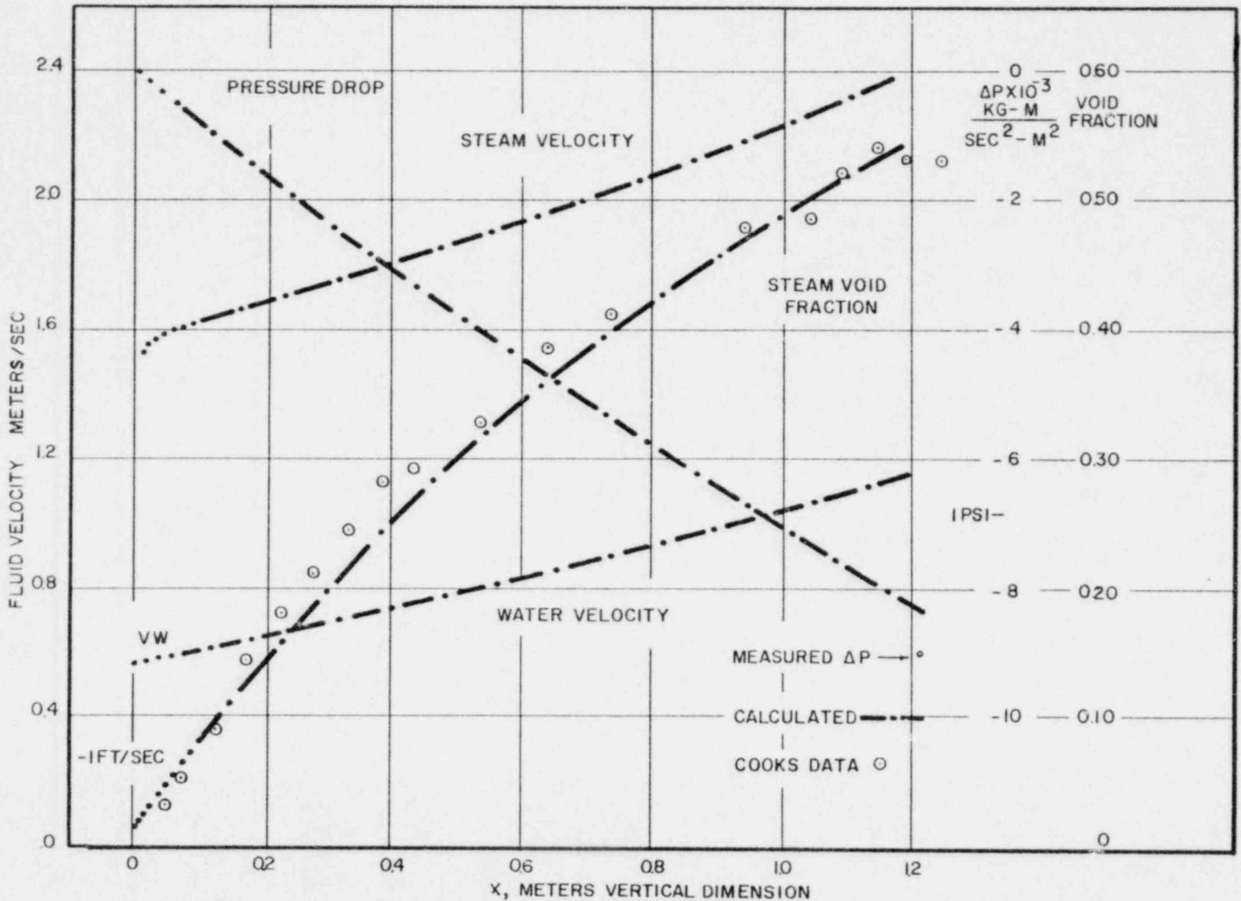
COMPARISON OF MEASURED AND EXPERIMENTAL VOID FRACTION OF COOK'S RUN 445
