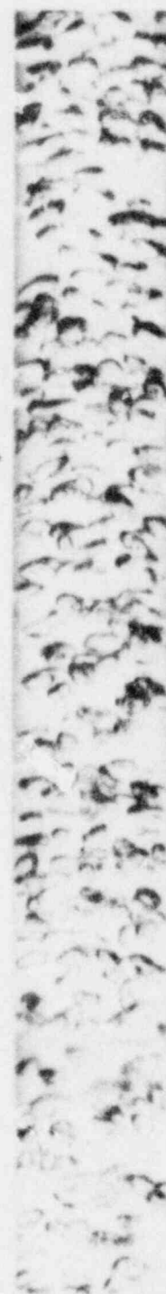
Figure 4.7 A photograph (a), diameter PDF (b), and diameter PSD (c), for 13 percent area-averaged void fraction, U_L = 0.25 m/sec, U_g = 0.073 m/sec
