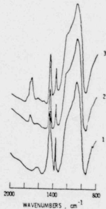
Figure 5. Infrared spectra of ethylene propylene rubber insulation. Curve 1 - unaged material. Curve 2 - aged in air at 1.2 Mrad/hr. Curve 3 - aged in air at 9.3 krad/hr.
