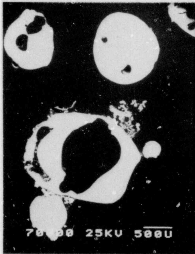
Figure 3.5-3 Fragments From FRAG 4 Showing Internal Voids 25X BEI
