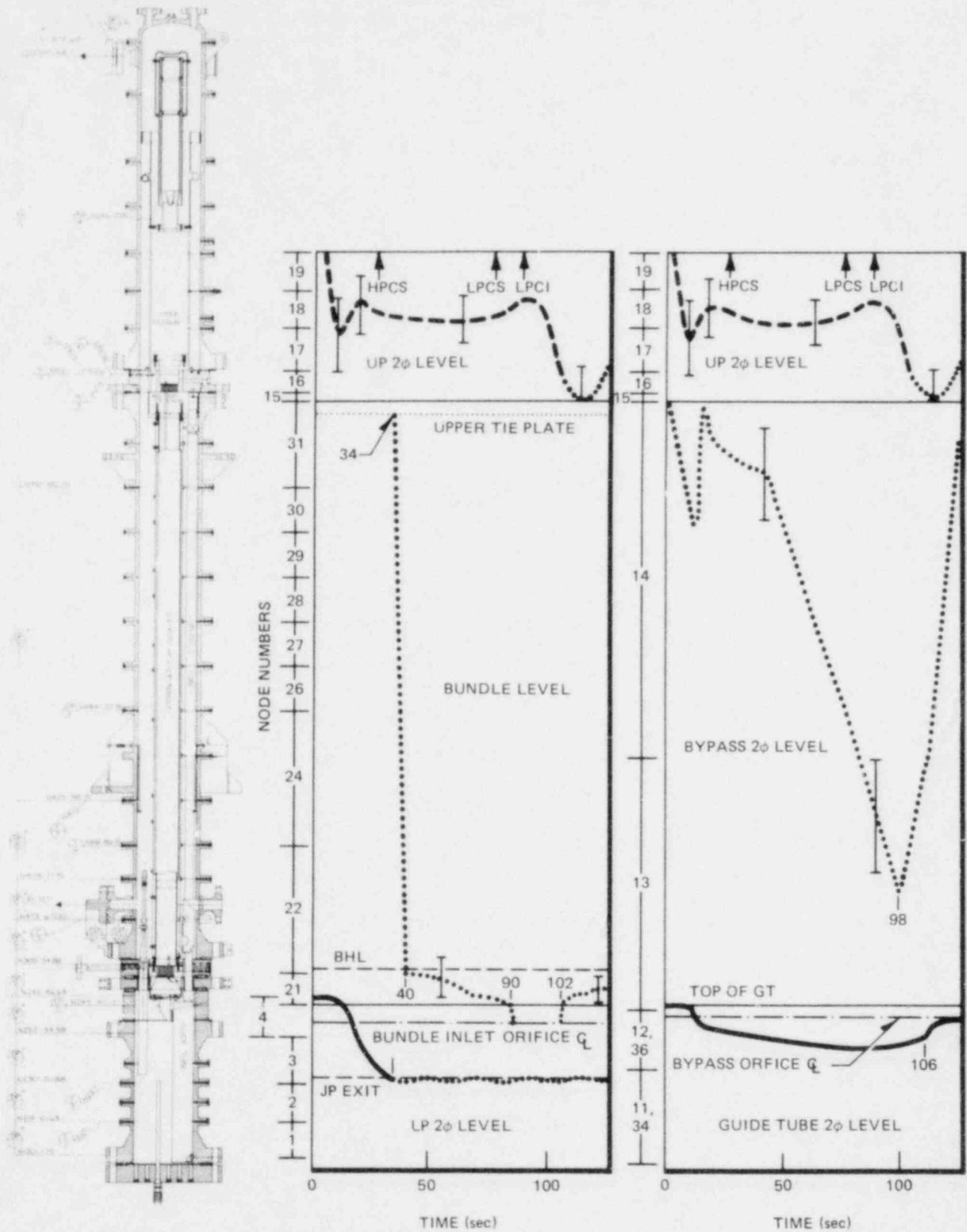
Figure C-5. Two-Phase Mixture Level Responses for the Reference Test (6406 Run 1, Average Power, Average ECC)
