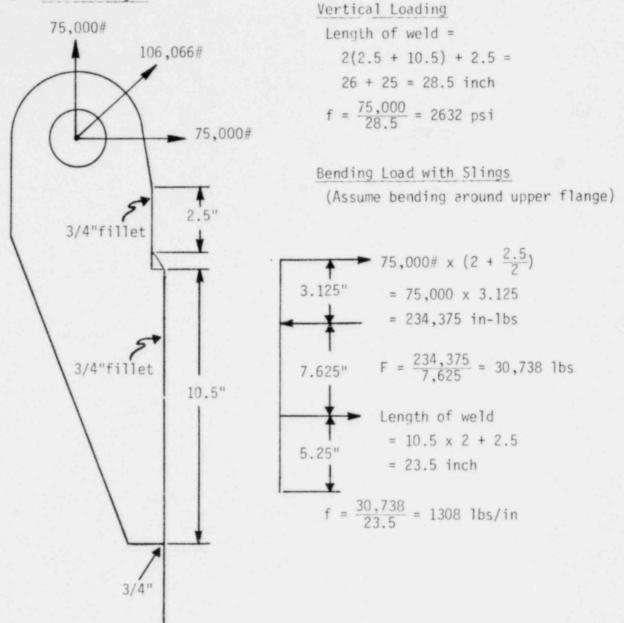
Combined stress  $\sqrt{2632^2 + 1308^2} = 2939$  psi Allowable stress 3/4" weld = 7200 x 0.85 = 6120 lbs/in Safety Factor =  $\frac{6120}{2939} = 2.08$  5) Bearing Stress in Hole
