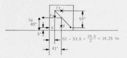
$$\begin{split} \Sigma M_b &= 0 \\ 5(W) \times (40-6) &= W \times 41 + F_t \times 59 + F_v \times 14.25 \\ &= \frac{F_v}{F_t} &= \frac{59}{60.5} \\ &= F_t = \frac{60.5}{59} \times F_v = 1.025 \ F_v \\ (170 - 41)(W) &= 59 \times 1.025 \times F_v + 14.25 \ F_v \\ F_v &= \frac{129 \times 50,000}{74.725} &= 86,316 \\ F_v \text{ each cable} &= \frac{86,312}{2} &= 43,158 \\ \text{Tension due to 5g transverse load} &= 43,158 \times \frac{97.68}{59} = 71,492 \end{split}$$
