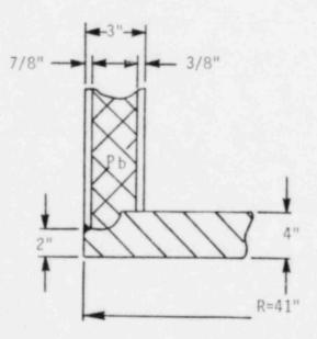
At an impact angle of  $45^{\circ}$  the steel corner will be deformed in the shape of an ungula and the volume of the deformation is determined by the following equation:
