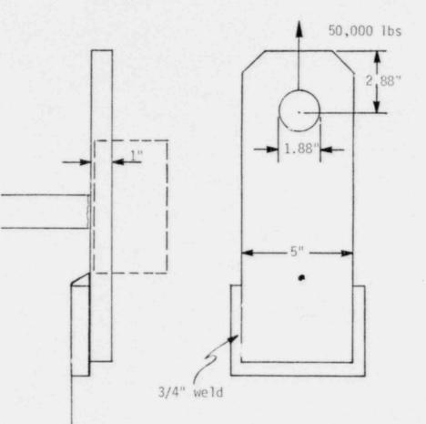
1. <u>Tension Stress</u> Load =  $\frac{50,000 \times 3}{3}$  = 50,000# min. area = (5 - 1.88) x 1 = 3.12 in<sup>2</sup> stress =  $\frac{50,000}{3.12}$  = 16,025 #/in<sup>2</sup> safety factor =  $\frac{30,000}{16,025}$  = 1.87 2) Shear Due to Bolt Load
