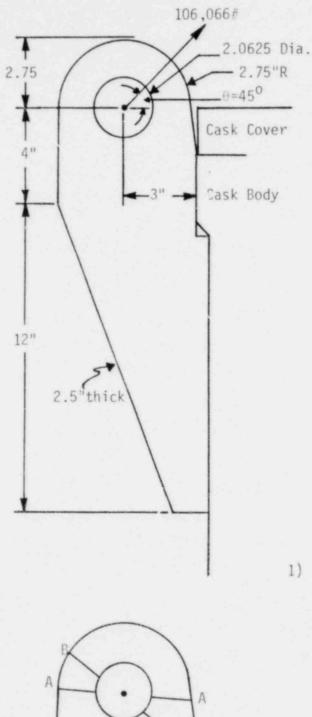
Weight of cask = 50,000 lb Number of lift lugs = 2 Vertical load per lug =  $\frac{50,000 \times 3}{2} = 75,000 \text{ lb}$
