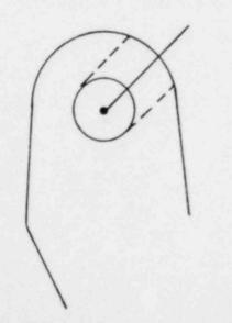
Area =  $2 \times 2.75 \times 2.5 = 13.75 \text{ in}^2$ Stress =  $\frac{106,066}{13.75}$  = 7714 psi Yield Strength Shear = 0.6 x 30,000 = 18,000 psi
