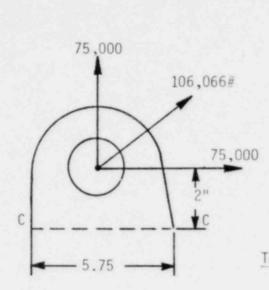
Bending Stress  $I_{c-c} = \frac{1}{12} bh^3$   $= \frac{1}{12} \times 2.5 \times 5.75^3$   $= 39.6 in^4$   $M = 75,000 \times 2 + 75,000 \times 0.125$  = 150,000 + 9375 = 159,375 in-1bs  $f_b = \frac{MC}{1} = \frac{159.375 \times 2.875}{39.6} = 11,571 psi$ Tensile Stress
