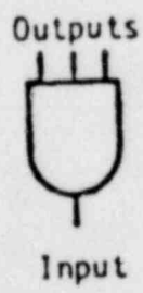
Figure A.9 (10) Symbols for Event Tree Segment of Cause-Consequence Diagram
