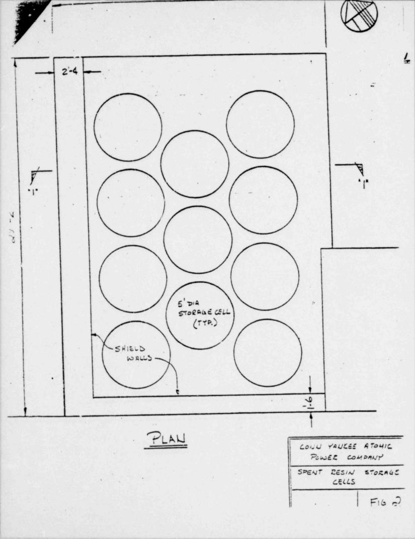
M009 SPENT RESIM STOCKER COUL YPULEE MONIC POUSE COMPANY 13,-0, 3-6 EXISTING GENDE GENDE -SHIELL WALLE 5' DIA STORNGE CELLIS (TYF.) SECTION 1-1" 29,-4" REMOUNDLE COVERS -TO EXISTING RESILL -EXISTING RESIN
